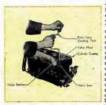
Method of grinding valve. (Cut No. 6)
