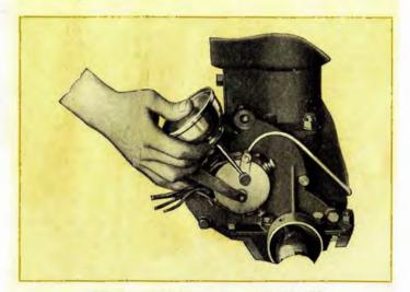
Oiling the Ford Commutator. (Cut No. 21)
