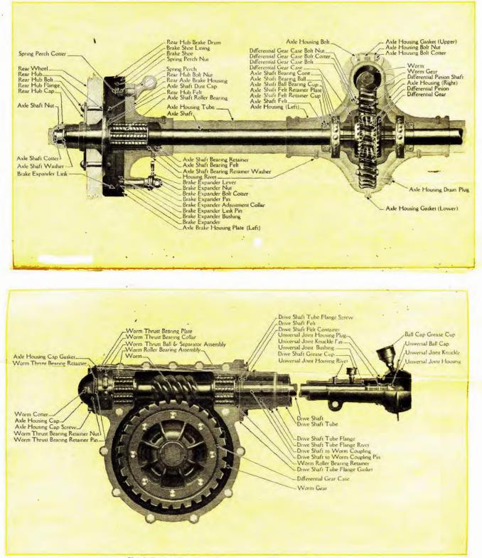
Truck Rear Axle Cross Section showing Worm and Worm Gear
