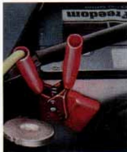
7. Don't let the other end touch metal. Connect it to the positive (+) terminal of the good battery. Use a remote positive (+) terminal if the vehicle has one.
