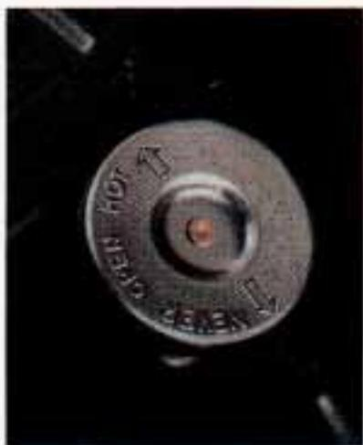
8. Then replace the pressure cap. Be sure the arrows on the pressure cap line up like this.
