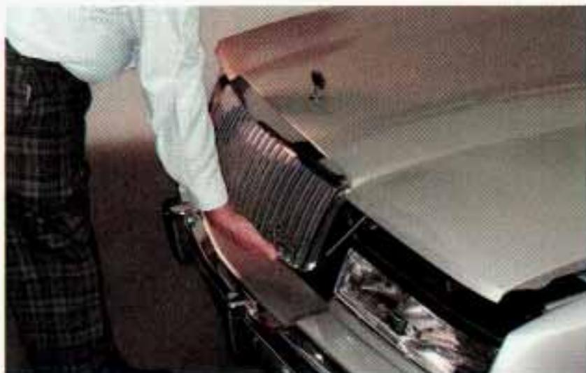
Then go to the front of the vehicle and locate the secondary hood release. It is located under the front edge of the grill.
