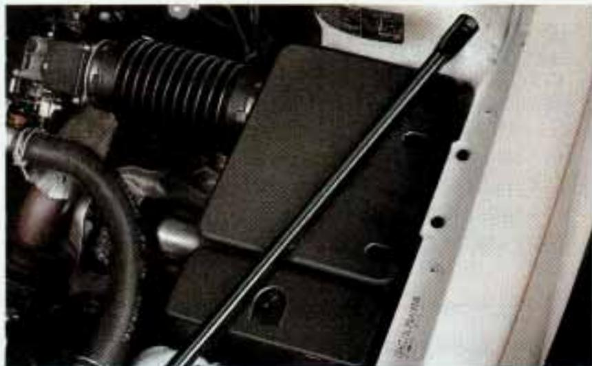
As you face the front of the vehicle, the air cleaner is in the front right section of the engine compartment. There is a filter inside the air cleaner.
