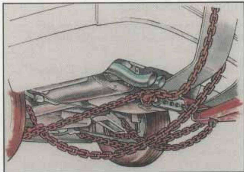
Position the lower sling crossbar just ahead of the front edge of the rear bumper. A 4" x 4" wood beam is not needed.
