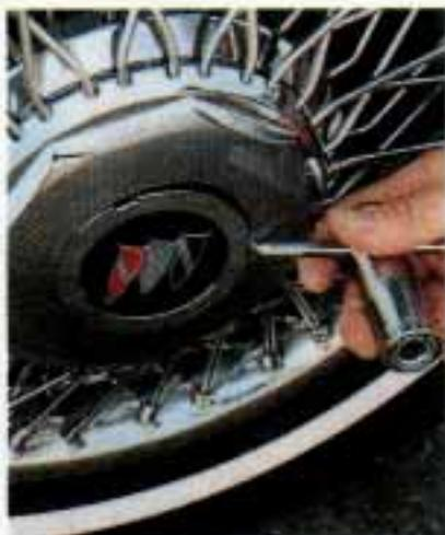
Put the flat end into the notch and carefully pry off the small cover.
