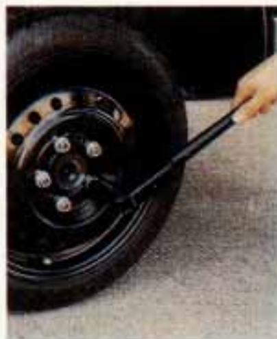
Tighten the wheel nuts firmly in a criss-cross sequence as shown.
