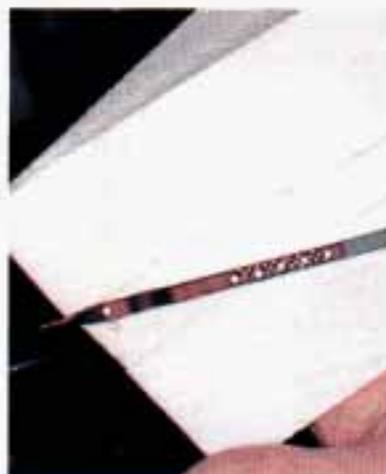
**To Check Engine Oil:** Pull out the dipstick and clean it with a paper towel or cloth, then push it back in all the way. Remove it again, keeping the tip lower.
