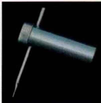
To remove the wire wheel cover, remove the center of the wheel cover by using the wire wheel key wrench.
