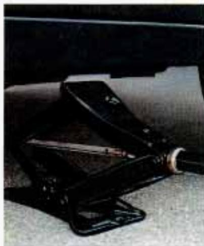
Position the jack under the vehicle. There is a notch in the frame near each of the wheels. Fit the lift head of the jack into the notch nearest the wheel with the flat tire.
