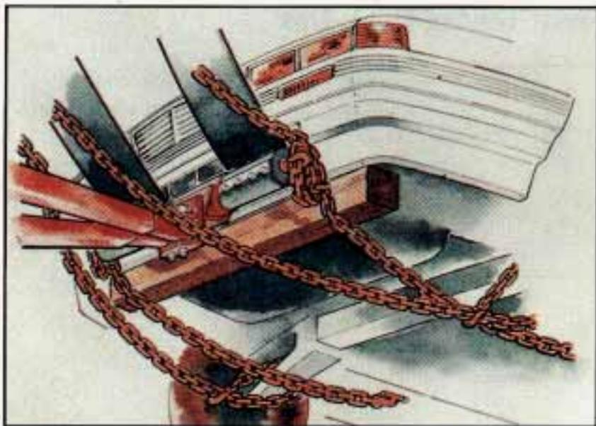
Position a 4" x 4" wood beam across the sling chains contacting the forward extensions of the engine cradle.
