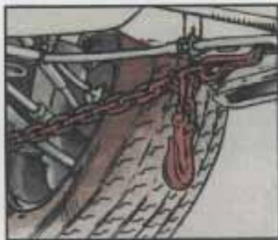
Attach "T" hook chains to the slots in the bottom of the floor pan just ahead of the rear wheels on both sides.
