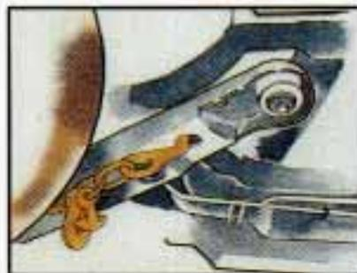
Attach "T" hook chains behind the front wheels into the bottom of slots of the cradle rails on both sides.
