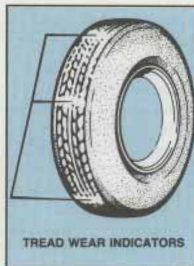
One way to tell when it's time for new tires is to check the treadwear indicators, which will appear when your tires have only 2/32 inch (1.6 mm) or less of tread remaining.
