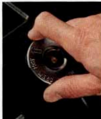
1. You can remove the radiator pressure cap when the cooling system, including the radiator pressure cap and upper radiator hose, is no longer hot.
