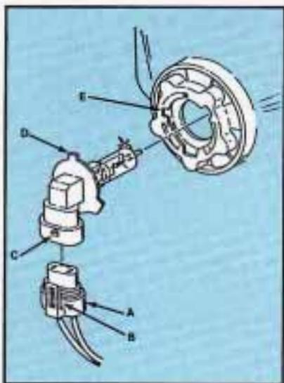
To reassemble: Attach the wire connector (A) to the plastic base making sure the lock tab (B) is over the lock (C). Install the bulb by putting the small tab (D) in the small notch in the lamp (E). Turn the bulb socket 1/4 turn clockwise to lock into place. Replace the access cover.
