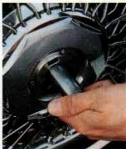
Remove the lock nut by inserting the key wrench into the hole in the center of the wheel cover and turn it clockwise to loosen the lock nut completely.
