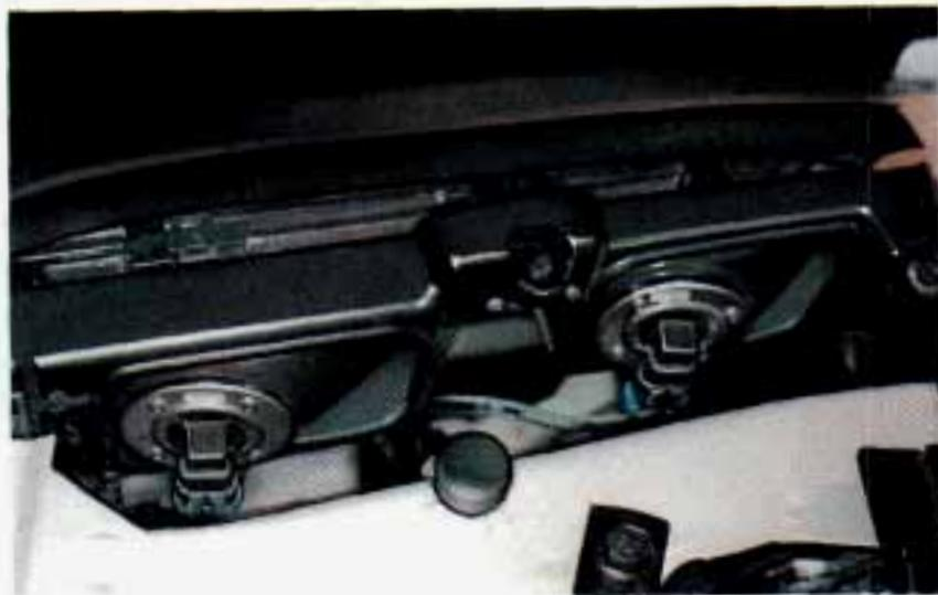
The bulb socket can be accessed, turn the bulb socket 1/4 turn counter-clockwise, while pressing it firmly.
