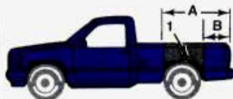
1. Recommended location for cargo center of gravity for cargo weight rating (Pickup Truck).
