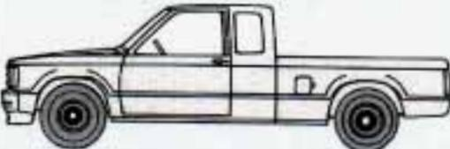
A line drawing of a club coupe/extended cab pickup truck, shown from a side profile. It has a two-door cab with a longer wheelbase and a standard bed, providing more interior space than the regular cab. | <b>CLUB COUPE/EXTENDED CAB</b> |
