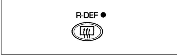
The button that controls the rear window defroster and heated side view mirrors
