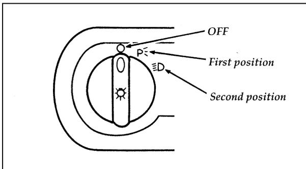
The knob for the headlamps, parking lamps, license plate lamps and tail lamps
