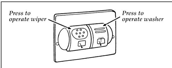
The liftgate window wiper and washer switches
