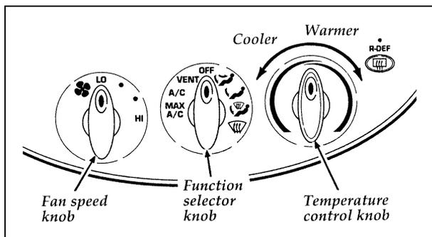
The knobs that control the manual heating and air conditioning system
