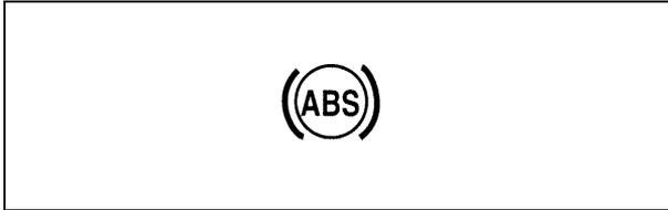
Anti-lock brake system warning light
