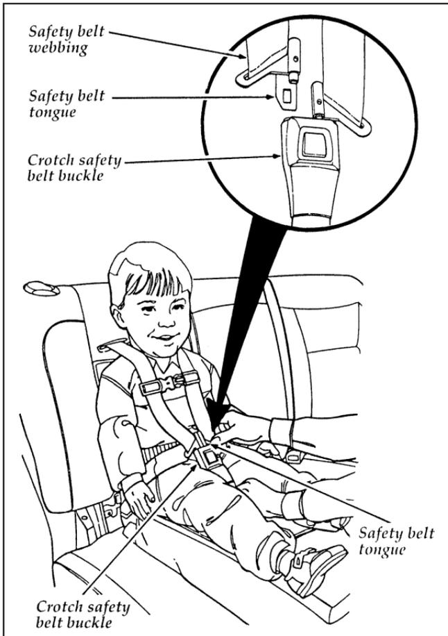
**Figure 6: Fastening the crotch safety belt buckle**
