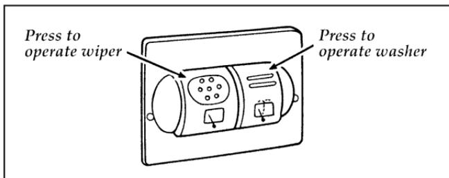
The liftgate window wiper and washer switches
