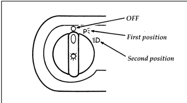
The knob for the headlamps, parking lamps, and tail lamps
