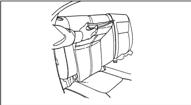
**Figure 2: Releasing the latch**
