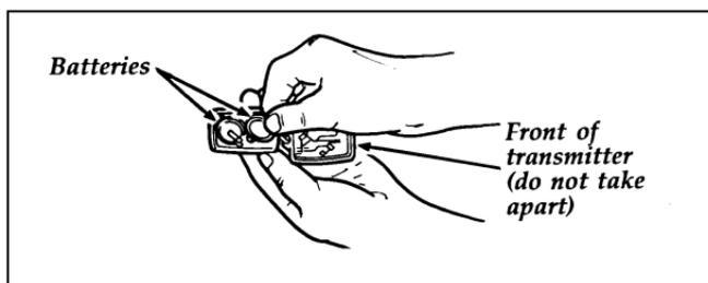
**Replacing the batteries**
