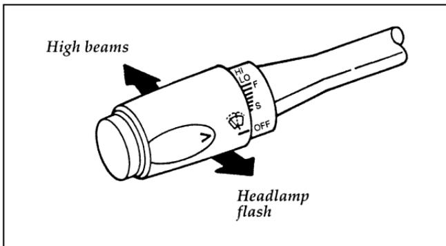
Turning on the high beams
