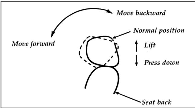
**Adjusting the four-way head restraint**
