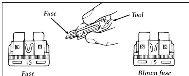
Fuse puller tool and fuse
