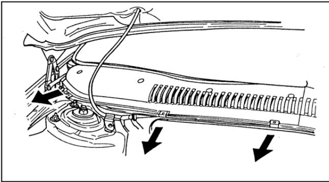
Removing the vacuum hose clips
