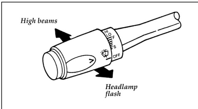
Turning on the high beams
