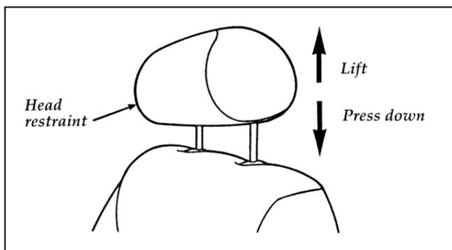
Adjusting the standard head restraint
