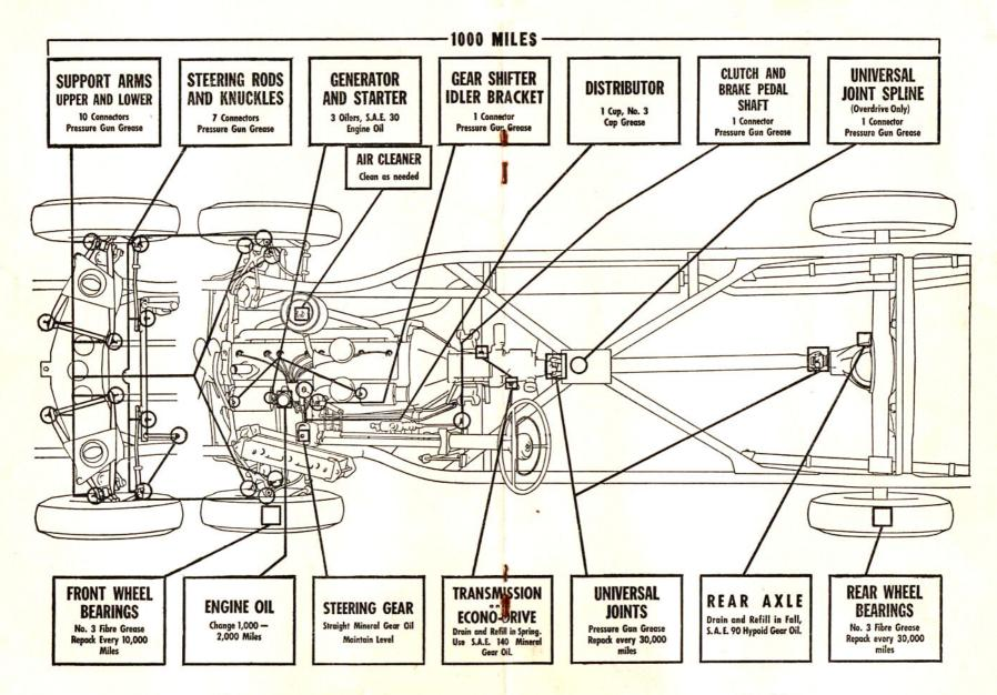
S.A.E. 80 Hypoid Lubricant should be used in localities where the temperature drops 10° or more below zero for long
