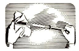
Changing Crankcase Oil—Under normal driving conditions, draining the crankcase and replacing with fresh oil every 1000 to 2000 miles is recommended
