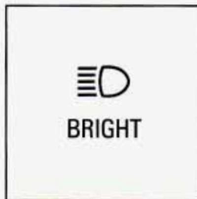
To change the headlights from low beam to high or high to low, pull the turn signal lever all the way toward you. Then release it. When the high beams are on, this blue light on the instrument panel also will be on.
