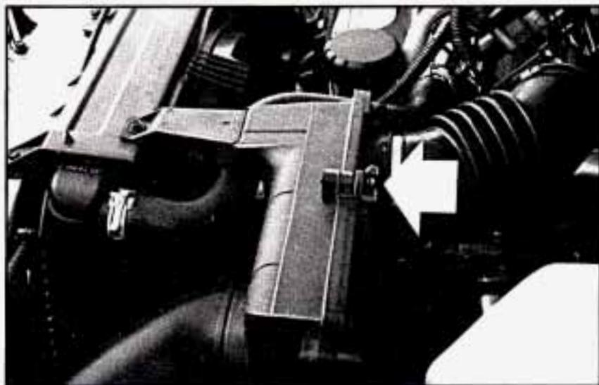
The air cleaner and filter are located on the driver's side of the engine compartment. To check or replace the filter, undo the wing screws and pull the air cleaner open. Replace the filter, then close the cover and tighten the wing screws.
