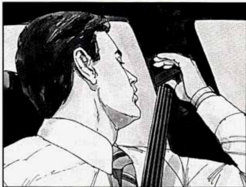
To move it up or down, squeeze the release handle. When you release the handle, try to move it down a little to make sure it has locked into position.
