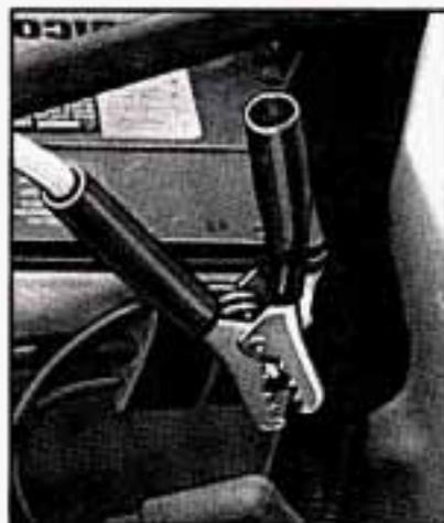
8. Now connect the black negative (-) cable to the good battery's negative (-) terminal.
