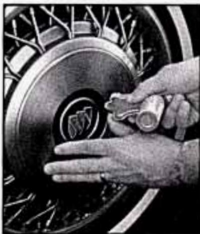
Using the flat end of the key wrench handle, between the wire wheel cover and the center cap, pry off the center cap.
