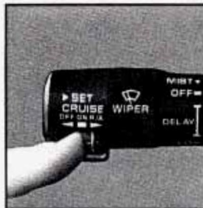
1. Move the Cruise switch from "ON" to "Resume/Accelerate." Hold it there until you get up to the speed you want, and then release the switch.
