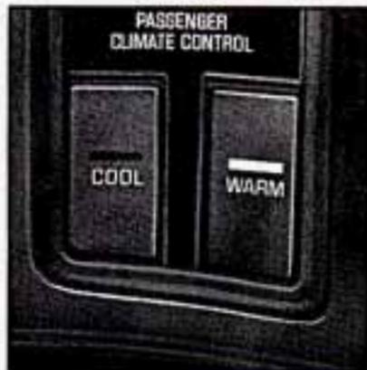
The right front seat passenger can activate the dual zone function by pressing the WARM or COOL buttons on the passenger door.
