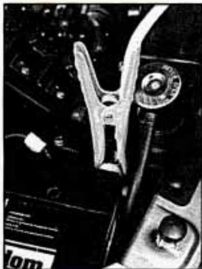
6. Connect the red positive (+) cable to the positive (+) terminal of the vehicle with the dead battery. Use a remote positive (+) terminal if the vehicle has one.
