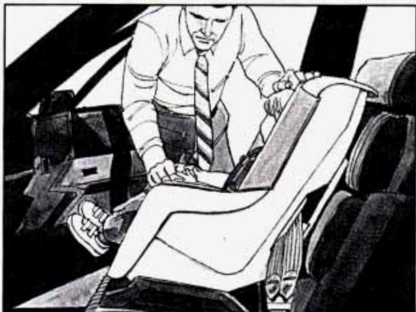
8. Push and pull the child restraint in different directions to be sure it is secure.
