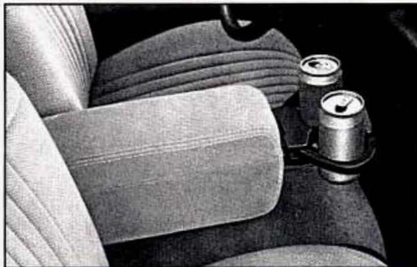
The armrest between the front seats opens into a storage area. To open it, press the lever at the front edge.
