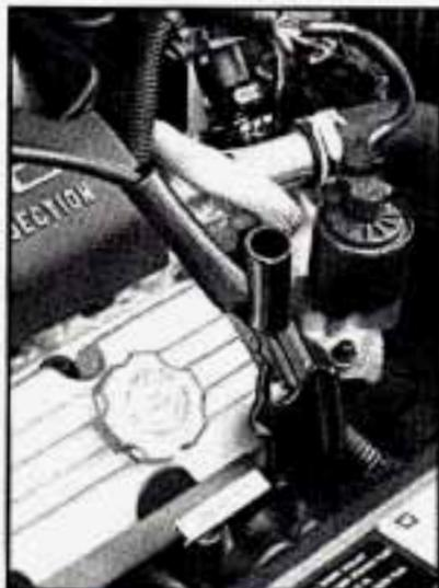
9. Attach the cable at least 18 inches (45 cm) away from the dead battery, but not near engine parts that move. The electrical connection is just as good there, but the chance of sparks getting back to the battery is much less.
