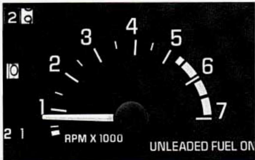
The tachometer tells you how fast the engine is going. It displays engine speed in thousands of revolutions per minute (RPM).
