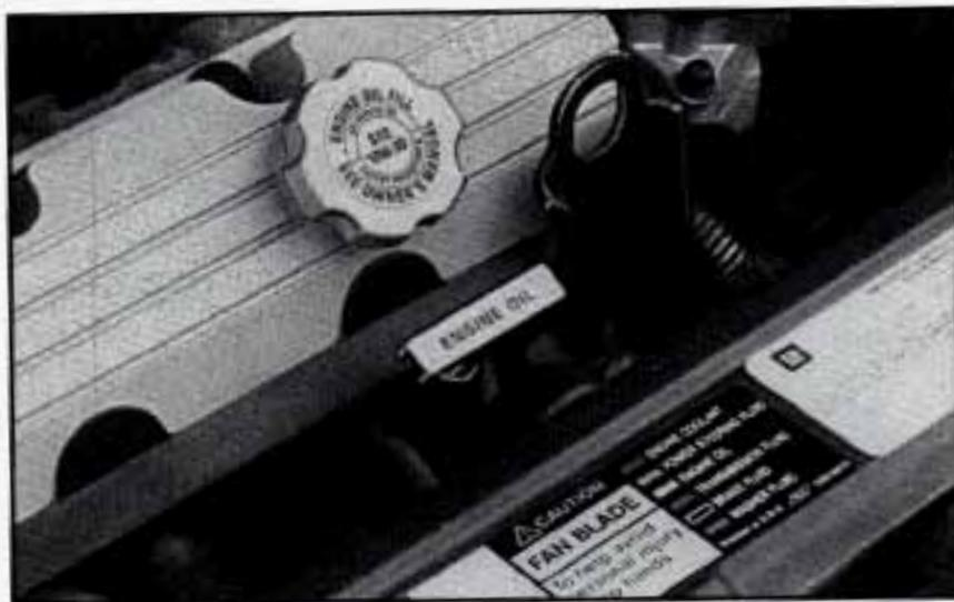
The engine oil dipstick is directly behind the engine fan. Turn off the engine and give the oil a few minutes to drain back into the oil pan. If you don't, the oil dipstick might not show the actual level.
