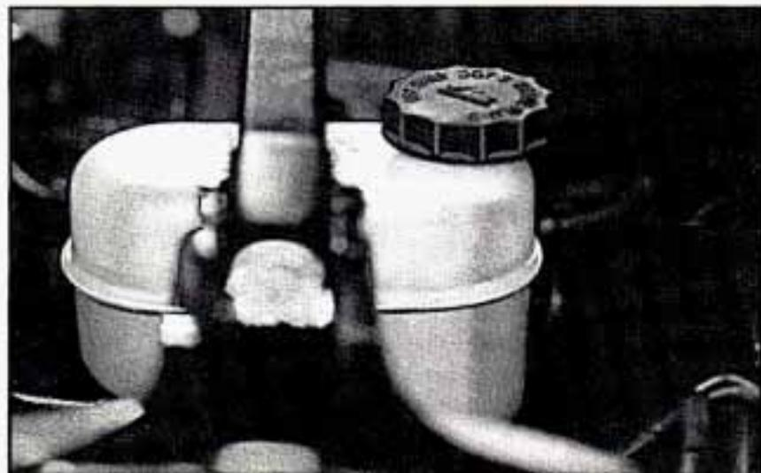
There are only two reasons why the brake fluid level in your master cylinder might go down. The first is that the brake fluid goes down to an acceptable level during normal brake lining wear. When new linings are put in, the fluid level goes back up. The other reason is that
