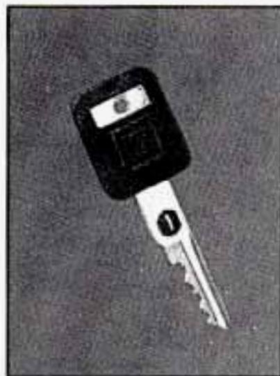
Your vehicle is equipped with the PASS-Key® II (Personalized Automotive Security System) theft deterrent system. PASS-Key® II is a passive theft deterrent system. This means you don't have to do anything different to arm or disarm the system. It works when you insert or remove the key from the ignition. PASS-Key® II uses a resistor pellet in the ignition key that matches a decoder in your vehicle.
