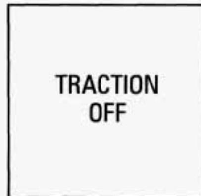
The "TRACTION OFF" warning light means that the system is not working. When this warning light is on, the system will not limit wheel spin. Adjust your driving accordingly.
