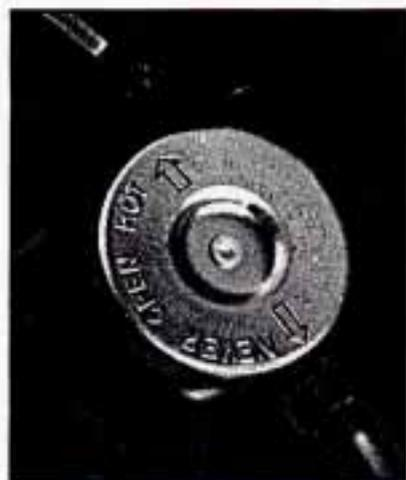
8. Then replace the pressure cap. At any time during this procedure if coolant begins to flow out of the filler neck, reinstall the pressure cap. Be sure the arrows on pressure cap line up like this.
