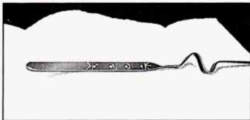
3. Check both sides of the dipstick, and read the lower level. The fluid level must be in the cross-hatched area.
