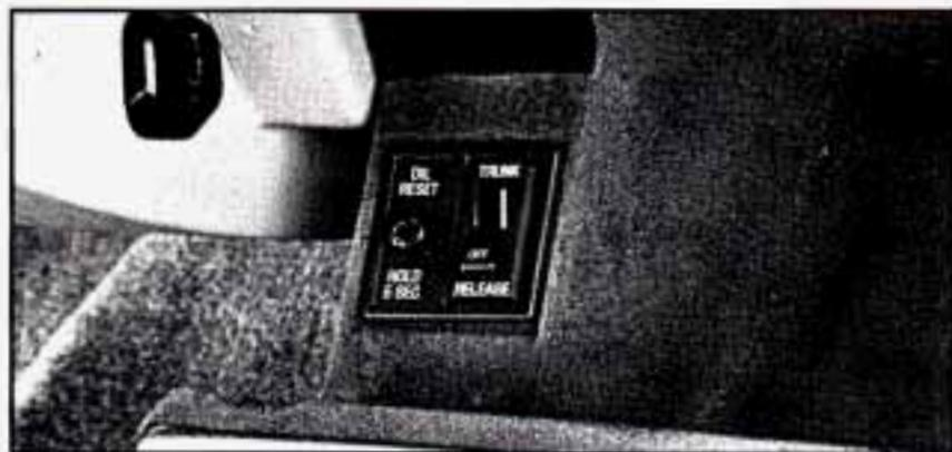
The reset button is in the glove box. With the ignition key in the RUN position, push the reset button, hold it in for at least 5 seconds but not more than 60 seconds. After 5 seconds, the "Change Oil Soon" light will flash 4 times and then go off. This indicates that the Oil Life Monitor System has been reset.
