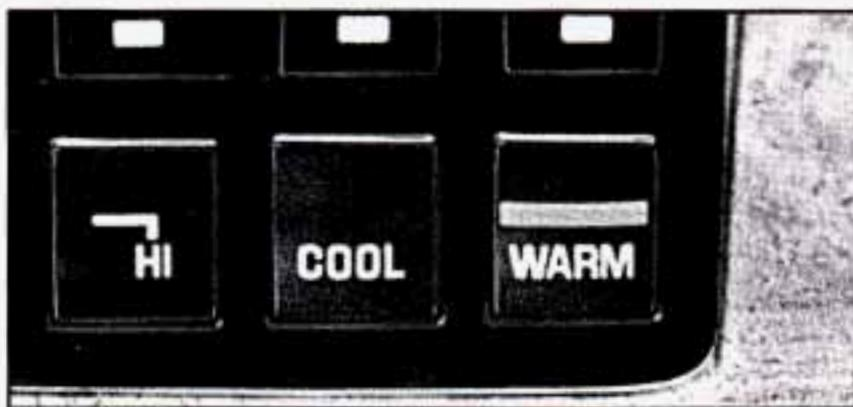
To adjust the temperature to a comfortable level, push either COOL or WARM.
