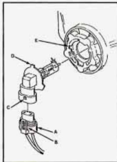
Turn the bulb socket 1/4 turn counter-clockwise, while pressing it firmly.
