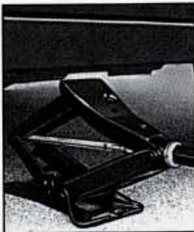
Position the jack under the vehicle. There is a notch in the frame near each of the wheels. Fit the top of the jack into the notch nearest the wheel with the flat tire.
