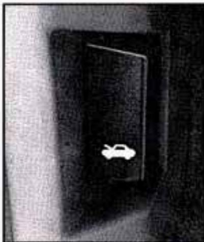
To open the hood, first pull the handle inside the vehicle. It is located on the lower left side of the instrument panel, next to the parking brake. When you pull this handle the hood latch will release.
