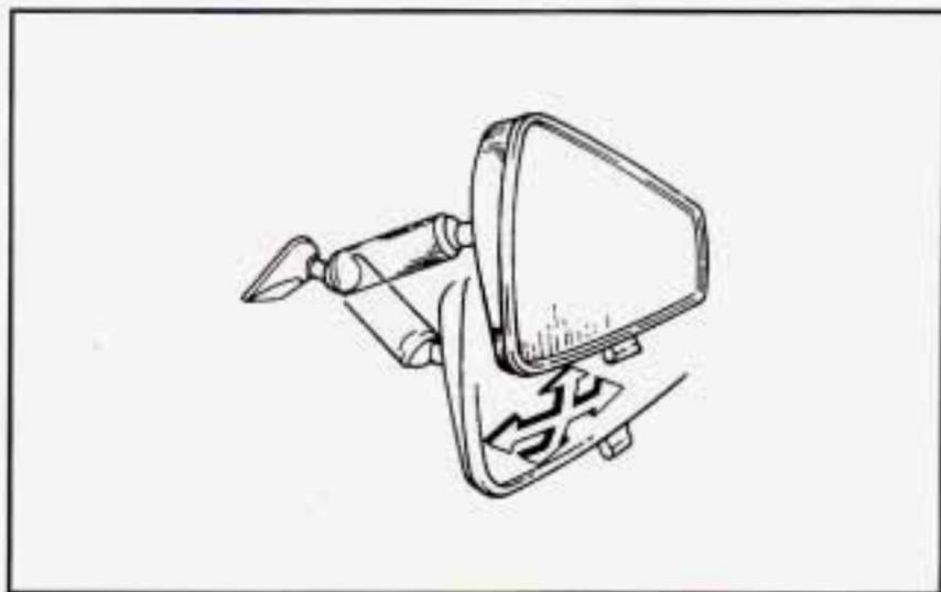
The mirror mount is designed to detach during air bag deployment. Excessive force and/or excessive up, down, side-to-side adjustment can cause the mirror to detach from the windshield. If this occurs, re-install the mirror according to this procedure.
