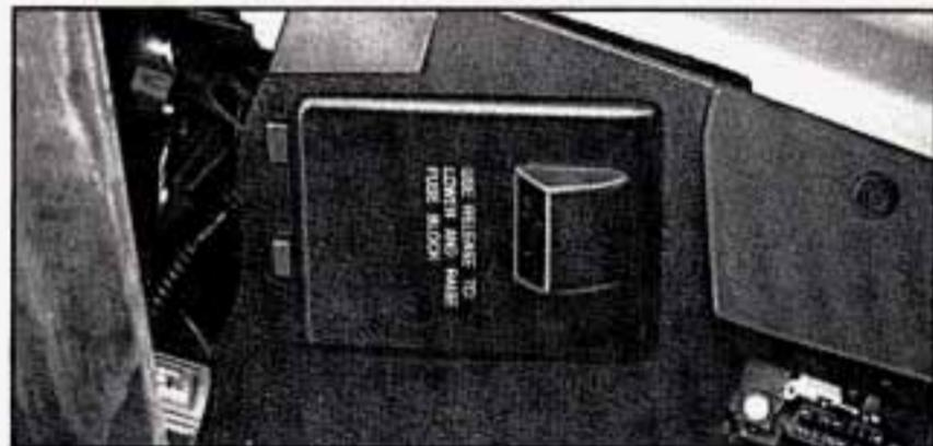
Remove the cover to access the fuses. To put the cover on, insert the tabs into the lower part of the fuse panel and snap it in place.
