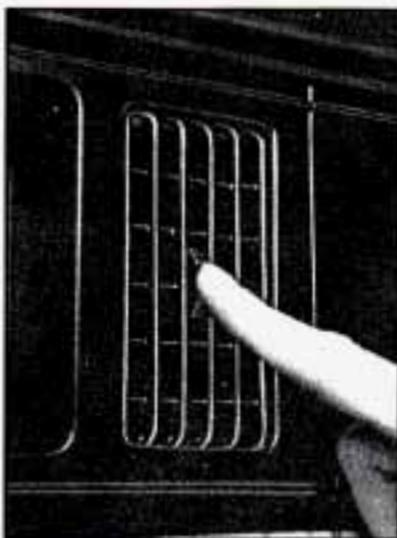
Adjust the direction of air flow by moving the louvered vents.
