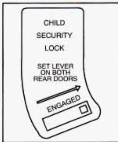
1. Move the lever all the way up to the ENGAGED position.
