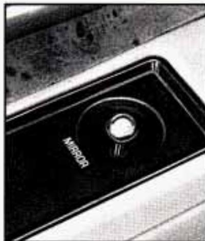
To adjust the left outside mirror, rotate the knob located on the driver's door. The right outside mirror must be adjusted manually.
