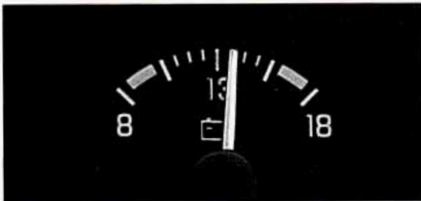
If you have the optional gage cluster, this gage shows voltage in the electrical system. The normal range is 11 to 15 volts. If the gage reading stays in either red range, have your Buick dealer check the electrical system.
