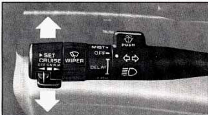
The turn signal has two upward (for Right) and two downward (for Left) positions. These positions allow you to signal a turn or a lane change.
