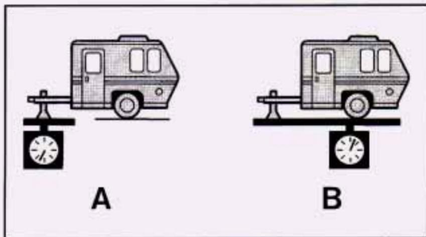
If you're using a "dead-weight" hitch, the trailer tongue (A) should weigh 10% of the total loaded trailer weight
