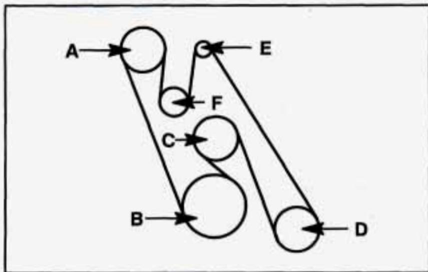
The 3800 (L27) engine uses an engine accessory belt. This diagram shows the features connected by the belt routing. See "Maintenance Schedule" in the Index for when to check the belt.
