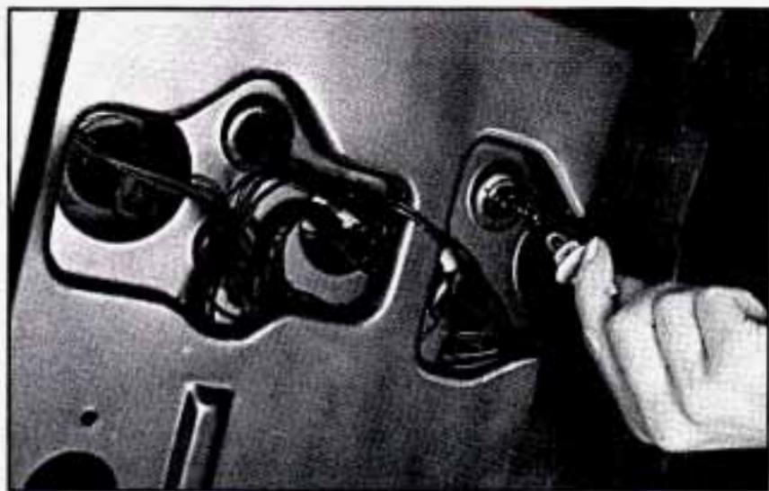
To replace the trunk lid taillamp bulbs, pull the bulb assembly straight out of the socket. Pull the bulb straight out of the assembly. Replace the bulb and reassemble.
