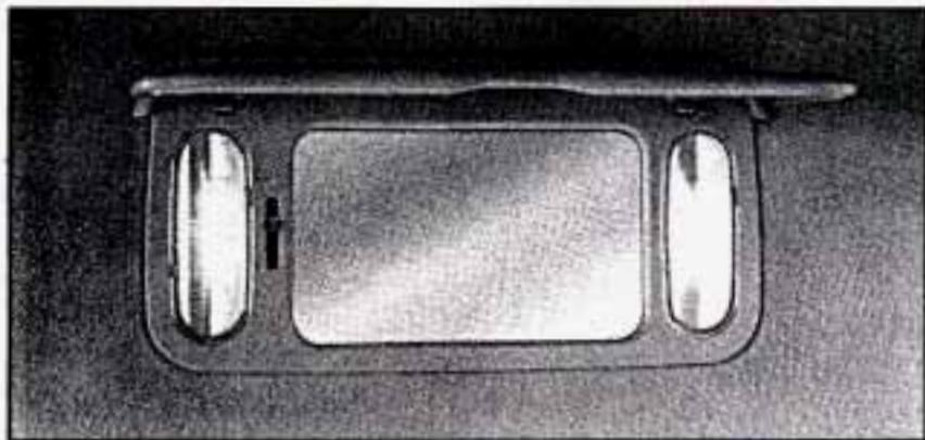
The brightness of the light can be adjusted by sliding the switch.
