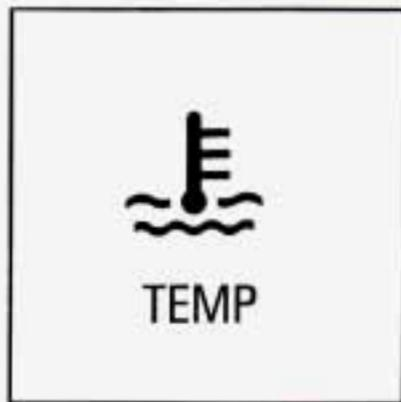
This light tells you that your engine coolant has overheated or your radiator cooling fans are not working. If you have been operating your vehicle under normal driving conditions, you should pull off the road, stop your vehicle and turn the engine off as soon as possible.
