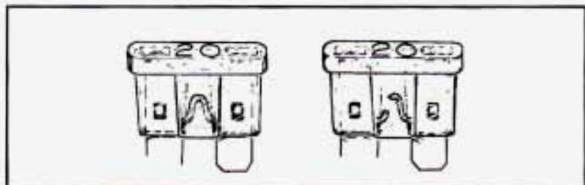
Look at the silver-colored band inside the fuse. If the band is broken or melted, replace the fuse. Be sure you replace a bad fuse with a new one of the identical size and rating.
