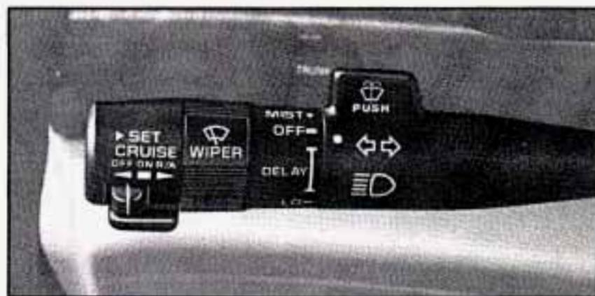
You control the windshield wipers by turning the band marked "WIPER."
