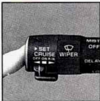
3. Push in the set button at the end of the lever and release it. (The "CRUISE" light on the instrument panel will come on.)
