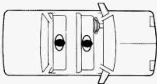
When you secure a child restraint in a center seating position, you'll be using the lap belt.
