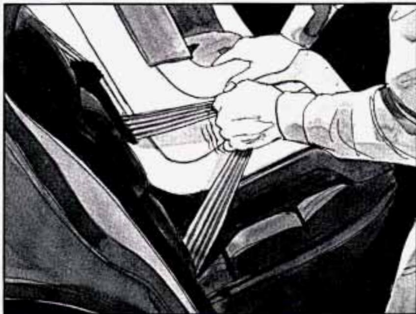
6. To tighten the belt, feed the lap belt into the retractor while you push down on the child restraint.
