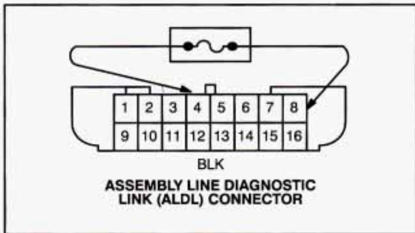
3. Use a jumper wire with alligator clips at both ends to ground (Terminal 4) to program (Terminal 8). Grounding the program terminal erases the system memory and causes the doors to lock and unlock once. This means the system is ready to be matched to the transmitter.
