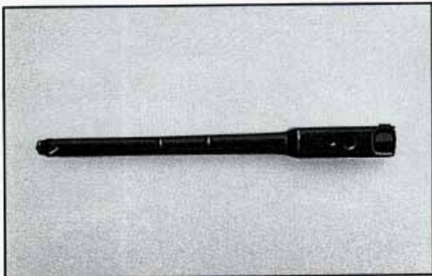
The jack handle has markings at 8" for the rear; 10" for the front to help you locate the jacking notches in the frame.
