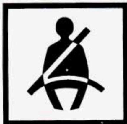
When the key is turned to “Run” or “Start,” a chime will come on for about eight seconds to remind people to fasten their safety belts. The safety belt light will also come on and stay on for about 70 seconds. If the driver’s belt is already buckled, neither the chime nor the light will come on.
