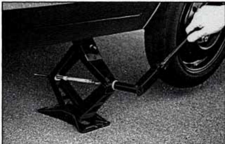
Raise the vehicle by rotating the wheel wrench clockwise. Raise the vehicle far enough off the ground so there is enough room for the spare tire to fit.
