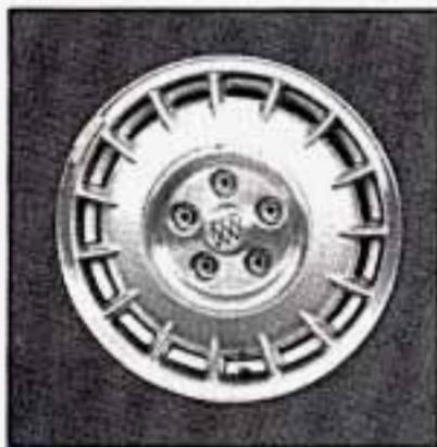
If your vehicle has this aluminum wheel, you may have plastic wheel nut caps. Use the wheel nut wrench to remove the wheel nut caps and to loosen the wheel nuts.
