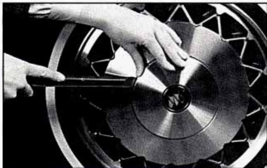
If your vehicle has an aluminum wheel with a center cover, remove it by using the flat end of the wheel wrench to access the wheel nuts.
