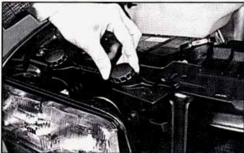
Each headlamp is attached by retainers with round plastic knobs. Remove the retainers by turning in a counter-clockwise direction.
