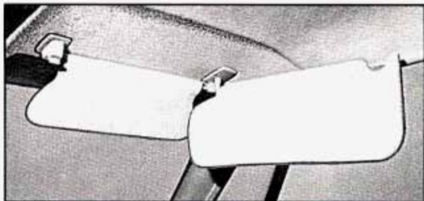
Each sunvisor has two parts, so that both the windshield and door glass can be shaded at the same time.
