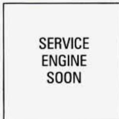
A computer monitors operation of your fuel, ignition and emission control systems. This light should come on when the ignition is on, but the engine is not running, as a check to show you it is working.
