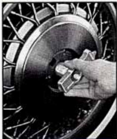
Remove the theft deterrent wheel nut, by placing the key end of the wire wheel key wrench over the nut and turning it to the left.
