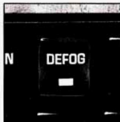
When the outside temperature is mild, use DEFOG to keep fog off the windshield.
