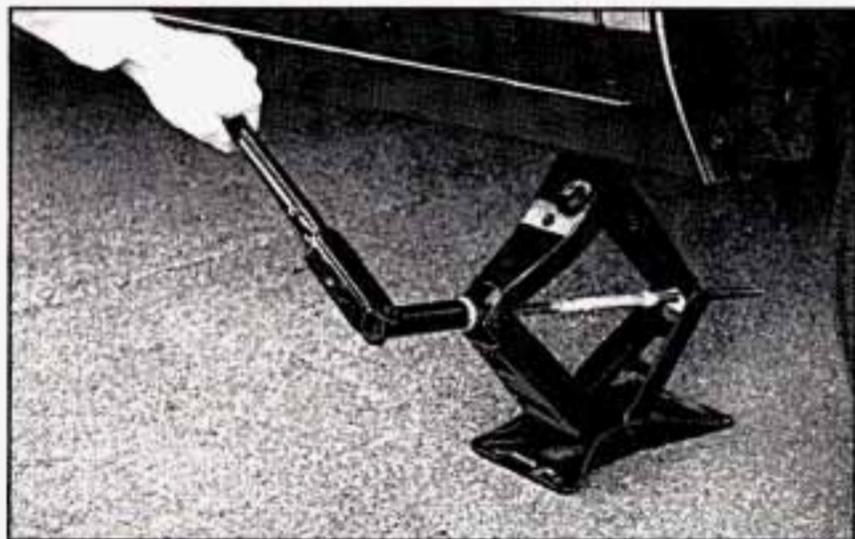
Lower the vehicle by rotating the wheel wrench counterclockwise. Lower the jack completely.
