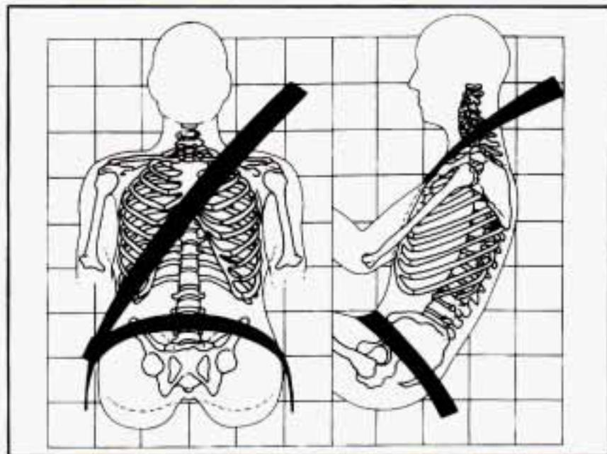
The lap part of the belt should be worn low and snug on the hips, just touching the thighs. In a crash, this applies force to the strong pelvic bones. And you'd be less likely to slide under the lap belt. If you slid under it, the belt would apply force at your abdomen. This could cause serious or even fatal injuries. The shoulder belt
