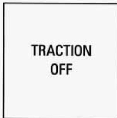
The “TRACTION OFF” warning light will come on when you turn the traction control system off.
