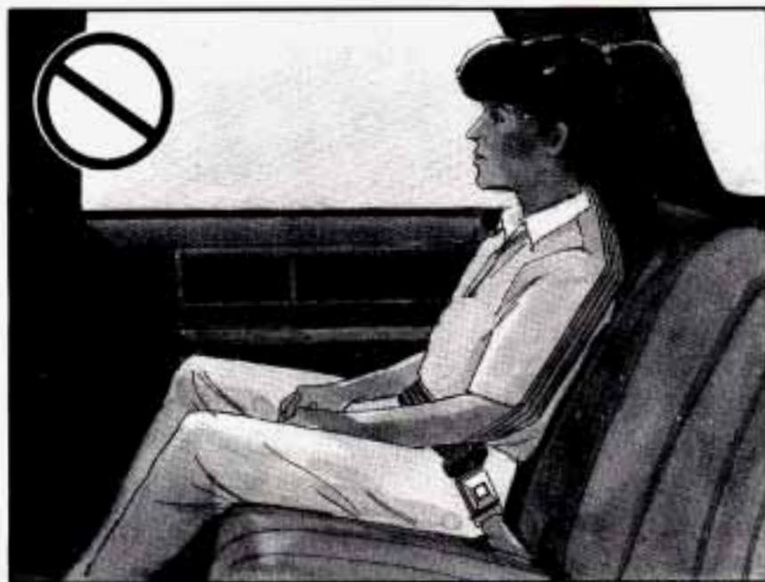
Wherever the child sits, the lap portion of the belt should be worn low and snug on the hips, just touching the child's thighs. This applies belt force to the child's pelvic bones in a crash.
