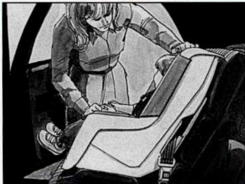
7. Push and pull the child restraint in different directions to be sure it is secure.
