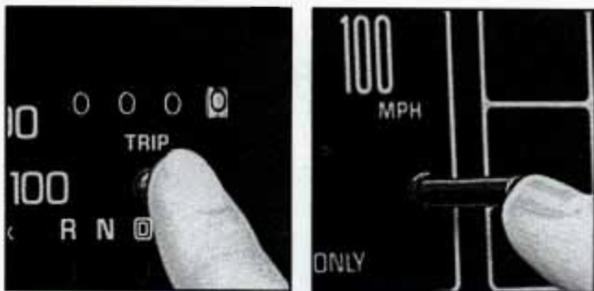
A trip odometer can tell you how many miles you have driven since you last set it to zero. To reset it, push the button.
