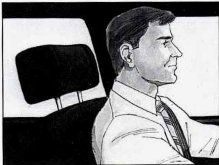
Slide the head restraint up or down so that the top of the restraint is closest to the top of your ears. This position reduces the chance of a neck injury in a crash.
