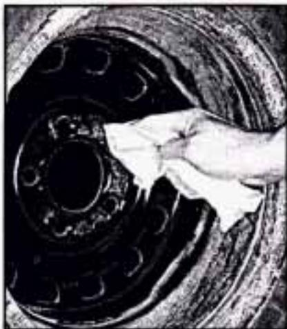
Remove any rust or dirt from the wheel bolts, mounting surfaces or spare wheel.
