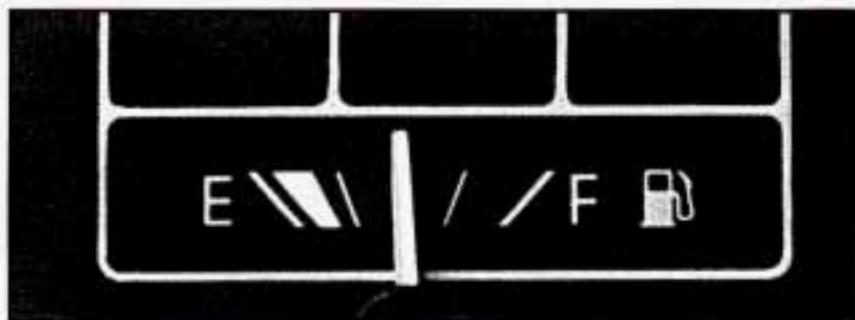
Your fuel gage shows about how much fuel is in your tank. It works only when the engine is on. When the indicator nears "E," you still have a little fuel left. You need to get more fuel right away.
