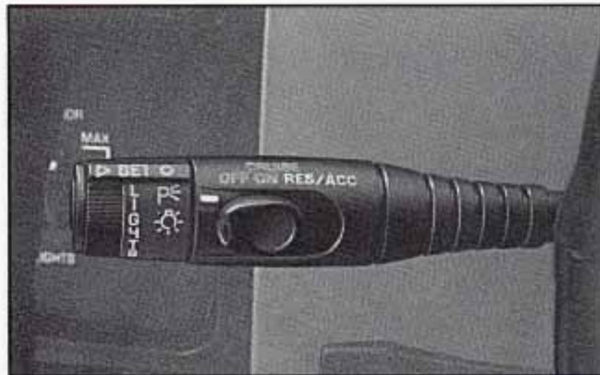
1. Move the Cruise switch from "ON" to "RES/ACC" Hold it there until you get up to the speed you want, and then release the switch.
