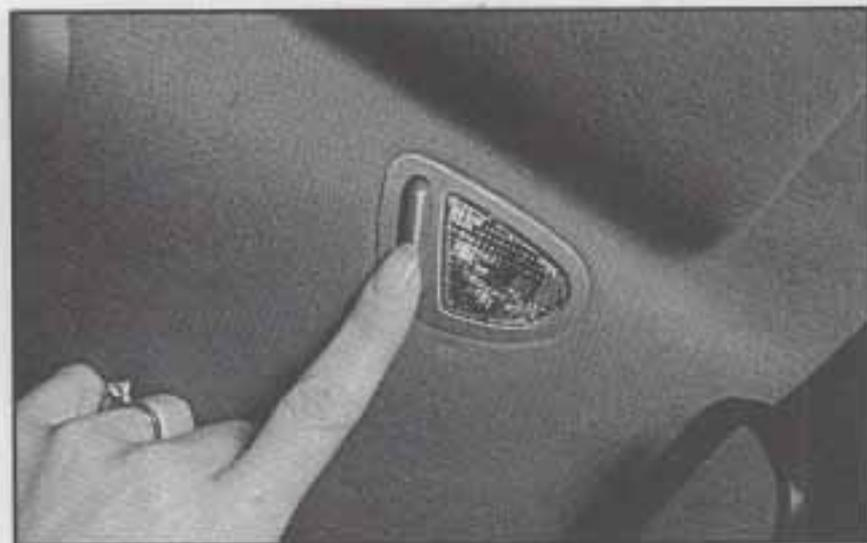
The front seat reading lights are turned on by pressing the switch next to the light.
