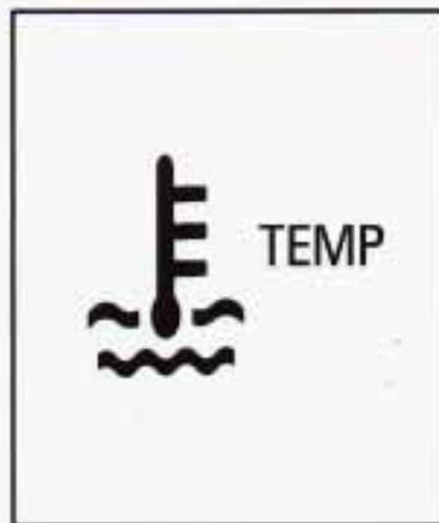
This light tells you that your engine coolant has overheated or your radiator cooling fan is not working. If you have been operating your vehicle under normal driving conditions, you should pull off the road, stop your vehicle and turn off the engine as soon as possible.
