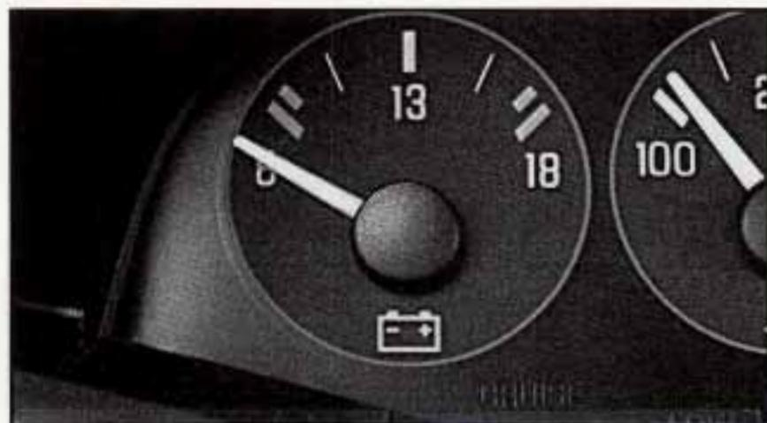
This gage shows the voltage in the electrical system. The normal range is 11 to 15 volts. If the reading stays outside the normal range, have your Buick dealer check the electrical system.
