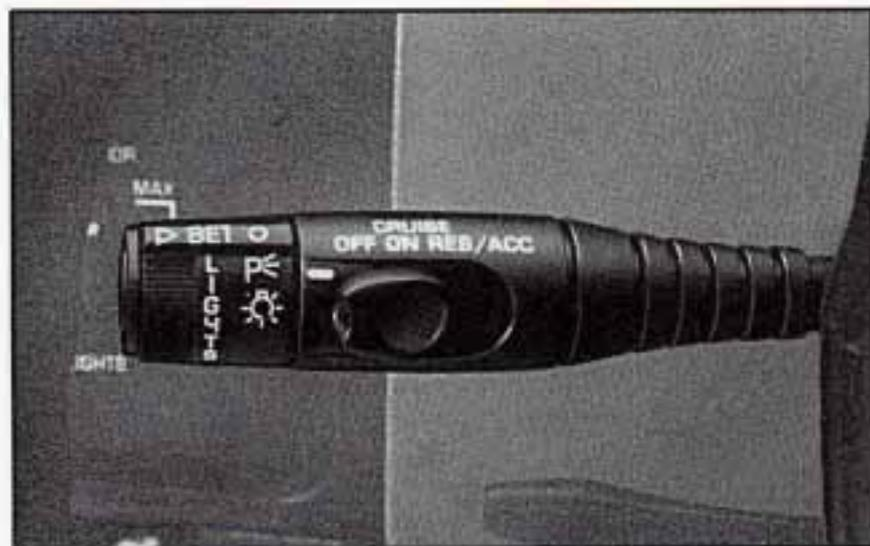
The headlight switch is located on the control left of the steering column.
