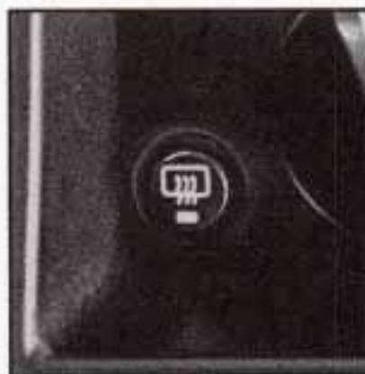
The lines you see on the rear window warm the glass. Press the button to start warming your window. Pressing the button again will shut it off.
