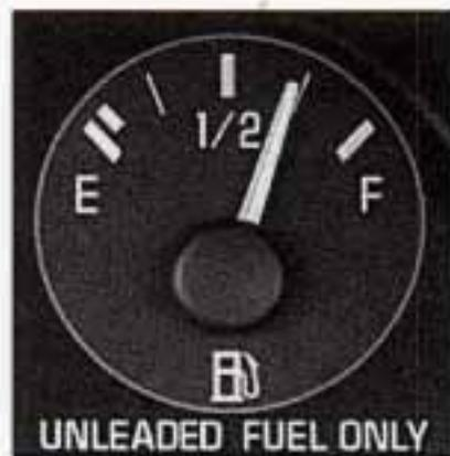
Your fuel gage shows how much fuel is in your tank. It works only when the engine is on. When the indicator nears "E," you still have a little fuel left. You need to get more right away.
