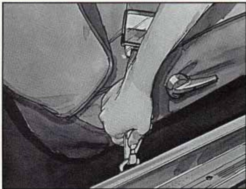
2. Push the spring on the hook near the door and remove the special belt.
