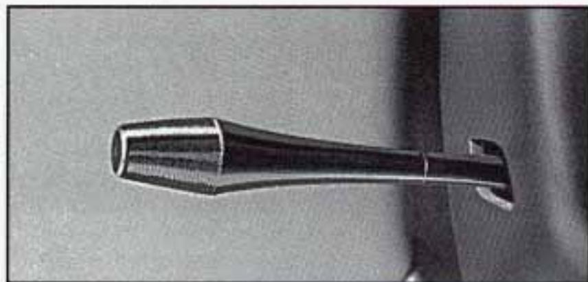
A tilt steering wheel allows you to adjust the steering wheel before you drive.
