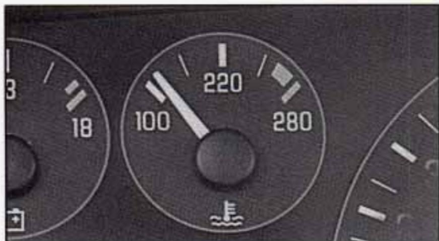
This gage shows the engine coolant temperature. If the gage pointer moves into the red area, your engine is too hot!
