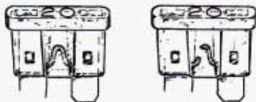
Look at the silver-colored band inside the fuse. If the band is broken or melted, replace the fuse. Be sure you replace a bad fuse with a new one of the identical size and rating.
