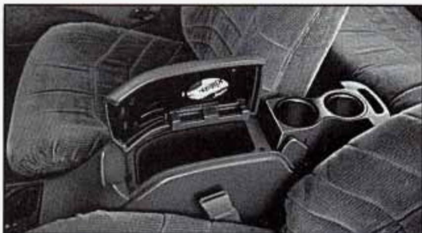
The console between the front seats has rear seat cupholders that when pulled up and rotated backward can be used. There is also a small tissue holder in the cover.
