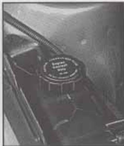
1. You can remove the coolant surge tank pressure cap when the cooling system, including the coolant surge tank pressure cap and upper radiator hose, is no longer hot. Turn the pressure cap slowly about one-quarter turn to the left and then stop.
