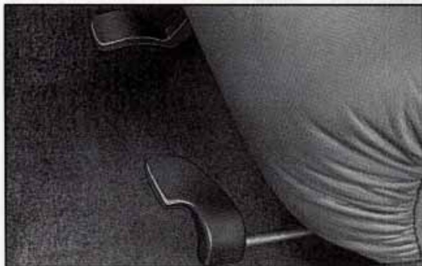
If you have this option, you have two levers under the front edge of the seat. The lever near the outer side of the seat unlocks the seat allowing it to slide forward and back. The lever near the center allows you to tilt the seat up and down.
