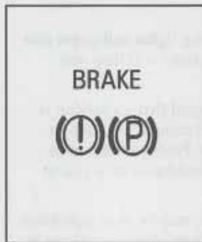
Your Buick's hydraulic brake system is divided into two parts. If one part isn't working, the other part can still work and stop you. For good braking, though, you need both parts working well.
