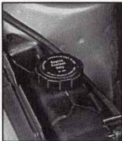
The coolant level should be at or above "FULL COLD." If it isn't, you may have a leak in the radiator hoses, heater hoses, radiator, water pump or somewhere else in the cooling system.
