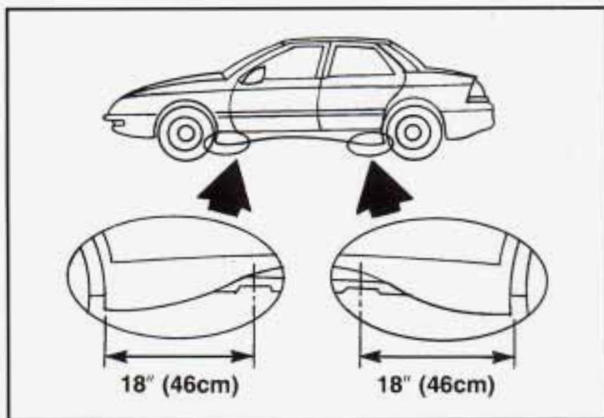
Position the jack under the vehicle near the flat tire. There is a notch in the frame about 18" (46 cm) from the front or rear tire well.
