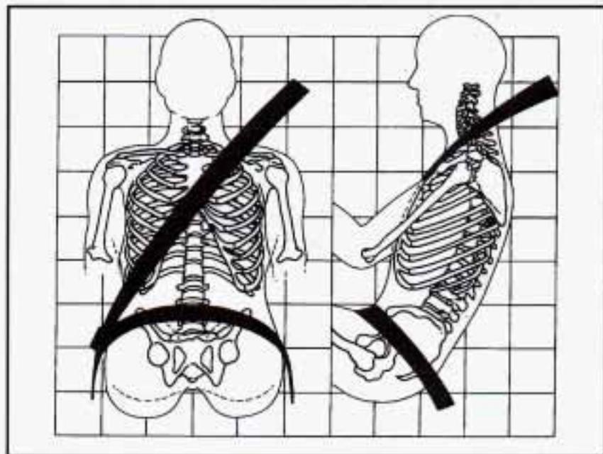
The lap belt should be worn as low on the hips as possible. In a crash, this applies force to the strong pelvic bones. And you'd be less likely to slide under the lap belt. If you slid under it, the belt would apply force at your abdomen. This could cause serious or even fatal injuries. The shoulder belt should go over the shoulder and across the chest. These parts of the body are best able to take belt restraining forces.
