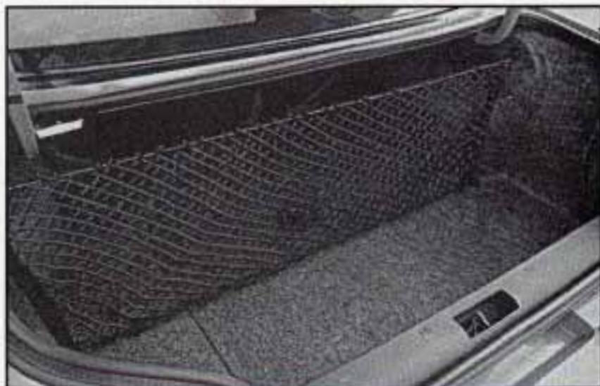
Your vehicle may have a convenience net. You'll see it just inside the back wall of the trunk. Put small loads, like grocery bags, behind the net. It can help keep them from falling over during sharp turns or quick starts and stops. The net isn't for larger, heavier loads. Store them in the trunk as far forward as you can. You can unhook the net so that it will lie flat when you're not using it.
