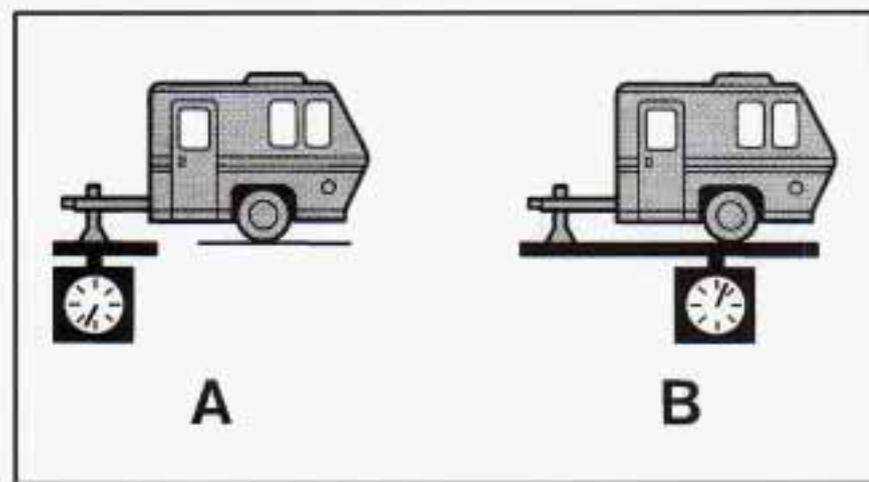
The trailer tongue (A) should weigh 10% of the total loaded trailer weight (B).
