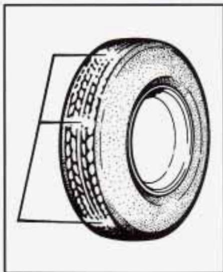
One way to tell when it's time for new tires is to check the treadwear indicators, which will appear when your tires have only  $\frac{2}{32}$  inch (1.6 mm) or less of tread remaining.
