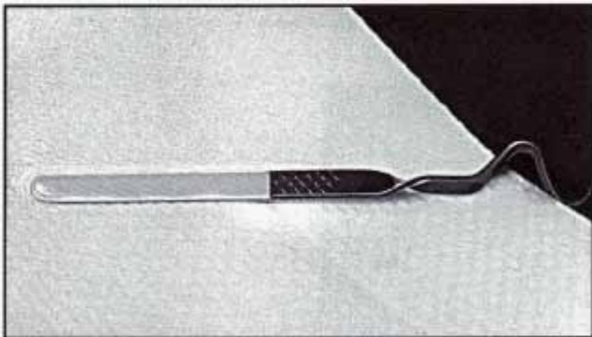
3. Check both sides of the dipstick, and read the lower level. The fluid level must be in the cross-hatched area.
