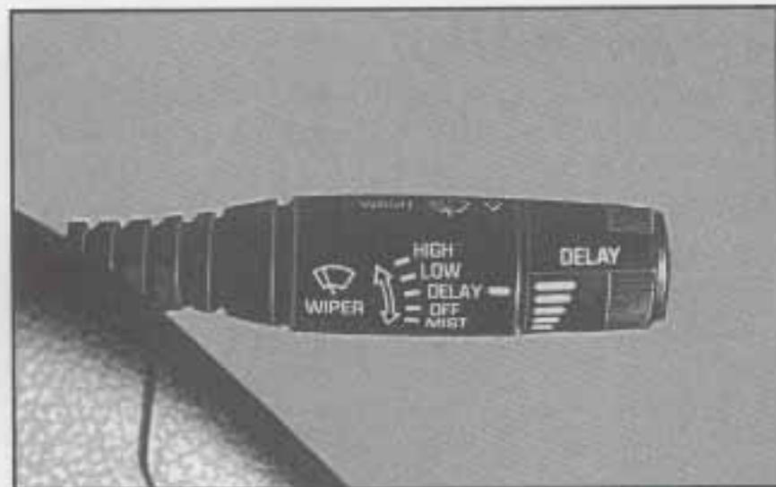
You control the windshield wipers by moving the lever marked "WIPER."
