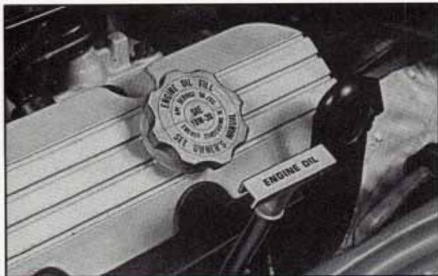
The engine oil dipstick is located directly behind the engine fan.
