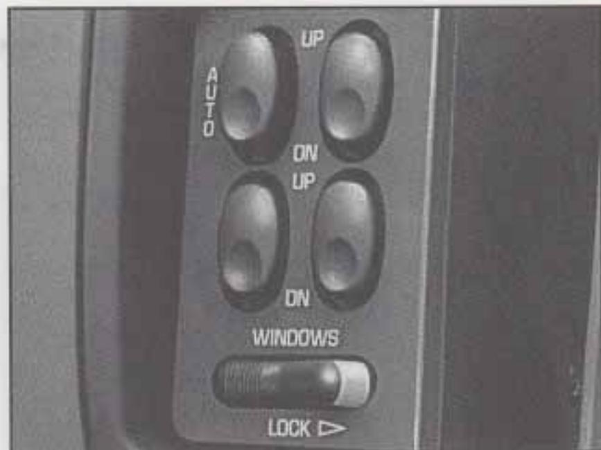
If your car has this option, the controls are near each window. Your driver's window has an express-down feature. Quickly press and release the AUTO switch and the driver's window will open a small amount. If the AUTO switch is pressed for more than a few seconds, the window will go all the way down. To stop a power window while it is lowering, press and release the
