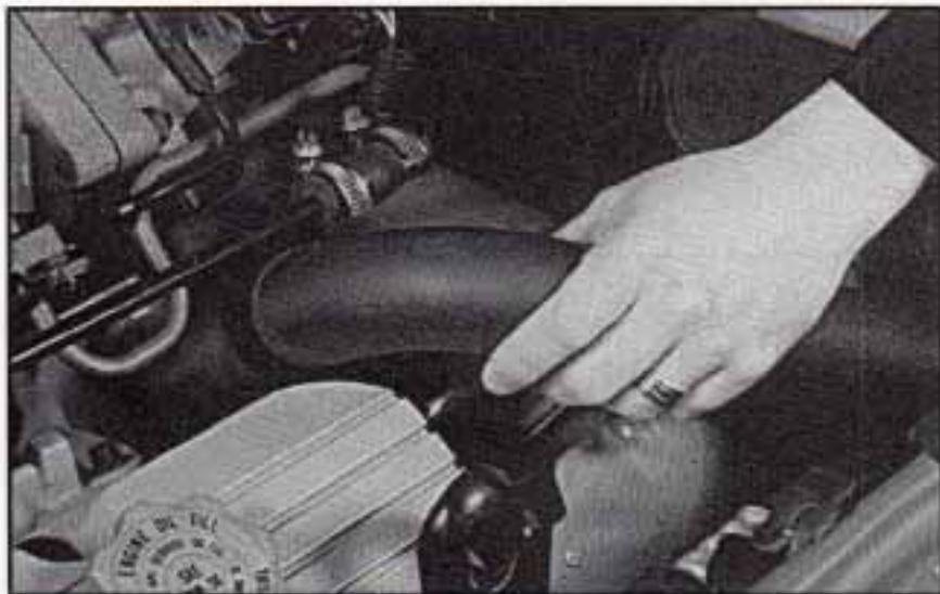
By this time, the coolant level inside the coolant surge tank may be lower. If the level is lower, add more of the proper mix to the coolant surge tank until the level reaches the split line formed by the black and white part of the tank.
