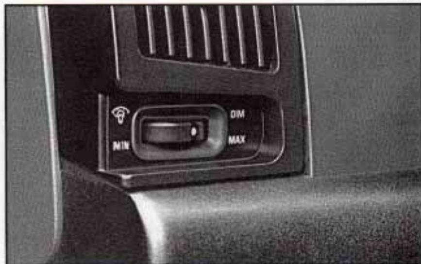
The interior courtesy lights can be turned on by rotating the control located on the instrument panel to **MAX**. The instrument panel brightness can be adjusted between **MIN** and **MAX** by rotating the control also.
