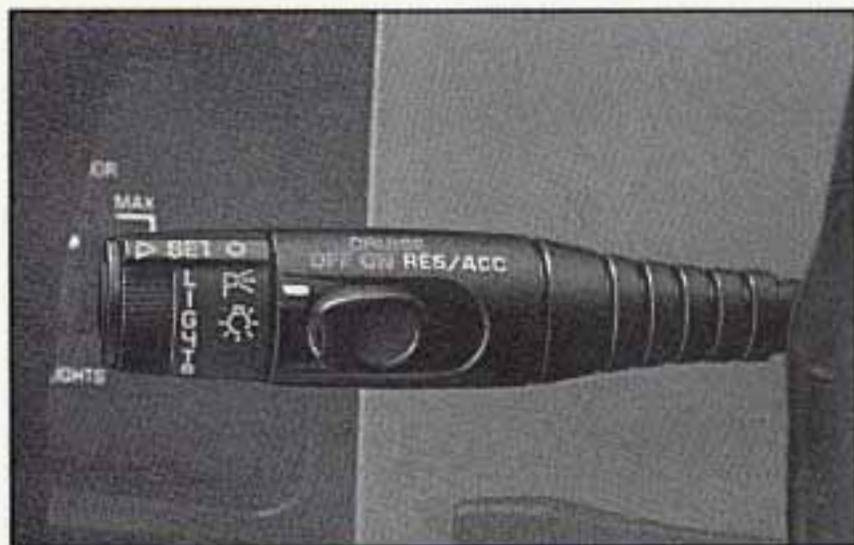
Remember, if you hold the switch at "RES/ACC" (Resume/Accelerate) longer than half a second, the vehicle will keep going faster until you release the switch or apply the brake. You could be startled and even lose control. So unless you want to go faster, don't hold the switch at "RES/ACC."
