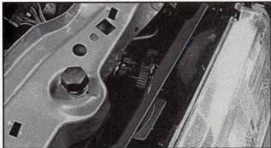
Raise the hood and locate the headlamp bulb retainers. To remove the access cover retainers, turn them 1/4 turn and lift the cover off.
