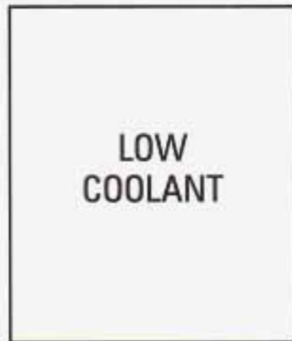
If this light comes on and stays on, the vehicle should promptly be pulled off the road and the coolant level checked. See "Engine Coolant" in the Index. If there are visible signs of steam see "Engine Overheating" in the Index before opening the hood.
