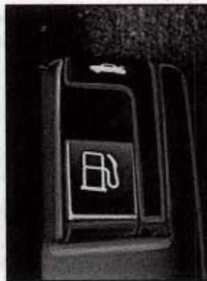
Pull up on the release lever to unlatch the fuel door. It is located on the floor to the left of the driver's seat.
