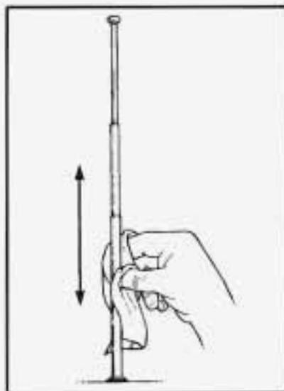
3. Wipe cloth over the mast sections, removing any dirt.
