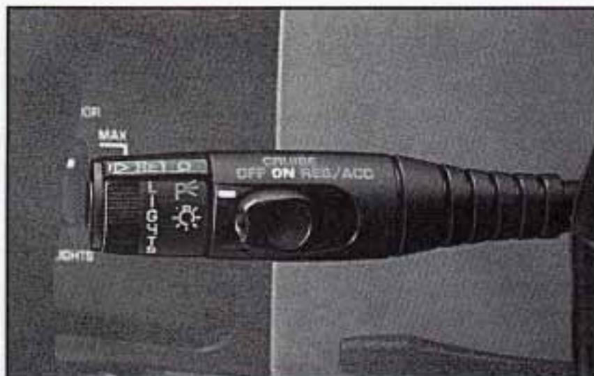
1. Move the Cruise Control switch to "ON."
