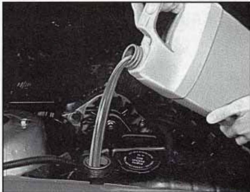
3. Fill the coolant surge tank with the proper mix, up to "FULL COLD" or just above the small cylinder at the base of the opening.
