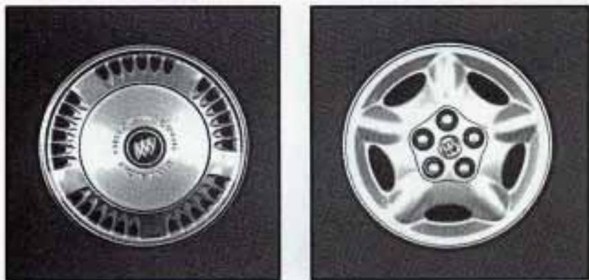
Remove either of these wheel covers by using the flat end of the wheel wrench. Pry along the edge of the wheel cover until it comes off. Be careful; the rim edges may be sharp. Don't try to remove it with your bare hands.
