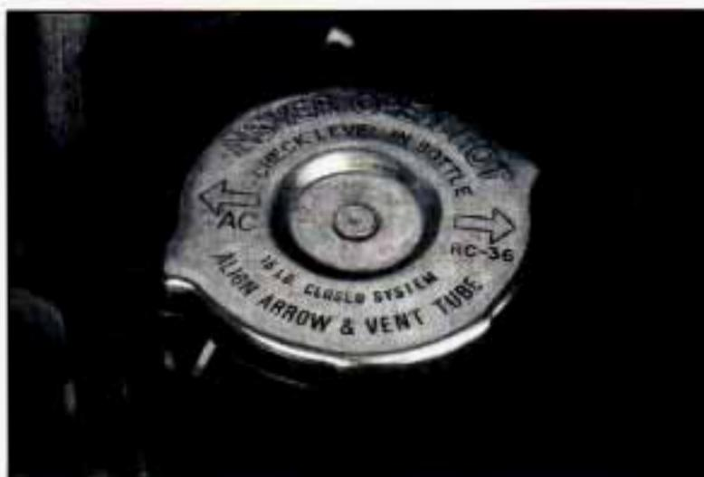
When you replace your radiator pressure cap, an AC<sup>®</sup> cap is recommended. See “Service Replacement Part and Filler Recommendations” in the Index.
