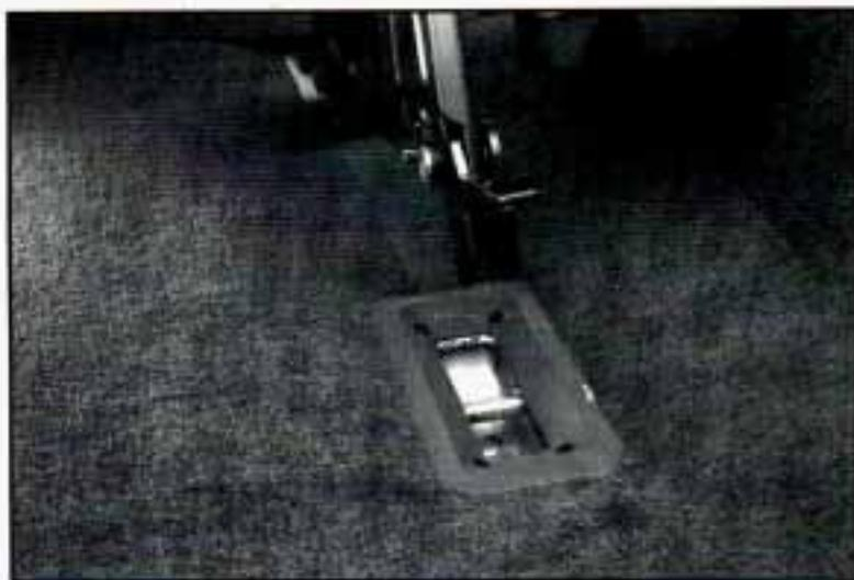
6. Lift up on the rear of the seat to remove the seat assembly from the rear latch pins. Then, pull back and lift the seat out of the vehicle.
