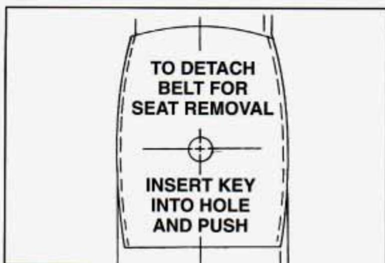
2. If you are removing the center seat, remove the right lap-shoulder belt. To do this, press the tip of a key into the release hole of the safety belt attachment while pulling up on the safety belt.
