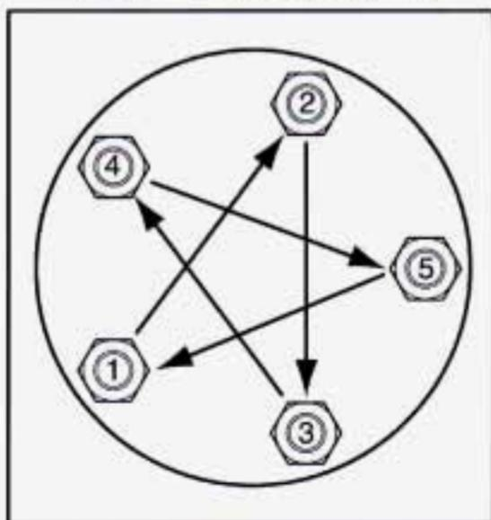
Tighten the wheel nuts firmly in a criss-cross sequence as shown. Rotate the ratchet to the right with the **UP** marking facing you.
