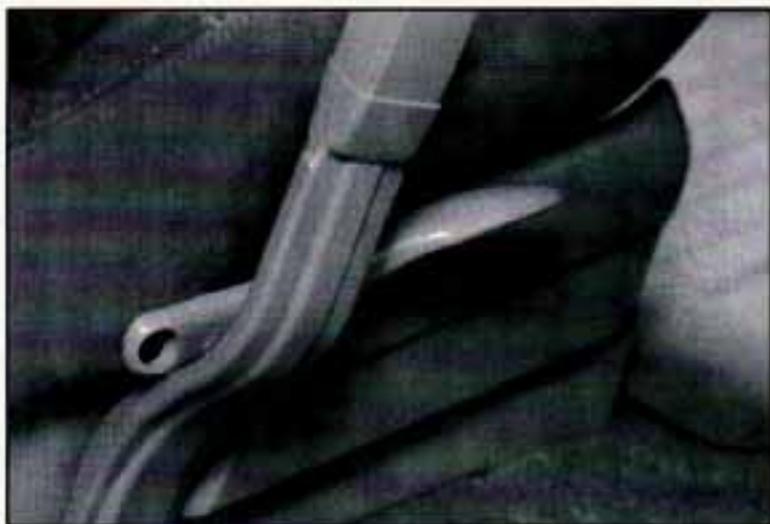
If you have the lever, you can adjust the seatback by lifting the lever. Release the lever to lock the seat back where you want it. Pull up on the lever and the seat will go to an upright position.
