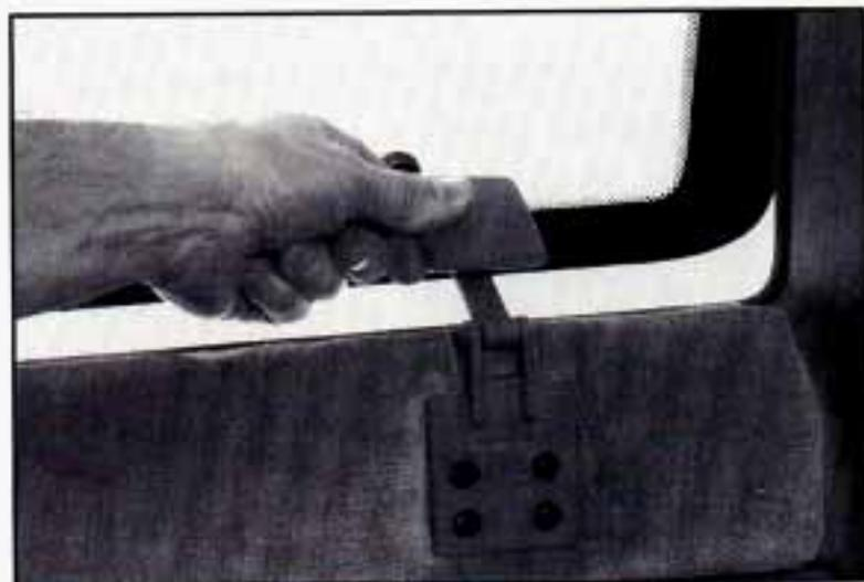
To open your swing-out windows, pull up on the latch and push the window out.
