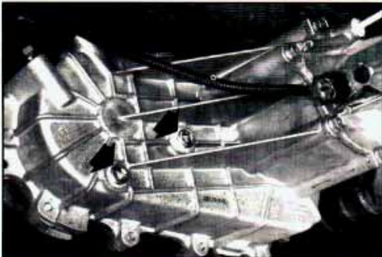
If the level is below the bottom of the filler plug hole, you'll need to add some lubricant. Add enough lubricant to raise the level to the bottom of the filler plug hole (top arrow shows filler plug hole, lower arrow shows drain plug hole.)
