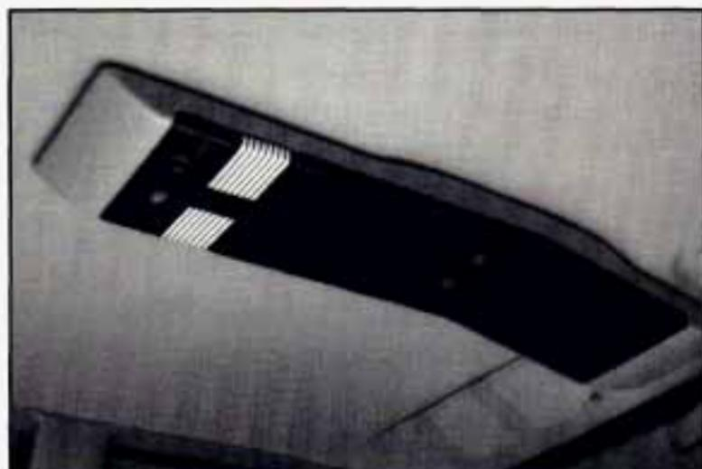
The optional roof console has two storage compartments. To open the compartments, push up and slide the door forward. To close the compartments, slide the door back. Use the straps to secure items.
