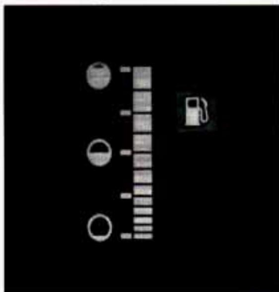
The fuel gage tells you how much fuel you have remaining when the ignition is on. When the gage first indicates empty you still have a little fuel left, but you should get more fuel as soon as possible.
