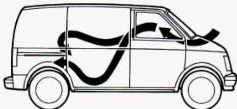
Your vehicle's flow-through ventilation system supplies outside air to the inside of your vehicle when it is moving. With the side windows closed, air will flow into the front air inlet grilles at the base of the windshield, through the vehicle and out the rear air exhaust valves. Outside air will also enter the vehicle when the heater or the air conditioning fan is running.
