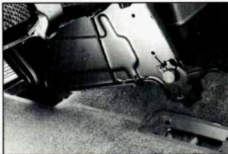
1. Lower the seat into position. Make sure the front retainers are hooked onto the anchor pins. Pull the seat down to latch the rear retainers.
