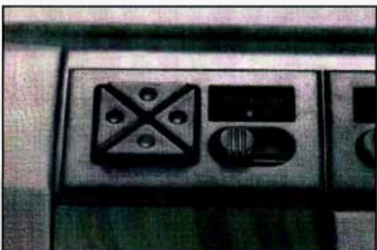
Some vehicles come with the optional remote control switch for adjusting the outside mirror. The switch is on the instrument panel above the radio.
