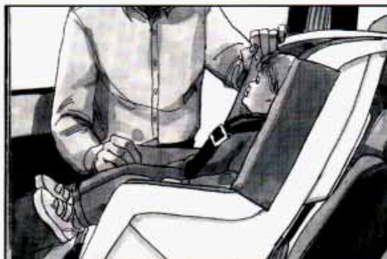
7. Push and pull the child restraint in different directions to be sure it is secure.
