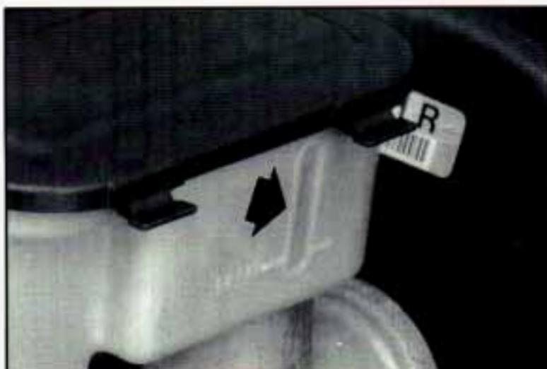
You can check the brake fluid without taking off the cap. Just look at the windows on the brake fluid reservoir.
