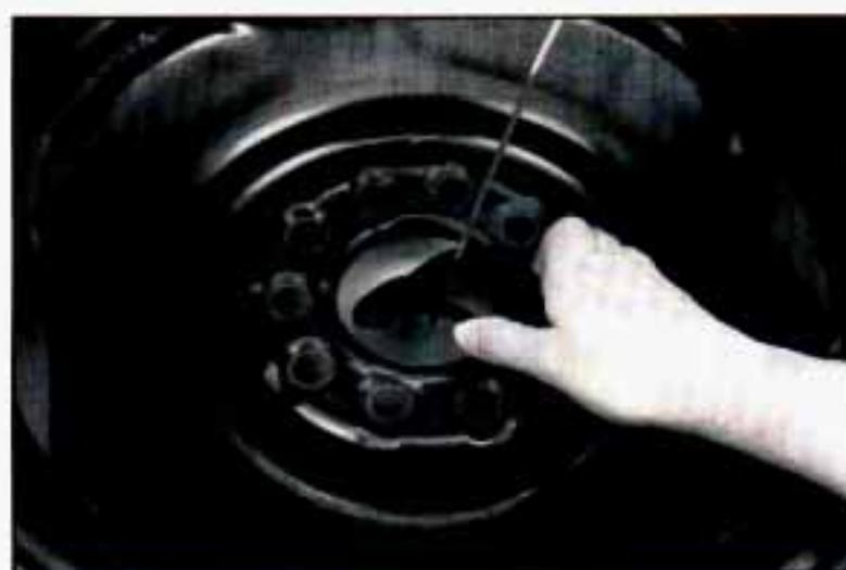
When the tire has been lowered, tilt the retainer at the end of the cable and pull it through the wheel opening.
