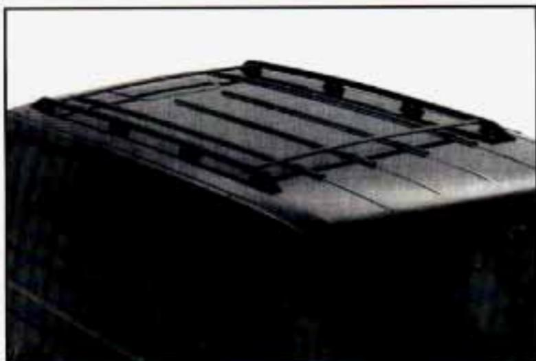
If you have the luggage carrier, you can load things on top of your vehicle. The luggage carrier has slats attached to the roof, side rails, and tiedowns.
