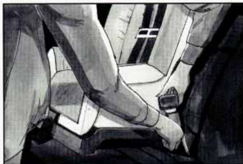
5. Buckle the belt. Make sure the release button is positioned so you would be able to unbuckle the safety belt quickly if you ever had to.
