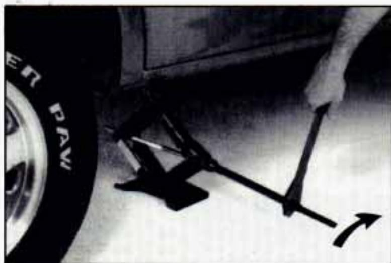
Raise the vehicle by rotating the ratchet to the right. Make sure the **UP** marking faces you. Raise the vehicle far enough off the ground so there is enough room for the spare tire to fit.
