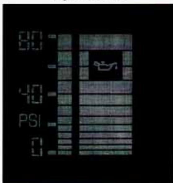
The oil pressure gage shows the engine oil pressure in psi (pounds per square inch) when the engine is running. Canadian vehicles indicate pressure in kPa (kilopascals). Oil pressure may vary with engine speed, outside temperature and oil viscosity, but readings above the low pressure zone indicate the normal operating range.
