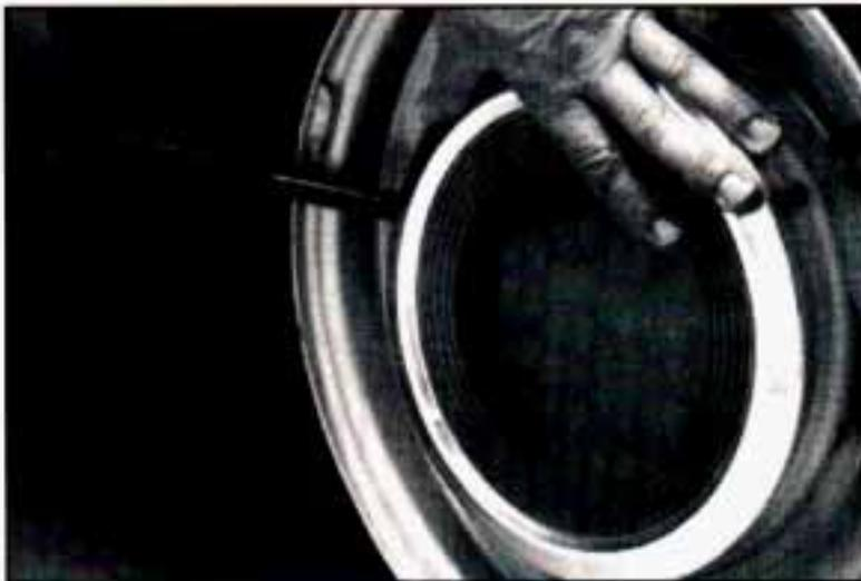
If you have an aluminum hub cap, remove it by using the flat end of the extension.
