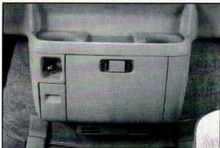
Your front storage compartment is at the center of the engine cover. To open the compartment, press the two tabs together and pull.
