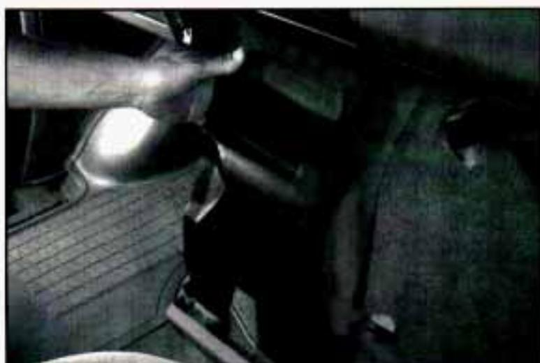
6. Grasp the top of the heater duct and pull down gently to remove.
