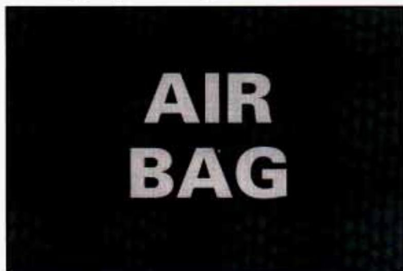
There is an air bag readiness light on the instrument panel, which shows **AIR BAG**. The system checks for electrical malfunctions, and the light tells you if there is a problem.
