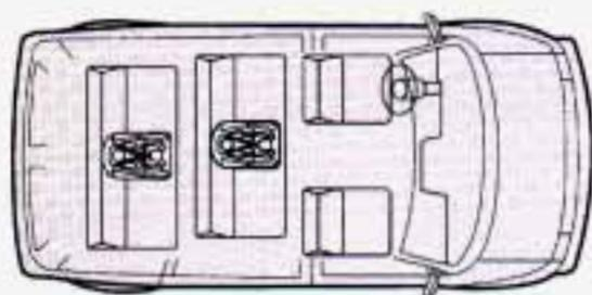
When you secure a child restraint in a center seating position, you'll be using the lap belt.
