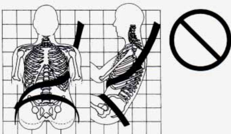
**A:** The shoulder belt is worn under the arm. It should be worn over the shoulder at all times.
