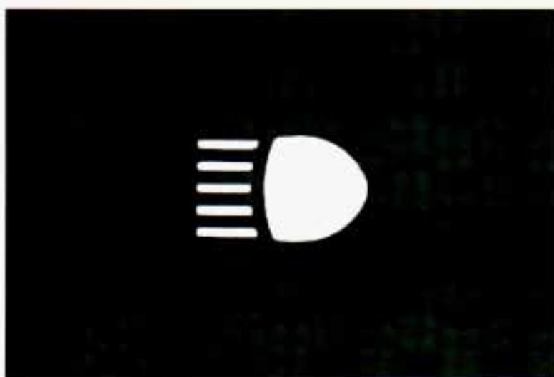
The high beam indicator is on whenever you use your high beam headlights. For more details, see “Headlight High–Low Beam Changer” in this part.
