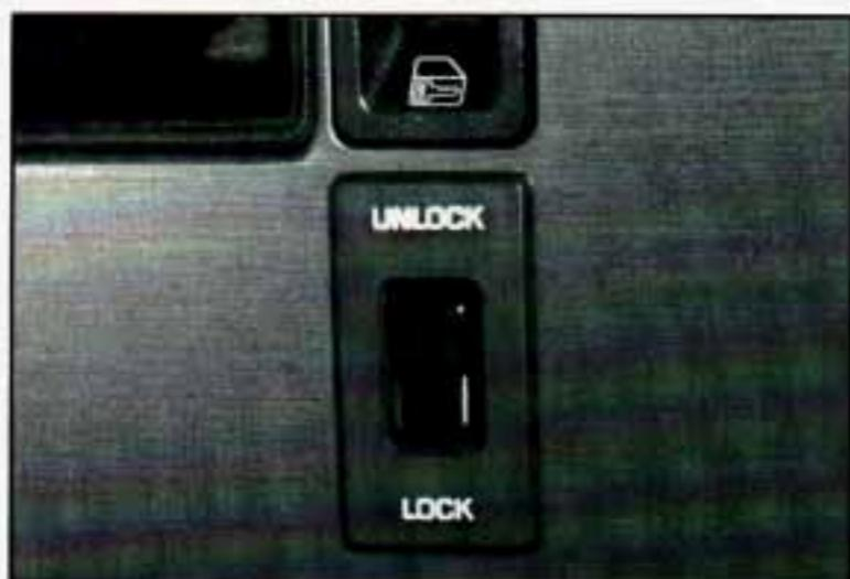
If your vehicle has power door locks, push the power door lock switch to lock or unlock all the doors at once.
