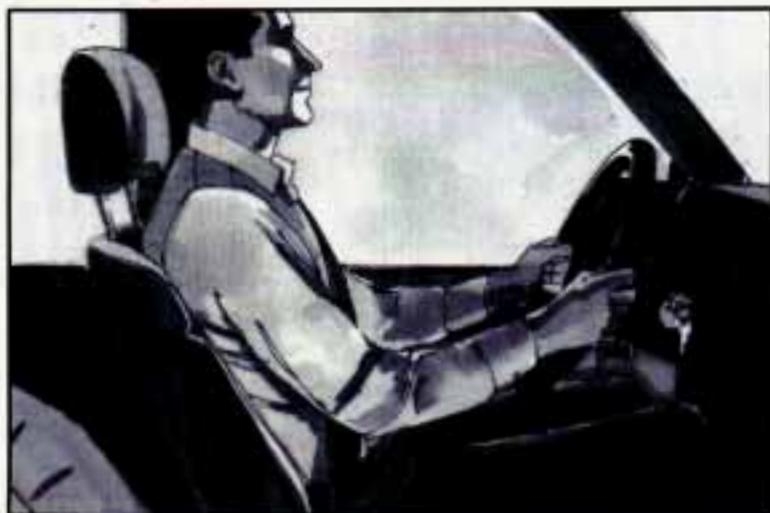
Slide the head restraint up or down so that the top of the restraint is closest to the top of your ears. This position reduces the chances of a neck injury in a crash.
