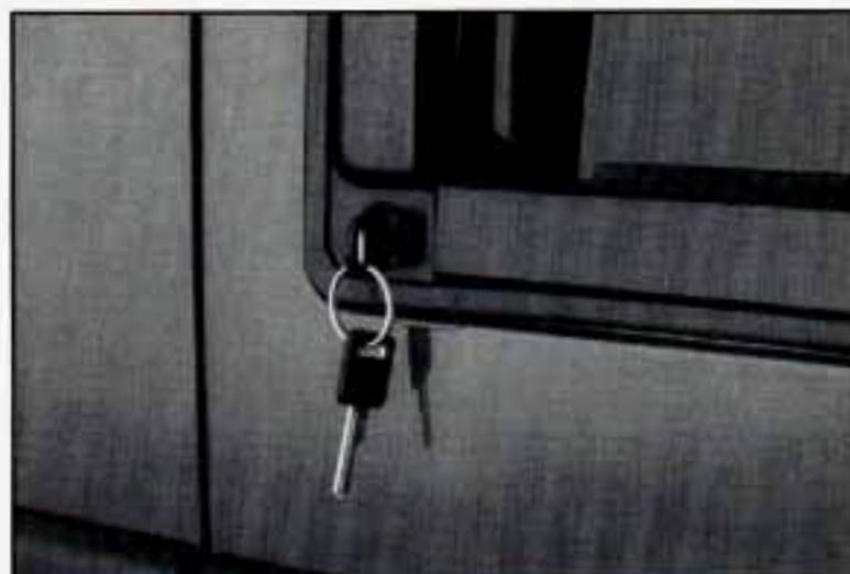
To release the hatch and unlock the doors from the outside of the vehicle, put the key in the lock and turn to the right. Then, pull up on the hatch and open the right rear door first. Grasp the handle and pull the door open.
