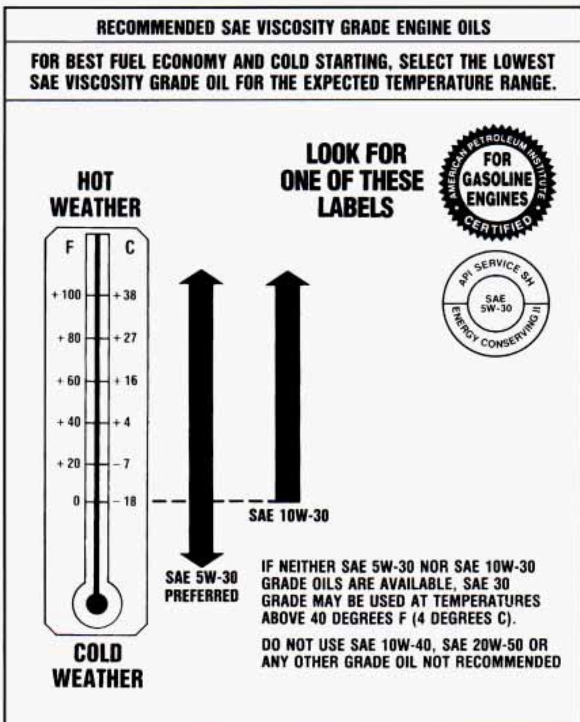
As shown in the chart, SAE 5W-30 is best for your vehicle. However, you can use SAE 10W-30 if it's going to be 0°F (-18°C) or above. These numbers on an oil container show its viscosity, or thickness. Do not use other viscosity oils, such as SAE 10W-40 or SAE 20W-50.
