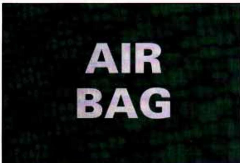
You will see this light flash for a few seconds when you turn your ignition to **RUN** or **START**. Then the light should go out, which means the system is ready.
