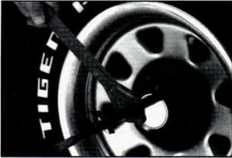
Place the ratchet and socket on the wheel nut with the center cap on.
