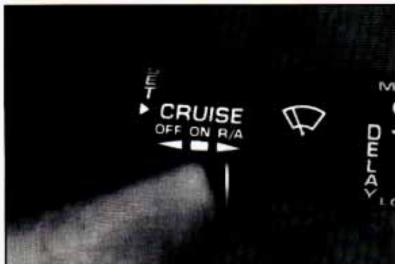
Suppose you set your Cruise Control at a desired speed and then you apply the brake. This, of course, shuts off the Cruise Control. But you don't need to reset it. Once you're going about 25 mph (40 km/h) or more, you can move the Cruise Control switch from **ON** to **R/A** (Resume/Accelerate) and hold it for about half a second.
