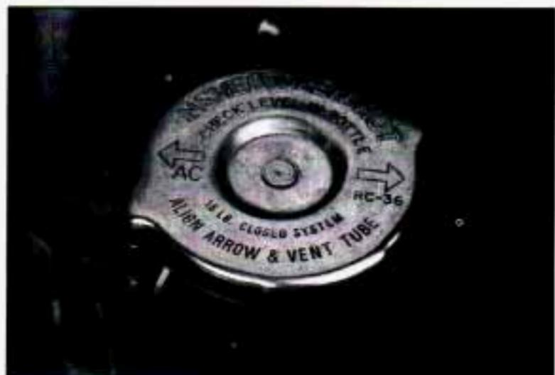
8. Then replace the pressure cap. At any time during this procedure if coolant begins to flow out of the filler neck, reinstall the pressure cap. Be sure the arrows on the pressure cap line up like this.
