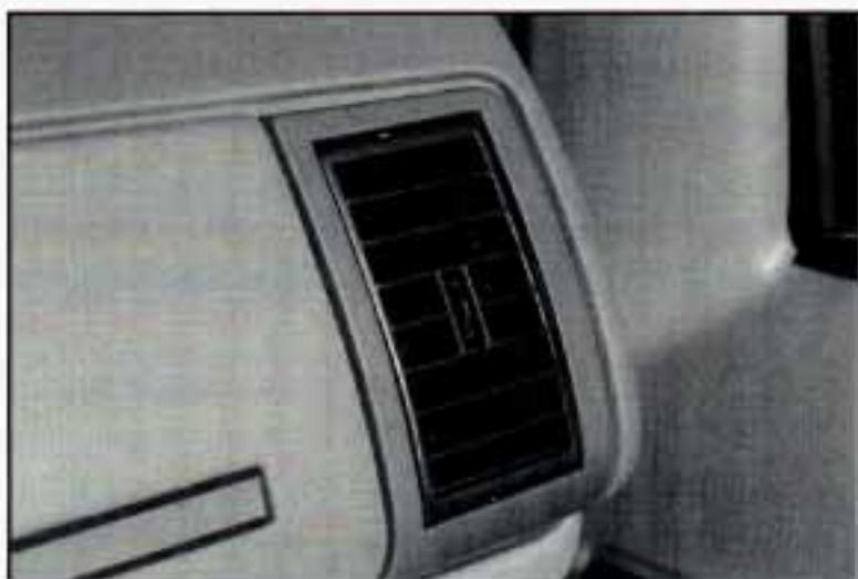
You can move the vents to direct the flow of air, or close the vents altogether. When you close a vent, it will increase the flow of air coming out of any vents that are open.
