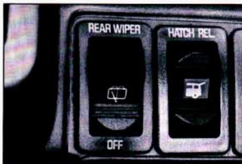
This switch is to the left of the steering column. It will release the rear hatch.
