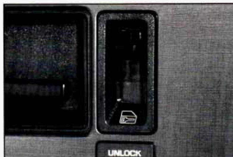
From the inside: To lock front doors and sliding side door, slide the lock levers down.
