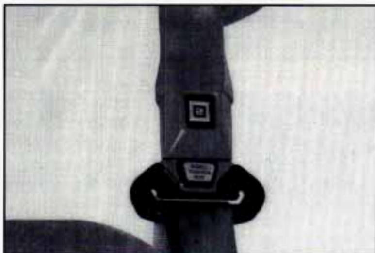
1. Disconnect the quick release latch plates for the lap-shoulder belt from the buckles in the roof.
