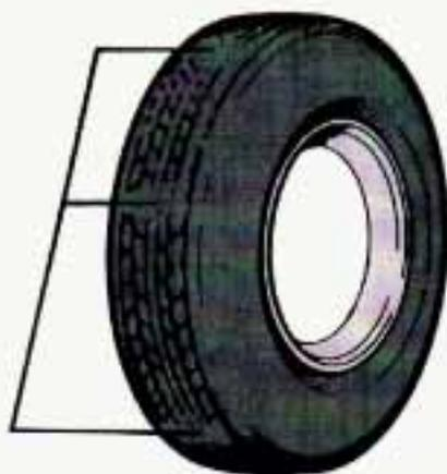
One way to tell when it's time for new tires is to check the treadwear indicators, which will appear when your tires have only 2/32 inch (1.6 mm) or less of tread remaining.
