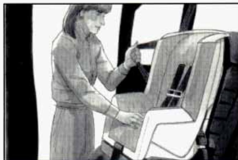
6. To tighten the belt, pull up on the shoulder belt while you push down on the child restraint.
