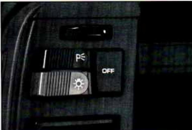
Your light switches are on the left side of the instrument panel above the vent.
