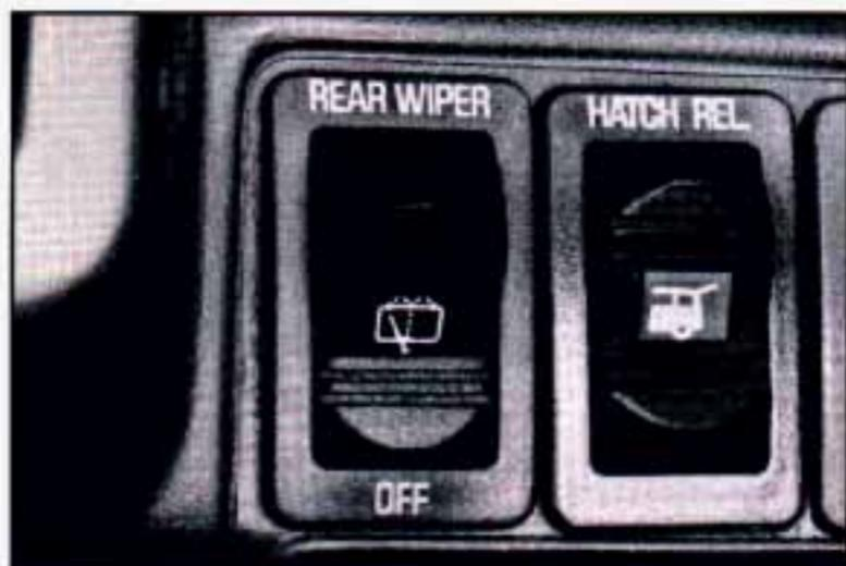
You control your rear window wiper/washer from a switch on your instrument panel, just left of your steering column.
