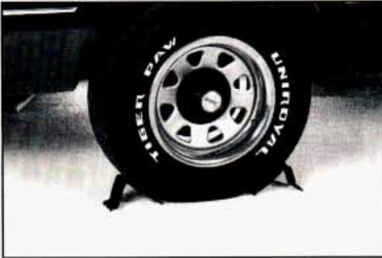
You have two wheel blocks stored with your jack. Place the blocks at the front and rear of the tire farthest away from the one being changed. That would be the tire on the other side of the vehicle, at the opposite end.
