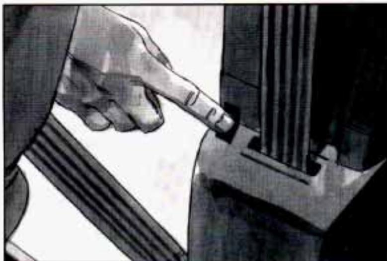
5. Press the button on the retractor cover to set the lock.
