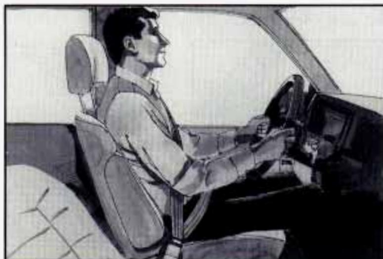
The driver has a lap–shoulder belt. Here's how to wear it properly.
