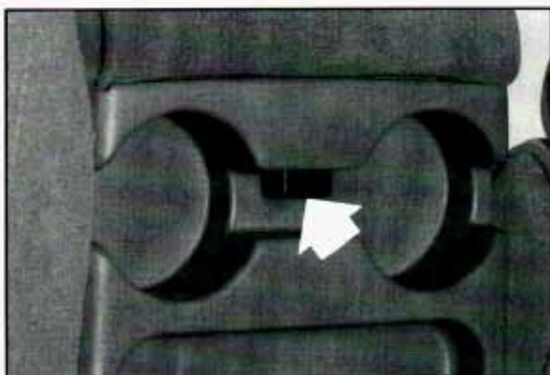
To raise or lower the center console, press the button between the beverage holders.
