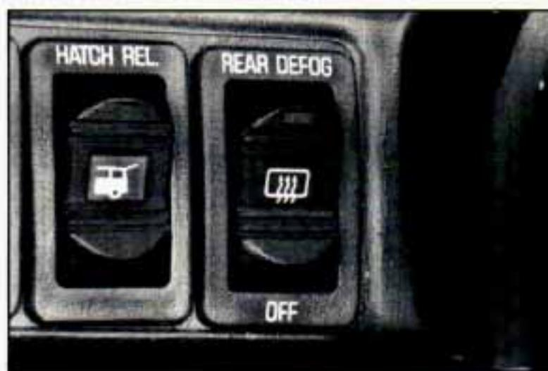
To turn on the rear window defogger, find the switch marked **REAR DEFOG** on your instrument panel to the left of the steering column. Press the top of this switch until the light in the switch comes on, then release it.
