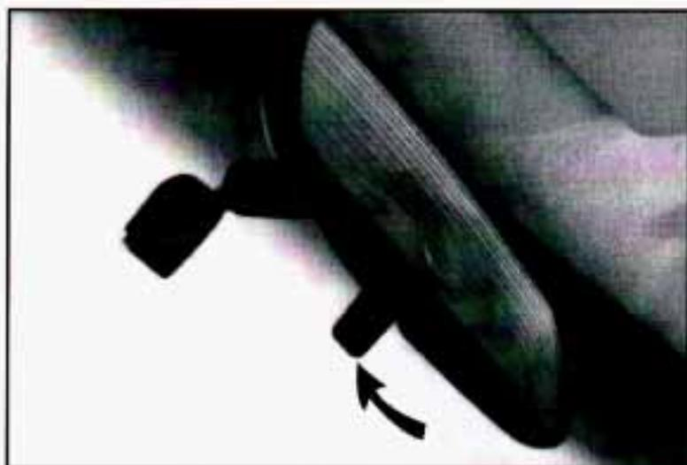
You can also adjust the mirror for day or night driving. Press the tab forward (away from you) for day driving. Pull the tab back (towards you) for night driving.
