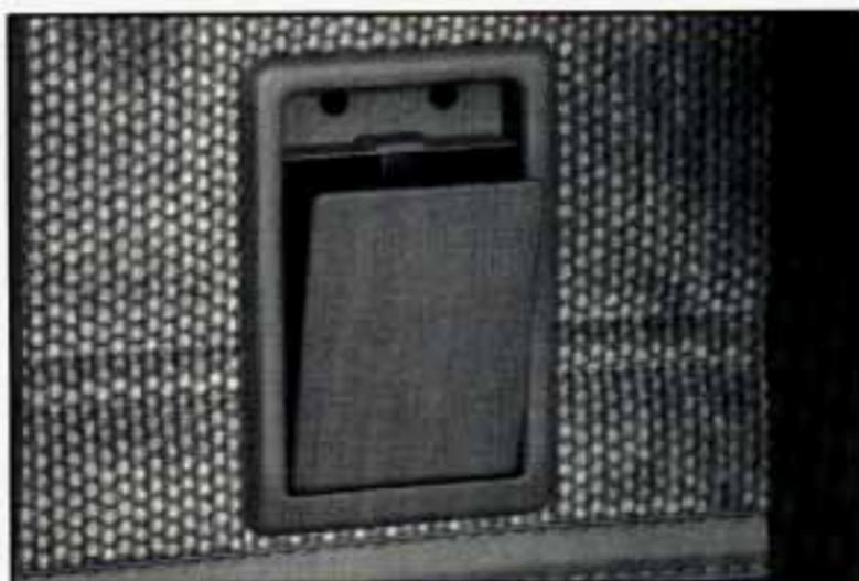
To remove the smaller ashtrays on each sidewall, press down on the tabs inside and pull out.
