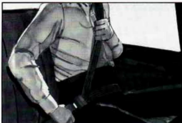
3. To make the lap part tight, pull down on the buckle end of the belt as you pull up on the shoulder.
