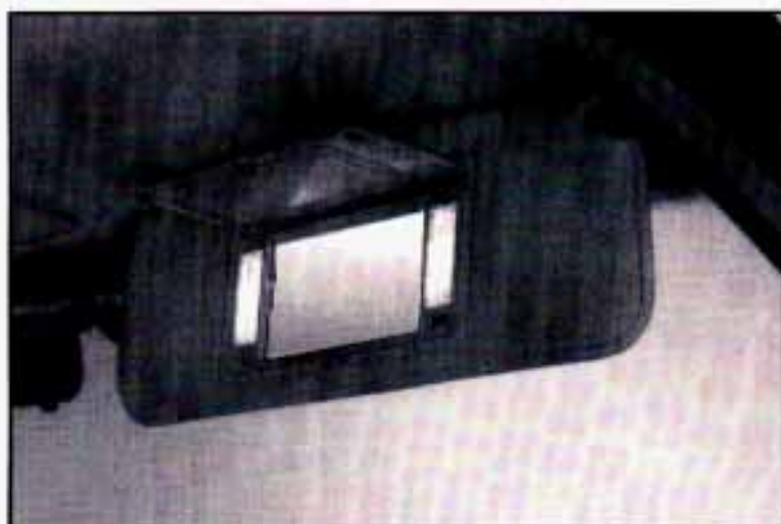
Some visors have mirrors built in, with or without lights. Just lift the mirror cover on each visor to turn the lights on if you have them.
