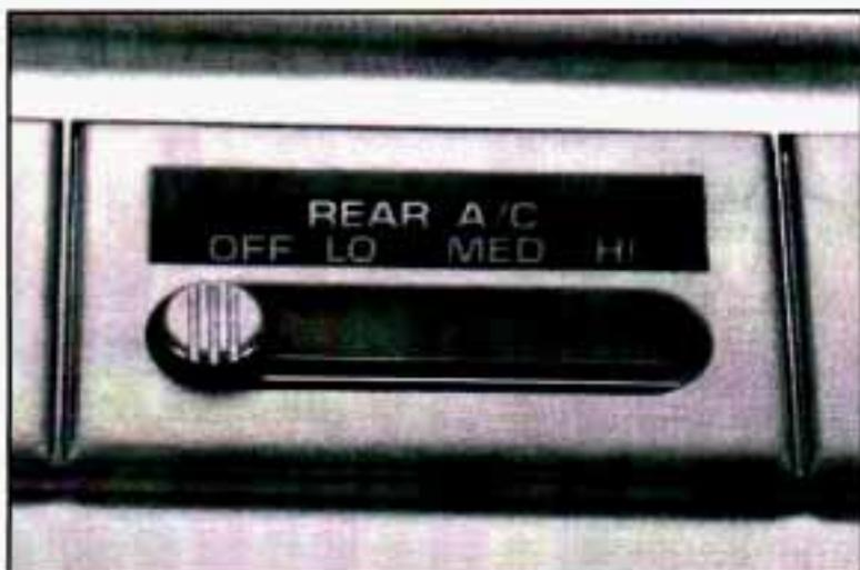
You may have rear air conditioning. The rear air conditioning switch is located above the radio at the top of the instrument panel. Slide the lever toward **HI** for cooler air in the rear area. Slide the lever to **OFF** to turn the system off.
