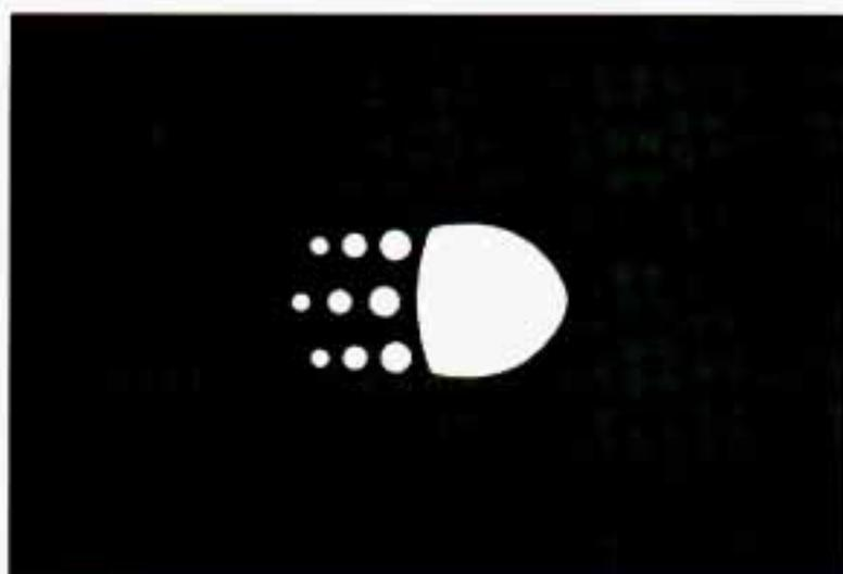
The DRL indicator is on whenever the ignition and the headlight switch and parking brake are off. For more details about DRL, see “Lights” in this part.
