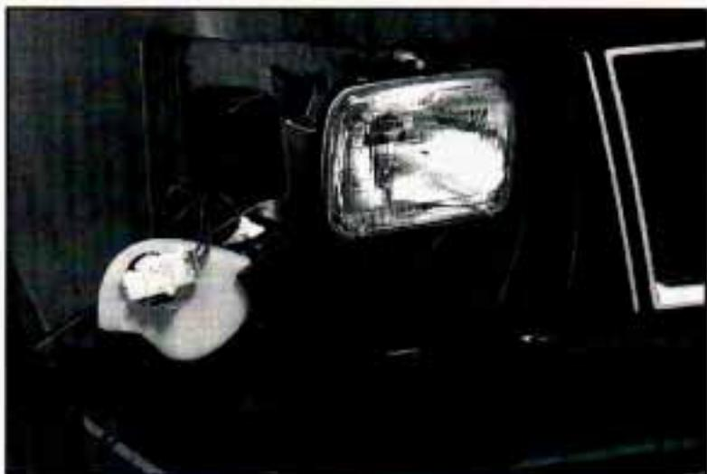
3. Press the tab and turn the socket to the left to remove the socket from the bezel. If the socket does not have a tab, turn the socket to the left. Set the bezel aside.
