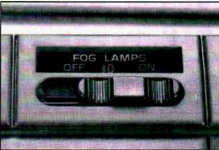
Your fog lamp switch is in the center of the instrument panel above the radio.
