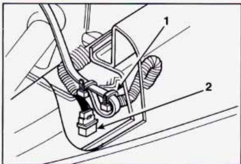
1. Engine Coolant Heater Strap
