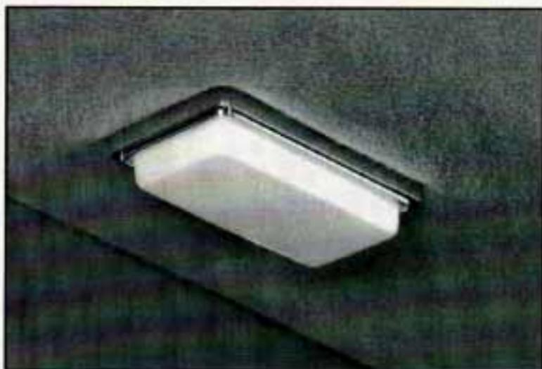
The dome lights may come on when you open any of the doors. You can also turn on the dome lights by turning the dimmer dial to the right until it clicks.
