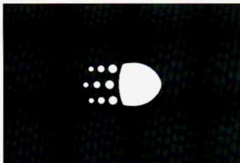
If your vehicle was first sold, when new, in Canada, you will have this light on the instrument panel. It goes on whenever the Daytime Running Lights are on, the ignition is on, the headlamp switch is off, and the parking brake is released.
