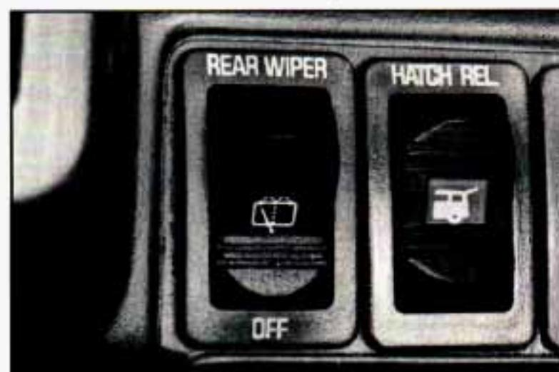
To unlock the rear hatch and split-panel doors from the inside: Push the top of the **HATCH REL** switch.
