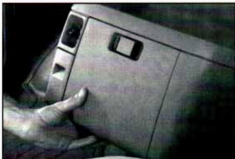
4. Grasp the bottom of the extension. Lift up and then pull out.
