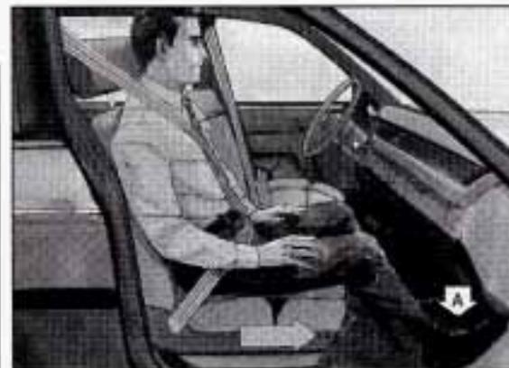
Adjust the seat (to see how, see *Seats* in the *Index*) so you can sit up straight. Move your seat far enough forward that your feet touch the part of the vehicle that is called the "toeboard" (A). That way you'd be less likely to slide under the lap belt in a crash.
