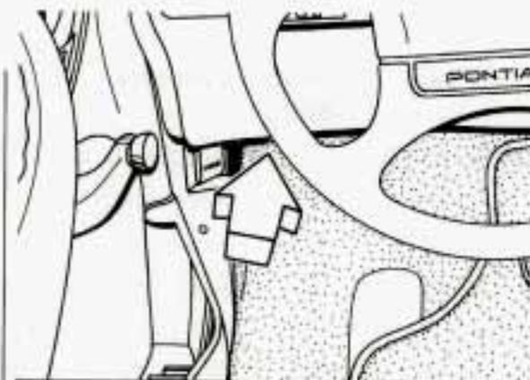
The fuse panel is located on the lower left side of the instrument panel. To open, pull the handle marked **FUSE** down and forward.
