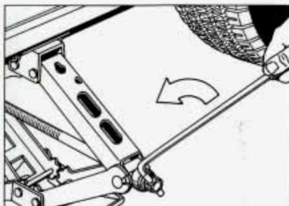
15. Lower the vehicle by rotating the jack handle counterclockwise. Lower the jack completely.
