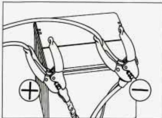
7. Don't let the other end touch metal. Connect it to the positive (+) terminal of the good battery. Use a remote positive (+) terminal if the vehicle has one.
