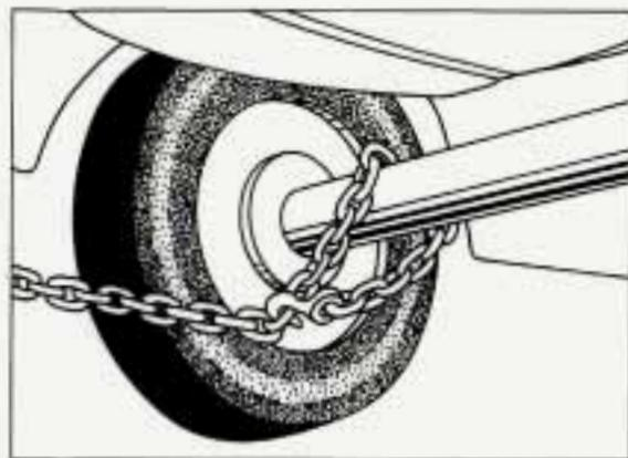
3. Attach a separate safety chain to each side of the axle inboard of the spring.
