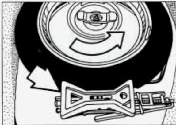
**4.** Remove the wing bolt securing the compact spare tire, spacer and wheel wrench by turning it counterclockwise. Then lift off the spacer and remove the spare tire.
