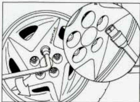
8. Using the wheel wrench, remove the plastic cap nuts and **loosen** all the wheel nuts. Don't remove the wheel nuts yet.
