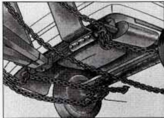
2. Position the lower sling crossbar directly below and to the rear of the rear bumper.
