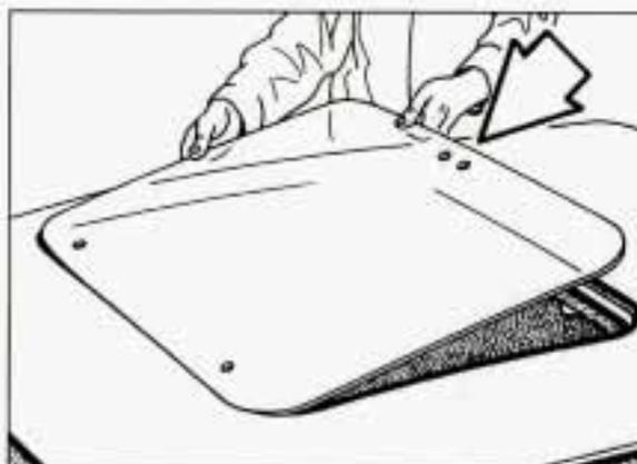
2. Push forward on the rear edge of the glass while lowering the panel. **Do not force** a hinge if it binds in a slot. Reposition the glass panel and start again. Finally, push the glass release tab, engage the latch with the striker and close the panel.
