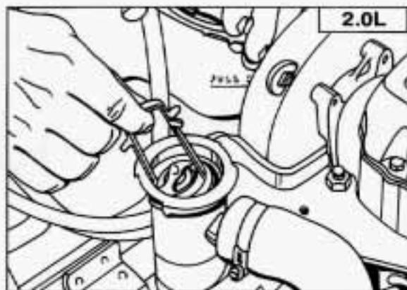
3. Pull the thermostat out of the housing.
