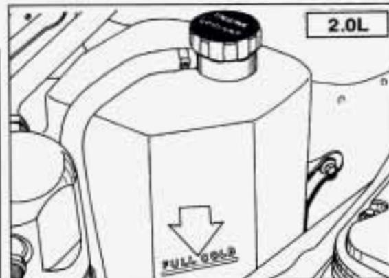
The coolant level should be at or above **FULL COLD**. If it isn't, you may have a leak in the radiator hoses, heater hoses, radiator, water pump or somewhere else in the cooling system.
