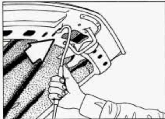
Lift the hood, release the hood prop from its retainer and put the hood prop into the slot in the hood.
