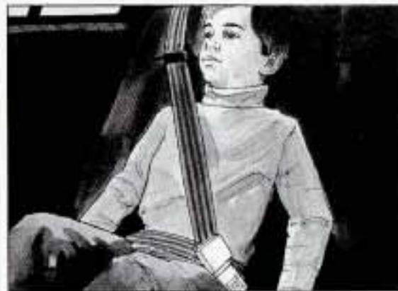
4. Buckle the belt around the child, and make sure that both the lap belt and the shoulder belt are secured properly. Make sure that the shoulder belt crosses the shoulder. See *Safety Belts, Rear Seat Passengers* in the *Index*.
