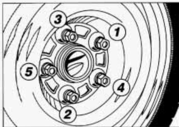
16. Tighten the wheel nuts firmly in a criss-cross sequence, as shown.
