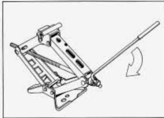
**6.** Remove the band around the jack. Turn the jack handle clockwise to raise the jack head a few inches.
