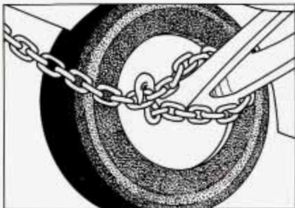
4. Attach a separate safety chain around the outboard end of each lower control arm.
