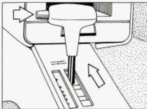
2. Move the shift lever into the **P** (Park) position like this: Hold in the button on the lever, and push the lever all the way toward the front of your vehicle.
