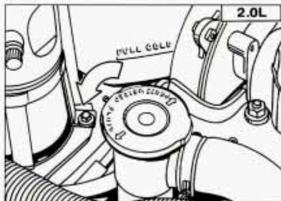
**How to Add Coolant to the 2.0L L4 Engine at the Thermostat Housing**
