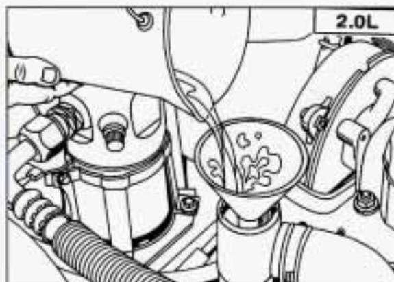
4. Fill the thermostat housing with the proper mix, up to the base of the filler neck.
