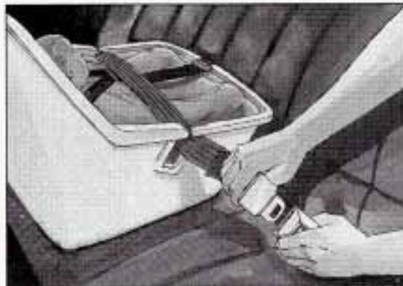
4. Run the vehicle's safety belt through or around the restraint. The child restraint instructions will show you how.
