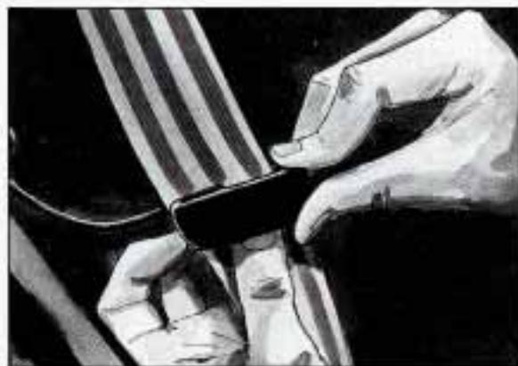
2. Slide the guide under and past the belt. The elastic cord must be under the belt. Then, place the guide over the belt, and insert the two edges of the belt into the slots of the guide.
