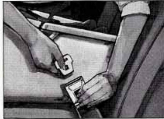
3. Put the belt's special latch plate into the vehicle's safety belt buckle.
