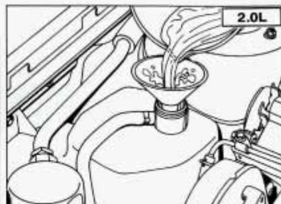
5. Then fill the coolant recovery tank to **FULL COLD**.
