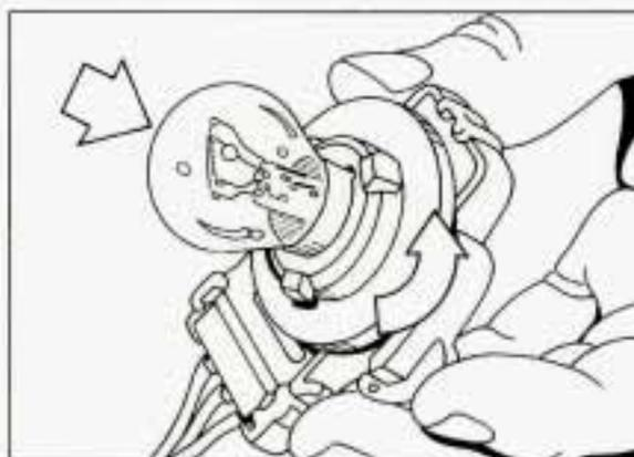
5. To remove the bulb, push in and turn it counterclockwise.
