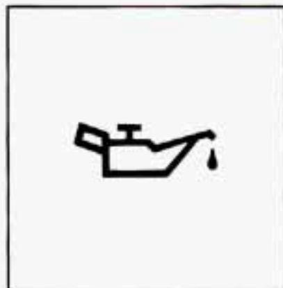
If you have a problem with your oil, this red oil pressure warning light may stay on after you start your engine, or come on when you are driving. Stop your vehicle and shut off the engine if this light stays on.
