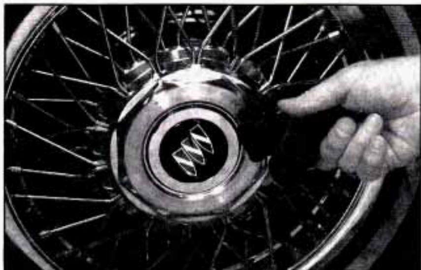
Removing the wire wheel cover requires this wire wheel key wrench.
