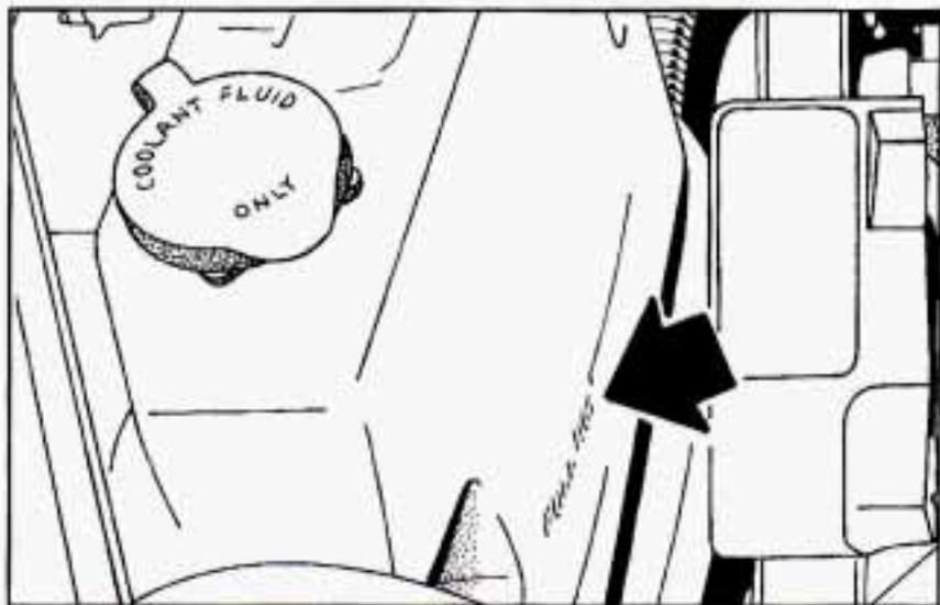
The coolant level should be at the FULL HOT mark. If it isn't, you may have a leak in the radiator hoses, heater hoses, radiator, water pump or somewhere else in the cooling system.
