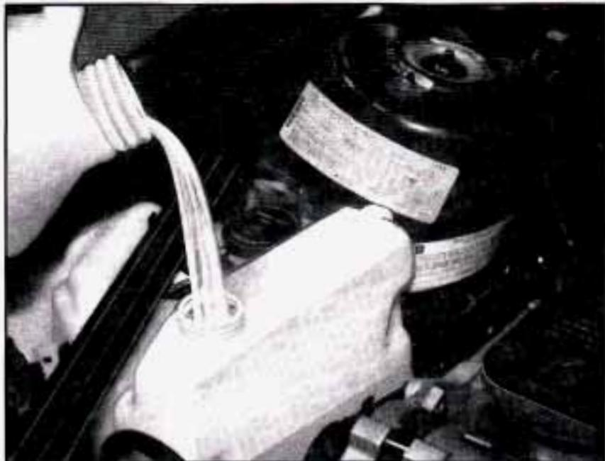
5. Then fill the coolant recovery tank to the **FULL HOT** mark.
