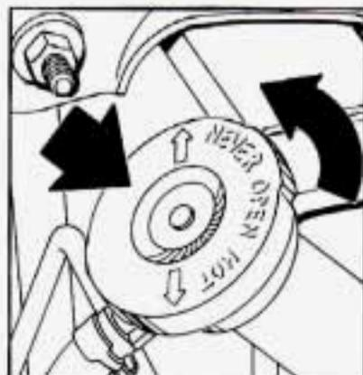
2. Then keep turning the pressure cap, but now push down as you turn it. Remove the pressure cap.
