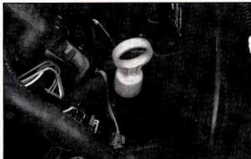
The red handle dipstick on the four speed (4T60-E) transaxle engine looks like this.
