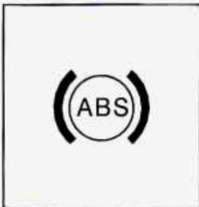
With the anti-lock brake system, this light will come on when you start your engine and it will stay on for three seconds. That's normal. If the light doesn't come on, have it fixed so it will be ready to warn you if there is a problem.
