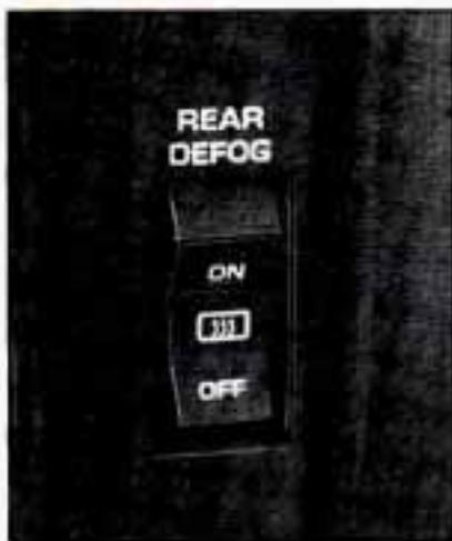
The rear window defogger uses a warming grid to remove fog from the rear window. In winter, it can also keep ice from forming on the rear window.
