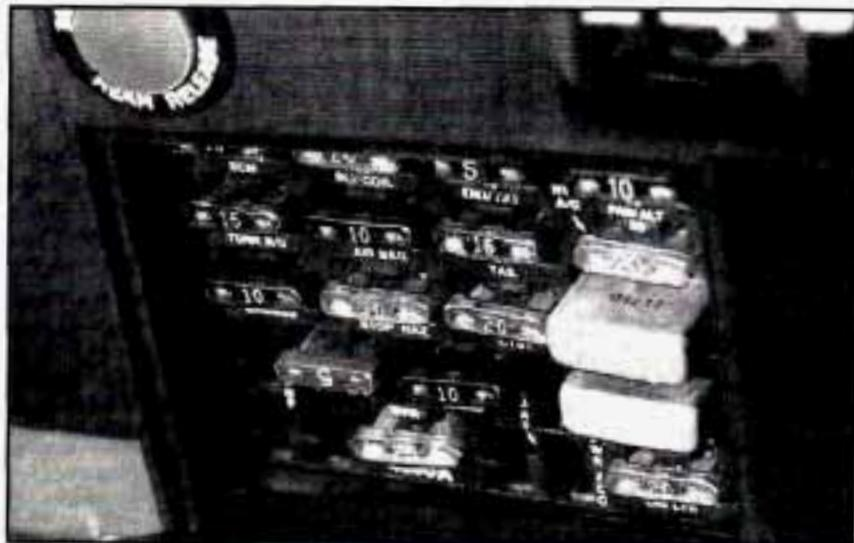
The wiring circuits in your vehicle are protected from short circuits by a combination of fuses, circuit breakers, and fusible thermal links in the wiring itself. This greatly reduces the chance of damage caused by electrical problems.
