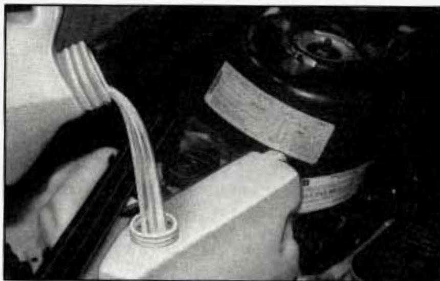
The coolant recovery tank is located on the passenger's side of the engine compartment.
