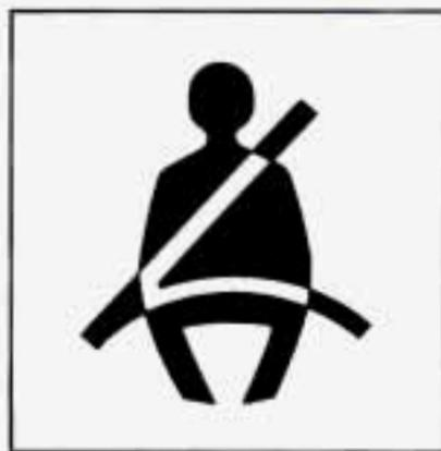
When the key is turned to RUN or START a chime will come on for about eight seconds to remind people to fasten their safety belts, unless the driver's safety belt is already buckled. The safety belt light will also come on and stay on for about 20 seconds, then it will flash for about 55 seconds. If the driver's belt is already buckled, neither the chime nor the light will come on.
