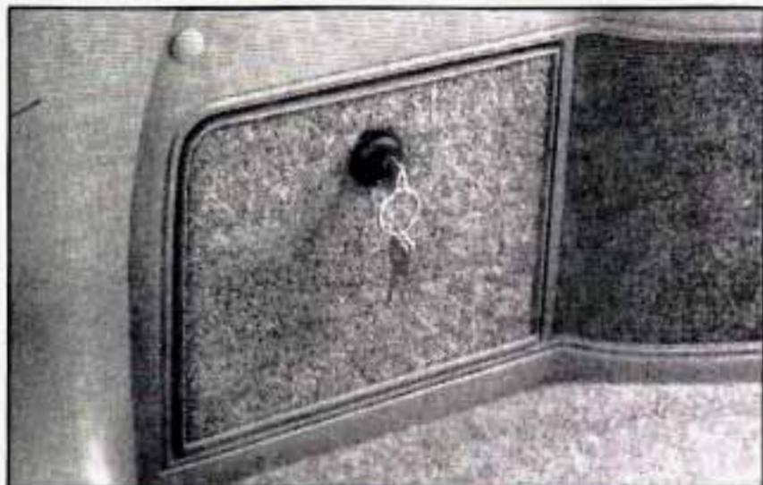
Use your door key to unlock the storage bin on the driver's side near the liftgate.
