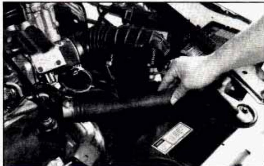
7. Start the engine and let it run until you can feel the upper radiator hose getting hot. Watch out for the engine fan.
