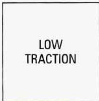
When your anti-lock system is adjusting brake pressure to help avoid a braking skid, the LOW TRACTION light will come on.
