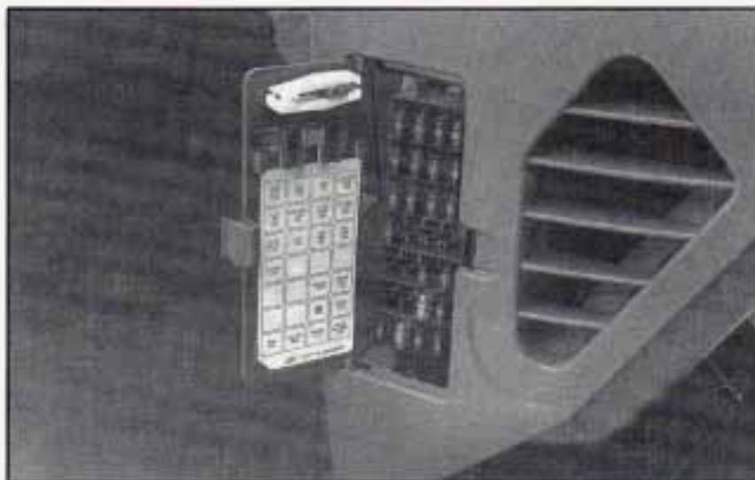
There is a fuse panel located at the end of the instrument panel near the driver's door.
