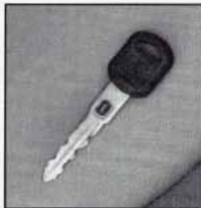
Your vehicle is equipped with the PASS-Key<sup>®</sup> II (Personalized Automotive Security System) theft deterrent system. PASS-Key<sup>®</sup> II is a passive theft deterrent system.
