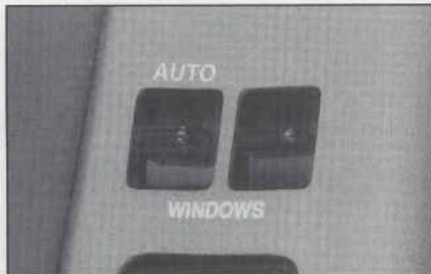
Your power window controls are on the armrest. The switch for the driver's window has an express-down feature. Pull the switch back all the way, release it and the window will lower automatically. To stop the window from lowering, push the switch forward. To partially open the window, pull the switch back and quickly release it.
