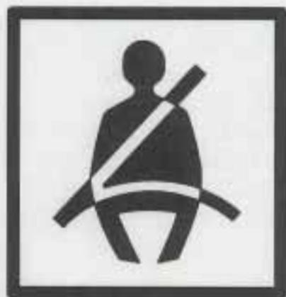
When the key is turned to RUN or START, a chime will come on for about eight seconds to remind people to fasten their safety belts. The safety belt light will also come on and stay on for about 70 seconds. If the driver's belt is already buckled, neither the chime nor the light will come on.
