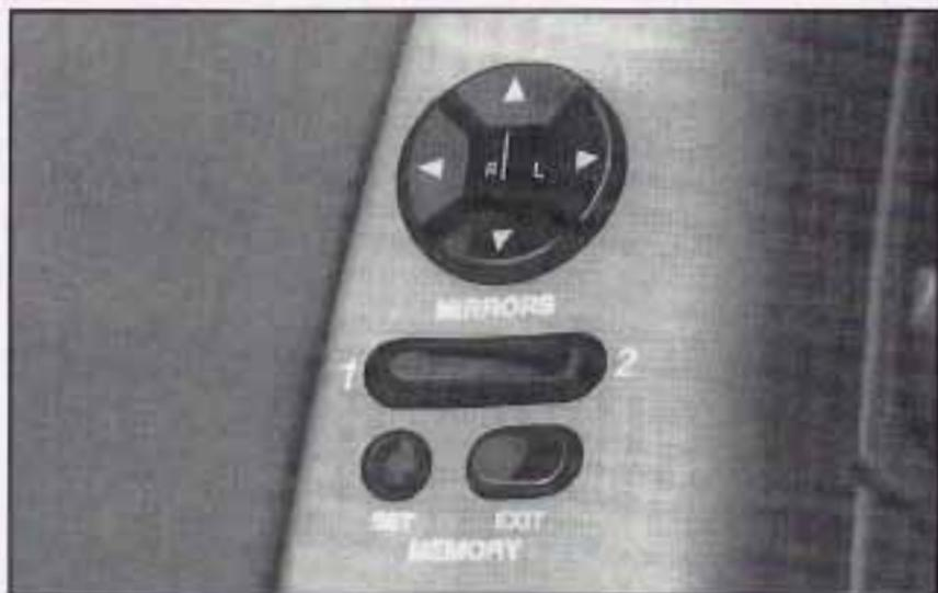
Your Buick has an electric mirror control located on the driver's door armrest.
