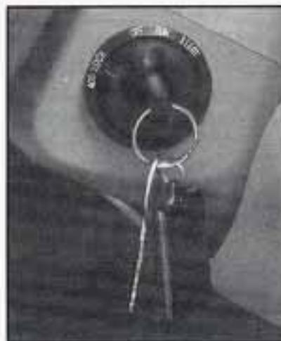
The key with the black plastic head operates the ignition lock.
