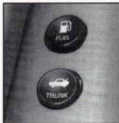
Press the TRUNK release button located below the driver's door handle to release the trunk lid. The trunk will open if the transaxle is in PARK (P) and if the trunk security release is not in the OFF position.
