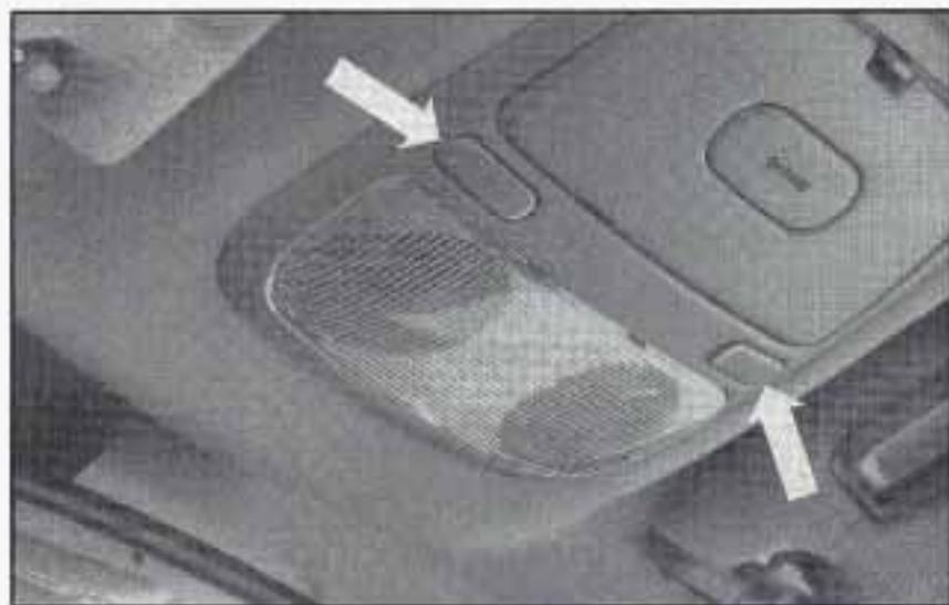
Turn on the front seat reading lamp by pressing the switch. Press it again to turn off the lamp.
