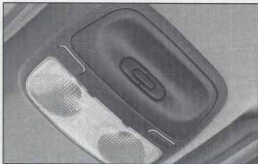
Your vehicle may come equipped with this transmitter located in the overhead console. It allows you to consolidate the functions of up to three individual hand-held transmitters. It will “learn” and transmit the frequencies of most current transmitters and is powered by your vehicle’s battery and charging systems.
