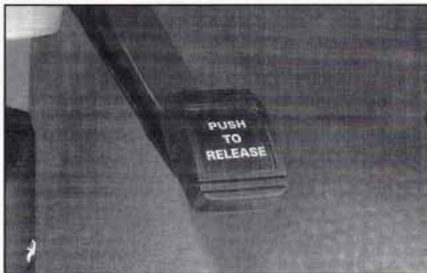
**To set the parking brake:** Hold the regular brake pedal down with your right foot. Push down the parking brake pedal with your left foot. If the ignition is on, the brake system warning light will come on.
