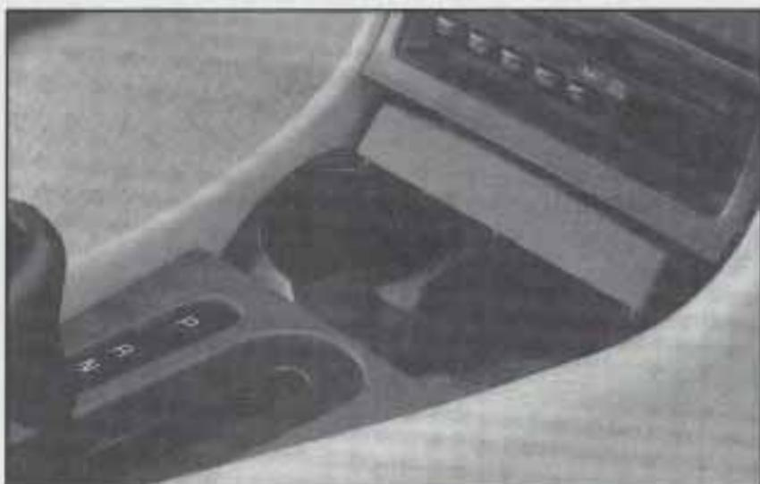
The center console has space for cassette storage, a removable coinholder and a cupholder. The cupholder is in front of the storage console. Push forward on the cover of the front storage area and it will open. Press the cover and it will close.
