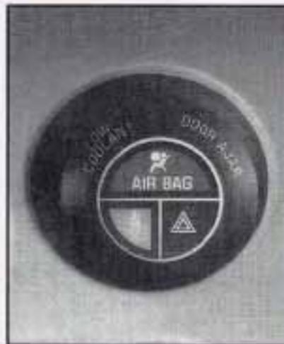
There is an air bag readiness light on the instrument panel, which shows AIR BAG.
