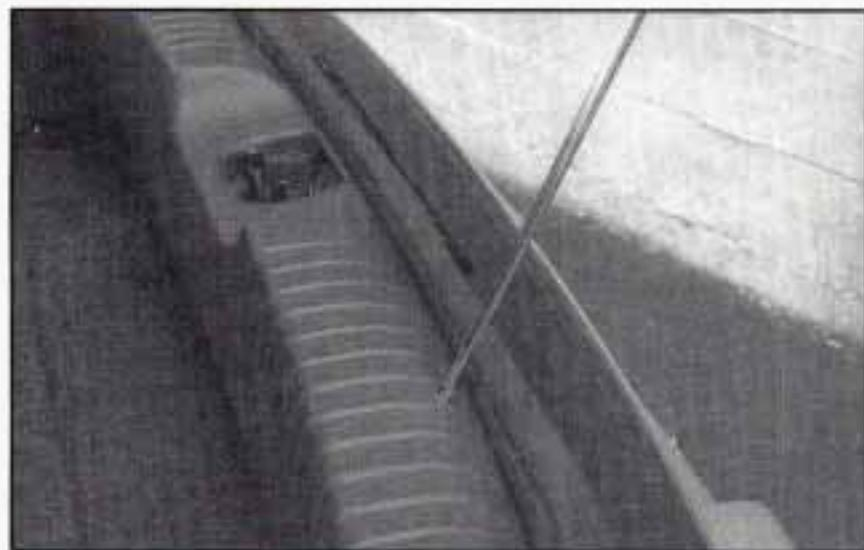
1. Remove the screws that secure the trunk trim over the taillamp area.
