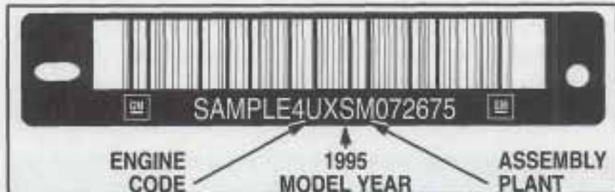
This is the legal identifier for your Buick. It appears on a plate in the front corner of the instrument panel, on the driver's side. You can see it if you look through the windshield from outside your vehicle. The VIN also appears on the Vehicle Certification and Service Parts labels and the certificates of title and registration.
