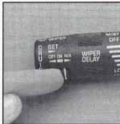
1. Move the cruise switch from ON to R/A. Hold it there until you get up to the speed you want, and then release the switch.
