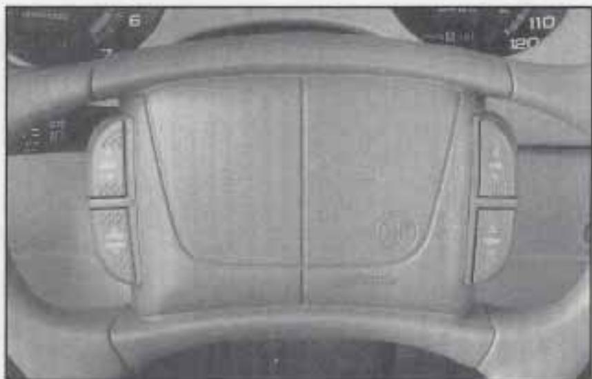
If your vehicle has this feature, you can control certain radio and comfort control functions using the pads on the steering wheel.
