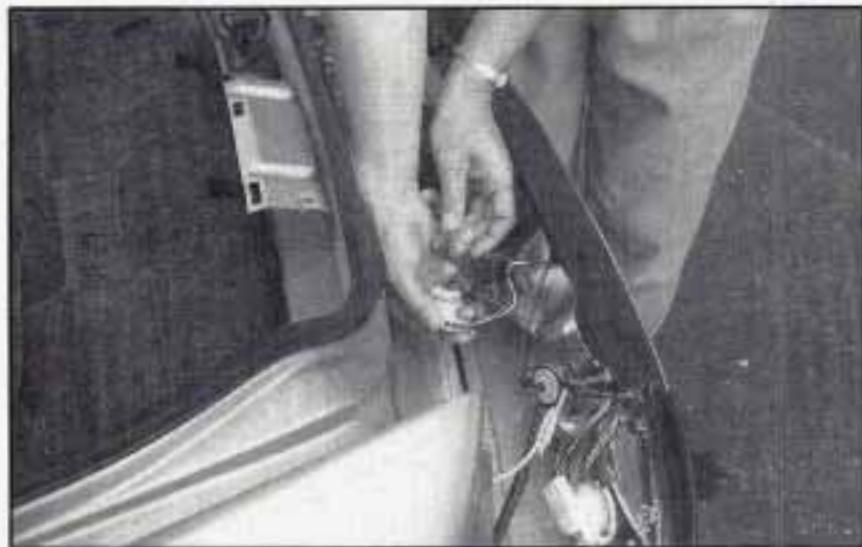
5. Pull the bulb straight out to remove it from the socket.
