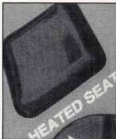
If your vehicle has this option, the switch is on the driver's armrest. Press the button once and the seat will warm up. The HI light on the button will come on.
