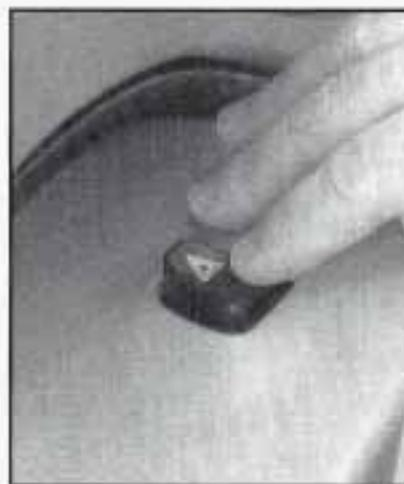
Press down on the button located on top of the steering column to make your front and rear turn signal lamps flash on and off.
