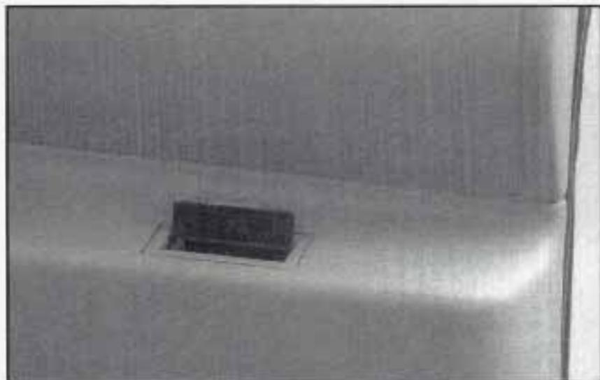
To remove the rear ashtray for cleaning, press down on the snuffer as you pull the ashtray down and out.
