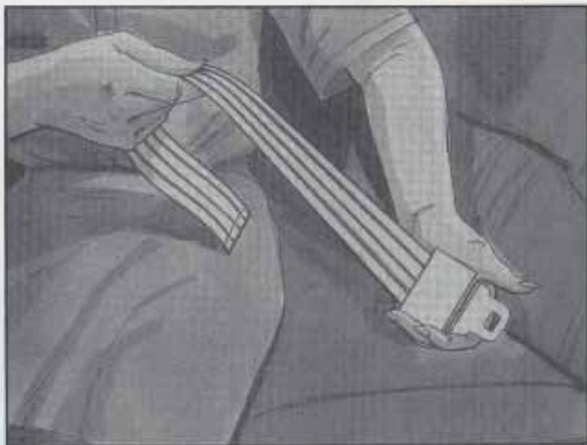
2. Put the restraint on the seat. Follow the instructions for the child restraint.
