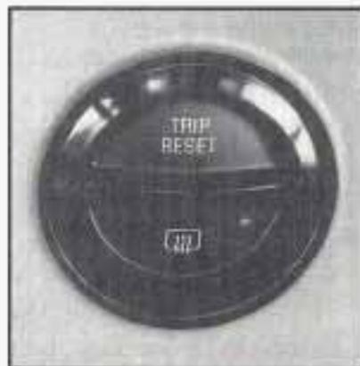
To reset the trip odometer, push the TRIP RESET button.
