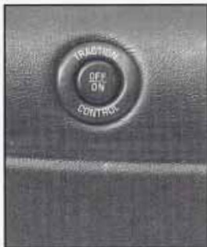
To turn the system off, press the OFF/ON traction control button located to the lower left of the steering column.
