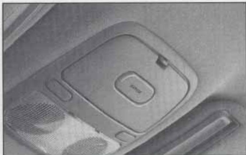
The garage door opener storage area is located in the headliner near the reading lamps. The following chart and instructions will help you install your garage door opener.
