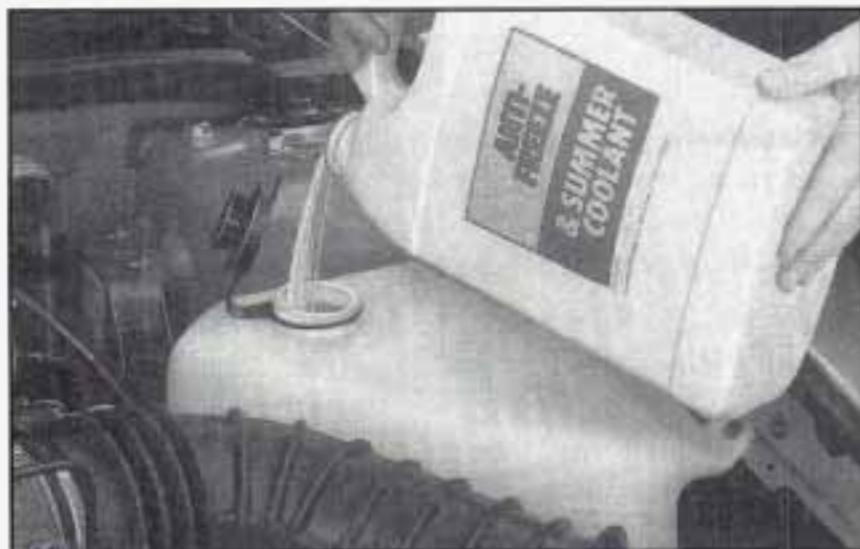
4. Then fill the coolant recovery tank to FULL COLD.
