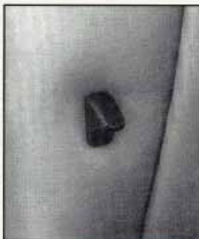
To fold a seatback forward if it does lock in place, push the seatback toward the rear as you lift this latch. Then the seatback will fold forward. The latch must be down for the seat to work properly.
