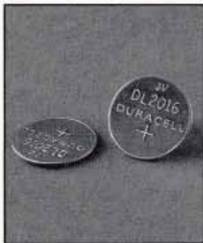
For battery replacement, use two Duracell<sup>®</sup> batteries, type DL-2016, or a similar type.
