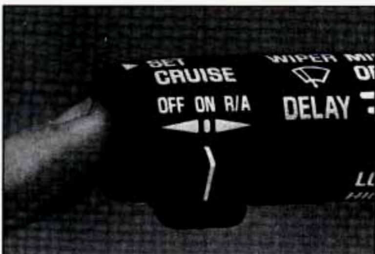
1. Use the accelerator pedal to get to the higher speed. Push the button at the end of the lever, then release the button and the accelerator pedal. You'll now cruise at the higher speed.
