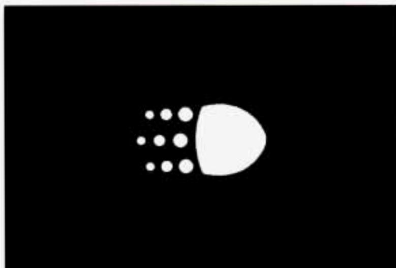
You may have this light on the instrument panel. It goes on whenever the Daytime Running Lamps are on, the ignition is on, the headlamp switch is off, and the parking brake is released.
