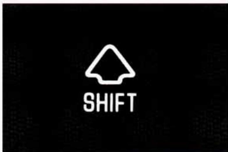
This amber SHIFT indicator light is at the top of the instrument cluster of vehicles with manual transmissions. Shifting when the indicator light is on will help you get the best fuel economy. See “SHIFT Light” in this section.
