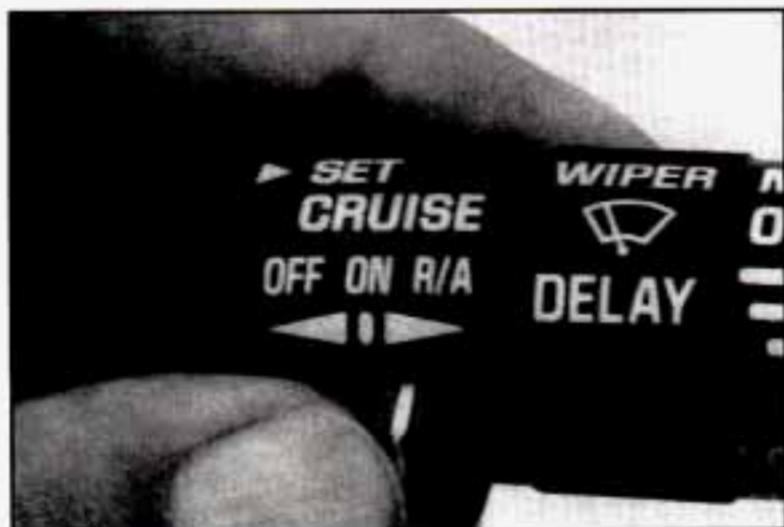
2. Move the Cruise switch from ON to R/A (Resume/Accelerate). Hold it there until you get up to the speed you want, and then release the switch.
