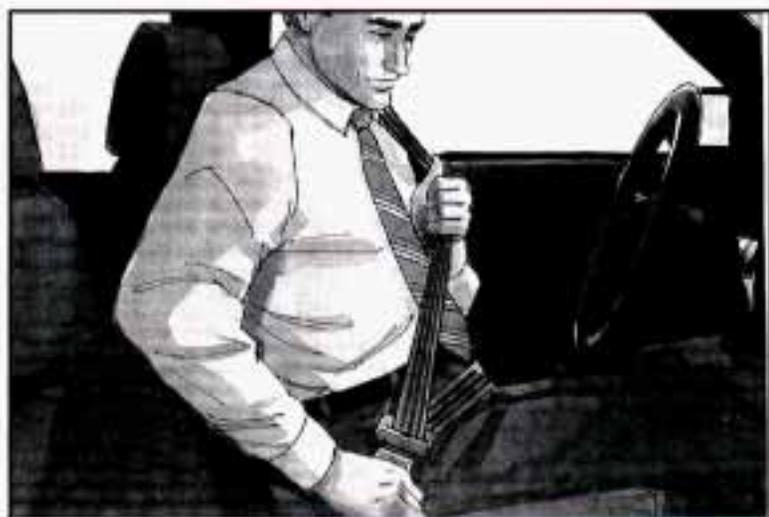
5. To make the lap part tight, pull down on the buckle end of the belt as you pull up on the shoulder belt.
