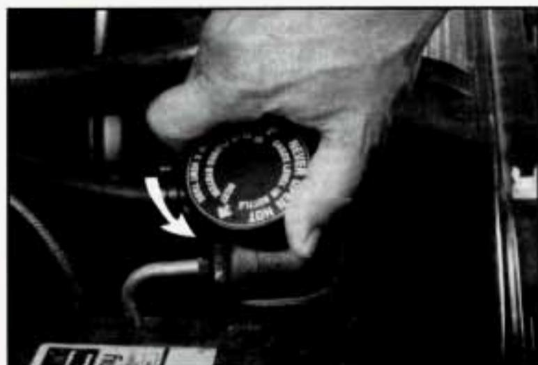
1. You can remove the radiator pressure cap when the cooling system, including the radiator pressure cap and upper radiator hose, is no longer hot. Turn the pressure cap slowly to the left until it first stops. (Don't press down while turning the pressure cap.)
