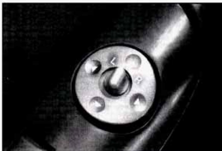
Turn the knob in the switch to L or R to choose the mirror, then press the arrows on the outside switch ring to adjust the mirror.
