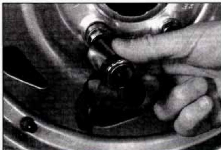
Insert the key and pull the lock case straight off. It is not necessary to turn the key.
