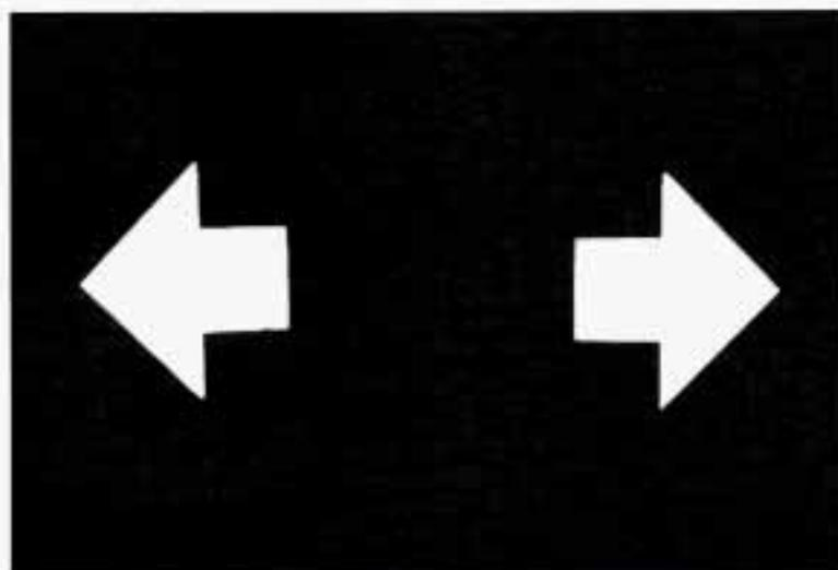
This light with the green arrows is on both sides of the speedometer on the instrument cluster. The turn signal indicator will come on whenever you signal a turn or lane change. See “Turn and Lane Change Signal” in this section.
