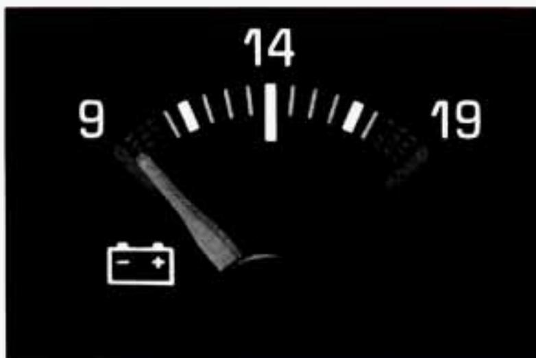
When your engine is not running, but the ignition is on (in the RUN position), this gage shows your battery's state of charge in DC volts.
