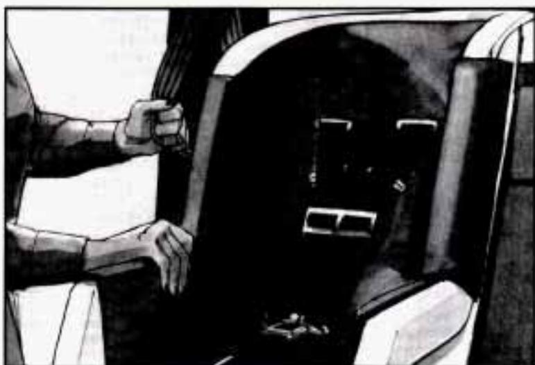
6. To tighten the belt, feed the shoulder belt into the retractor while you push down on the child restraint.
