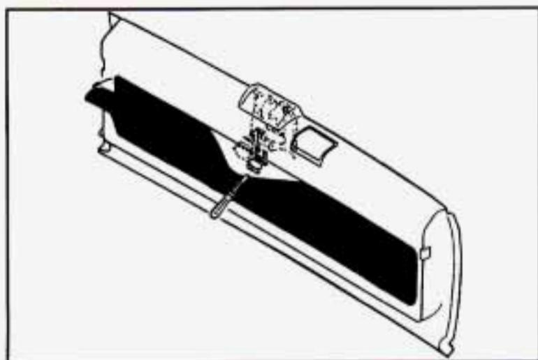
2. Use a thin screwdriver to reach through the access holes in both the trim panel and the hardware cover. Pry the release lever toward the passenger side until the glass latch pops open.
