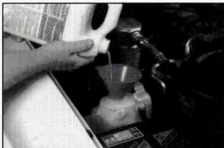
4. Then fill the coolant recovery tank to the ADD mark.
