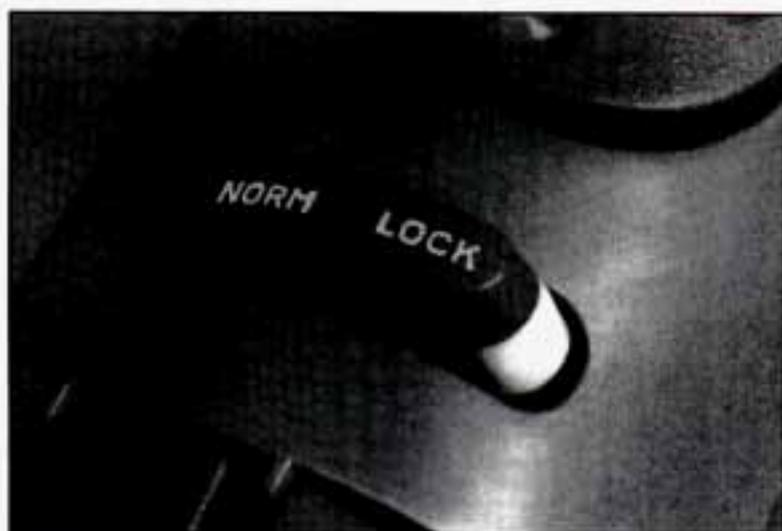
Four-door vehicles have a lockout feature to prevent passengers from operating power windows. It is located on the driver's door. Press LOCK and only the driver can operate all windows. Press NORM and the windows return to normal operation.
