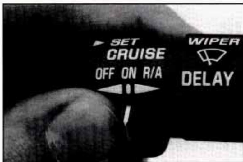
1. Move the Cruise Control switch to ON.
