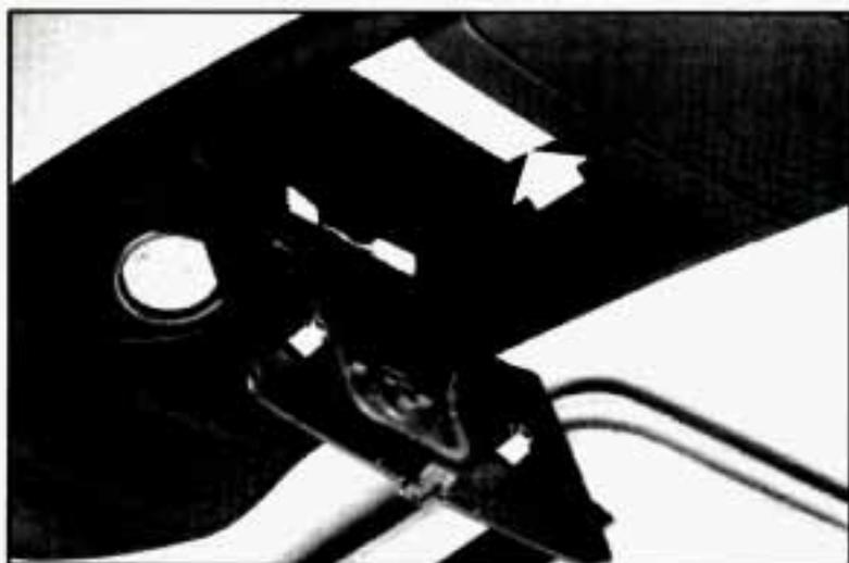
Peel the protective backing from the hook and loop patch. Press it firmly to the back of your garage door opener, as close to the center of the opener as possible.
