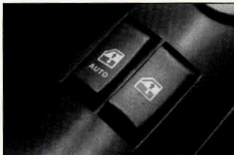
Push the side of the switch with the down arrow to lower the window.
