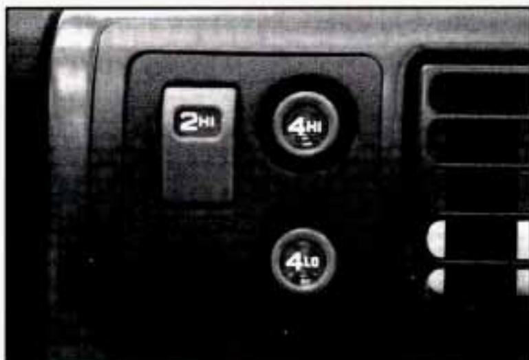
If your four-wheel drive vehicle has the electronic transfer case, the transfer case switches are on the right side of your instrument panel above the radio controls.
