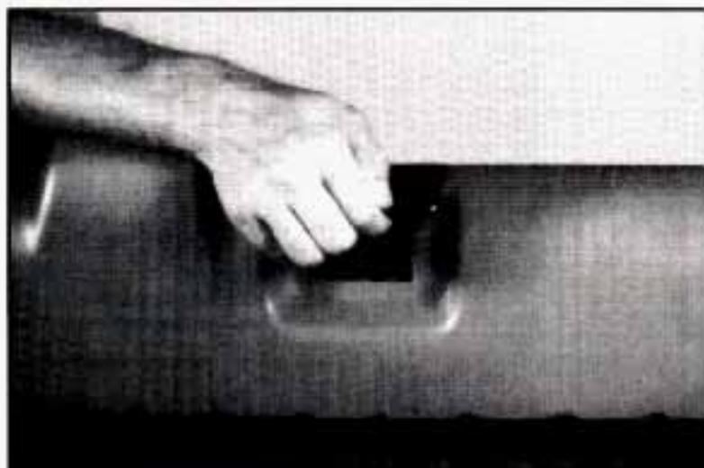
Open the glass and reach inside the endgate to lift the handle and open the endgate.
