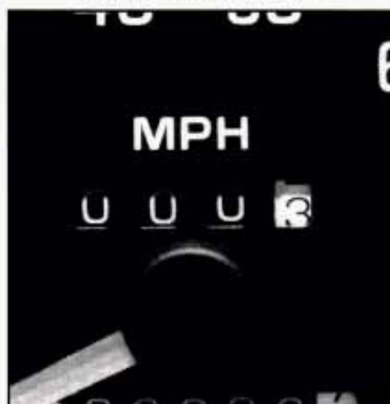
The trip odometer can tell you how far your vehicle has been driven since you last set the trip odometer to zero. Make sure the button is completely depressed.
