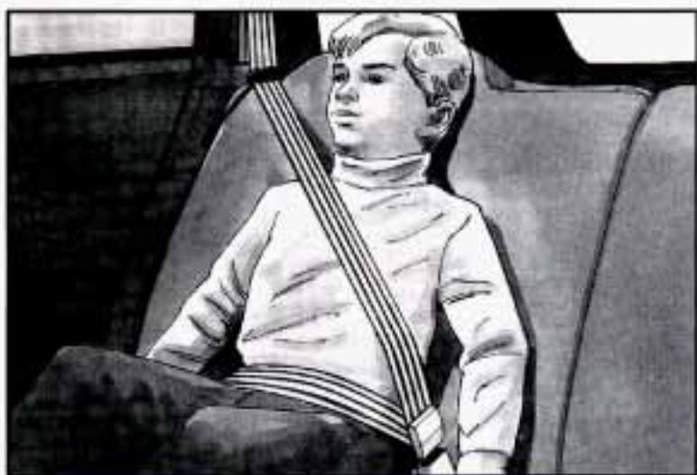
4. Buckle the belt around the child, and make sure that both the lap belt and the shoulder belt are secured properly. Make sure that the shoulder belt crosses the shoulder. See "Safety Belts, Rear Seat Passengers" in the Index.
