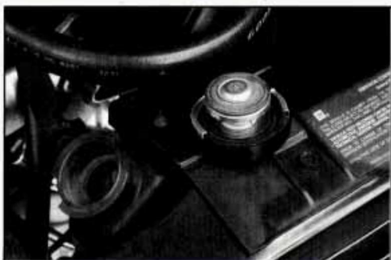
5. Put the cap back on the coolant recovery tank, but leave the radiator pressure cap off.
