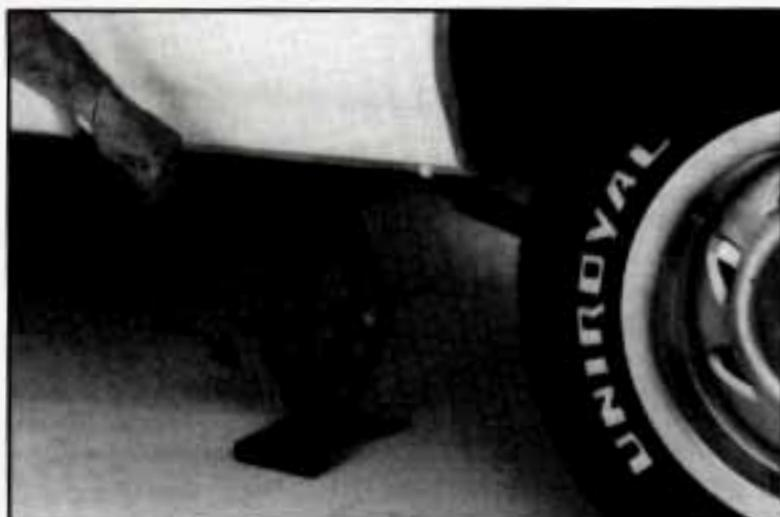
Raise the vehicle by turning the wheel wrench clockwise. Raise the vehicle far enough off the ground so there is enough room for the spare tire to fit.
