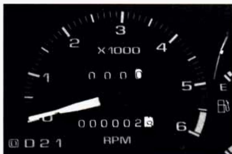
The tachometer displays the engine speed in revolutions per minute (rpm). Each tachometer has a different limit depending on the powertrain in your vehicle. The tachometer has three areas: normal operating range, red warning range, and red danger range.
