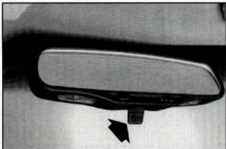
Press the tab under the mirror to reduce glare from headlamps behind you.
