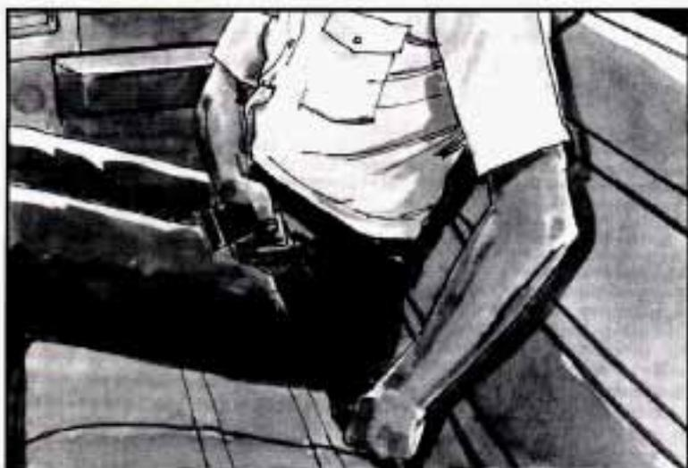
Buckle, position and release it the same way as the lap part of a lap-shoulder belt. If the belt isn't long enough, see "Safety Belt Extender" at the end of this section.
