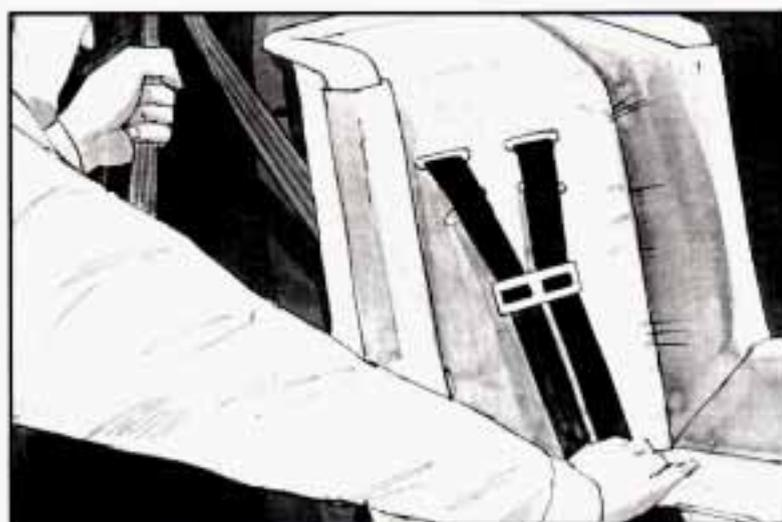
6. To tighten the belt, feed the shoulder belt back into the retractor while you push down on the child restraint.
