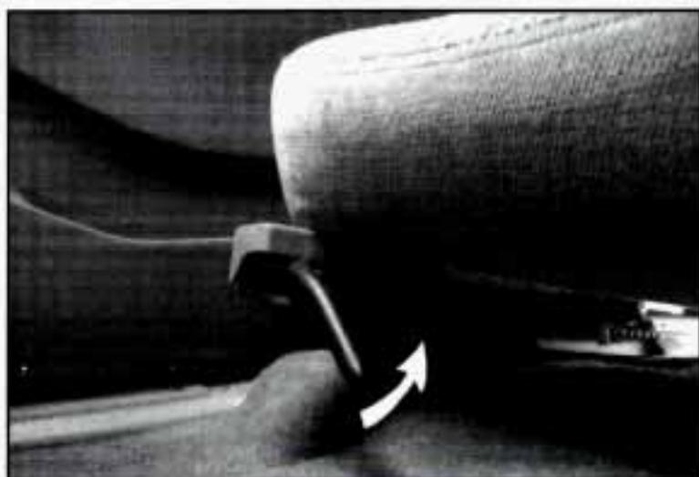
Move the lever under the front of the seat up to unlock it. Slide the seat to where you want it. Then release the lever and try to move the seat with your body to make sure the seat is locked into place.
