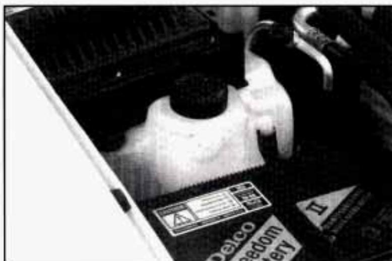
The coolant level should be at the ADD mark. If it isn't, you may have a leak in the radiator hoses, heater hoses, radiator, water pump or somewhere else in the cooling system.
