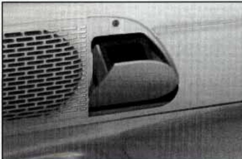
Press on the bottom area to open the rear seat ashtrays in two-door vehicles.
