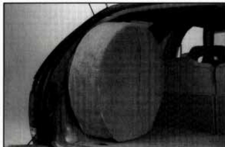
Reach into your tire's cover and unscrew the wingnut at the center of the wheel. Remove it and the retainer.
