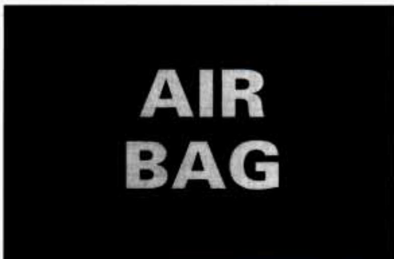
You will see this light flash for a few seconds when you turn your ignition to RUN or START. Then the light should go out. This means the system is ready.
