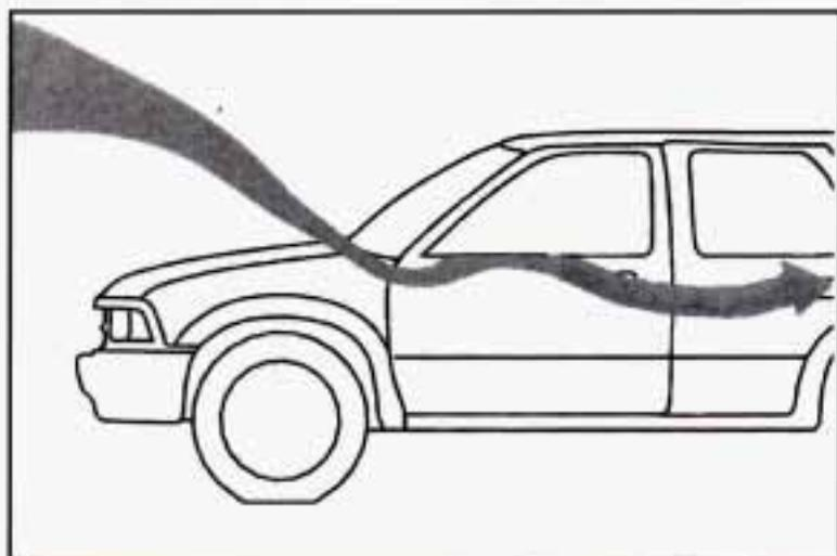
Your vehicle's ventilation system supplies outside air to the inside of your vehicle when it is moving. With the side windows closed, air will flow into the front air inlet grilles, through the vehicle, and out the rear air exhaust valve. Outside air will also enter the vehicle when the heater or the air conditioning fan is running.
