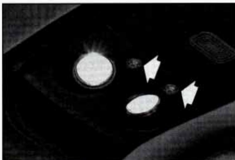
The console has reading lights that turn on and off by pressing in on the button by each light. The lights can also be swiveled to point in the direction you want.
