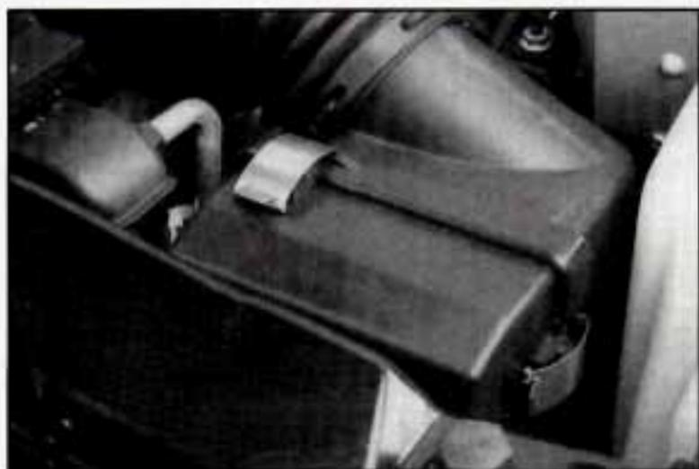
To remove the rectangular air cleaner filter for the 4.3L (VIN W) engine, open both clamps and push the rear of the air cleaner back toward the rear of the engine compartment to change the filter.
