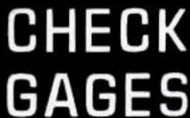
This amber CHECK GAGES light is above the fuel gage on the instrument cluster and will come on briefly when you are starting the engine.
