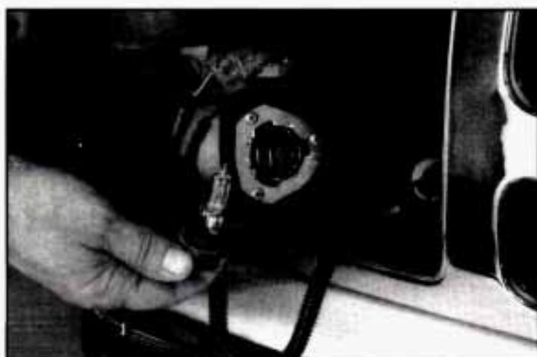
6. Put the new bulb into the headlamp lens assembly and turn it clockwise until it is tight.
