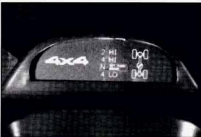
An indicator light near the lever shows you the transfer case settings:
