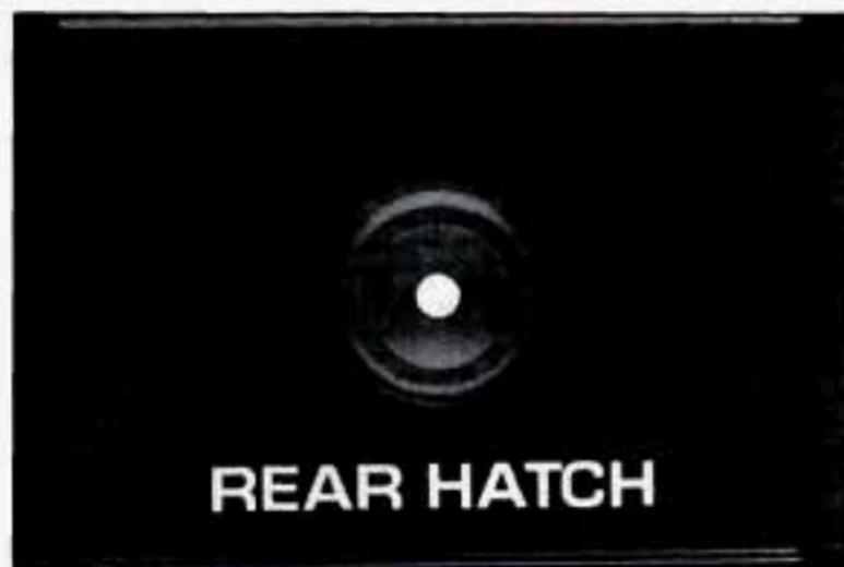
The electric hatch release lets you open your endgate glass by just pressing a button. The button is on the driver's side of the steering column.
