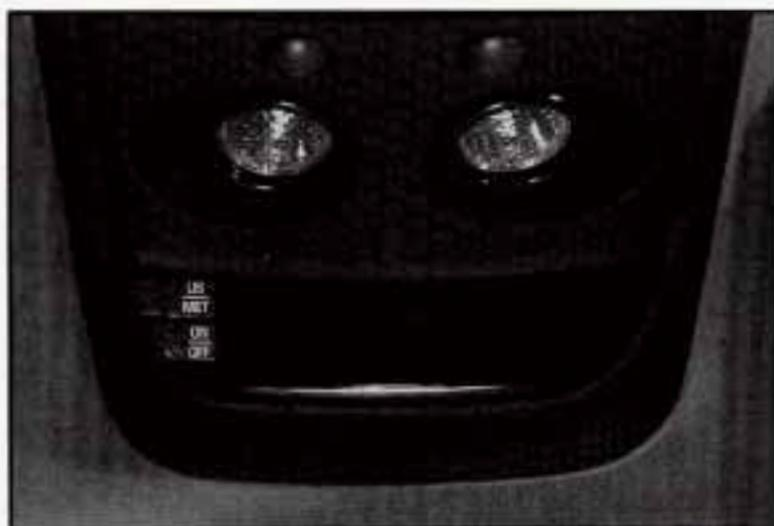
The outside air temperature and the compass are displayed at the front of the overhead console. The control switches are located on the driver's side of the display.
