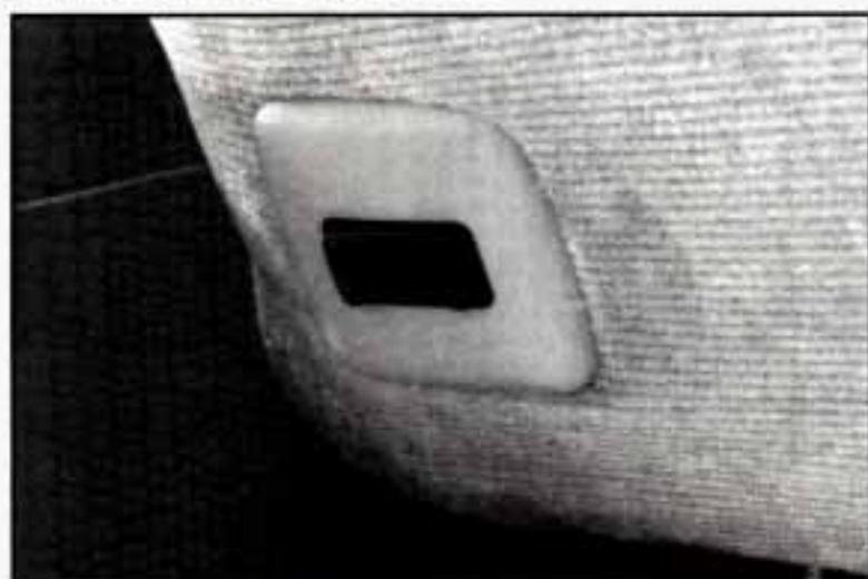
If you have this feature, there will be a control on the front of your driver's seat. Press and hold the passenger's side of the control until you have the desired lumbar support. To decrease lumbar support, press the driver's side of the control.
