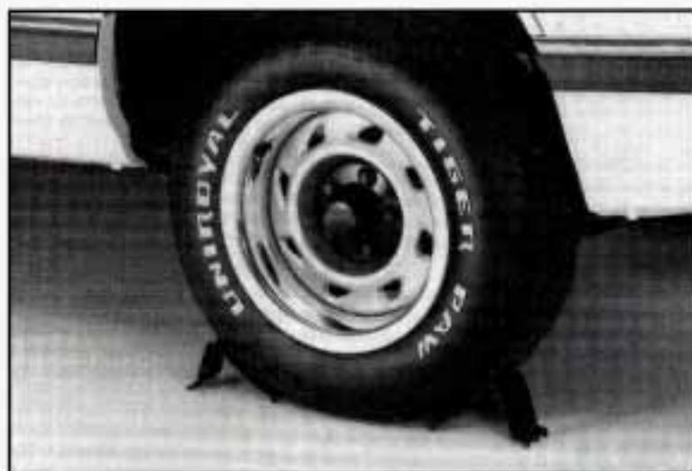
Before you start, block the front and rear of the tire farthest away from the one being changed. Put your spare tire near the flat tire.
