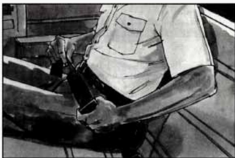
When you sit in the center front seating position, you have a lap safety belt, which has no retractor. To make the belt longer, tilt the latch plate and pull it along the belt.
