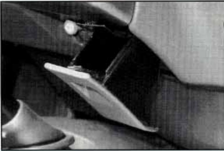
The front ashtray must be completely pulled out to open position before the ashtray cover opens and smoking material can be deposited.
