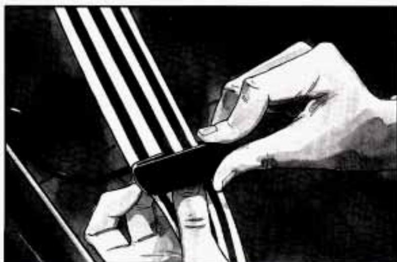
2. Slide the guide under and past the belt. The elastic cord must be under the belt. Then, place the guide over the belt, and insert the two edges of the belt into the slots of the guide.
