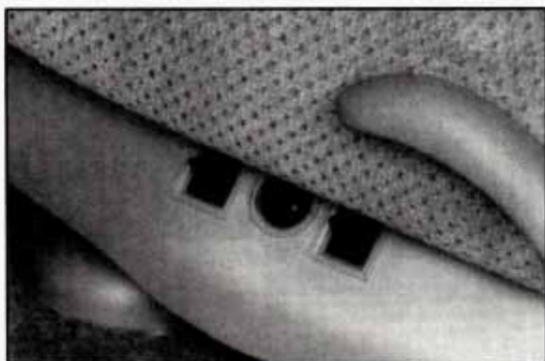
The left control makes the rear of the seat go up and down.
