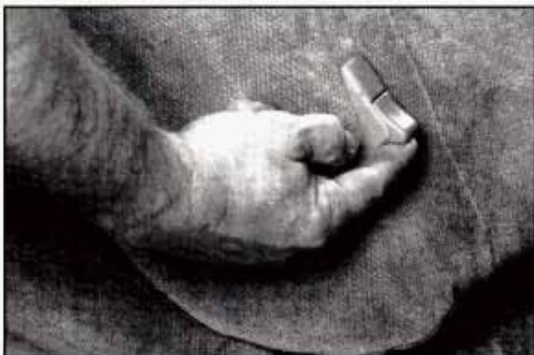
To fold a front seatback forward, push the seatback toward the rear as you lift this latch. Then the seatback will fold forward. The latch must be down for the seat to work properly.
