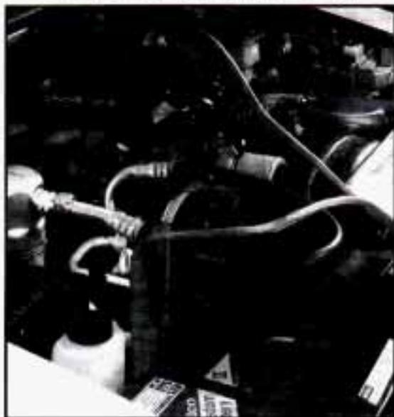
9. Attach the cable at least 18 inches (45 cm) away from the dead battery, but not near engine parts that move. The electrical connection is just as good there, but the chance of sparks getting back to the battery is much less.
