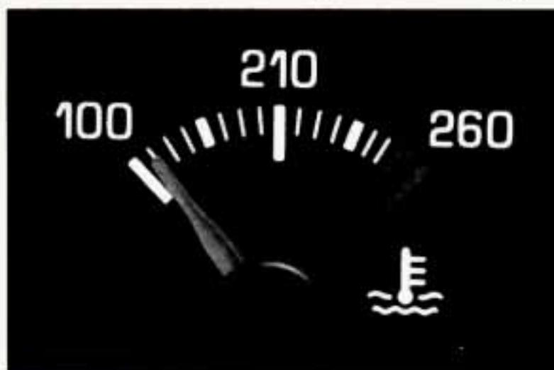
This gage shows the engine coolant temperature. If the gage pointer moves into the red area, your engine is too hot!
