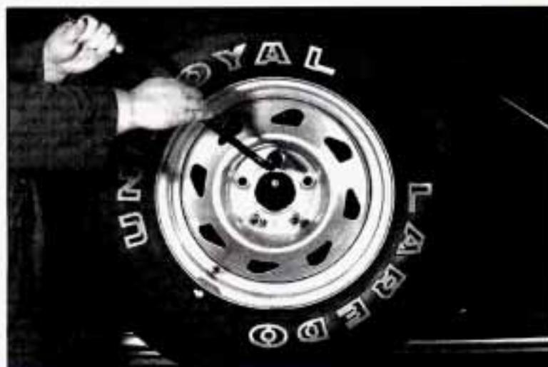
Use the socket end of your wheel wrench to remove the wheel nuts that secure the tire to the carrier. Then, lift the tire off its mounting bracket.
