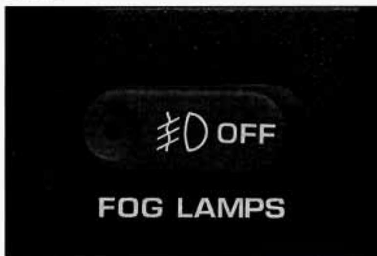
Press the side of the switch with the light to turn the fog lamps on, and OFF to turn them off. A light will glow in the switch when the fog lamps are on.
