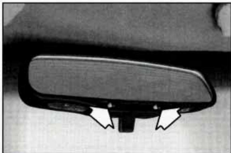
You can also turn the mirror lights on and off by pressing the switch near each light.
