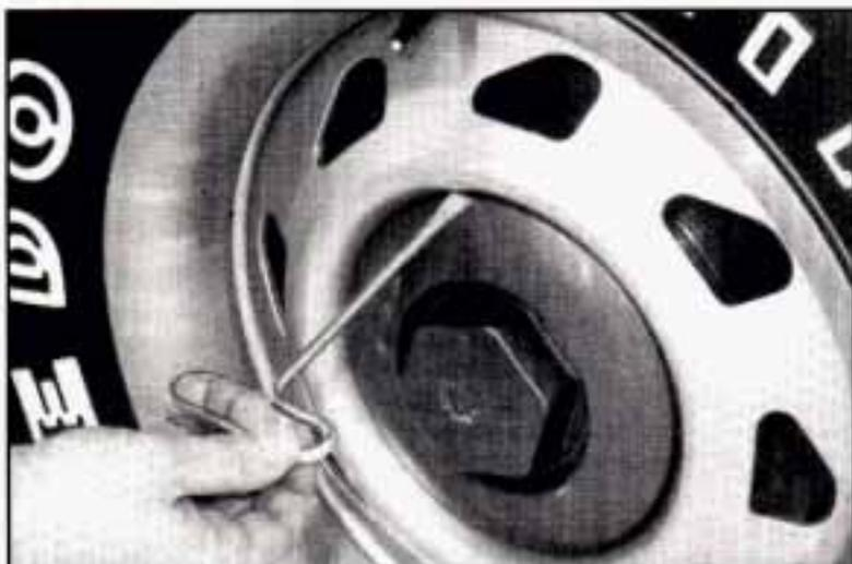
Some jack storage covers are equipped with a hub cap removal tool. Position the hub cap removal tool in the notch and pull straight away from the wheel to avoid potential damage to the hub cap and wheel paint/wheel surface.
