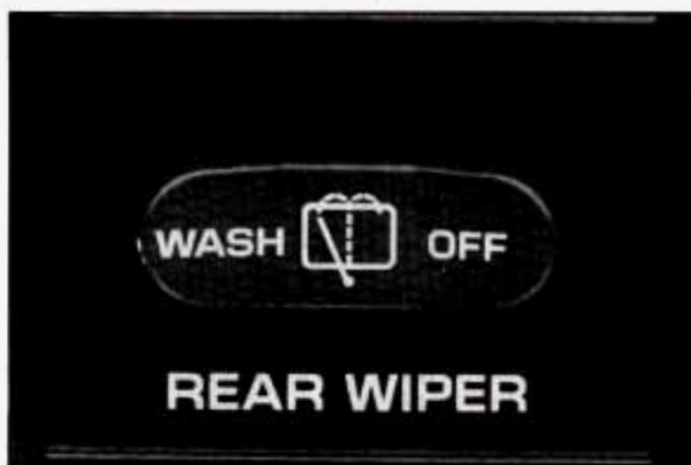
You control your rear window wiper/washer from a switch on your instrument panel located below the rear defogger switch.
