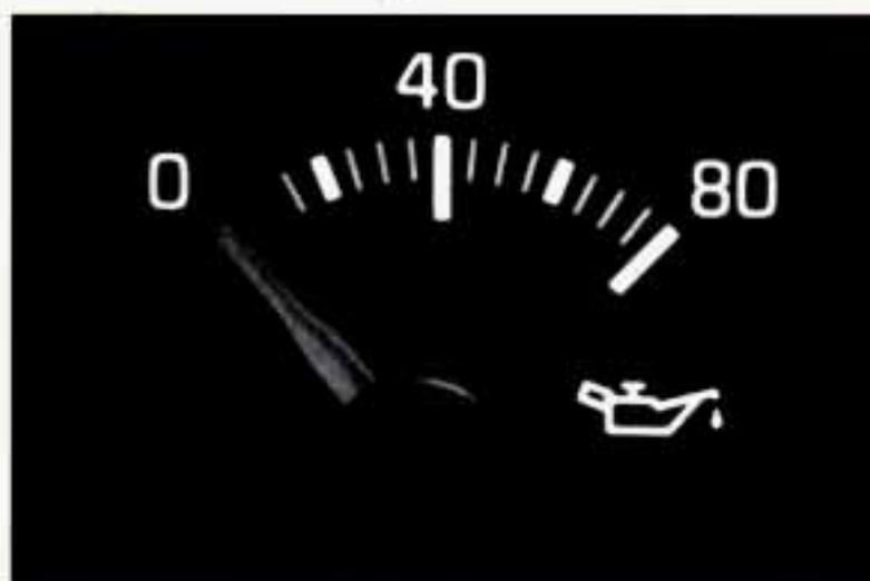
The oil pressure gage shows the engine oil pressure in psi (pounds per square inch) when the engine is running. Canadian vehicles indicate pressure in kPa (kilopascals).
