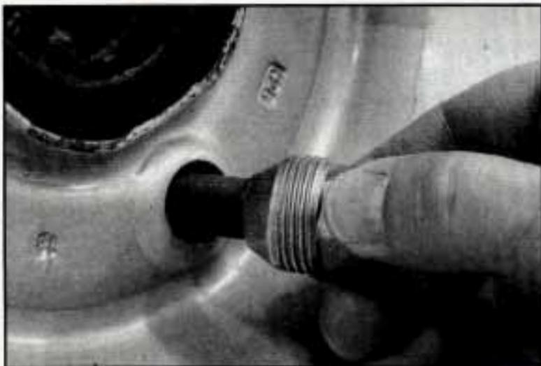
Put the nuts on by hand. Make sure the cone-shaped end is toward the wheel.
