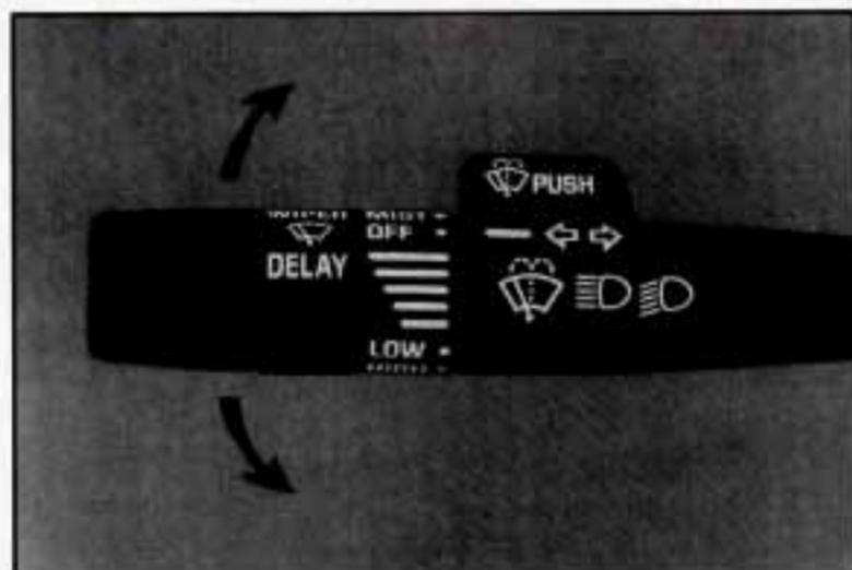
The turn signal has two upward (for Right) and two downward (for Left) positions. These positions allow you to signal a turn or a lane change.
