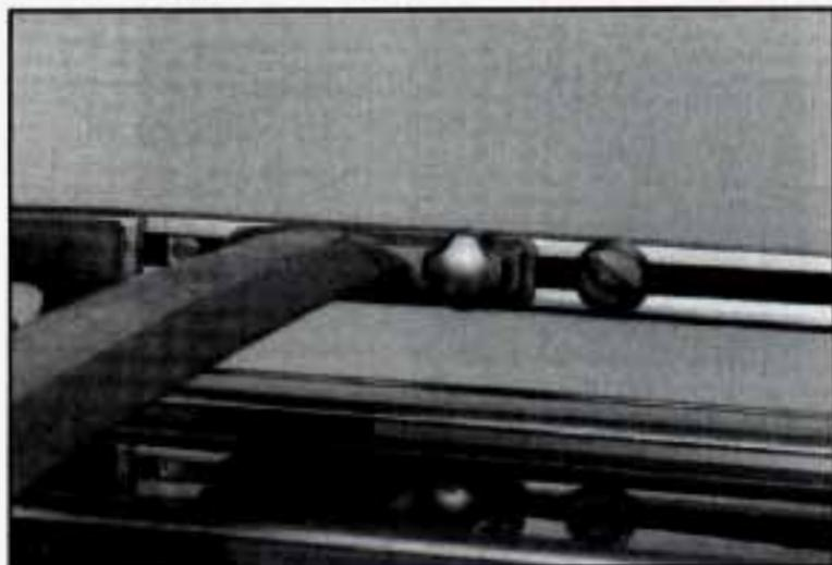
Remove the center rubber strips in the cross rails and attach the GM accessory rack to the nut plates provided through the center slots (four per cross rail).
