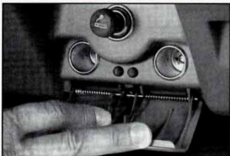
If you have accessory power outlets, you can plug in auxiliary electrical equipment. Just pull down from the top of the door and follow the proper installation instructions that are included with any electrical equipment you install.
