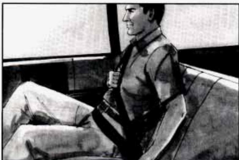
3. To make the lap part tight, pull down on the buckle end of the belt as you pull up on the shoulder part.
