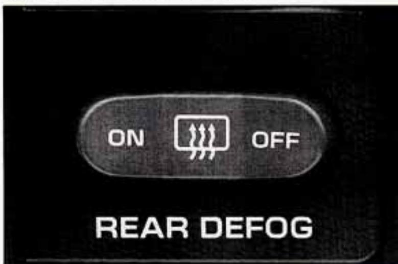
To turn on the rear window defogger, find the switch marked REAR DEFOG on your instrument panel below the headlight switch. Press ON until the light in the switch comes on, then release it.
