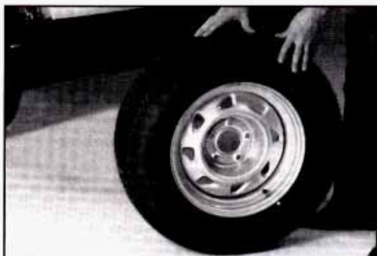
When the tire has been completely lowered, tilt the retainer at the end of the cable and pull it through the wheel opening. Pull the tire out from under the vehicle.
