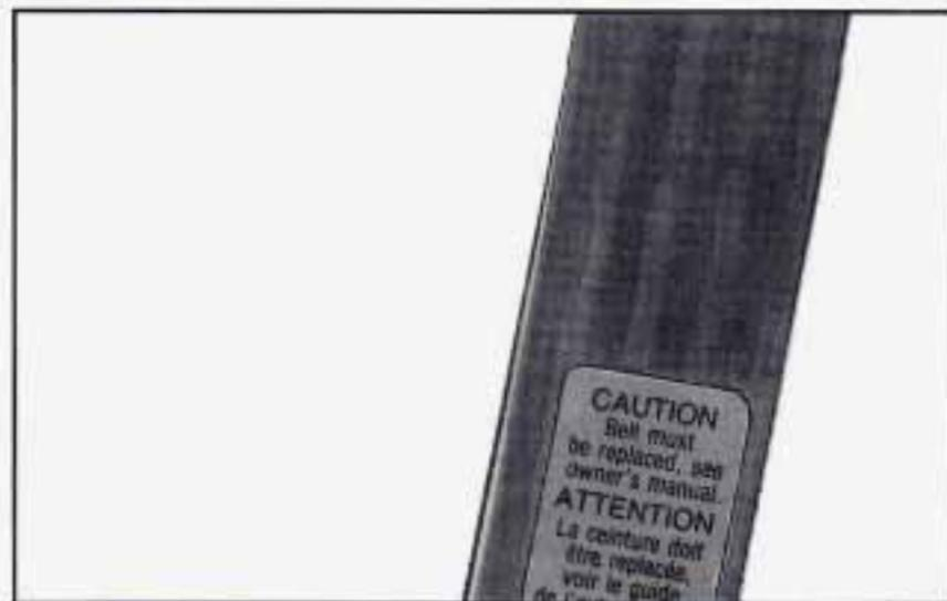
If you ever see a label on the driver's or the right front passenger's safety belt that says to replace the belt, be sure to do so. Then the new belt will be there to help protect you in a collision. You would see this label on the belt near the door opening.
