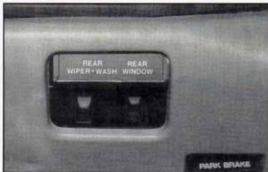
Press the top of the REAR WINDOW switch to unlock the rear window only when the vehicle is in PARK (P) or NEUTRAL (N). You can also unlock the rear window by using the oval key in the lock near the window. This also unlocks the tailgate.
