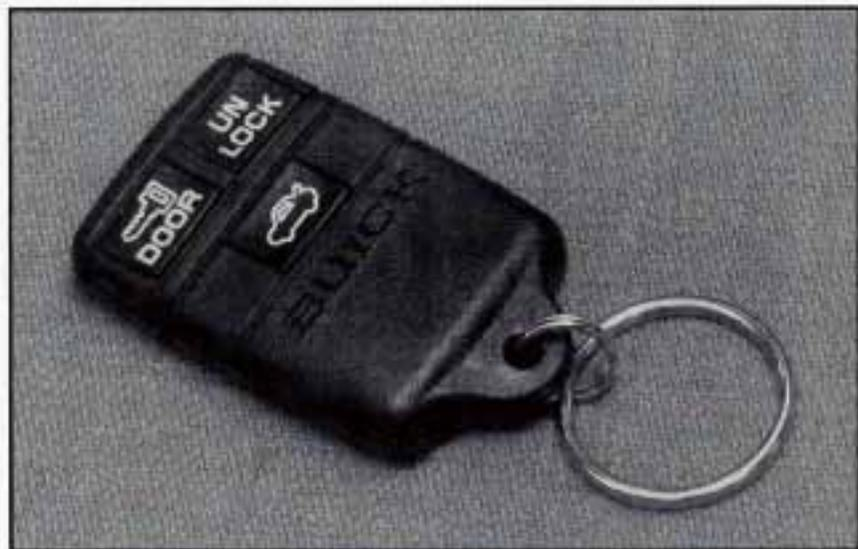
If your Buick has this option, you can lock and unlock your doors or unlock your trunk or tailgate from up to 30 feet (9 m) using the key chain transmitter supplied with your vehicle.
