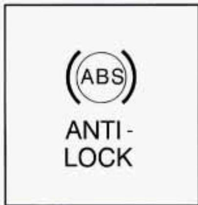
With the anti-lock brake system, this light will come on when you start your engine and may stay on for several seconds. That's normal.
