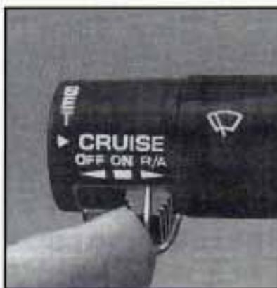
Once you're going about 25 mph (40 km/h) or more, you can move the cruise control switch from ON to R/A (Resume/Accelerate) for about half a second.
