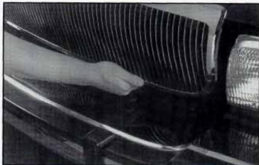
Then go to the front of the vehicle and release the secondary hood release.
