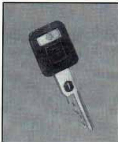
The square key is for the ignition only. It has a bar code attached. Your dealer or qualified locksmith can make extra ignition keys by reading the bar code tag.
