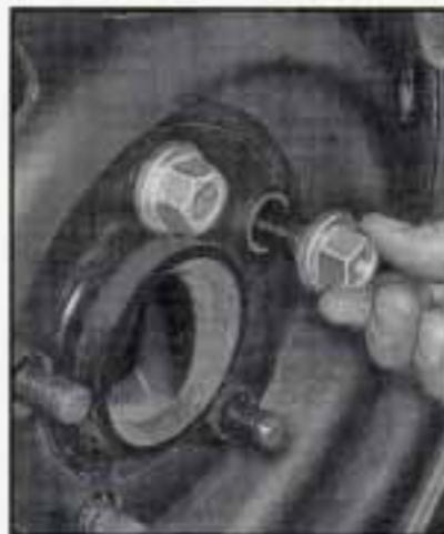
7. Replace the wheel nuts with the rounded end of the nuts toward the wheel. Tighten each nut by hand until the wheel is held against the hub.
