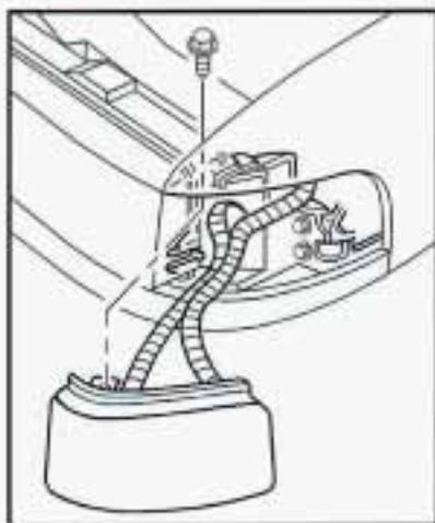
2. Remove the screw from the bracket.
