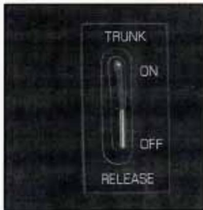
The security switch in the glove box must be ON for the TRUNK button to work.
