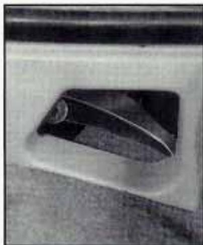
3. Pull the seat release handle in the lower right corner of the storage compartment. The seatback is now unlocked.
