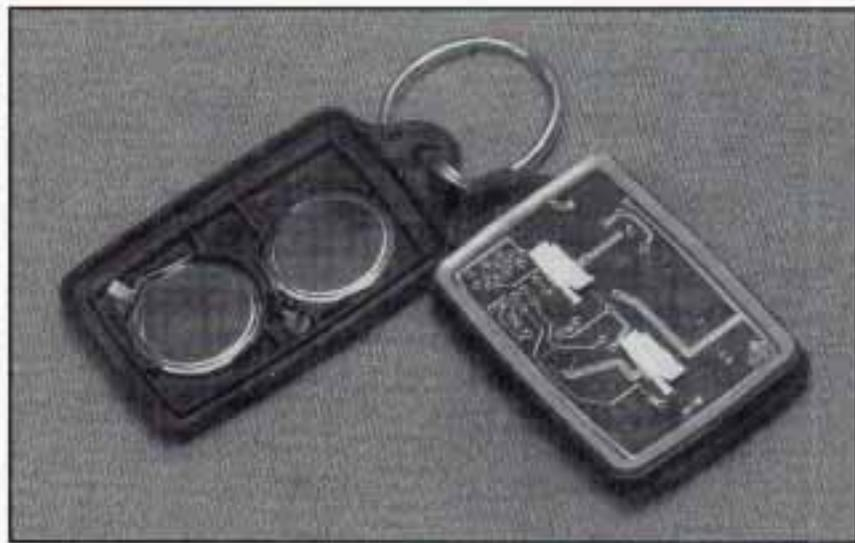
1. If your transmitter has a screw, remove the screw from the back cover. If there is no screw, carefully pry off the cover by inserting a dime (or similar object) in the slot between the covers and twisting.
