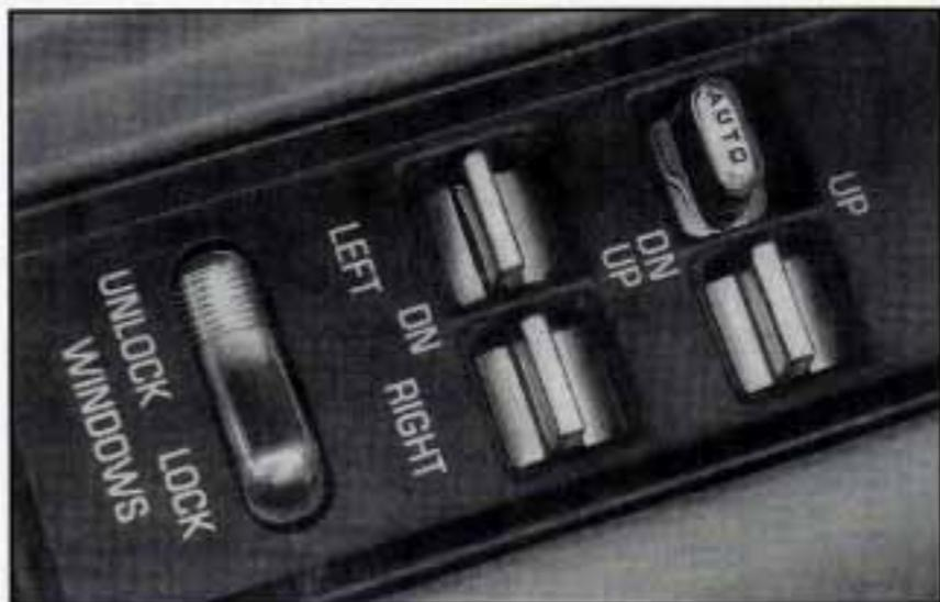
The power windows controls are on the driver's armrest. They control each of the four windows. To open a window, move the switch toward DN. To close it, move the switch toward UP.
