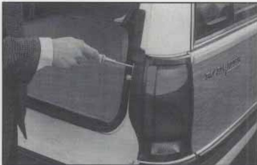
1. Remove the two Phillips<sup>®</sup> head screws.
