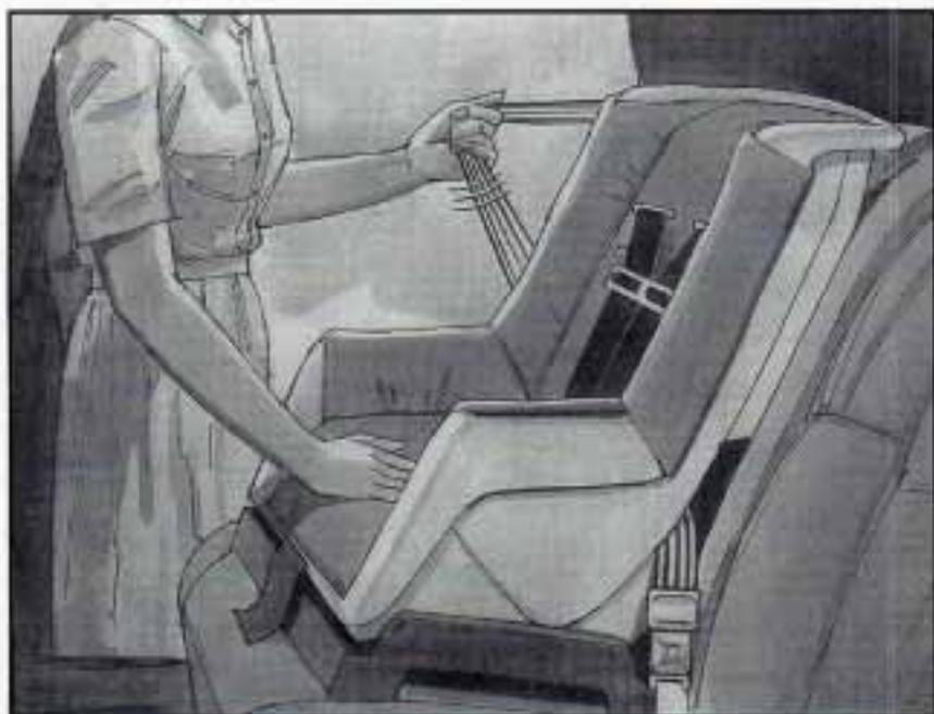
5. To tighten the belt, pull up on the shoulder belt while you push down on the child restraint.
