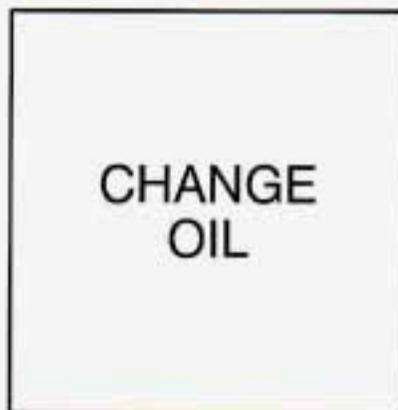
The CHANGE OIL light should come on briefly as a bulb check when you start the engine. If the light doesn't come on, have it serviced.
