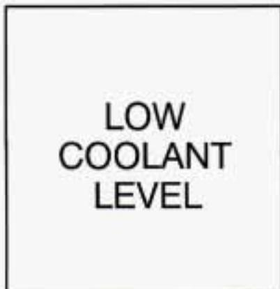
If you have this light and it comes on, the system is low on coolant and the engine may overheat.
