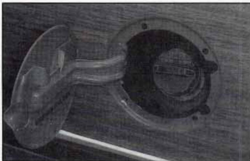
The wagon gas cap is behind a hinged door on the driver's side of your vehicle. While refueling, hang the cap inside the fuel door.
