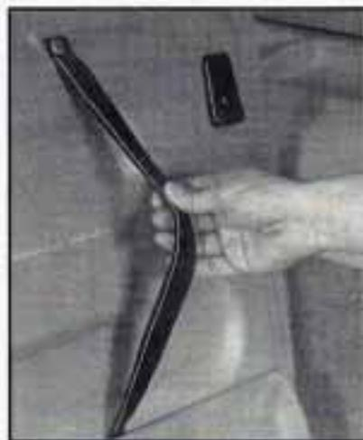
2. Pull the seatback down using the assist strap, then push down on it to lock it into place.
