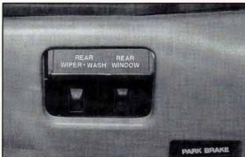
Press the top of the REAR WIPER-WASH switch to turn on the rear wiper. Press the bottom of the switch to turn it off.
