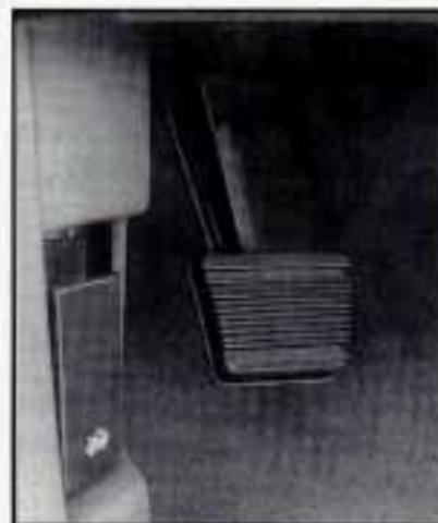
To set the parking brake, hold the regular brake pedal down with your right foot. Push down the parking brake pedal with your left foot. If the ignition is on, the brake system warning light will come on.
