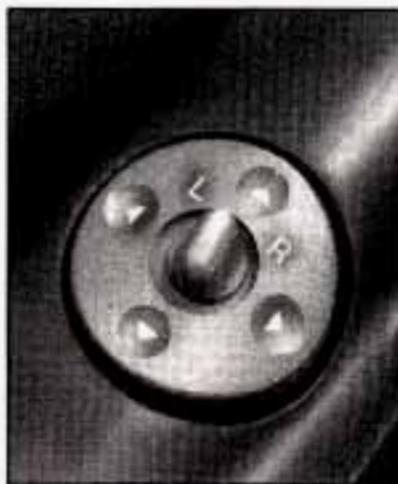
The control is located on the driver's door armrest. Turn the control to L or R to choose the mirror, then press the arrows on the outside switch ring to adjust the mirror.
