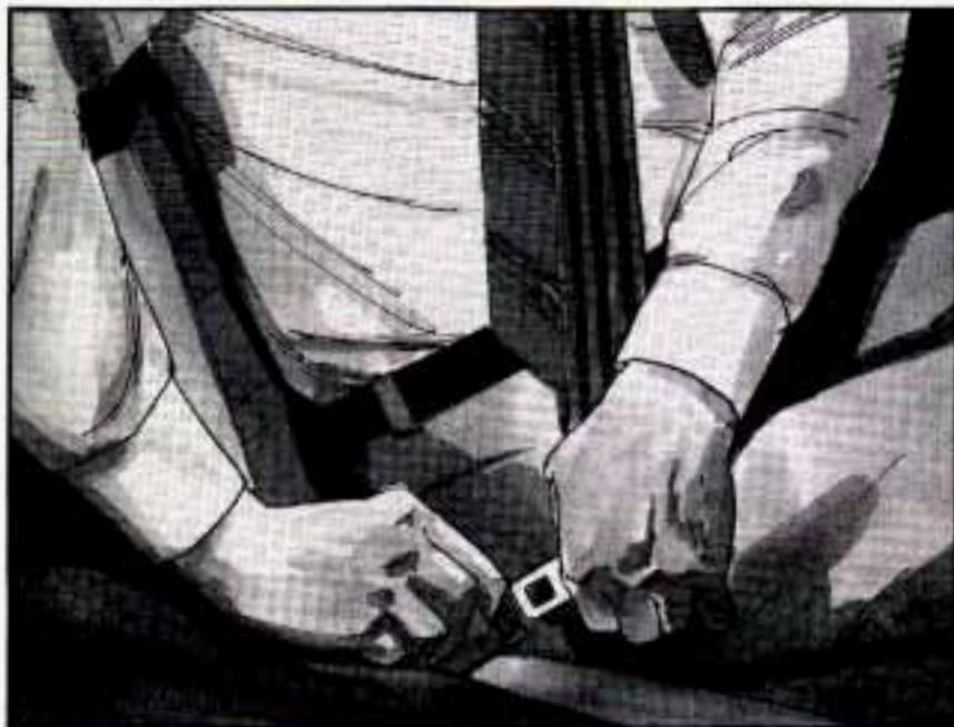
To unclatch the belt, just push the button on the buckle. The belt should go back out of the way.
