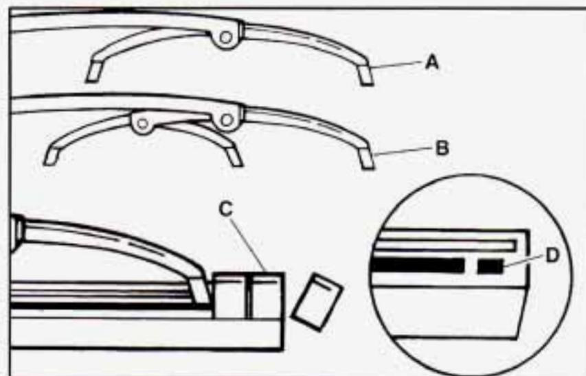
4. To install the new wiper insert, slide the insert (D), notched end last, into the end with two blade claws (A). Slide the insert all the way through the blade claws at the opposite end (B). Plastic caps (C) will be forced off as the insert is fully inserted.
