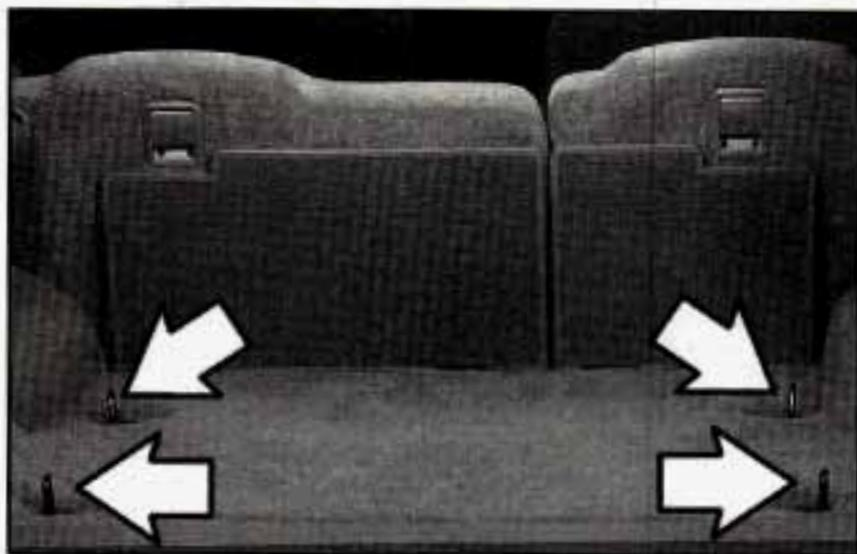
There are four cargo tie downs in the rear that allow you to strap cargo in and keep it from moving inside the vehicle.
