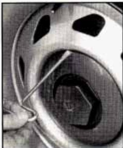
The optional hub cap removal tool is stowed with the jack. Position the hub cap removal tool in the notch and pull straight away from the wheel to avoid potential damage to the hub cap and wheel surface.
