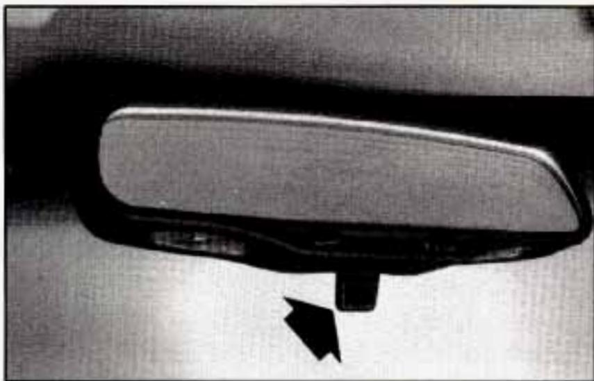
Press the tab under the mirror to reduce glare from headlamps behind you.
