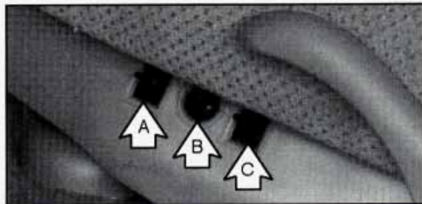
To make the front of the seat move up or down, use control A.
