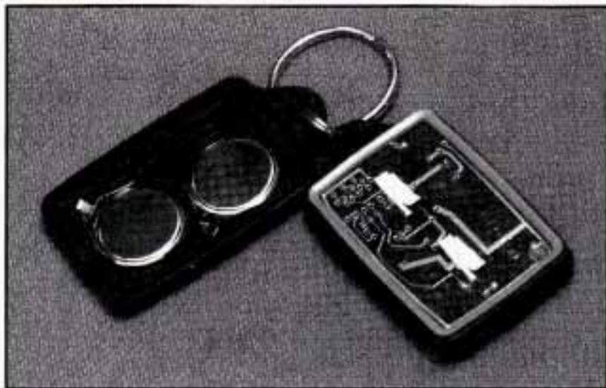
1. Insert a dime in the slot between the covers of the transmitter housing near the key ring hole. Remove the bottom by twisting the dime.
