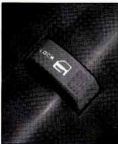
If your vehicle has power door locks, the switch is located on the armrest. Press LOCK to lock all the doors at once.
