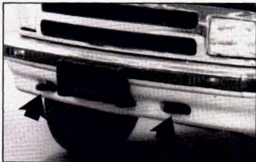
Your vehicle may be equipped with recovery hooks. The recovery hooks are provided at the front of your vehicle. You may need to use them if you're stuck off-road and need to be pulled to some place where you can continue driving.
