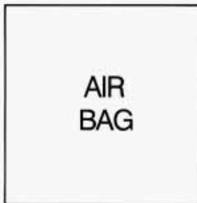
You will see this light flash for a few seconds when you turn your ignition to RUN or START. Then the light should go out. This means the system is ready.
