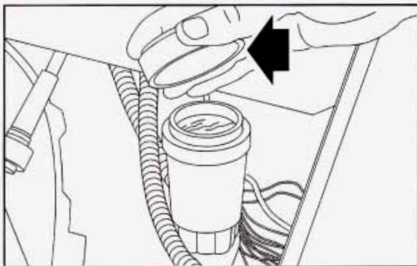
Refer to the Maintenance Schedule, Owners Checks and Services, to determine how often you should check the fluid level in your clutch master cylinder reservoir and for the proper fluid. See "Owner Checks and Services" and "Recommended Fluids and Lubricants" in the Index.
