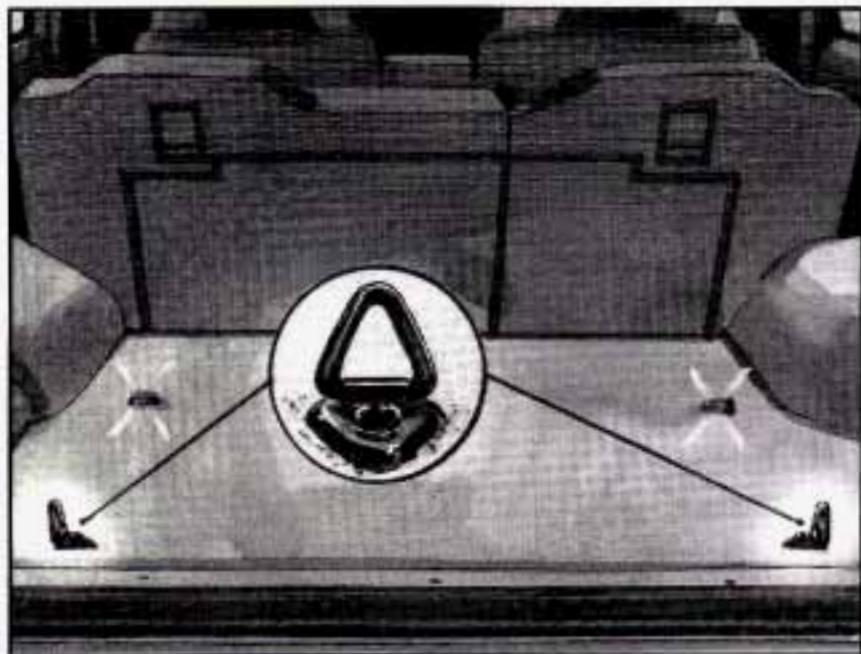
Don't use the front set of tie-down brackets. Anchor the top strap to the rearmost bracket on the same side of the vehicle as the child restraint.
