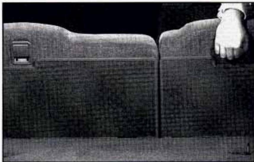
The rear seat release handles are in the upper center of the rear of the seatbacks. Push back on the seatbacks as you pull up on the handles.
