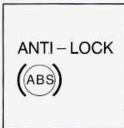
If there's a problem with the anti-lock brake system, this warning light will stay on. See "Anti-Lock Brake System Warning Light" in the Index.
