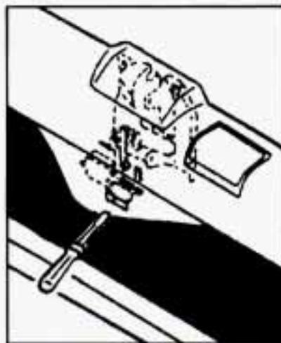
2. Use a thin screwdriver to reach through the access holes in both the trim panel and the hardware cover.
