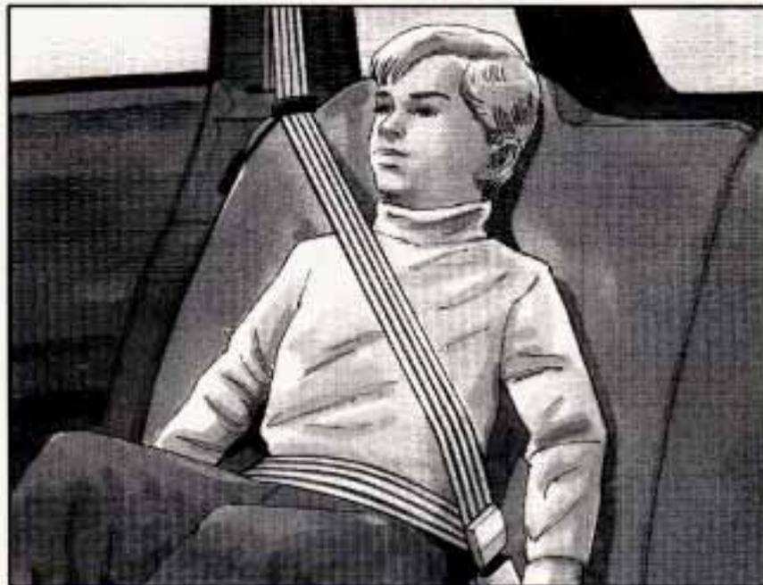
4. Buckle, position and release the safety belt as described in "Rear Seat Outside Passenger Positions" earlier in this section. Make sure that the shoulder belt crosses the shoulder.
