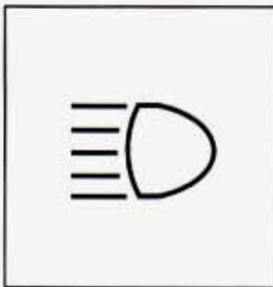
When the high beams are on, this indicator light on the instrument panel also will be on.
