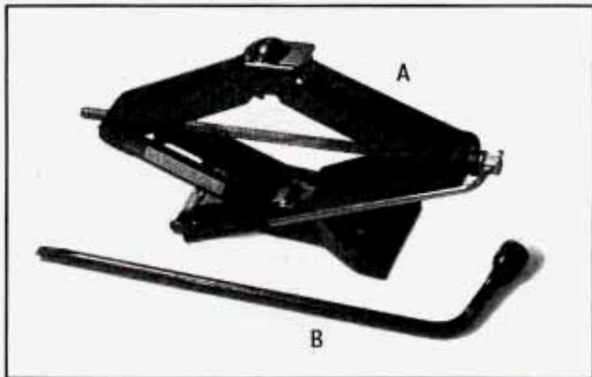
The tools you'll be using include the jack (A) and wheel wrench (B). Your vehicle may also have an optional hub cap removal tool.
