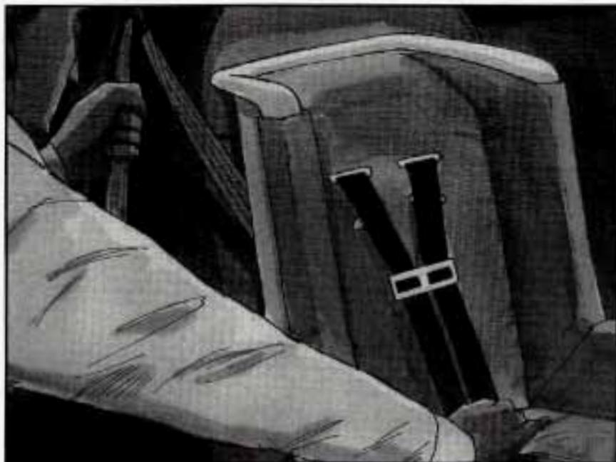
6. To tighten the belt, feed the shoulder belt back into the retractor while you push down on the child restraint.
