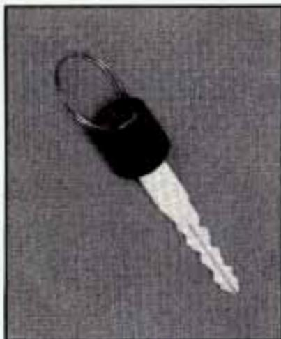
This vehicle has one double-sided key for the ignition, endgate, spare tire lock (two-door vehicles) and door locks. It will fit with either side up.
