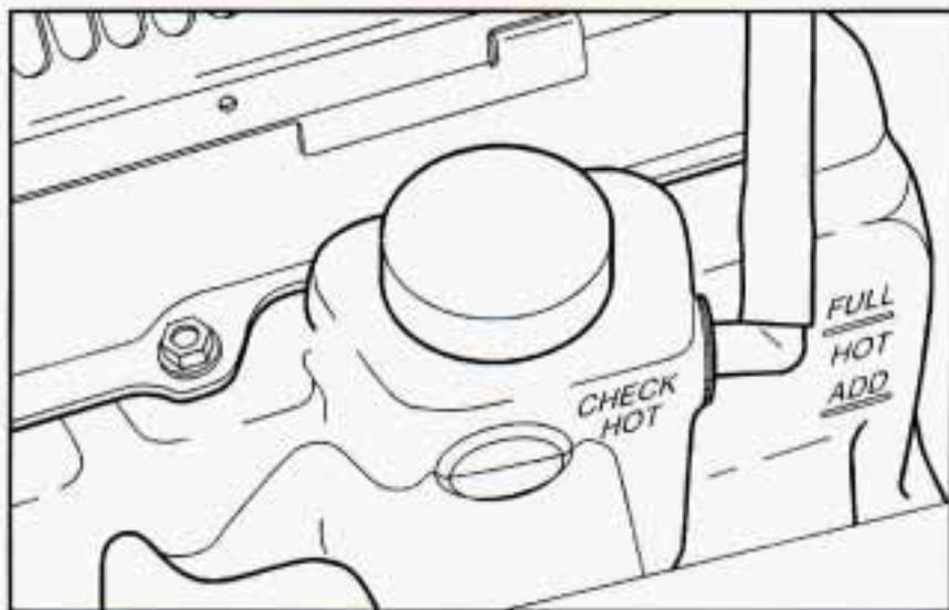
The coolant level should be at the ADD mark. If it isn't, you may have a leak in the radiator hoses, heater hoses, radiator, water pump or somewhere else in the cooling system.
