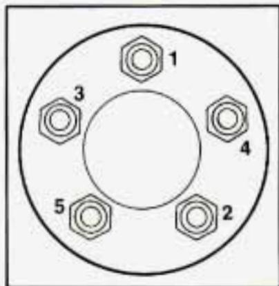
10. Use the wrench to tighten the wheel nuts firmly in a crisscross sequence as shown.
