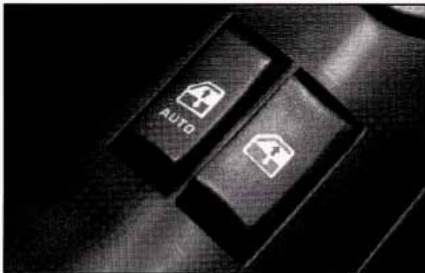
Press the side of the switch with the down arrow to lower the window.
