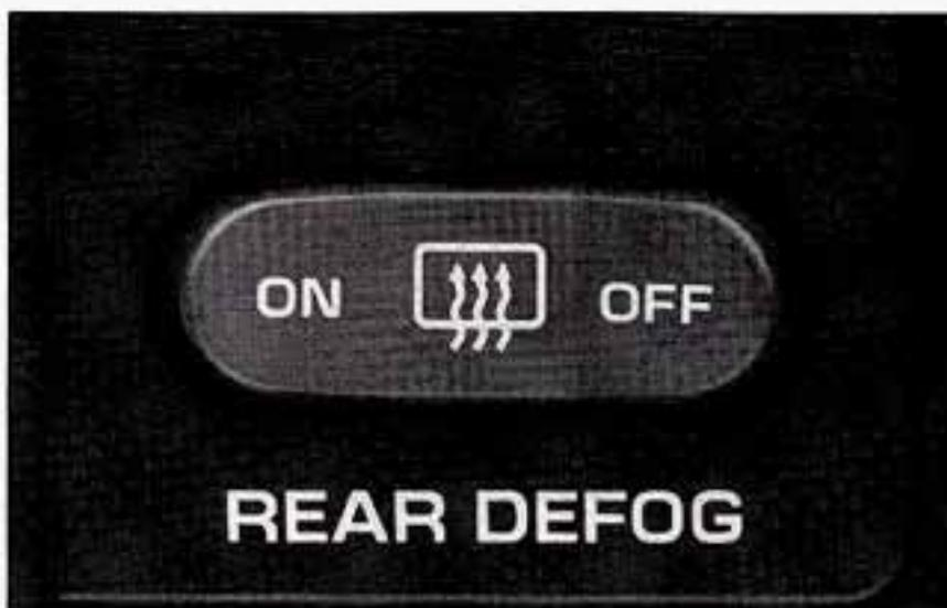
If your vehicle has this option, the rear window will have lines that warm the glass. For best results, clear the window of as much snow or ice as possible before using the rear window defogger.
