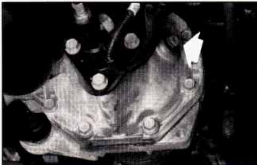
If the level is below the bottom of the filler plug hole, you'll need to add some lubricant.
