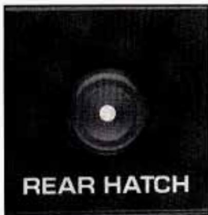
This button on the driver's side of the steering column allows you to release the endgate from inside the vehicle.
