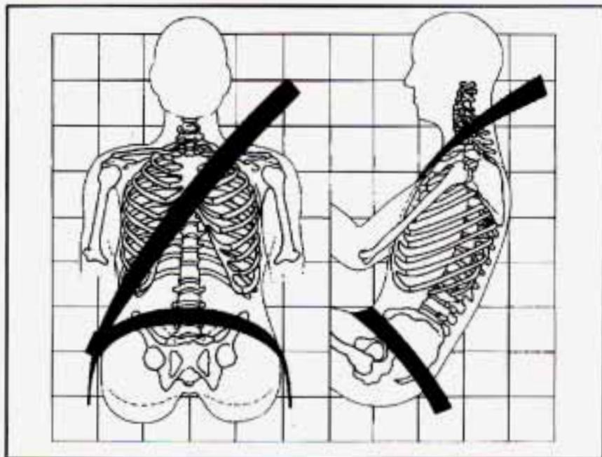
The lap part of the belt should be worn low and snug on the hips, just touching the thighs. In a crash, this applies force to the strong pelvic bones. And you'd be less
