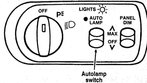
*The autolamp switch is on the left side of the instrument panel.*
