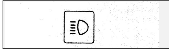
This light comes on when the headlamps are turned to high beam or when you flash the lights.
