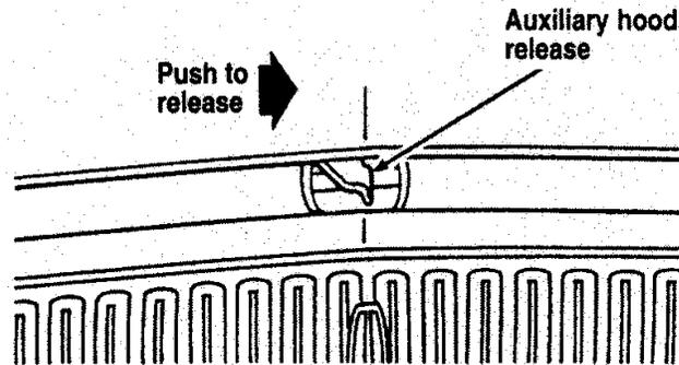
*The auxiliary latch under the front edge of the hood*
