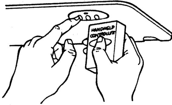
4. When the Universal Transmitter light begins to flash rapidly (this could take up to 60 seconds), release both buttons. You can now use your Universal Transmitter instead of the hand-held controller.
