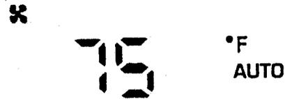
You can override the fan speed at any time. If you use the thumbwheel to override the fan speed, the EATC will continue to control the temperature but you control the fan speed. To return to auto fan control, press the AUTOMATIC button. If you are operating in one of the override functions (FLOOR, MAX A/C, etc.), automatic fan control will continue unless you rotate the fan thumbwheel. To
