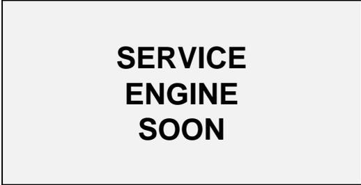
The light comes on briefly when you turn the ignition to the **ON** position, but should turn off when the engine starts. If the light does not come on when you turn the ignition to the **ON** position or if it comes on and stays on when you are driving, have your vehicle serviced as soon as conveniently possible.
