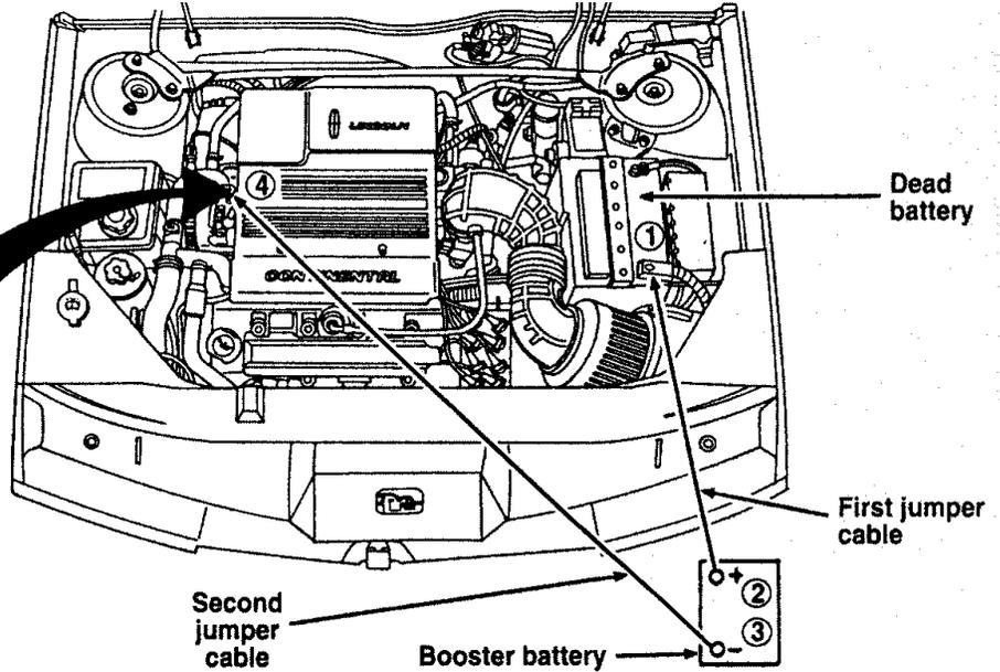
*The engine with jumper cables*
