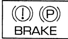
This light comes on when the parking brake is set, or if it is not set, it comes on briefly when you turn the ignition to the START position. It normally goes off shortly after the engine starts and you release the parking brake. If the light stays on after you have fully released the parking brake, have the hydraulic brake system serviced by your dealer or a qualified service technician.
