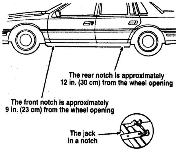
2. Turn the jack handle clockwise until the wheel clears the ground. Remove the wheel lug nuts.
