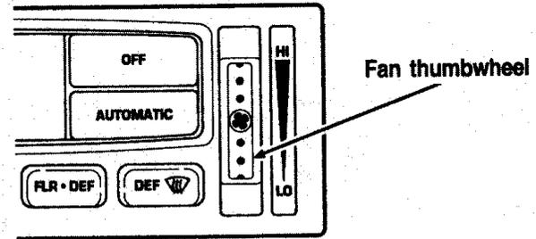
When you move the thumbwheel, the fan speed will go to manual control. The display window will show the
