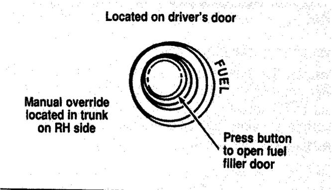
*The remote control fuel filler door release button*
