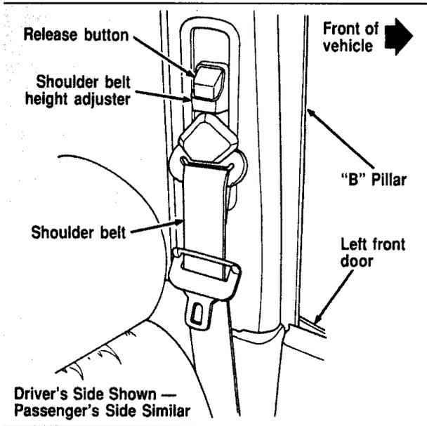
*Figure 1 - The shoulder belt height adjuster*
