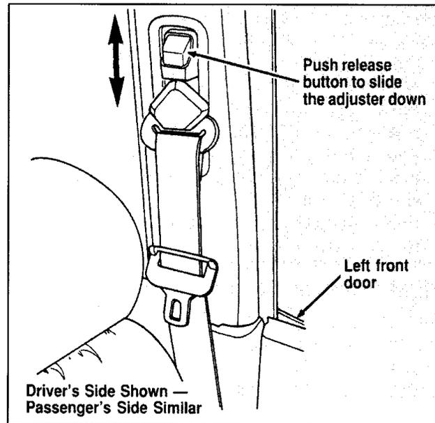
*Figure 2 - The shoulder belt height adjuster*
