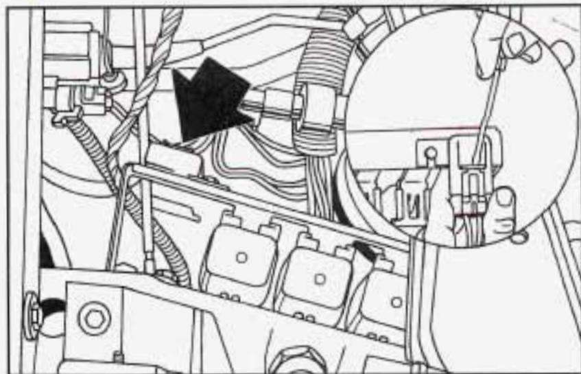
This fuse is located under the hood, on a bracket just behind the passenger's side headlamp. It is mounted on the face of the bracket in the position closest to the passenger's side of the vehicle. The fuse services the injectors, fuel pump, oil pressure sender and fuel pump switch.
