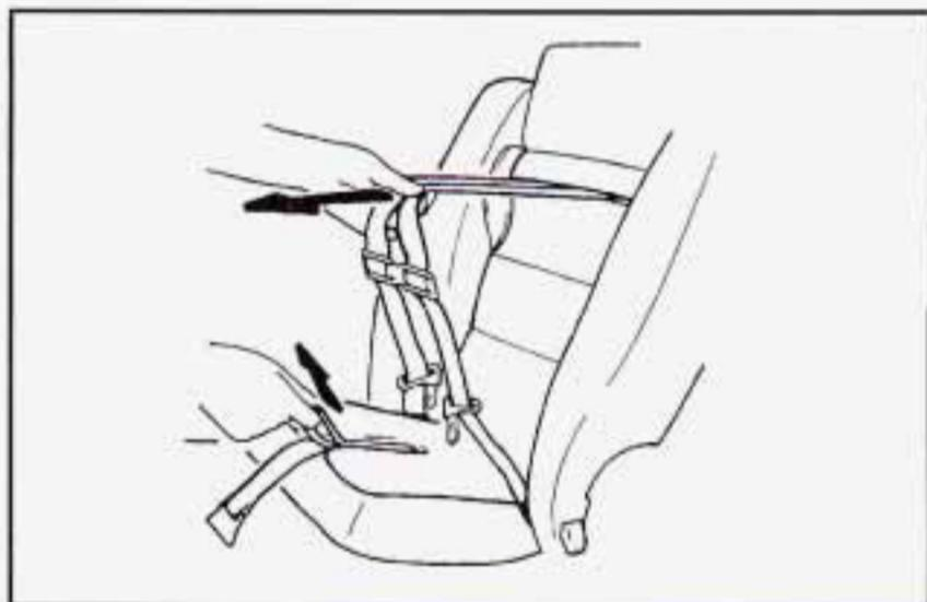
3. Before placing the child in the child restraint, add slack to the shoulder harness. Pull the black shoulder harness release strap firmly. At the same time pull both shoulder harness straps through the slots in the seatback as shown.
