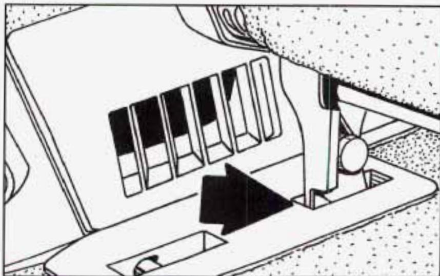
**Rear Air Vents:** To maximize airflow through the rear heater outlet, place the left bucket seat in the second row in the forward position (see “Adjusting Rear Seats” in the Index).
