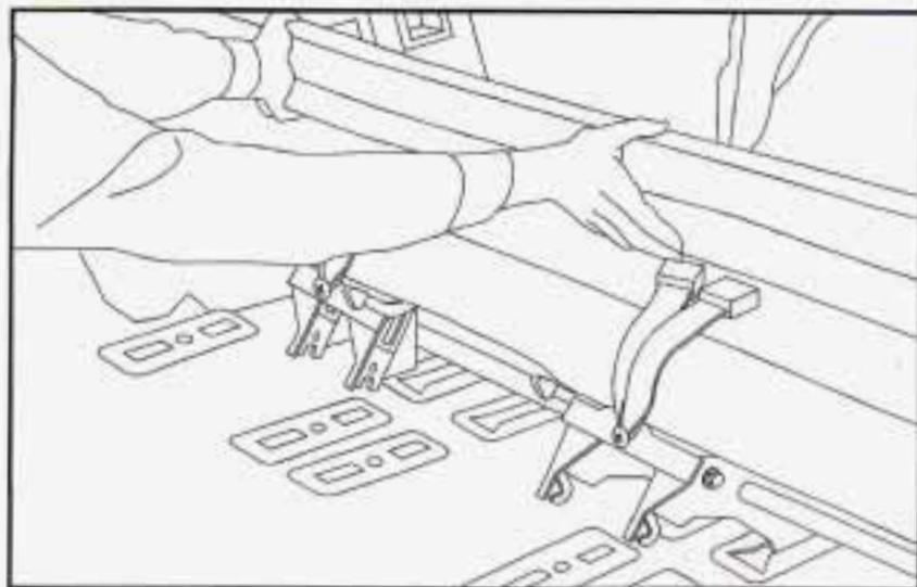
Don't put the bench seat in so it faces backward, because it won't latch that way. If you want more storage room behind the seat, use the floor pins closer to the front of the vehicle. See "Adjusting Rear Seats" later in this section.
