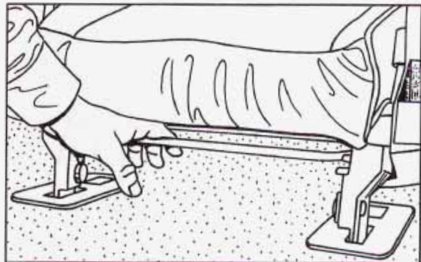
To get out of the third row seats, push down on the rear release bar under the seat ahead of you to tilt the entire seat forward.
