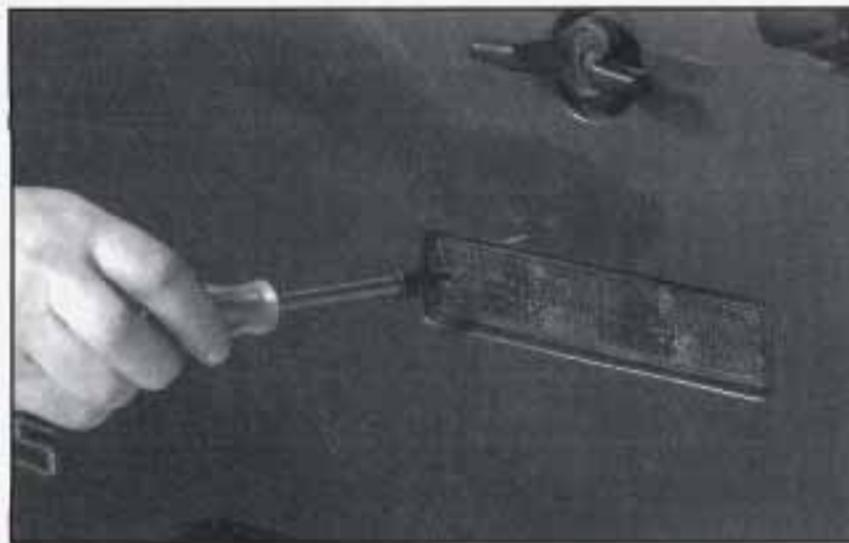
2. Pull the assembly out and away from the liftgate.
