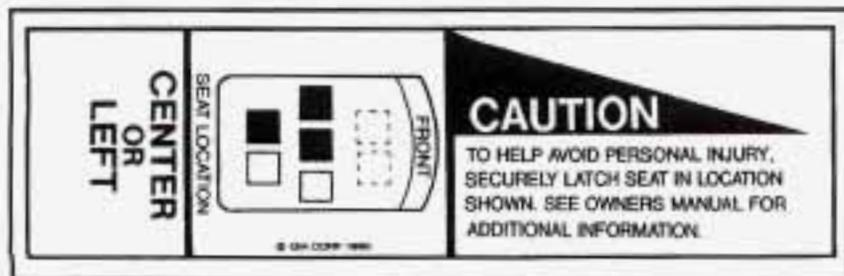
The center position bucket seat is a CENTER OR LEFT type seat. Because it is the only bucket seat with a lap belt, and has a buckle on only one side, there are certain places a CENTER OR LEFT type bucket seat should, and should not, be used. See "Seats" in the Index. If the CENTER OR LEFT bucket seat is used on the left side of the vehicle, the person sitting there should use the lap-shoulder belt. It works the same way as the driver's safety belt. See "Driver Position" in the Index.
