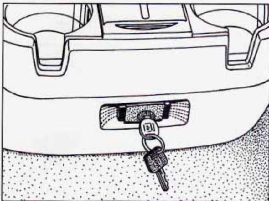
At the base of the center instrument panel console is a storage bin. Use the door key to lock and unlock it. To open the bin, pinch the latch release. Inside the bin, you will find a coinholder.
