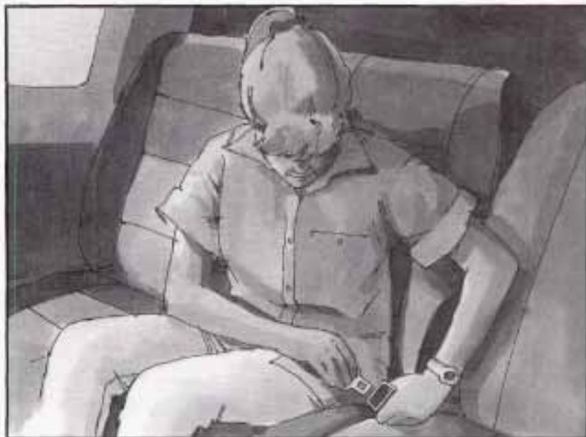
When you sit in the center position bucket seat, you have a lap safety belt which has a retractor.
