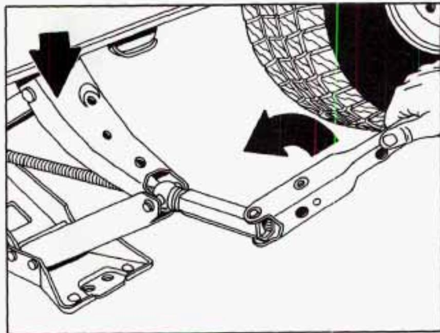
9. Lower the vehicle by attaching the folding wheel wrench to the jack and rotating the wrench counterclockwise. Lower the jack completely.
