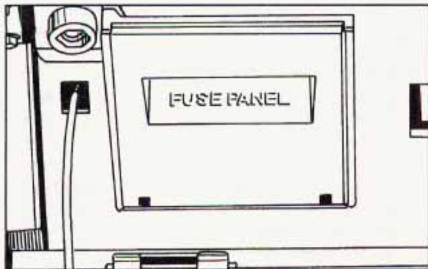
The instrument panel fuse block is in the glovebox. Pull the door open to gain access to the instrument panel fuse block.
