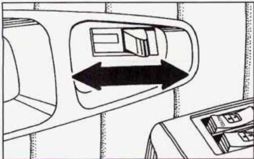
To lock the door from the inside, slide the locking lever rearward.
