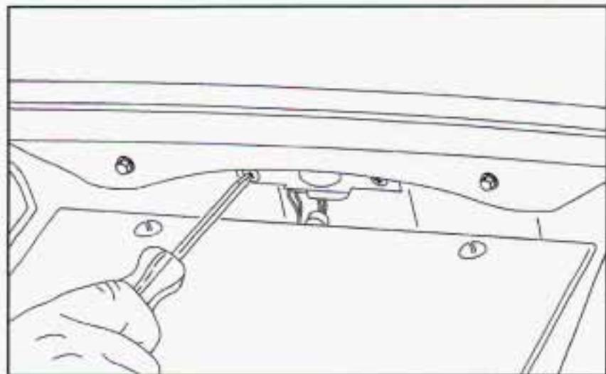
2. Remove the lamp lens from the liftgate.
