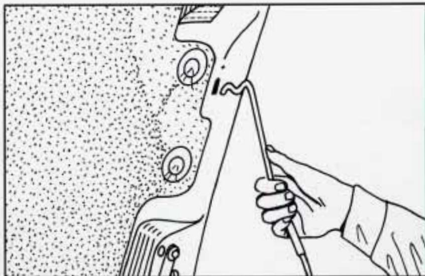
The hood prop may be hot due to increased engine temperatures under the hood, so be careful when handling it. Use your hood prop sleeve when handling the hood prop.
