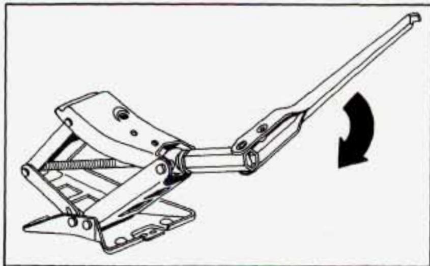
4. Attach the folding wrench to the jack, and rotate the wrench clockwise to raise the jack head a few inches.
