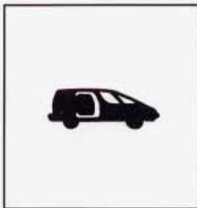
With the optional power sliding door, the sliding door ajar light will come on if your sliding door is not completely closed.
