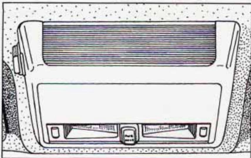
The front overhead console includes two reading lamps and a storage compartment.
