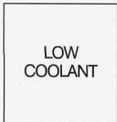
If this light comes on, your system is low on coolant and the engine may overheat.
