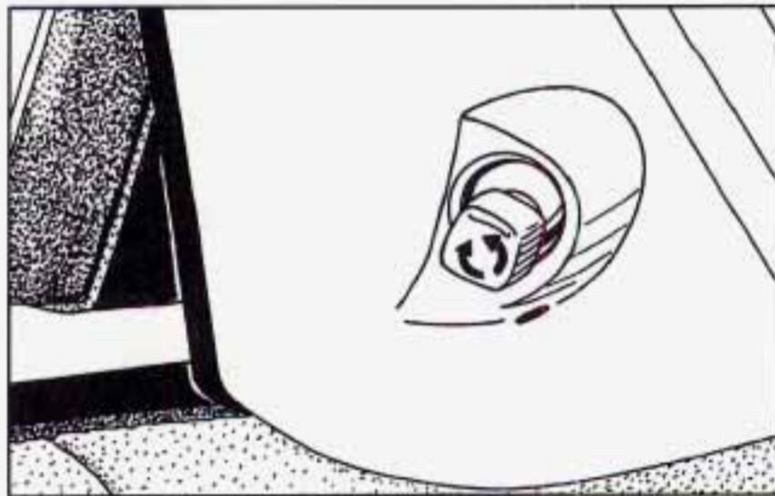
The control on the driver's door controls both outside rearview mirrors. Turn the control to the left to select the driver's side rearview mirror, or to the right to select the passenger's side rearview mirror. Then use the control to adjust each mirror so that you can just see the side of your vehicle when you are sitting in a comfortable driving position.
