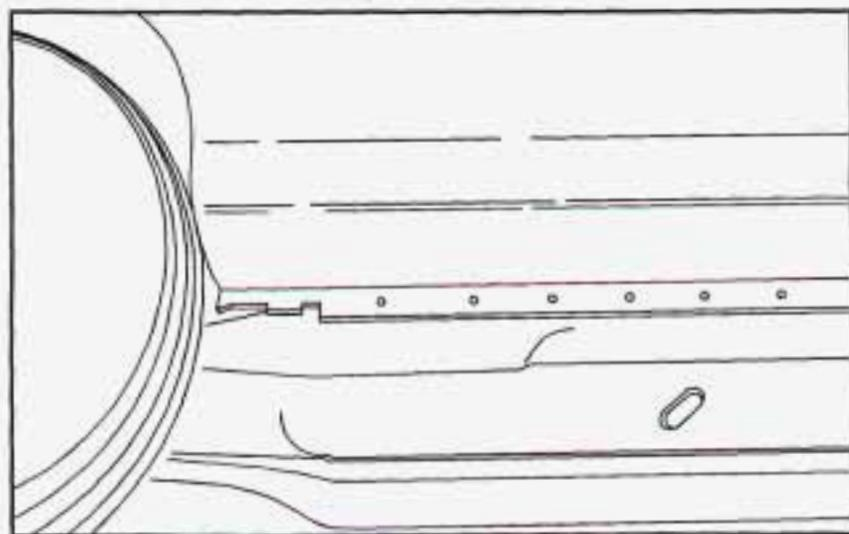
Position the lower sling crossbar directly under the rear bumper.
