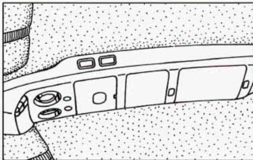
The optional front overhead console has reading lamps, two switches for the optional power sliding door, storage compartments, including one for your garage door opener and one for sunglasses, a compass and an outside temperature display. The features of the optional overhead console are explained on the following pages.
