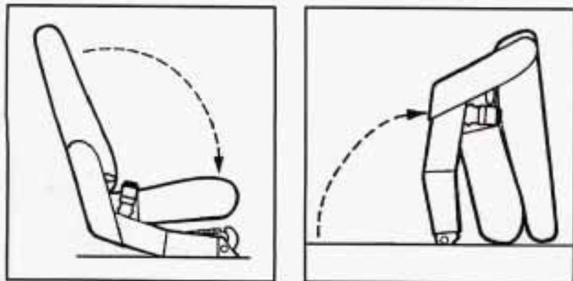
The second and third row bucket seats have been designed to allow them to fold fully upward and forward when the seats are anchored in the rear-most position. This design improves both luggage/cargo capacity and rear seat entry/exit.
