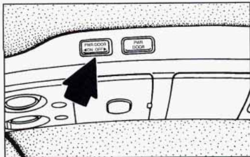
With this option, you can open and close the power sliding door with switches inside your vehicle. If you have the optional Remote Keyless Entry system, you can also operate the power sliding door with your remote transmitter. See “Keyless Entry” in the Index.
