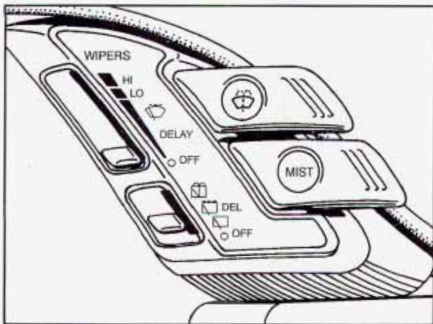
The windshield wiper and washer controls are located to the right of the instrument cluster.
