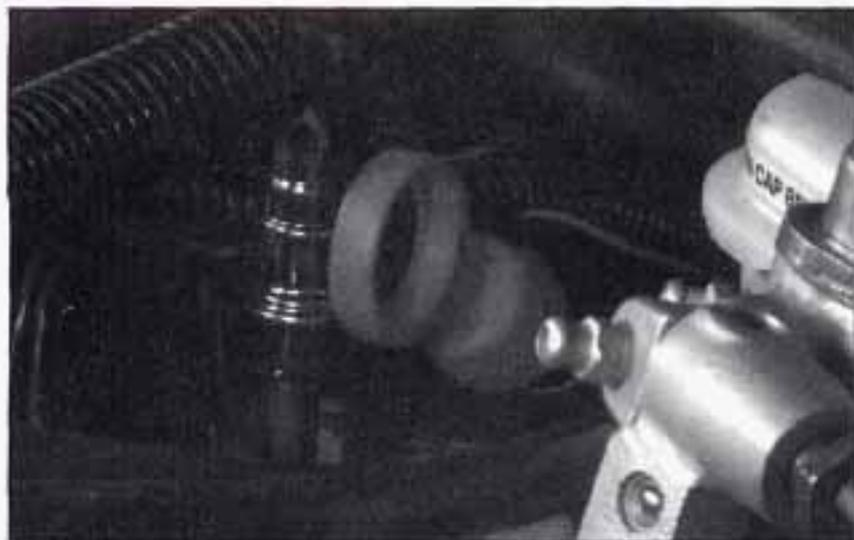
1. The dipstick is located toward the back of the engine compartment, near the center. The dipstick has a bright red loop design for easier identification. Pull out the dipstick and wipe it with a clean rag or paper towel.
