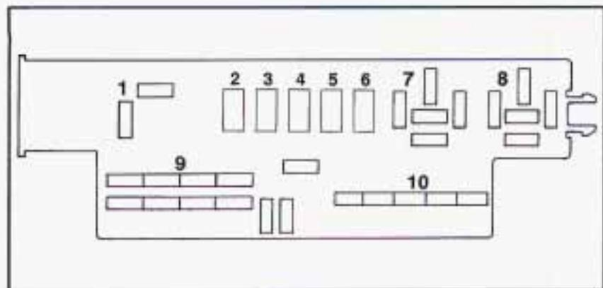
Circuit breakers and relays are located in the circuit breaker/relay panel. This is located behind the panel under the glove box, near the passenger's door.
