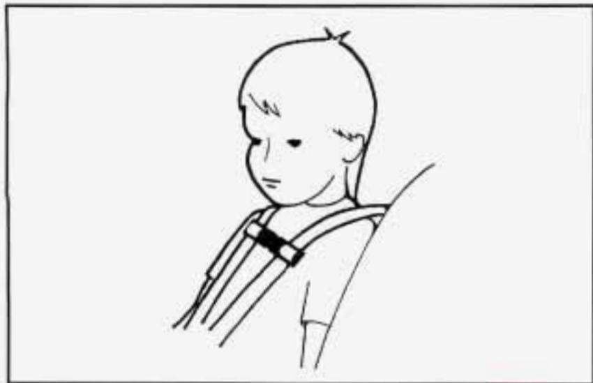
6. Fasten the two halves of the shoulder harness clip together and put it 2 to 3 inches (5 to 8 cm) below the child's chin. The purpose of the clip is to keep the shoulder harness straps positioned correctly on the shoulders.
