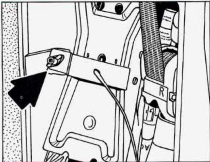
Remove the jack and jacking tools by loosening the wing nut and retainer bar.
