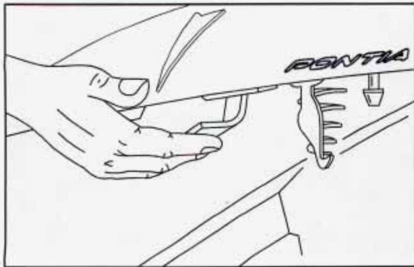
Next, go to the front of the vehicle and pull up on the underhood release.
