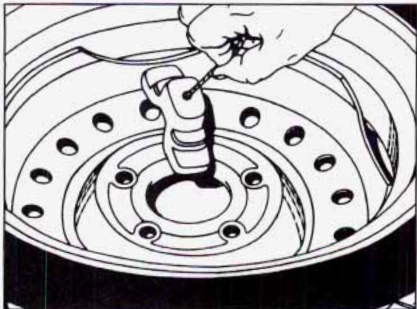
Slide the cable retainer through the center of the spare, then place the compact spare tire near the flat tire.
