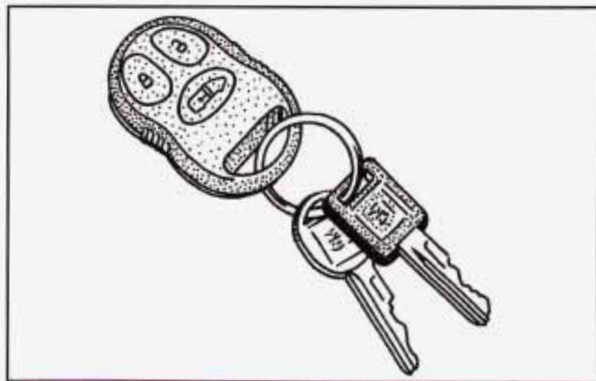
If you have the optional power sliding door (see “Power Sliding Door” later in this section), your remote transmitter will have a third button that has a van symbol on it. Press it to open or close the sliding door.
