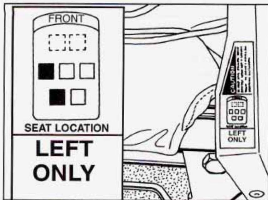
The rear bucket seats can be removed to provide extra storage. Each seat that has the built-in child restraint option fits in only one location in your vehicle, but seats that don't have the built-in child restraint can be moved to different floor locations. The back of each seat has a diagram (similar to the one pictured) that shows where the seat must be located in your vehicle.
