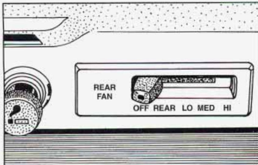
**Rear Fan -- Master Control:** The master control for the rear fan is located below the audio system.
