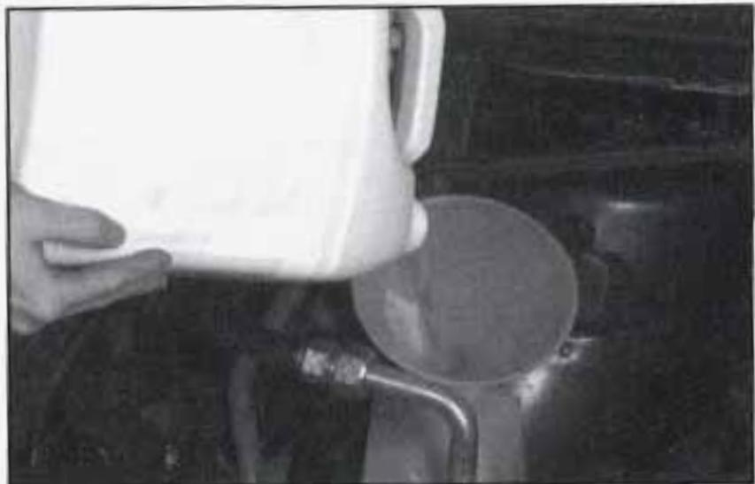
4. Then fill the coolant recovery tank to the FULL HOT mark.
