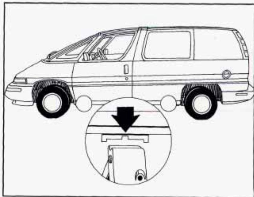
3. Near each wheel, there is a notch in the vehicle's frame. Position the jack and raise the jack head until it fits firmly into the notch in the vehicle's frame nearest the flat tire. Do not raise the vehicle yet. Put the compact spare tire near you.
