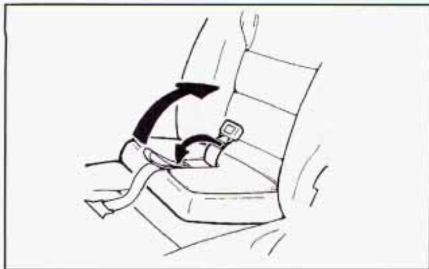
1. Make sure that the crotch strap is held flush to the child restraint cushion with the fastener strip. Also be sure the shoulder harness adjustment strap (grey) is folded up in the seat. This will allow the cushion to fold completely into the seatback. Raise the cushion.
