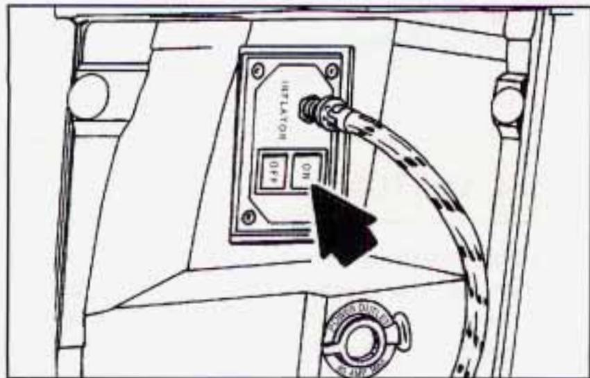
To use your air inflator system, attach the appropriate nozzle adapter, if required, to the end of the hose that has the pressure gage. Then attach that end of the hose to the object you wish to inflate. Remove the protective cap covering the outlet. Attach the other end of the hose to the outlet. Press the ON switch. The ON switch will work even with the ignition off.
