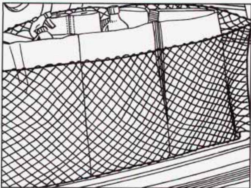
The optional convenience net is designed to help keep small loads, like grocery bags, from falling over during sharp turns or quick stops and starts.
