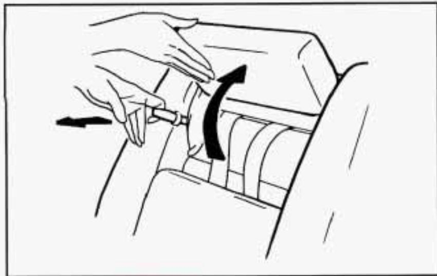
1. Pull the head restraint release strap and raise the head restraint until you hear the latch click.
