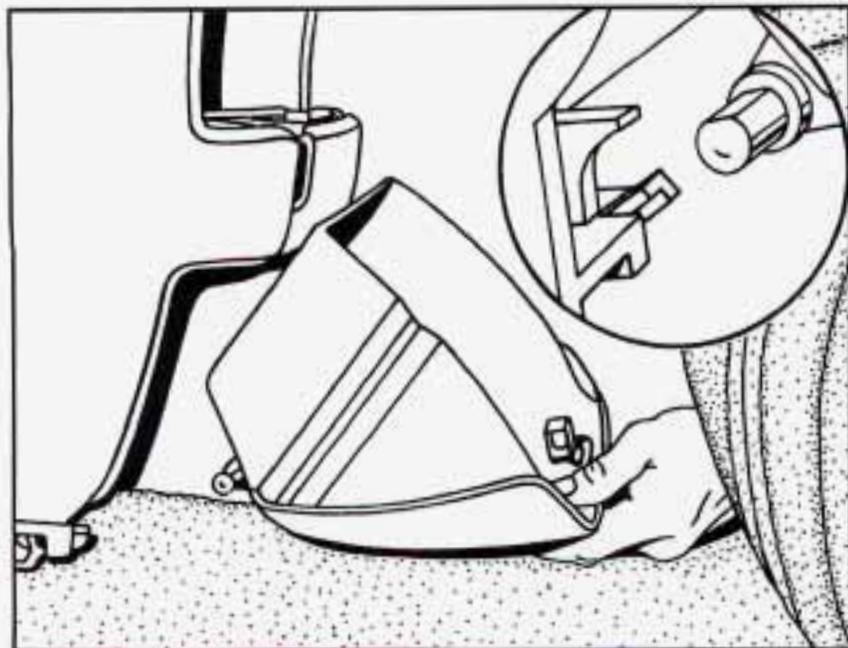
To replace the bin, set the hinge pins (one on each side of the bin, at the bottom) into the hinge guides (one at each side of the console opening, at the base), then close the bin. If the hinge pins are placed properly in the guides, the bin will close easily.
