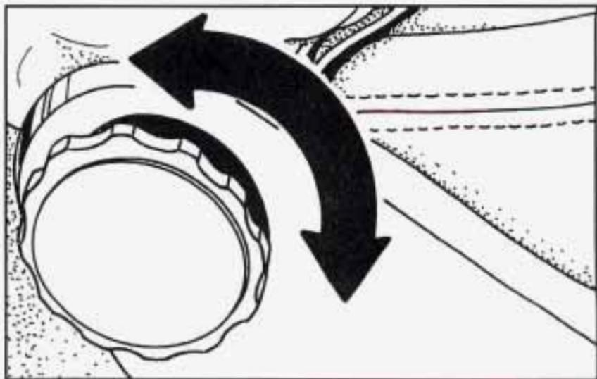
To adjust the seatback, rotate the knob. It is easier to recline the seat if you lean forward, taking your weight off of the seatback.
