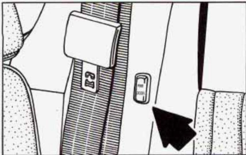
To open or close the sliding door, press and release one of two PWR DOOR switches. One is mounted on the wall, just in front of the sliding door. The other switch is located between the reading lamps on the compact overhead console. If you have the optional overhead console, the other switch is on the side of the overhead console, in the rear-most position.
