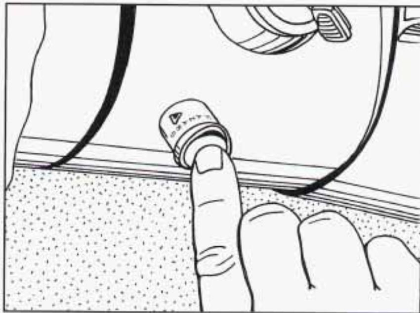
Your hazard warning flashers switch is on the steering column, below the ignition switch. Press the button in to turn your flashers on.
