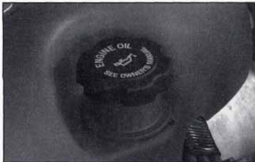
The engine oil fill cap is located just behind the engine oil dipstick.
