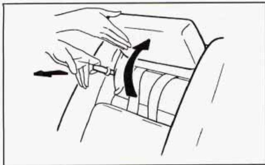
1. Pull the child head restraint release strap and raise the head restraint until you hear the latch click.
