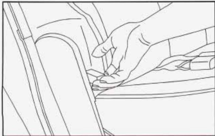
To fold down the seatback, lift the seatback latch release while folding the seatback forward.
