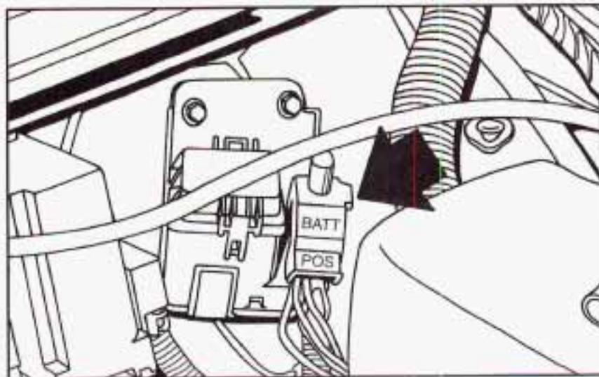
Your Pontiac has a remote positive (+) jump starting terminal. The terminal is in the red box on the same side of the engine compartment as your battery.
