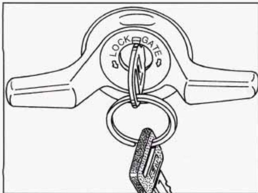
To unlock the liftgate, insert the door key and turn the lock clockwise. The liftgate will automatically lock when you close it.
