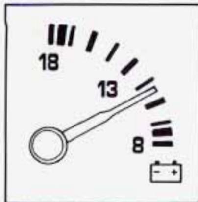
Your charging system gage will show the rate of charge when the engine is running.
