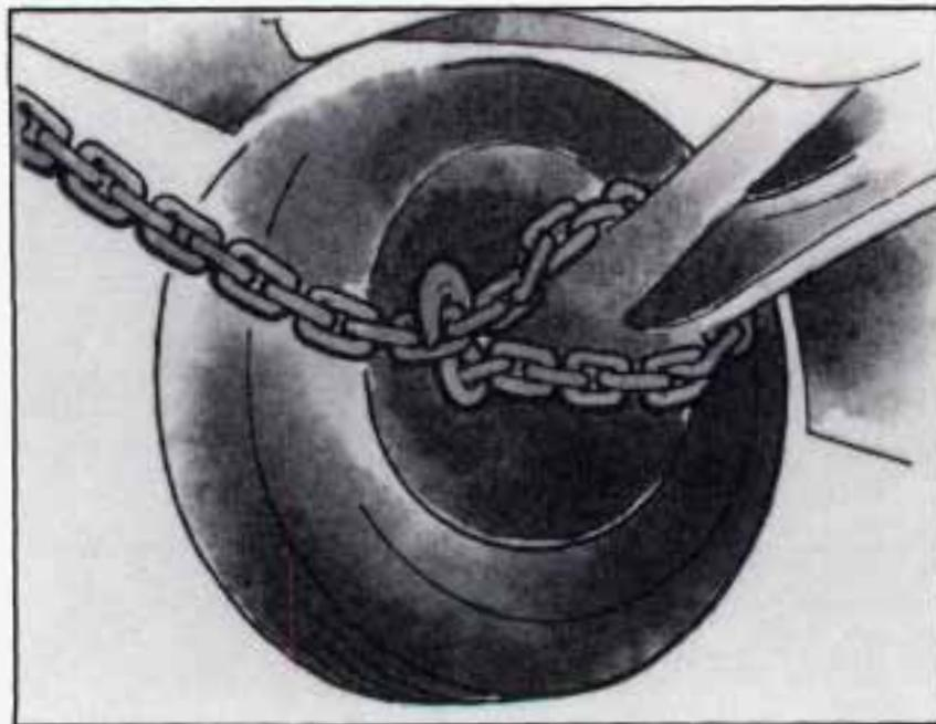
Attach a separate safety chain around the outboard end on each lower control arm.
