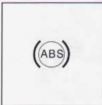
If there's a problem with the anti-lock brake system, this warning light will stay on or flash. See "Anti-Lock Brake System Warning Light" in the Index.
