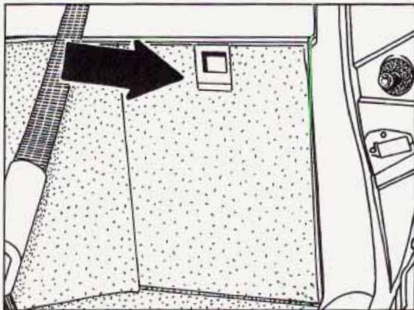
Open the jack storage compartment by sliding the latch down and removing the compartment cover.
