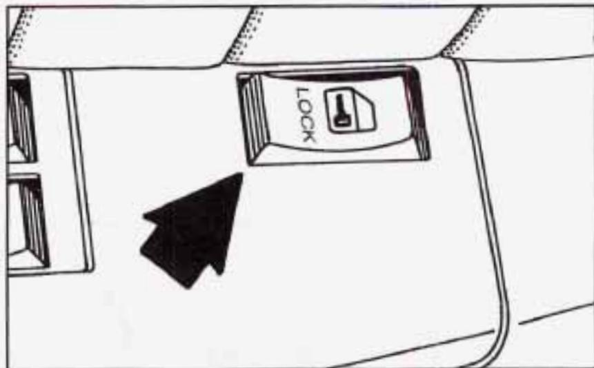
From the inside, press the front of the power door lock switch (on either front door) to unlock all doors and the liftgate.
