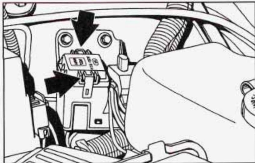
You'll find this fuse under the hood in the ABS junction block, located next to the remote positive jump starting terminal.
