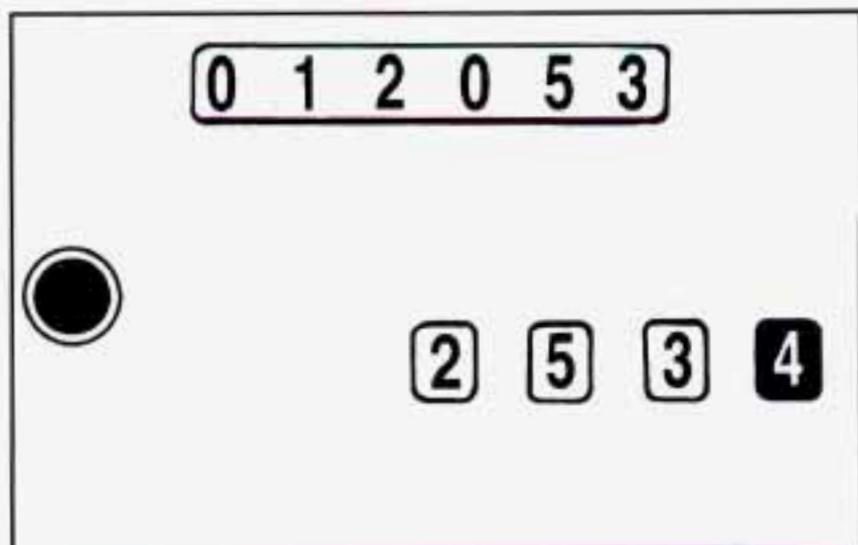
The trip odometer can tell you how far your vehicle has been driven since you last set it to zero. To set it to zero, push the reset button, located above the fuel gage, a little to the right.
