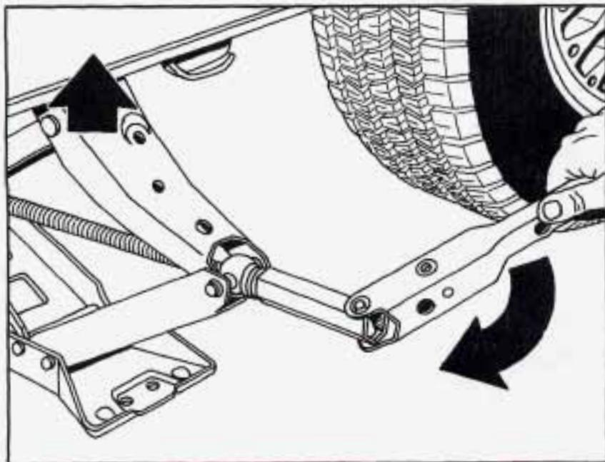
5. Raise the vehicle by rotating the folding wrench clockwise in the jack. Raise the vehicle far enough off the ground so there is enough room for the spare tire to fit.
