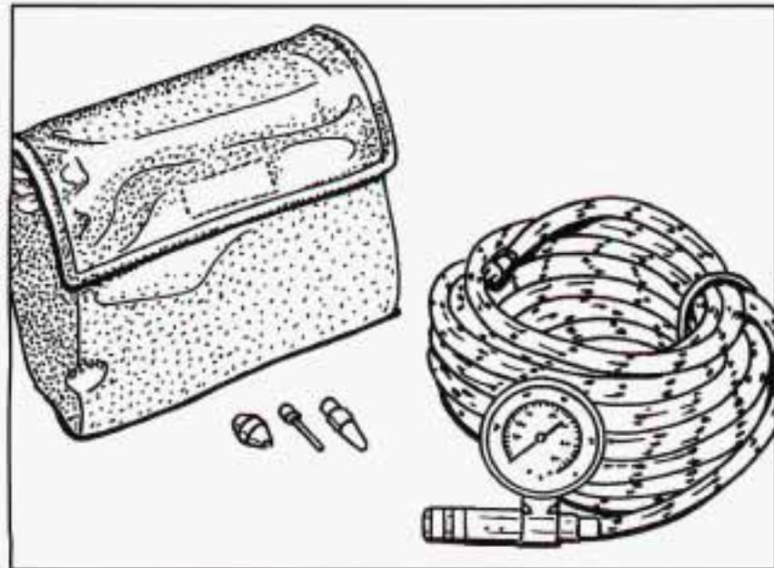
The air inflator kit is stored in a pouch in the glove box or in the rear saddlebag if you have this option. It includes a 20-foot (6 m) hose with an air pressure gage and nozzle adapters.
