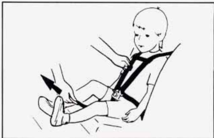
7. Pull the shoulder harness adjustment strap (grey) firmly until the shoulder harness straps are snug against the child's shoulders.
