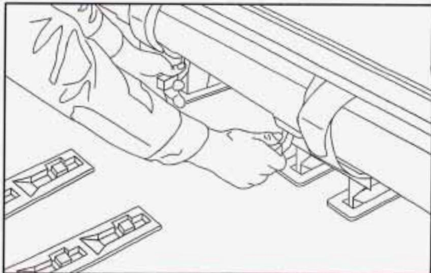
2. Push the rear hooks into the rear floor pins, then push down on the two levers to lock the rear of the bench in place.
