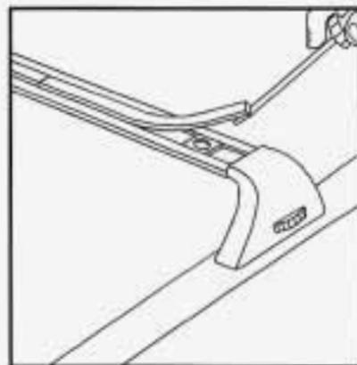
If you wish to attach the luggage tiedowns or other equipment, you will need to remove the outboard bumper strips to access the tapped plates on the crossbar. After the tiedowns or other equipment is removed, be sure to reinstall the bumper strips.
