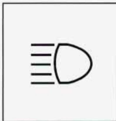
To change the headlamps from high to low beam, or low to high, simply pull the turn signal lever *all the way* toward you. Then release it.
