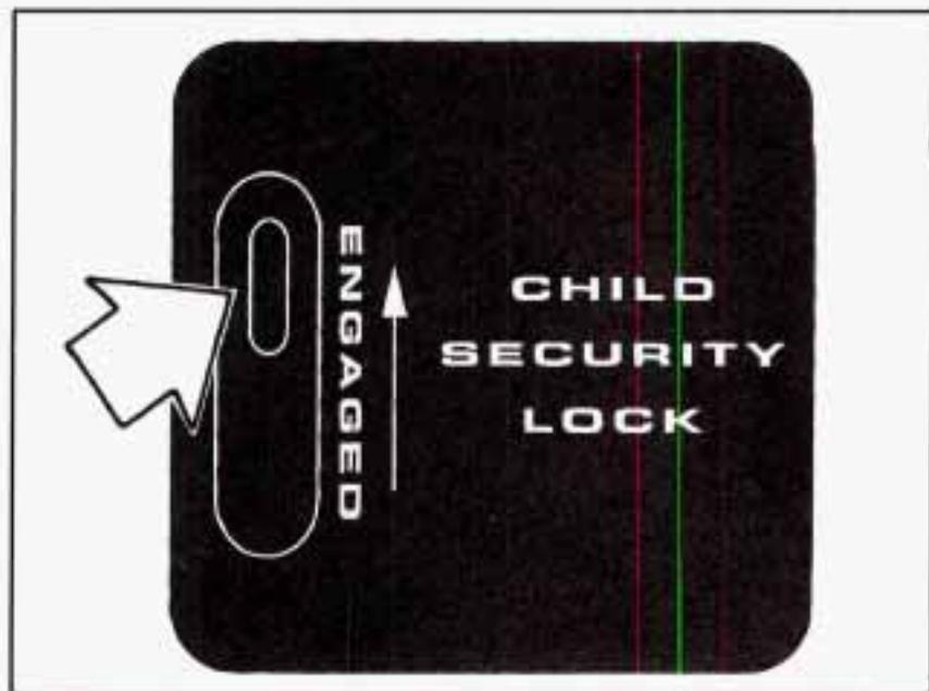
To use the security lock, move the security lock lever all the way up and close the door from the outside.
