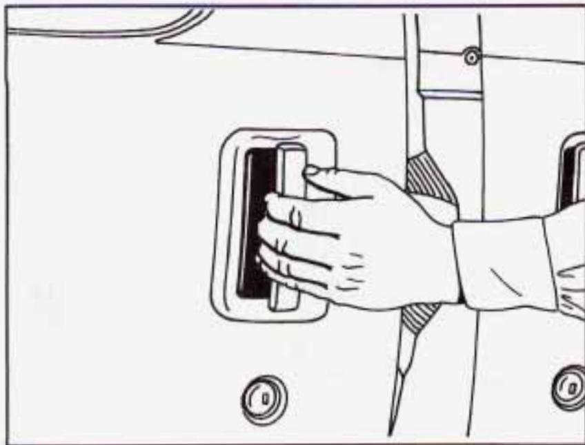
To move the door forward, you must first pull the inside or outside latch release out and then forward or the door will remain latched in the open position.
