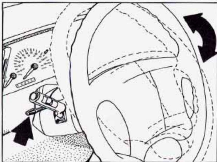
A tilt steering wheel allows you to adjust the steering wheel before you drive. You can also raise it to the highest level to give your legs more room when you exit and enter the vehicle.
