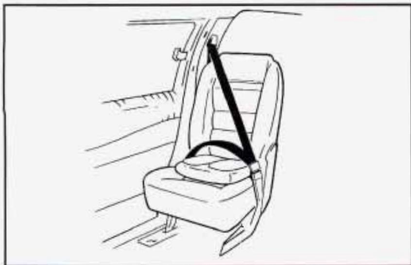
The booster seat can be used by children over 40 lbs. (18 kg) or whose shoulders are above the shoulder belt anchorages of the five-point child restraint harness. The vehicle's lap-shoulder belt is used instead of the
