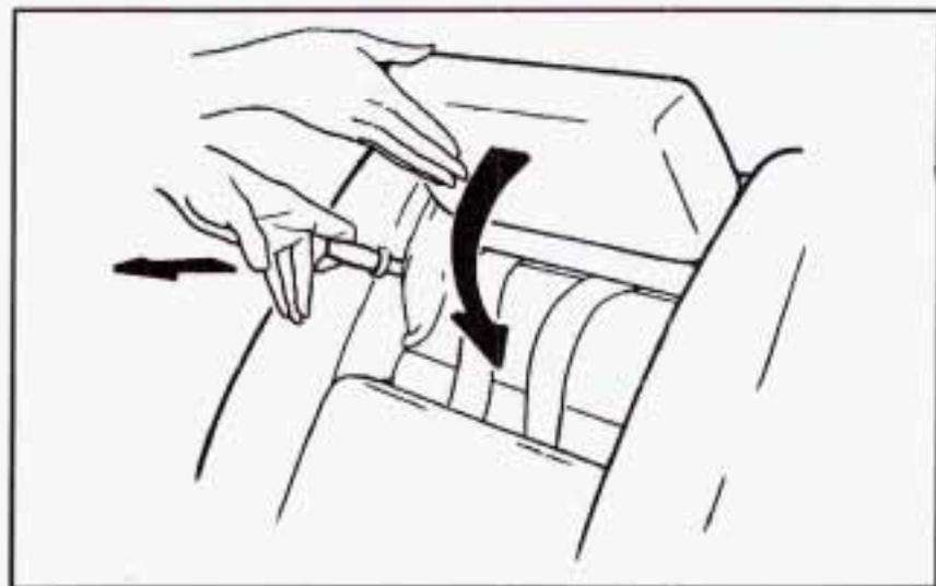
2. Unlatch the child head restraint by pulling the release strap. Lower the head restraint and press it firmly into the seatback until you hear the latch click.
