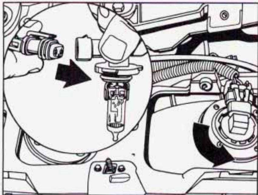
3. Twist the L-shaped bulb assembly counterclockwise one-sixth of a turn until the flanges align with the slots in the retainer ring.
