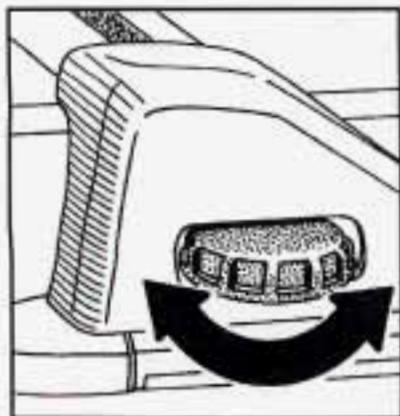
Your luggage carrier has release knobs set in the ends of each crossrail. Turn the release knobs counterclockwise to unlock the crossrails. Slide the crossrails forward or back, as needed, to accommodate loads of varying size.
