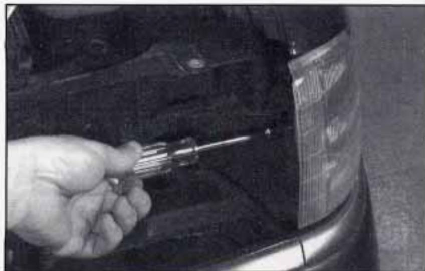
2. Unbolt the retaining nut from the sidemarker lamp assembly bolt.
