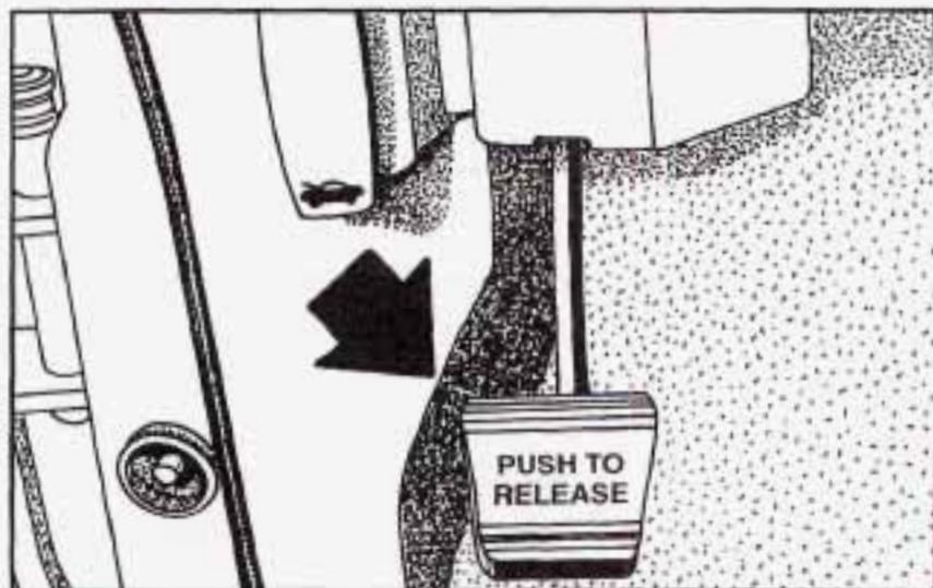
To set the parking brake, hold the regular brake pedal down with your right foot and push down the parking brake pedal with your left foot. If the ignition is on, the brake system warning light will come on. See "Brake System Warning Light" in the Index.
