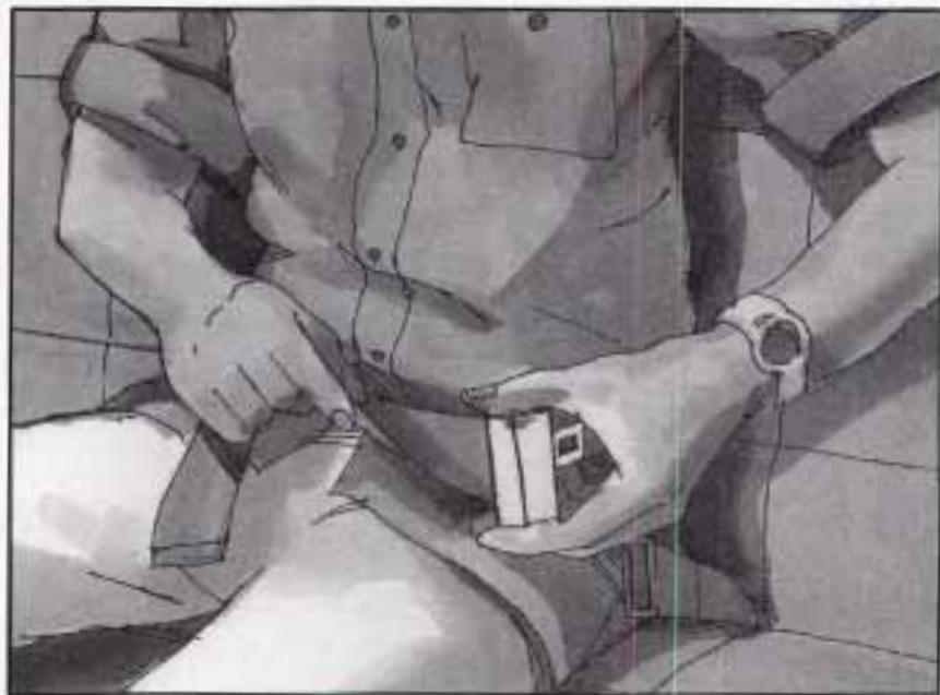
When you sit in the center position of the bench seat, you have a lap safety belt, which has no retractor. To make the belt longer, tilt the latch plate and pull it along the belt.
