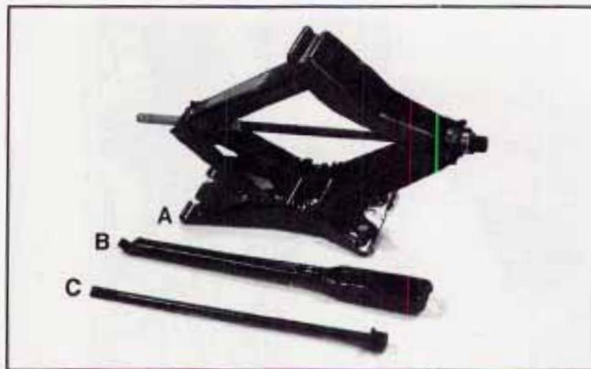
The tools you'll be using include the jack (A), folding wrench (B) and shaft (C).
