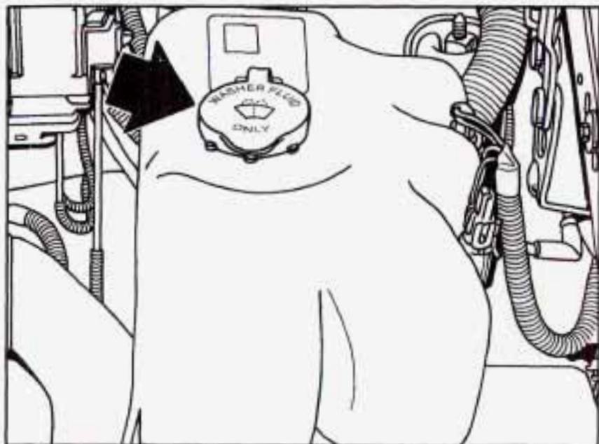
The windshield washer fluid reservoir is located on the driver's side of the vehicle, toward the front of the engine compartment.
