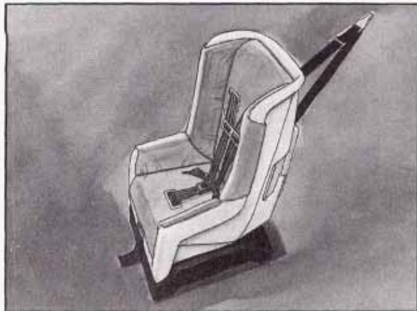
If your child restraint has a top strap, it should be anchored. If your vehicle has third row seats, anchor brackets for the second row outside positions are located just above the place where the third row lap-shoulder belts meet the floor.
