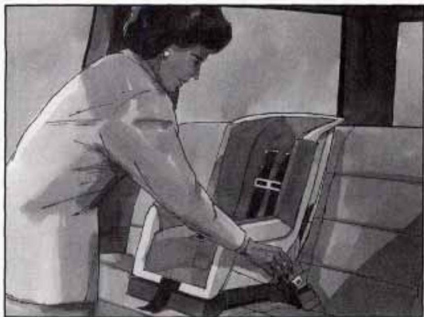
5. Buckle the belt. Make sure the release button is positioned so you would be able to unbuckle the safety belt quickly if you ever had to.
