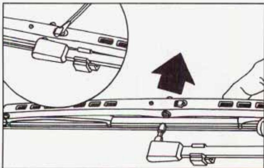
Replacement blades for your vehicle are 24 inches (61 cm) in length. They come in different types and are removed in different ways. Here's how to remove the type with a release clip:
