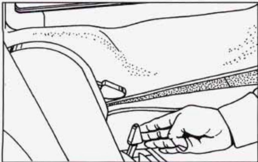
1. Lift the upper lever to fold the seatback forward.
