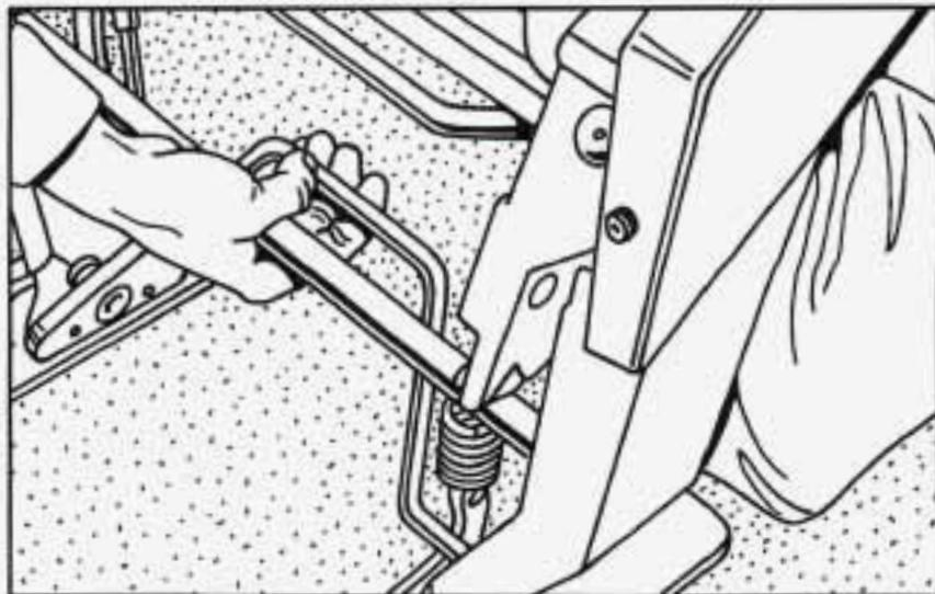
3. From behind the seat, support the top portion of the seat with one hand as you squeeze the front release bar toward the crossbar. The seat will release from the floor pins.
