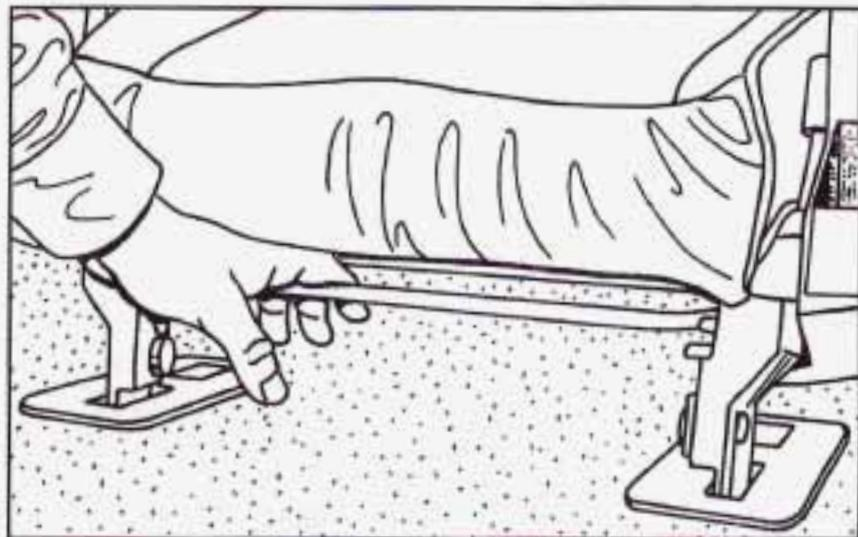
2. Push down on the rear release bar (located behind the seat), and tilt the entire seat forward.
