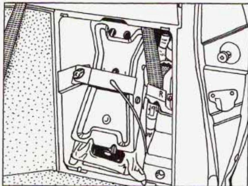
Replace all jacking tools as they were stored in the jack storage compartment and replace the compartment cover.
