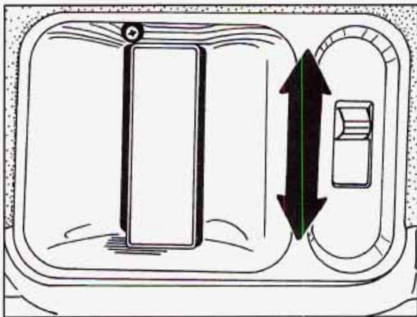
Lock the sliding door from inside the vehicle by moving the manual locking lever down. Unlock it by moving the lever up.
