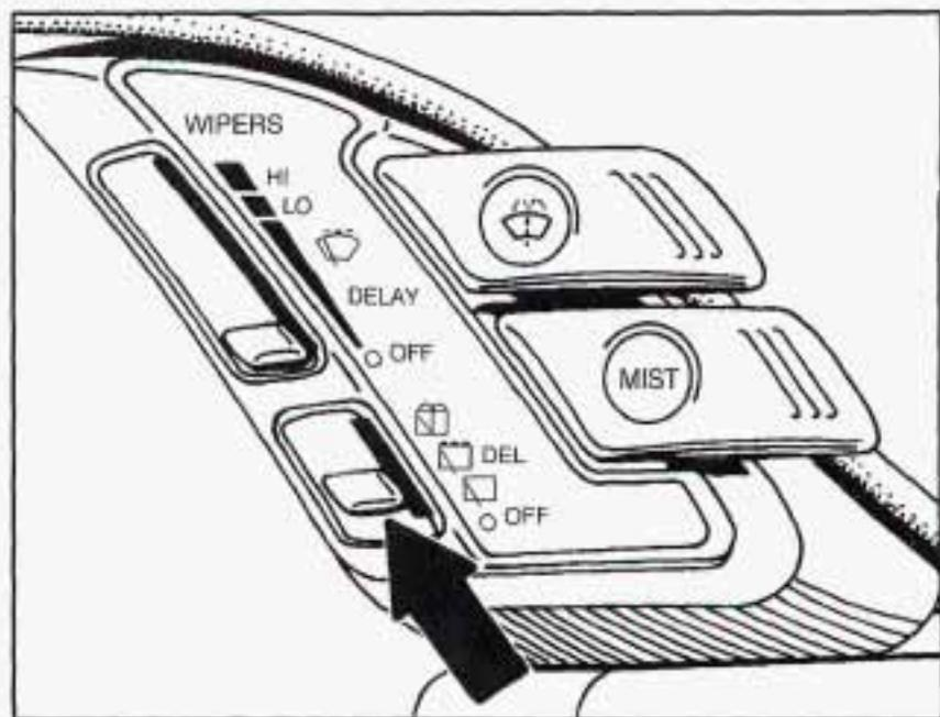
To use your rear wiper, slide the lower control to the rear window wiper symbol.
