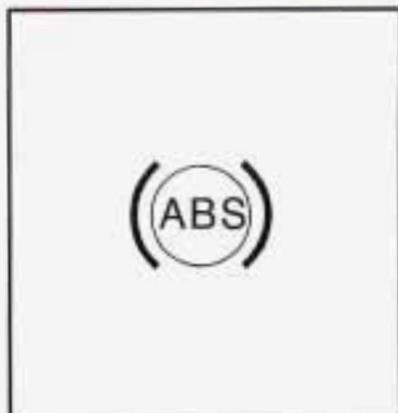
With the anti-lock brake system, this light will come on when you start your engine and it will stay on for three seconds. That's normal.
