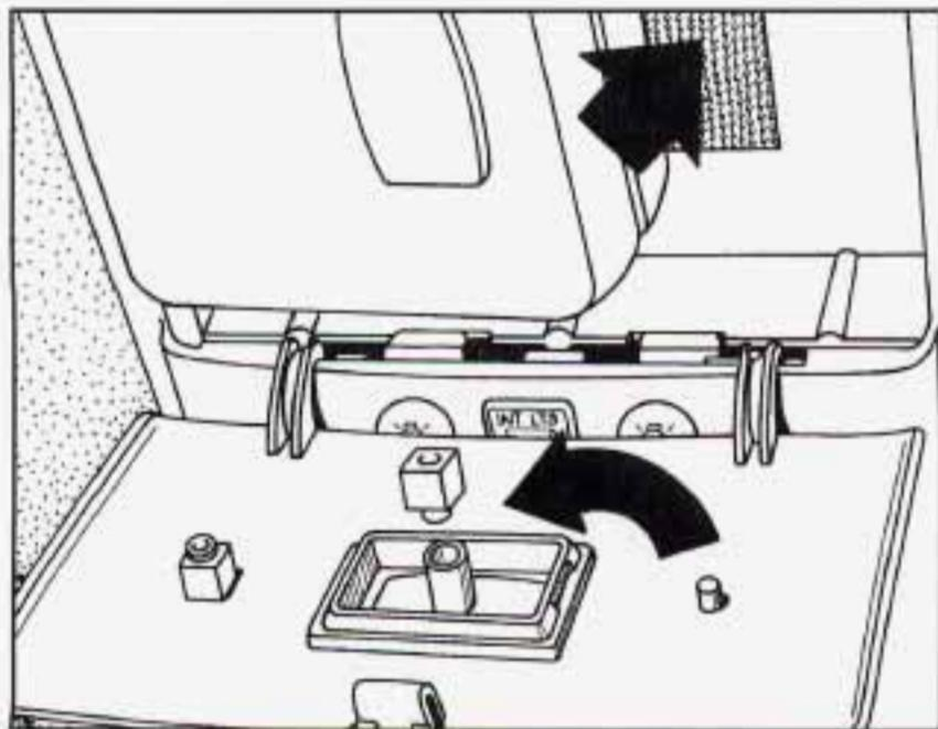
3. To make sure the button on your garage door opener is centered above the button on the compartment door, use the intersecting lines on the Velcro inside the compartment as a guide. Center the control button of your garage door opener over the point where the lines intersect, and press the opener firmly into place. Make sure the button is facing down.
