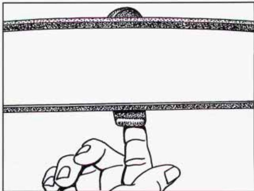
To reduce glare from lights behind you, pull the lever toward you (to the night position). To return the mirror to the day position, push the lever away from you.
