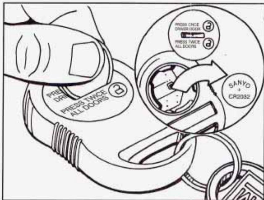
1. Insert a coin into the slot in the back of the transmitter and turn it counterclockwise to open the cover.
