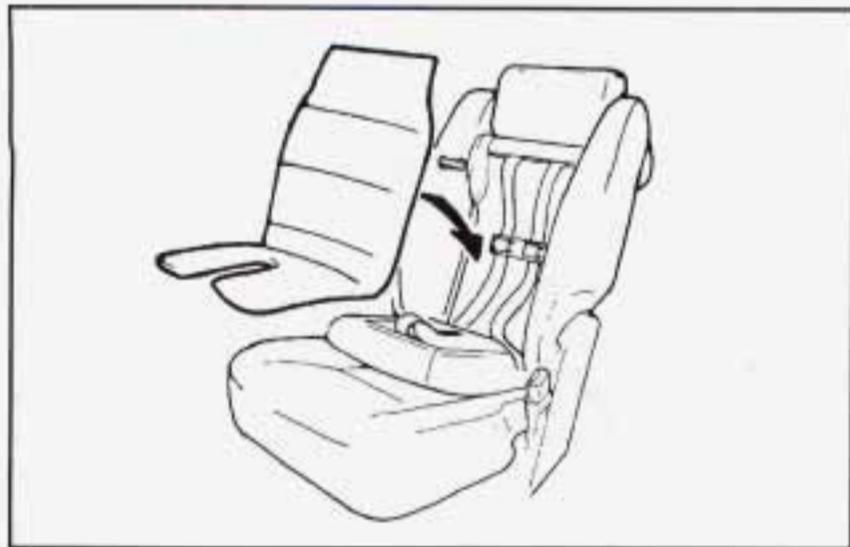
3. Store the five-point child restraint harness behind the removable pad. The pad is held in place by fastener strips.
