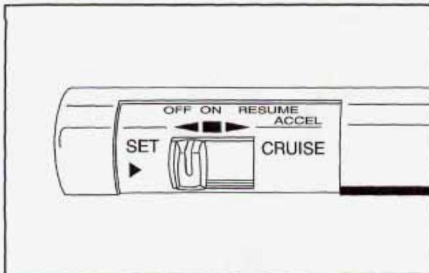
With cruise control, you can maintain a speed of about 25 mph (40 km/h) or more without keeping your foot on the accelerator. This can really help on long trips.
