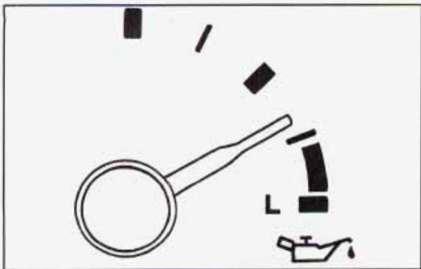
Your vehicle is equipped with an oil pressure indicator. Your oil pressure indicator lets you know when you may have a problem with your engine oil pressure.
