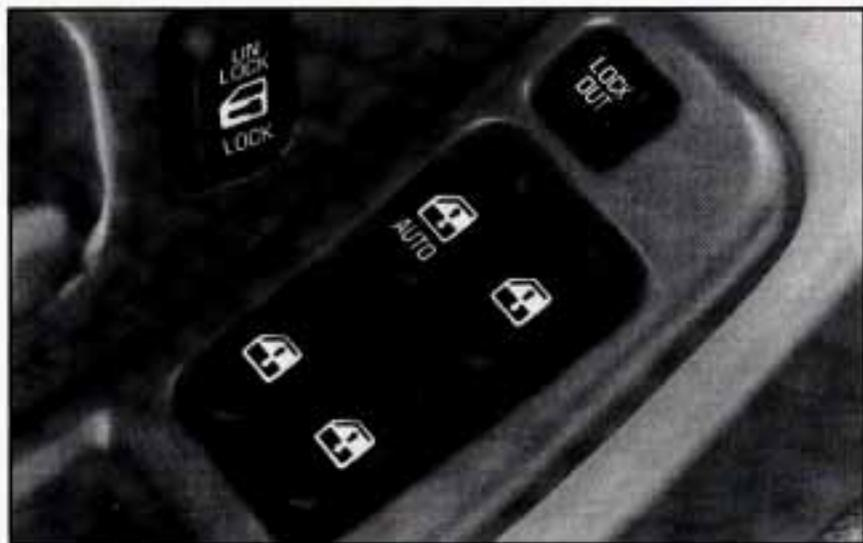
Switches on the driver's door armrest control each of the windows when the ignition is on. In addition, each of the passenger's doors has a switch for its own window.
