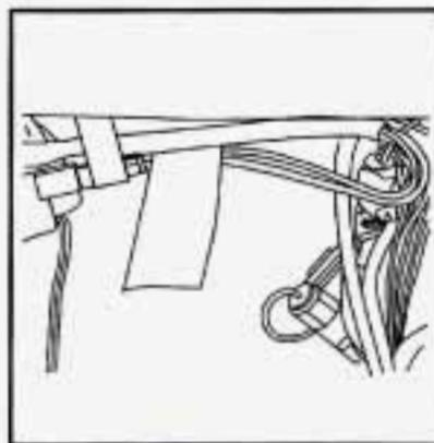
Your vehicle is equipped with auxiliary power leads. These leads can be used to power aftermarket electrical equipment added to your vehicle.
