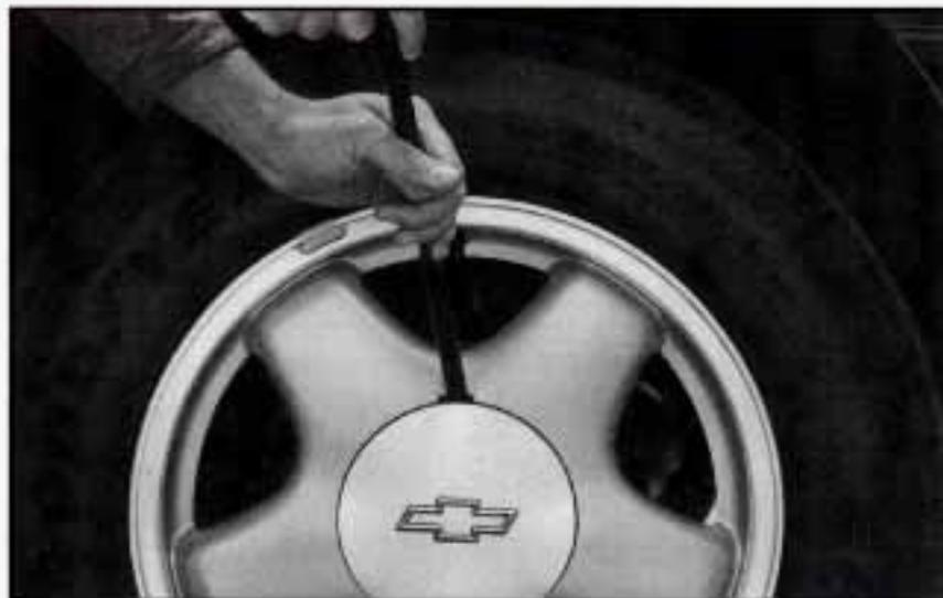
To remove a center cap, use the wrench to pry gently at the notch. Don't use a tool that is narrower than the wrench to pry at this notch.
