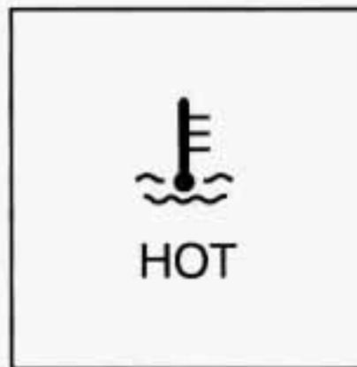
This light tells you that your engine coolant has overheated or your radiator cooling fan(s) are not working.
