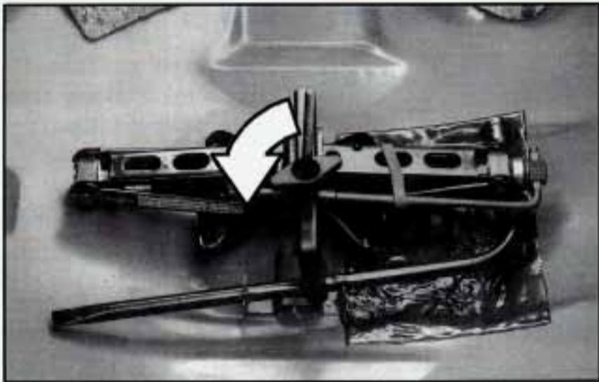
Turn the nut holding the jack and wrench counterclockwise and remove it. Then remove the jack and wrench.
