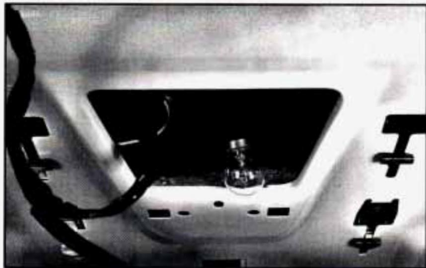
1. Open the trunk lid. Locate the stoplamp behind the rear seats, in front of the trunk hinges.
