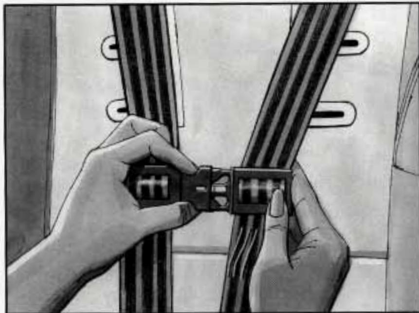
2. If the left and right halves of the shoulder harness clip are fastened together, separate them.
