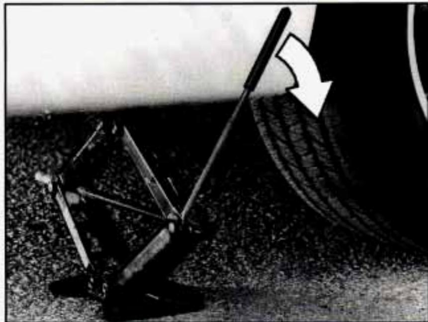
4. Raise the vehicle by turning the jack handle clockwise. Raise the vehicle far enough off the ground for the spare tire to fit under the vehicle.
