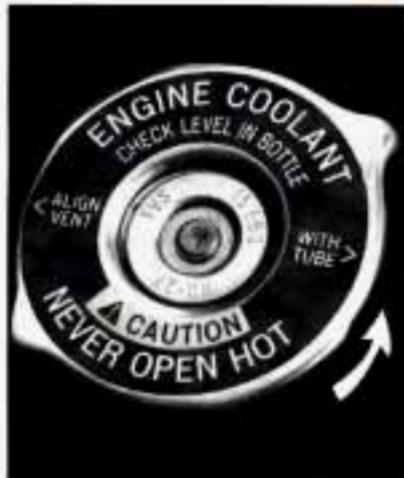
1. You can remove the radiator pressure cap when the cooling system, including the radiator pressure cap and upper radiator hose, is no longer hot. Turn the pressure cap slowly counterclockwise until it first stops. (Don't press down while turning the pressure cap.)
