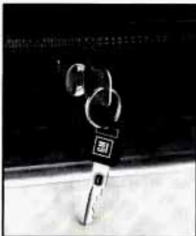
To unlock the trunk from the outside, insert the door key and turn it. You can also use the remote keyless entry function if your vehicle has this option. Just press the trunk symbol on the transmitter, making sure your shift lever is in PARK (P).
