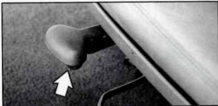
Lift the handle to tilt the seat up or down.
