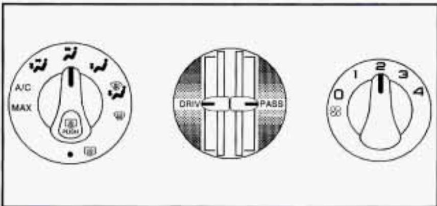
If your system does have the auxiliary temperature control option, the center levers change the temperature of the air coming through the system. The DRIV lever sets the temperature for the driver and rear seat passengers, and the PASS lever sets the temperature for the front seat passenger. For maximum defroster performance, set the DRIV and PASS levers at full warm.
