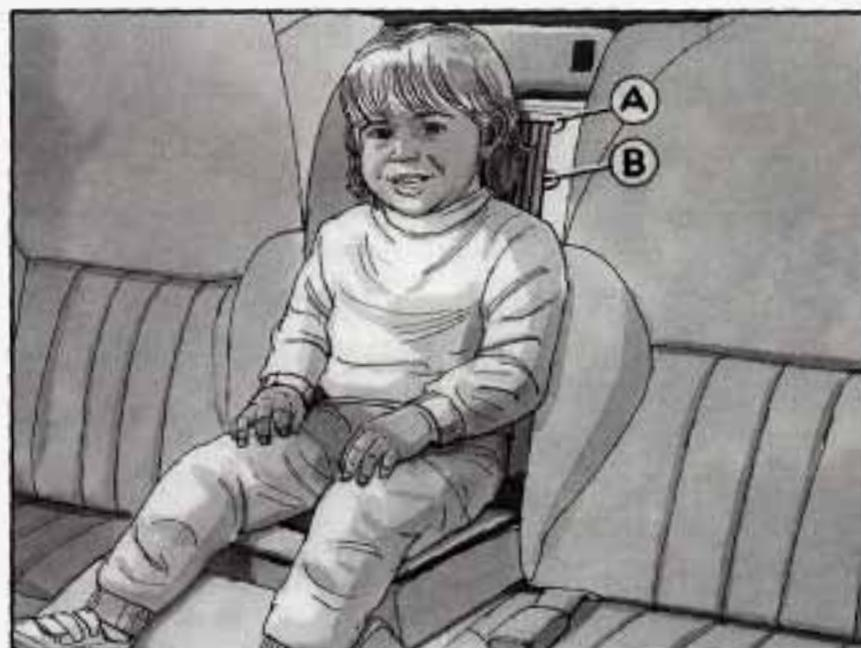
For the child shown here, the harness should go through the middle pair of slots (B).
