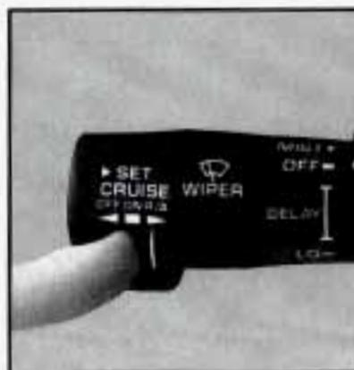
Once you're going about 25 mph (40 km/h) or more, you can move the cruise control switch from ON to R/A (Resume/Accelerate) for about half a second. You'll go right back up to your chosen speed and stay there.
