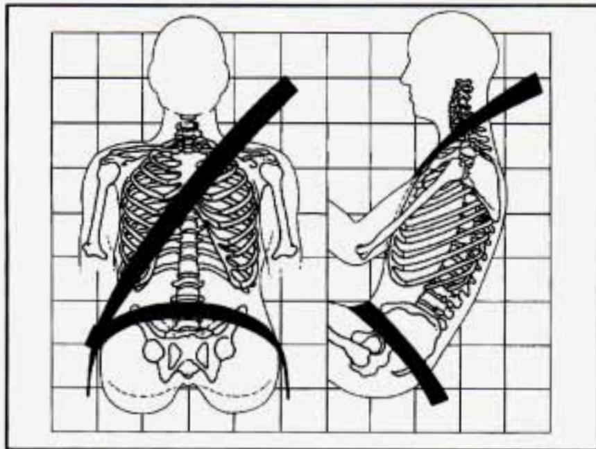
The lap part of the belt should be worn low and snug on the hips, just touching the thighs. In a crash, this applies
