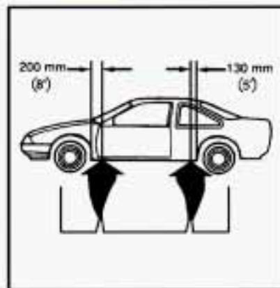
3. Position the jack under the vehicle and raise the jack lift head until it fits firmly into the notch in the vehicles frame nearest the flat tire.
