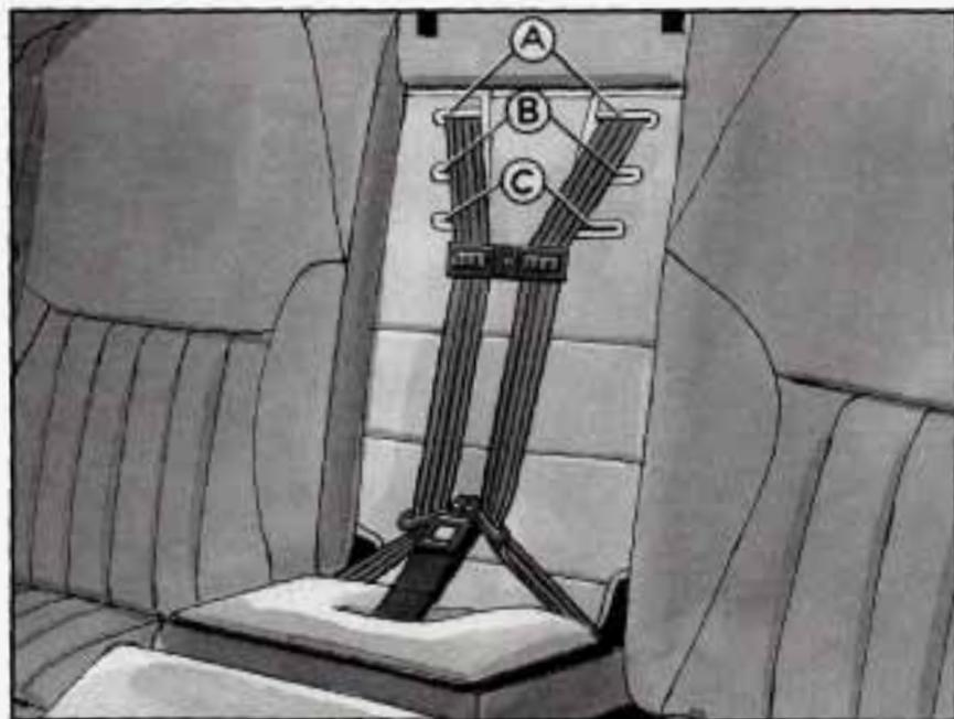
With this built-in child restraint, you can adjust the height of the harness. Depending on the seated height of the child, you can route it through the upper pair of slots (A), the middle pair of slots (B) or the lower pair of slots (C).
