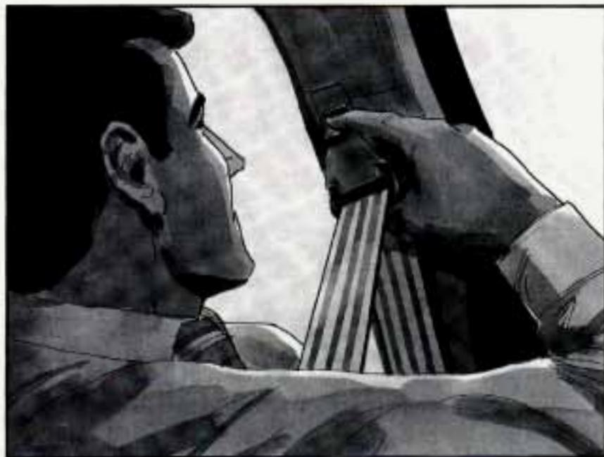
To move it down, squeeze the release lever and move the height adjuster to the desired position. You can move the adjuster up just by pushing up on the shoulder belt guide. After you move the adjuster to where you want it, try to move it down without squeezing the release lever to make sure it has locked into position.
