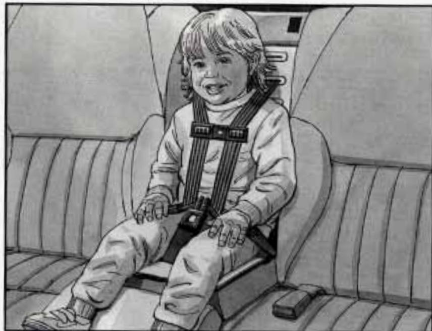
9. On both sides of the harness, pull up on the lap part a little to be sure it's locked.
