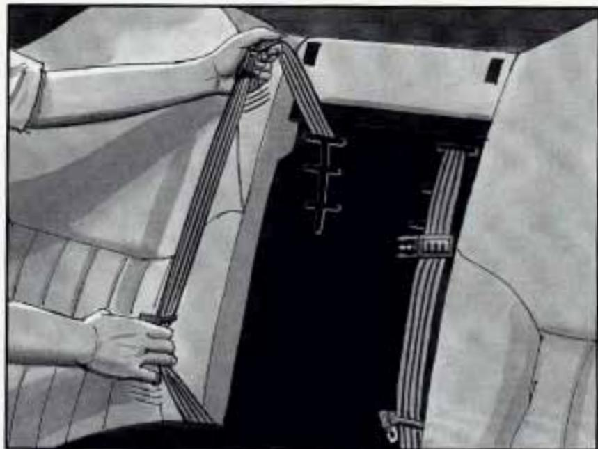
5. Select one side of the harness. Add some slack to the shoulder part by pulling up on the lap part. You'll keep most of this slack until you finish Step 9.
