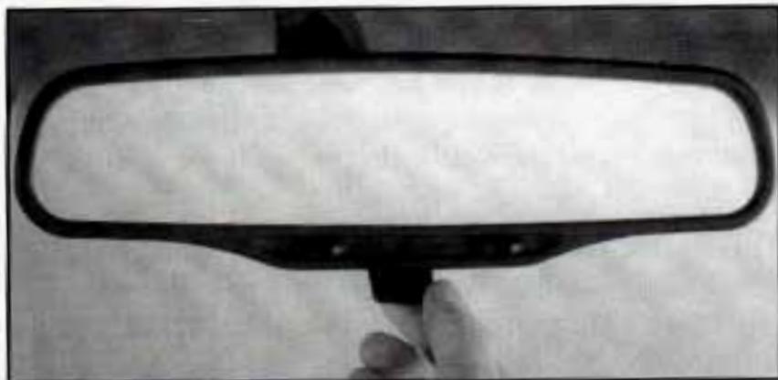
To reduce glare from headlamps behind you, push the lever forward (to the night position). To return the mirror to the day position, pull the lever toward you.
