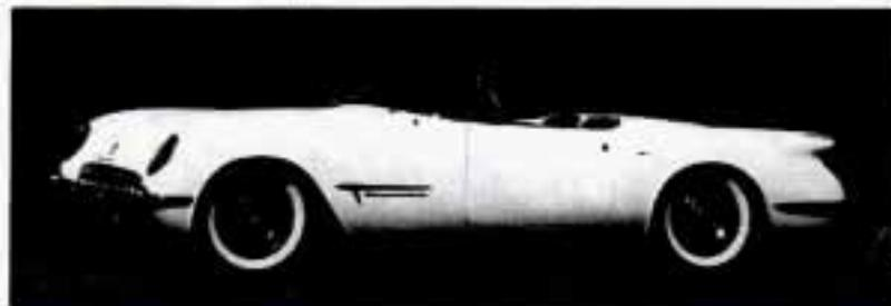
*launched the first use of a fiberglass body in a production car.*
