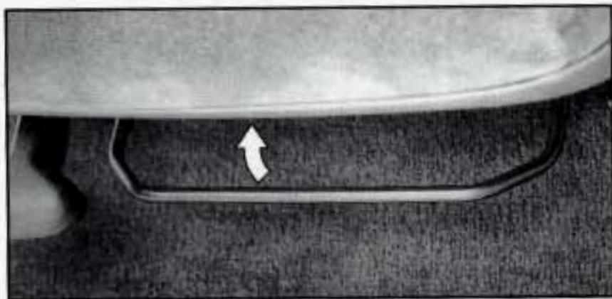
The driver's seat may have a bar and a handle under the front edge of the seat. Lift the bar to unlock the seat and to slide it forward and backward.
