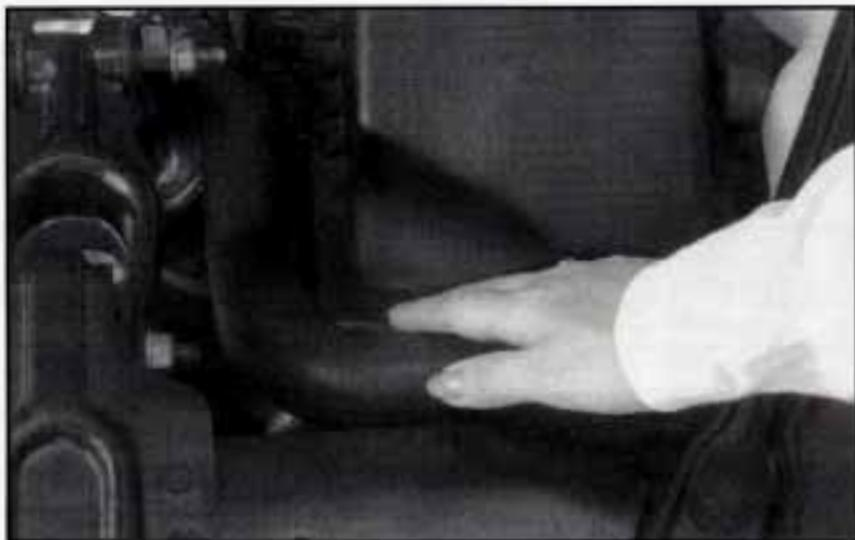
8. Start the engine and let it run until you can feel the upper radiator hose getting hot. Watch out for the engine fans.
