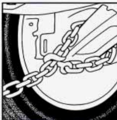
Attach a separate safety chain around the outboard end of each lower control arm.
