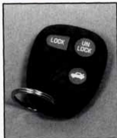
Press UNLOCK once to unlock the driver's door. Press UNLOCK again within five seconds to unlock all remaining doors; pressing UNLOCK will also cause the vehicle's interior lamps to come on for a period of time--(see "Sustained Interior Illumination" in the Index for more details).
