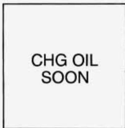
The CHANGE OIL SOON light should come on as a bulb check when you start the engine. If this light stays on for about 20 seconds after you turn on the ignition, have the oil changed.
