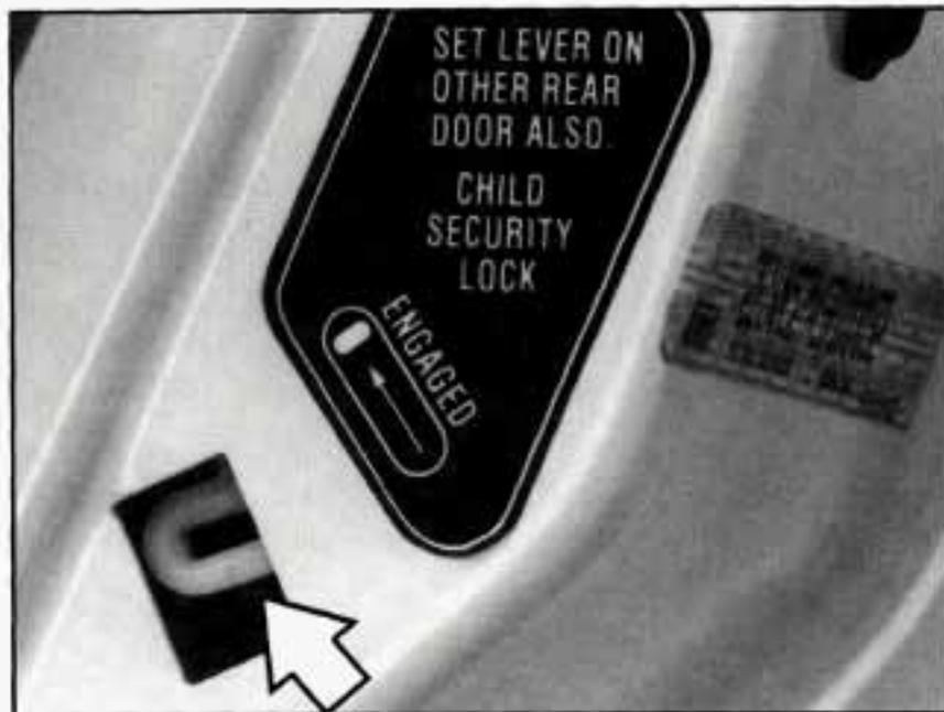
1. Open the rear door. Use a key to move the lever all the way up.
