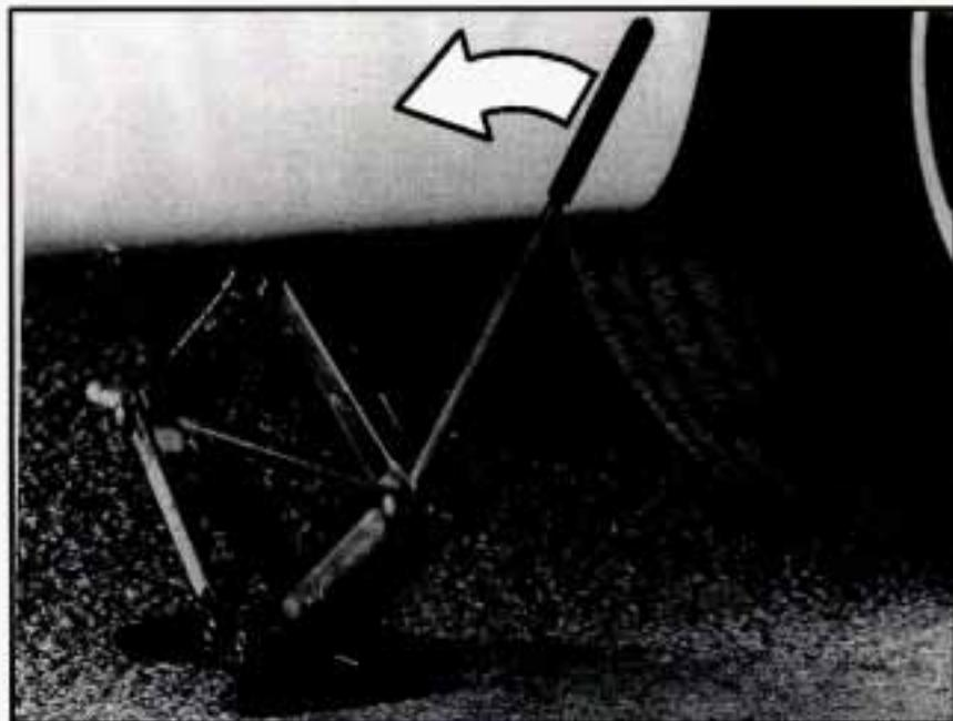
8. Lower the vehicle by turning the jack handle counterclockwise. Lower the jack completely.
