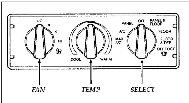
**The controls for the manual heating and air conditioning system**
