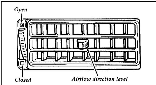
Controlling the airflow from panel registers
