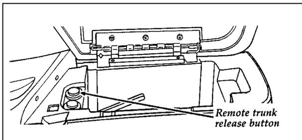
The trunk release button located under the armrest
