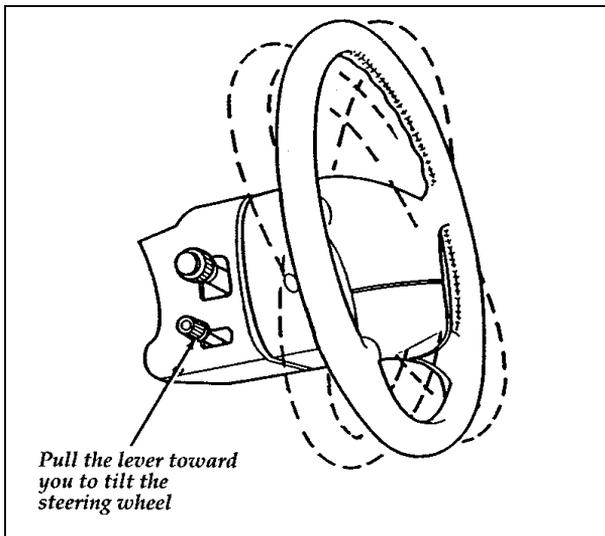
**The lever to tilt the steering wheel**
