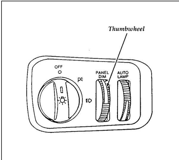
The thumbwheel controls the light on the instrument panel and the interior light
