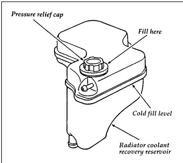
The engine coolant reservoir
