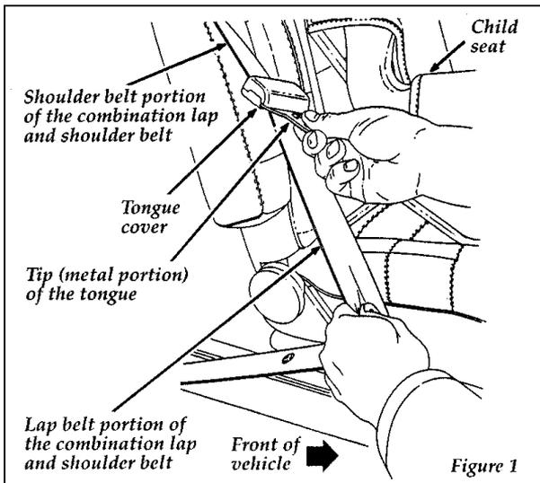
**NOTE:** The belt webbing below the tongue is the lap belt portion of the combination lap/shoulder belt, and the belt webbing above the tongue is the shoulder belt portion of the combination lap/shoulder belt.
