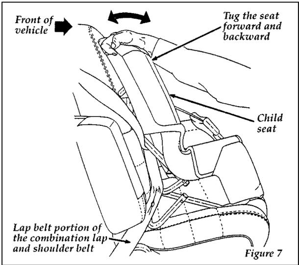
9. Check from time to time to be sure that there is no slack in the lap/shoulder belt. The shoulder belt must be snug to keep the lap belt tight during a collision.
