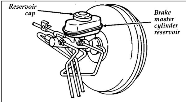
The brake system fluid reservoir
