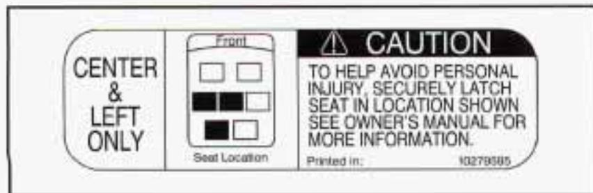
The center position bucket seat is a CENTER OR LEFT type seat. Because it is the only bucket seat with a lap belt, and has a buckle on only one side, there are certain places a CENTER OR LEFT type bucket seat should, and should not, be used. See “Seats” in the Index. If the CENTER OR LEFT bucket seat is used on the left side of the vehicle, the person sitting there should use the lap-shoulder belt. See “Rear Seat Outside Passenger Positions” in the Index.
