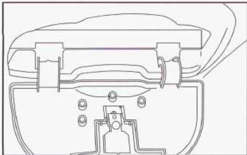
3. Line up the button of the garage door opener with one of the four buttons on the compartment door. Make sure the garage door opener button is facing down and press the opener firmly into place.
