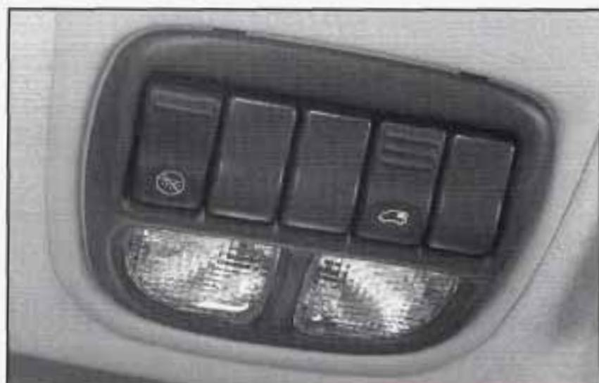
There are two reading lamps in the overhead console. To turn on either reading lamp, press the lens of the lamp. To turn off the lamp, press the lens again.
