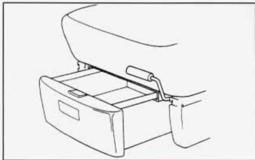
The storage bin is under the manual front passenger's seat. To open the bin, lift the handle and slide the drawer out.
