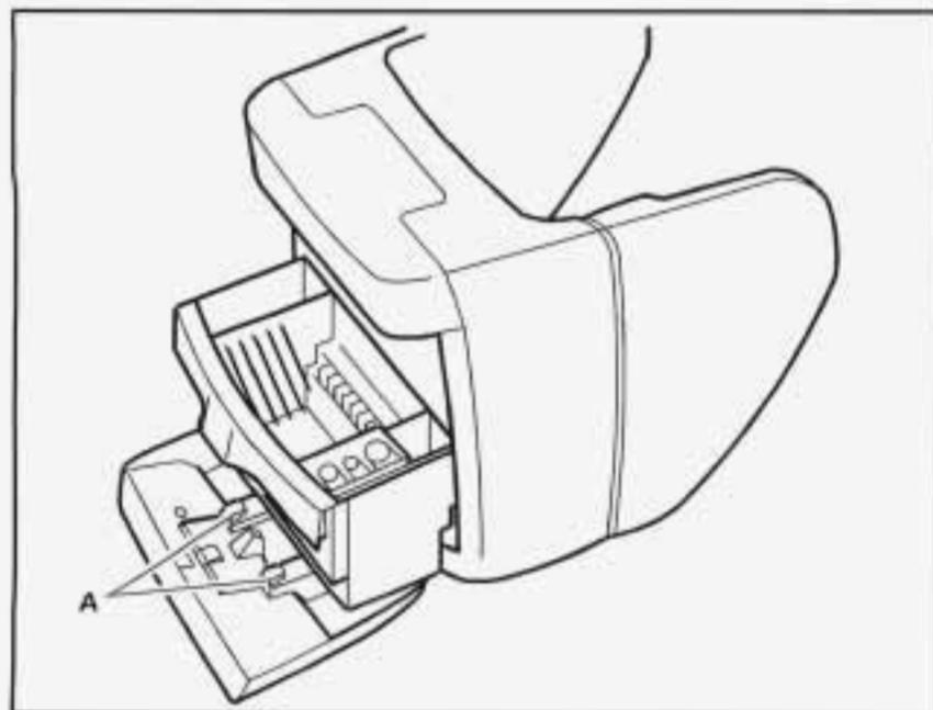
To remove the tray, slide it almost all the way out. Don't let the tray lock over the plastic tabs at the end of the guide rails (A). Lift the tray out of the guide rails. The rubber mat under the tray also lifts out for cleaning. When the rubber mat is replaced, be sure the tabs at the back of the mat are seated in the slots at the back of the storage bin.
