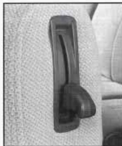
The seatback on the driver's seat folds forward to put items behind the seat. Lift the lever and fold the seatback forward. The seatback will lock into place when you push it back to the upright position.
