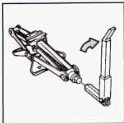
5. Attach the folding wrench to the jack, and rotate the wrench clockwise to raise the jack head a few inches.
