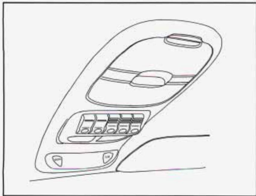
The optional front overhead console has reading lamps, a switchbank, storage compartments, including one for your garage door opener and one for your sunglasses, and a Driver Information Center (DIC). The features of the optional overhead console are explained on the following pages.
