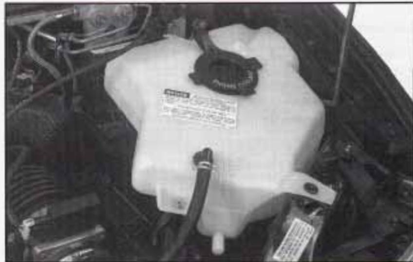
The coolant level should be at or above the FULL HOT mark. If it isn't, you may have a leak in the radiator hoses, heater hoses, radiator, water pump or somewhere else in the cooling system.
