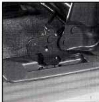
2. To do this, the bench seat will need to be angled so that the front hooks clear the floor pins.
