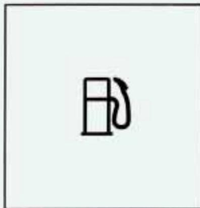
When there is between 4 gallons (15 L) and 2 gallons (7.6 L) of fuel left in the tank, the warning light next to the fuel symbol will go on.
