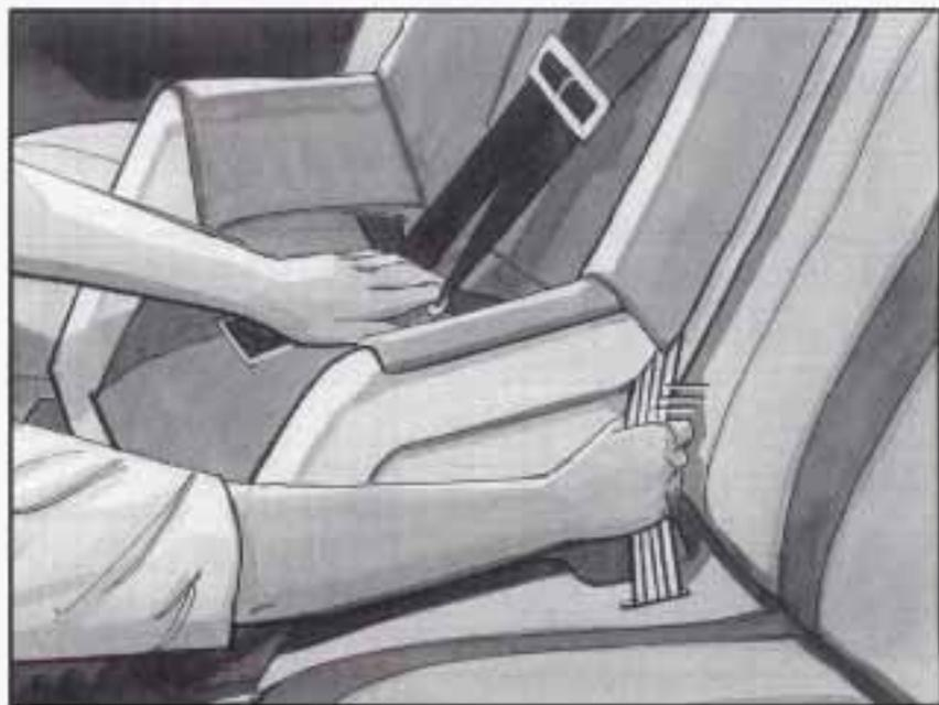
6. To tighten the belt, feed it back into the retractor while you push down on the child restraint.
