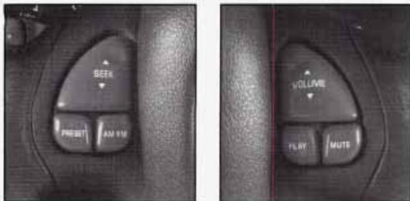
If your vehicle has this feature, you can control certain radio and remote playback functions using the buttons on your steering wheel.
