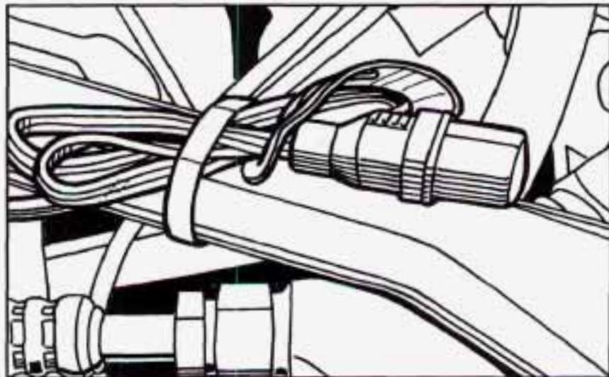
In very cold weather, 0°F (-18°C) or colder, the engine coolant heater can help. You'll get easier starting and better fuel economy during engine warm-up. Usually, the coolant heater should be plugged in a minimum of four hours prior to starting your vehicle.
