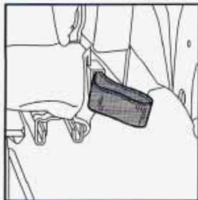
To fold down the seatback, pull the nylon strap on the back of the seat.
