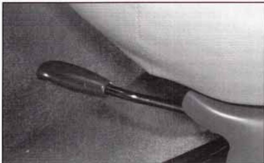
Use the lever on the front left side of the seat to adjust the seat forward or backward. Pull up the lever on the front of the seat to unlock it. Slide the seat to where you want it. To make sure the seat is locked into place, release the lever and try to move the seat with your body.
