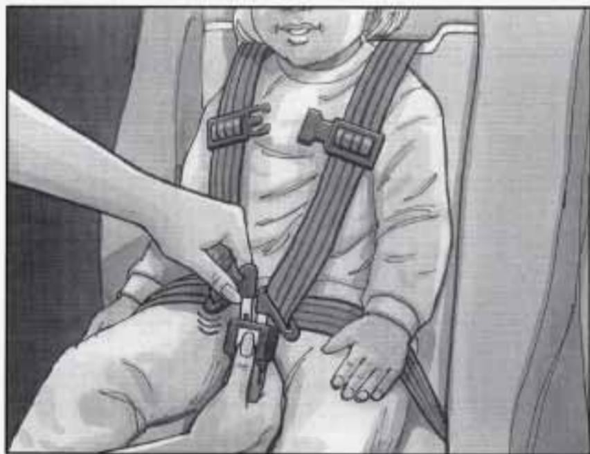
2. Unlatch the harness by pushing the button on the buckle.
