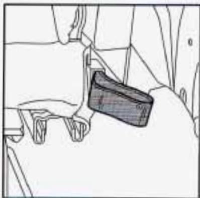
To fold down the seatback, pull the nylon strap on the back of the seat or lift up on the lever on the front of the seatback.
