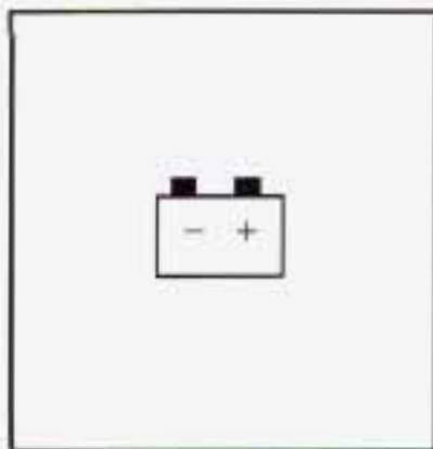
The charging system light will come on when you turn on the ignition as a check to show you it is working. It will remain on as long as the engine is not running.
