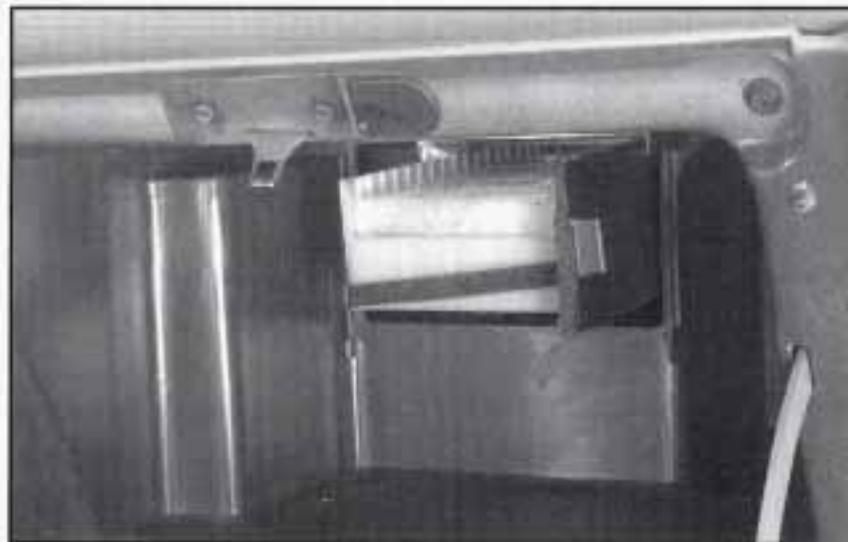
4. Replace the filters by reversing Step 3. Make sure the filters are inserted so that the sealing foam is angled in the same direction on both filters. For the type of filter to use, see "Normal Replacement Parts" in the Index.
