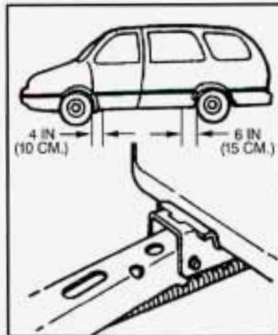
4. Near each wheel, there is a notch in the vehicle's body. Position the jack and raise the jack head until it fits firmly into the notch in the vehicle's frame nearest the flat tire.
