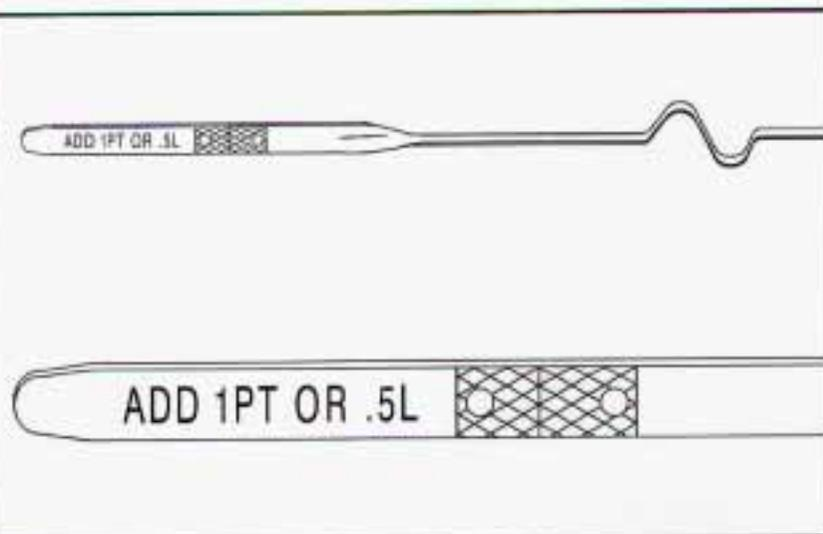
If the fluid level is low, add only enough of the proper fluid to bring the level into the cross-hatched area on the dipstick.
