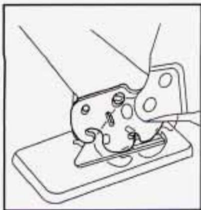
6. Remove the seat by rocking it slightly towards the rear of the vehicle and then pulling it out.
