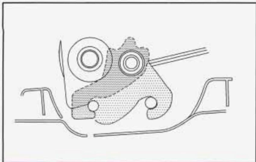
3. If the front legs are not attached correctly, the rear legs will not attach to the rear set of floor pins.
