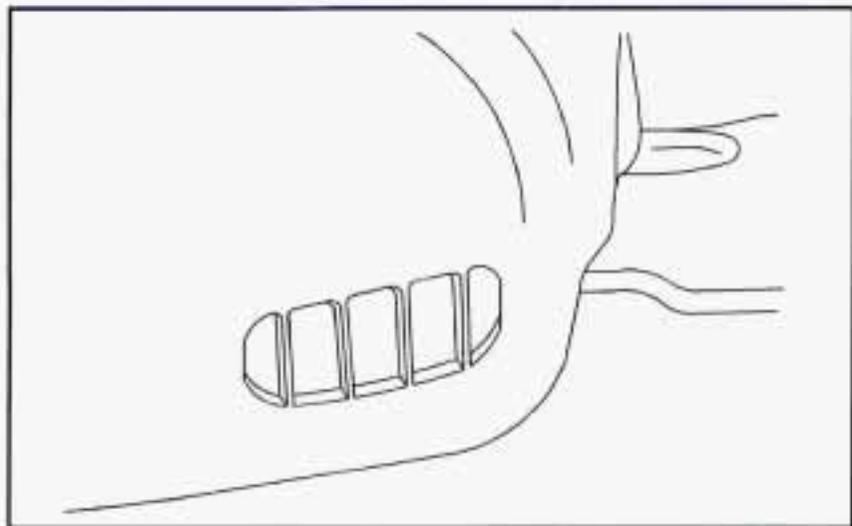
The vent behind the left rear seat is the cold air return vent. Be sure to keep it free of obstructions.
