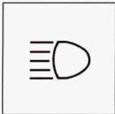
When the high beams are on, this light on the instrument cluster will also be on.
