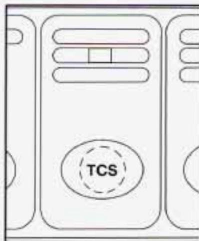
To turn the system off, press the TCS symbol on the bottom of the button in the center console switchbank. The indicator light on the traction control button will go off.
