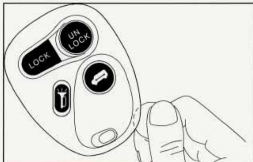
1. Insert a flat object like a dime into the slot on the side of the transmitter and twist to separate the halves.
