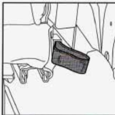
To fold down the seatback on either section of the split bench seat, pull the nylon strap on the back of the seat or lift up on the lever on the front of the seatback.
