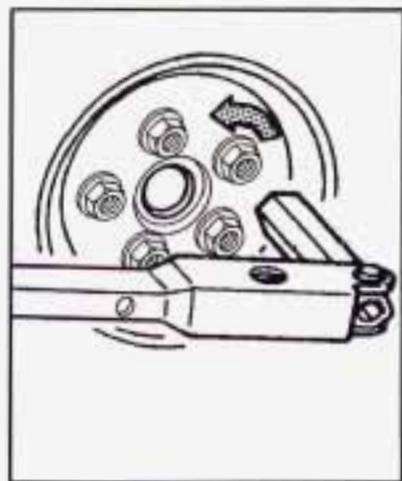
3. Loosen the wheel nuts -- but do not remove them -- using the folding wrench. (Turn the handle about 180°, then flip the handle back to the starting position. This avoids taking the wrench off the lug nut for each turn.)
