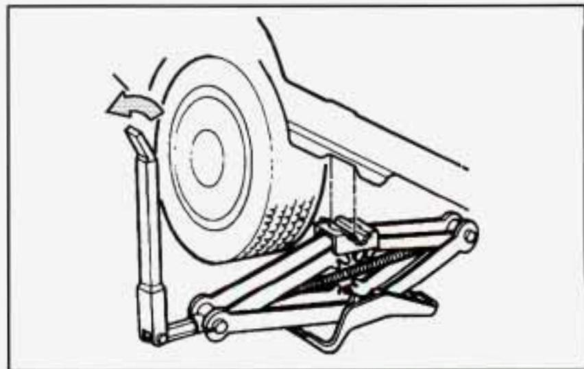
9. Lower the vehicle by attaching the folding wheel wrench to the jack and rotating the wrench counterclockwise. Lower the jack completely.
