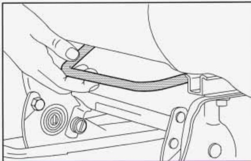
There are two adjustment levers on each section of the split bench seats to adjust the seat forward or rearward. They are located below the center of each section of the split bench, one in front and one in back of the seat.
