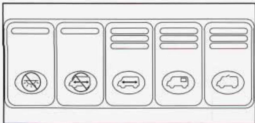
This switchbank is located in the overhead console. The switches that you may find in this switchbank are the Interior Lights Override, Power Sliding Door Override, Power Sliding Door, Power Rear Quarter Windows and Sunroof. If your vehicle does not have some of the options controlled by these switches, there will be a blank button in its place.
