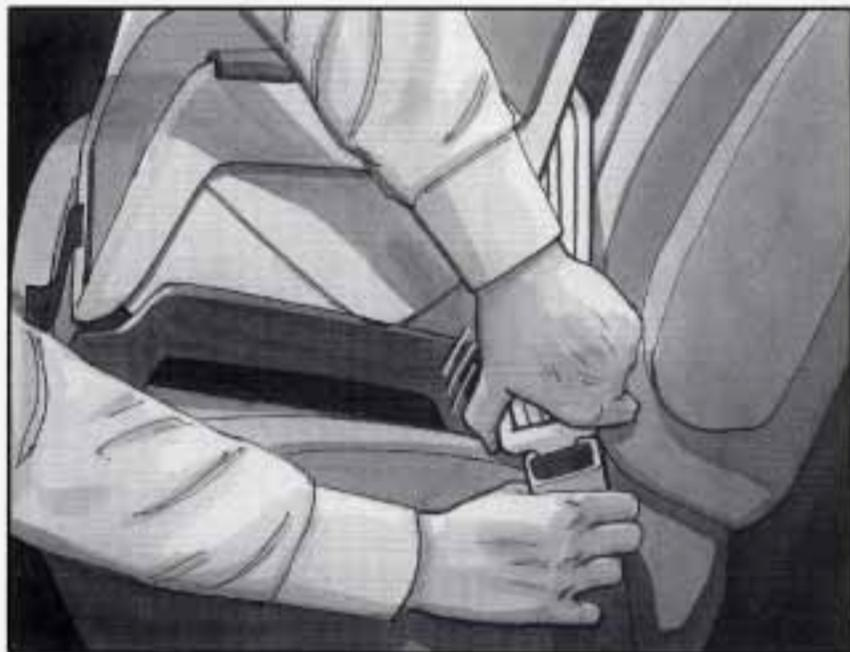
5. Buckle the belt. Make sure the release button is positioned so you would be able to unbuckle the safety belt quickly if you ever had to.
