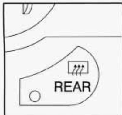
Press REAR (the light will glow) to warm the defogger grid on the rear window.
