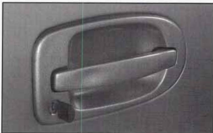
To unlock either sliding door from the outside using your key, insert the key and turn it toward the rear of the vehicle. To lock the sliding door from the outside, turn the key toward the front of the vehicle.
