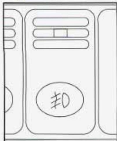
The fog lamps switch is located in the Instrument Panel switchbank.
