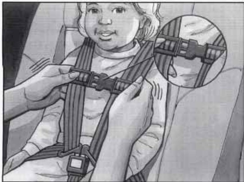
11. Now fasten the left and right halves of the shoulder harness clip together. The purpose of this clip is to help keep the harness positioned on the child's shoulders.
