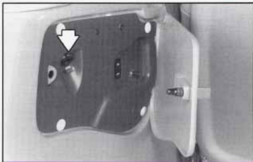
The rear power outlet is located in the rear compartment on the driver's side. To remove the cover, pull the tab on the cover and pull it off.
