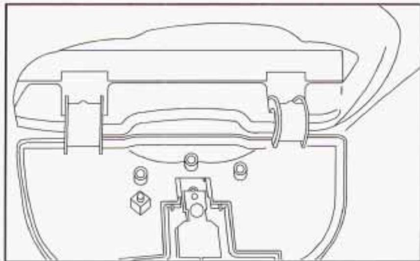
5. Add one peg at a time until your garage door opener operates with the compartment door closed when you press the button.
