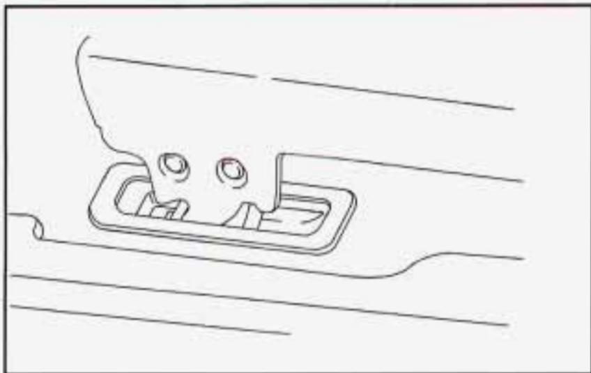
2. Push the rear of the seat down to lock the rear latches onto the rear set of floor pins.
