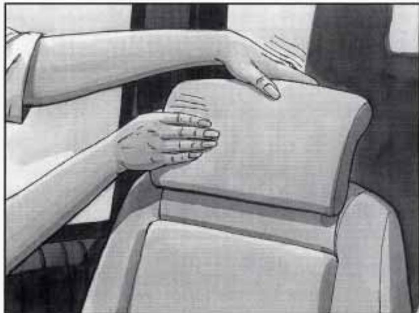
5. Rotate the head restraint forward and push it all the way down.
