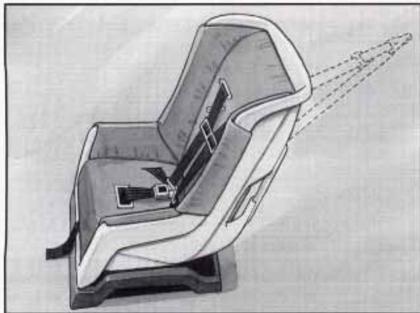
If your child restraint has a top strap, it should be anchored. A child restraint with a top strap should only be used in the second row. If your vehicle has third row seats, anchor brackets for the second row outside positions are located just above the place where the third row lap-shoulder belts meet the floor.
