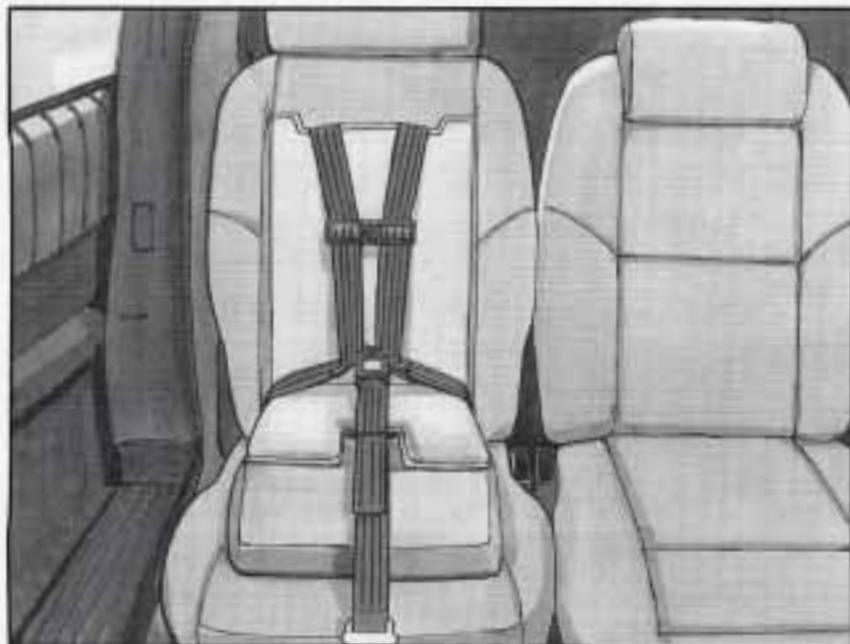
If your vehicle has this option in a bucket seat, each bucket seat that has the built-in child restraint fits in only one location in your vehicle. To find out where a bucket seat that has a built-in child restraint must be located in your vehicle, see "Removable Rear Bucket Seats" in the Index.
