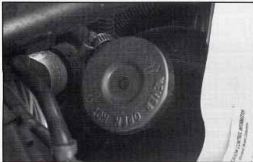
6. Then replace the pressure cap. At any time during this procedure if coolant begins to flow out of the filler neck, reinstall the pressure cap. Be sure the arrows on the pressure cap line up like this.
