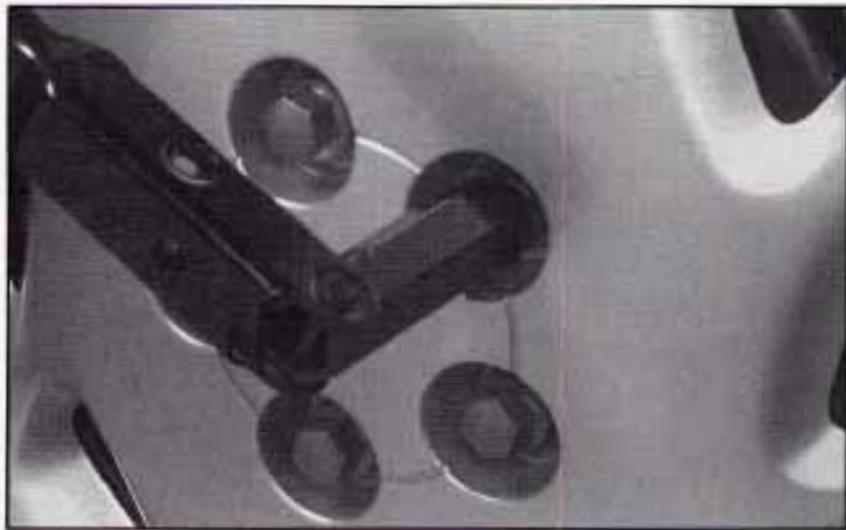
2. If your vehicle has the plastic "bolt-on" wheel covers, you cannot separate the nylon wheel nut caps from the cover. Loosen them completely using the folding wrench, and remove the wheel cover. If the wheel nut caps have been completely loosened, the wheel cover will come off easily.
