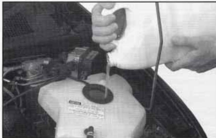
7. Then fill the coolant recovery tank to just below the words FULL COLD.
