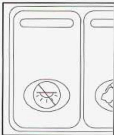
This switch is located in the overhead console switchbank. Press the symbol on the bottom of the rocker switch to override control of the interior lights and turn off power to the courtesy lamps, reading lamps, and glove box lamp.
