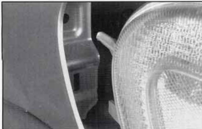
7. To replace the lamp assembly, line up and insert the tabs on the back of the assembly with the slots in the fender. Engage the lower clip on the front of the lamp assembly, keeping upper tab on the parking/turn signal lamp assembly inboard of the headlamp bracket tab.
