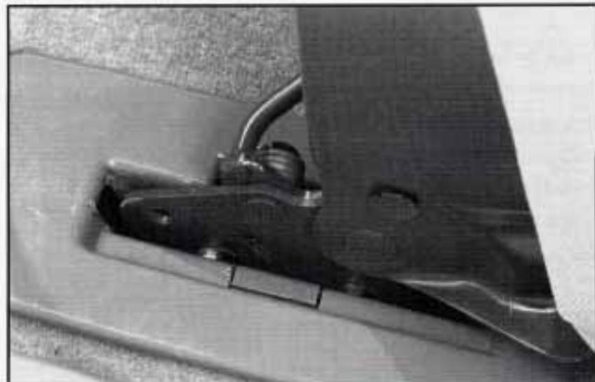
4. Firmly push the rear hooks into the rear floor pins by pushing down on the rear of the seat.
