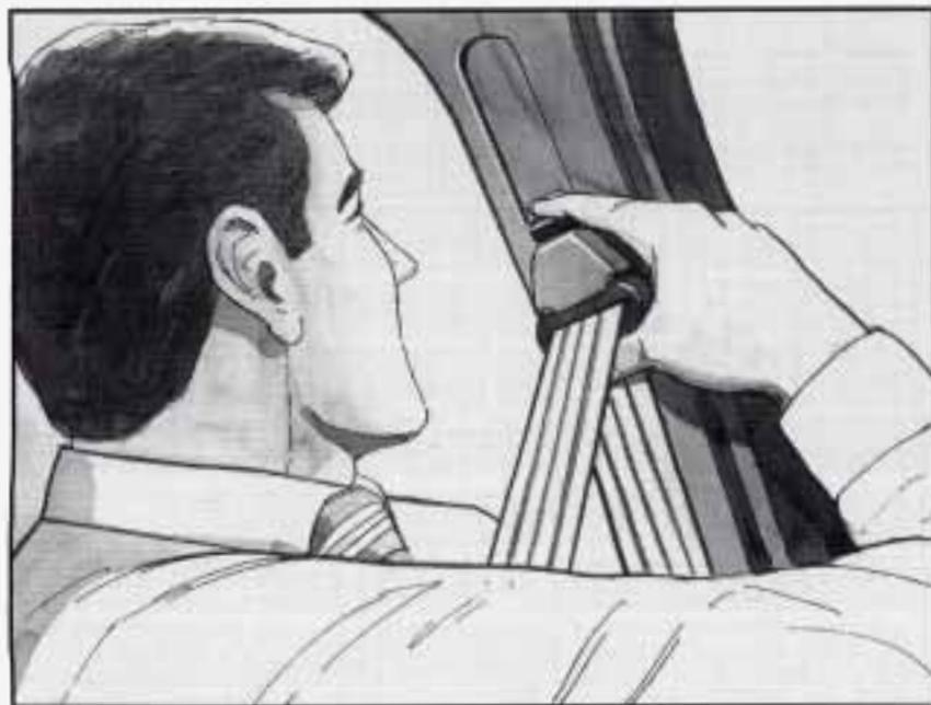
To move it down, push down on the button and move the height adjuster to the desired position. You can move the adjuster up just by pushing up on the shoulder belt guide. After you move the adjuster to where you want it, try to move it down without pushing the button down to make sure it has locked into position.
