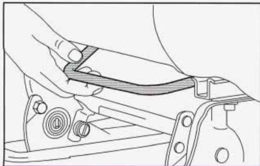
There are two adjustment levers on each seat to adjust the seat forward or rearward. They are located below the center, one in front and one in back of the seat.
