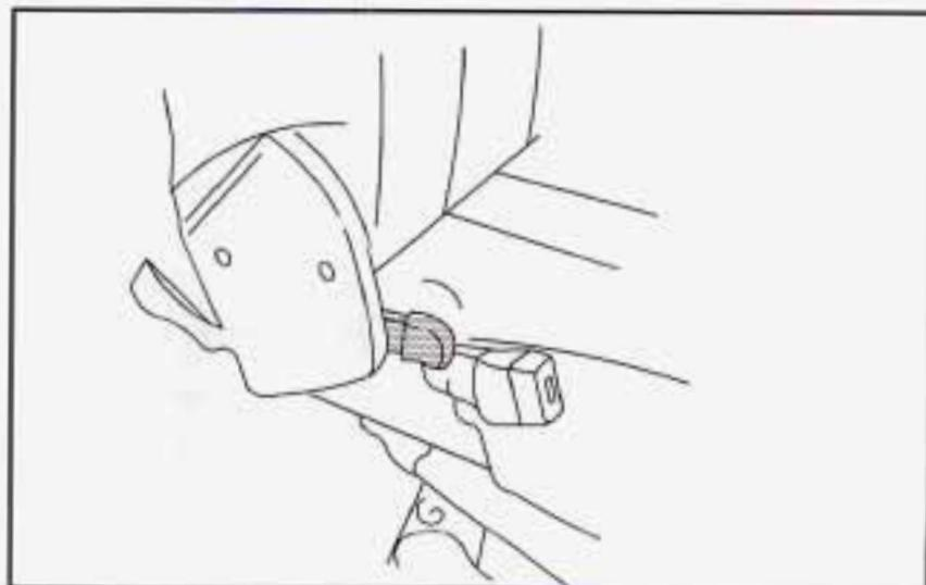
To raise the seatback, pull the nylon strap on the back of the seat while raising the seatback until it locks upright. Push and pull on the seatback to check that it is locked upright.
