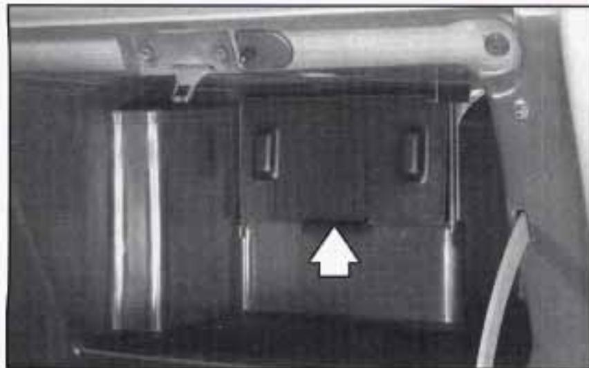
2. Then squeeze the tab on the left of the inner access panel.
