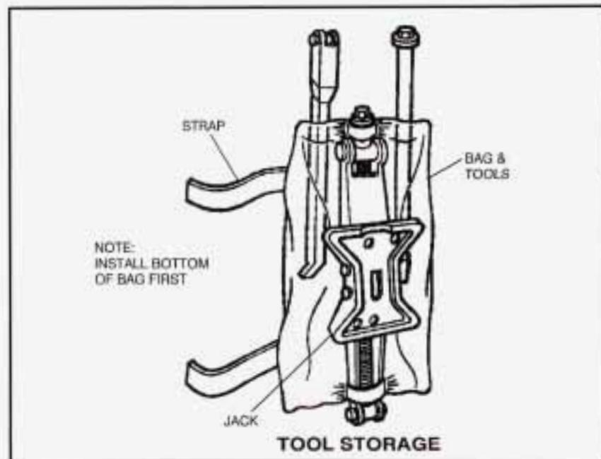
Replace all jacking tools as they were stored in the jack storage compartment and replace the compartment cover. To replace the cover, line up the tabs on the right of the cover with the slots in the cover opening. Push the cover in place and push down the tab so that it rests in the groove. This secures the cover in place.
