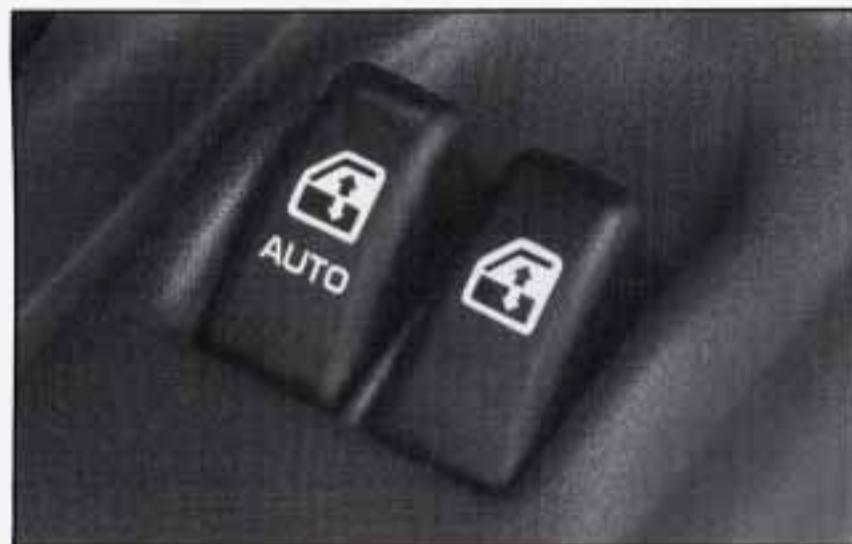
If you have power windows, the switches on the driver's door armrest control the front windows (when the ignition is on). The left switch controls the driver's window. The right switch controls the passenger's window.
