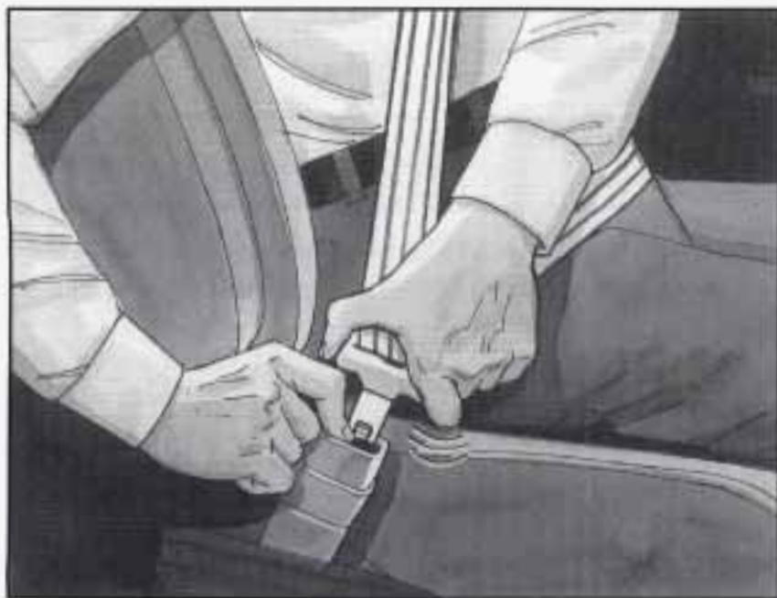
To unfasten the belt, just push the button on the buckle. The belt should go back out of the way.
