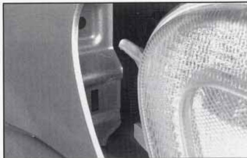
7. To replace the lamp assembly, line up and insert the tabs on the back of the assembly with the slots in the fender. Engage the lower clip on the front of the lamp assembly, keeping the upper tab on the parking/turn signal lamp assembly inboard of the headlamp bracket tab.
