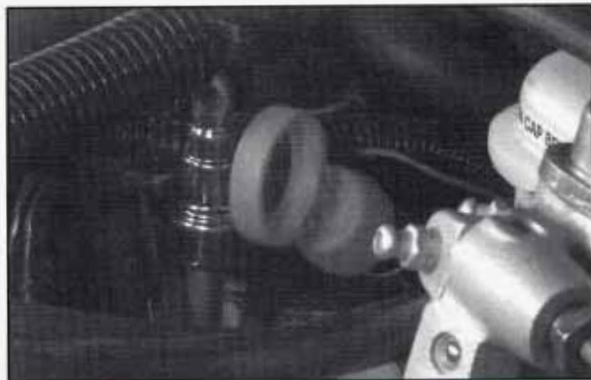
1. The dipstick is located toward the back of the engine compartment, near the center. The dipstick has a bright red loop design for easy identification. Pull out the dipstick and wipe it with a clean rag or paper towel.
