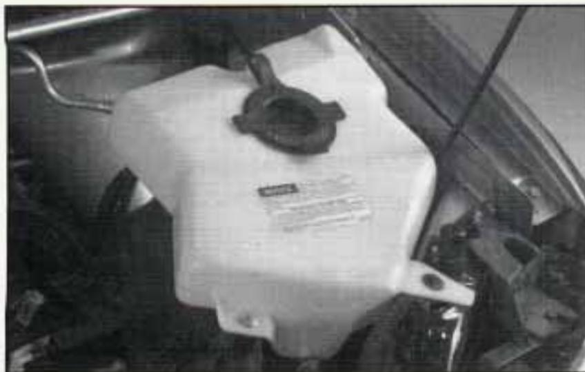
When your engine is cold, the coolant level should be at FULL COLD, or a little higher. When your engine is warm, the level should be up to FULL HOT, or a little higher.
