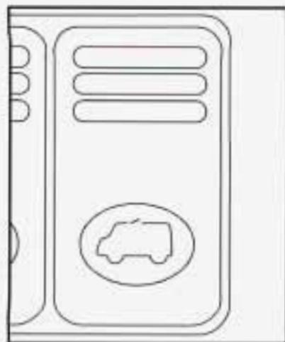
The power sunroof button is on the far right of the overhead console switchbank. The sunroof has two positions, vent and full open.
