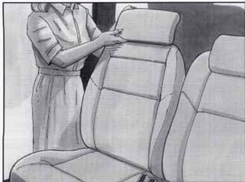
1. Raise the head restraint until the lower edge of the head restraint is even with the top of the seatback.
