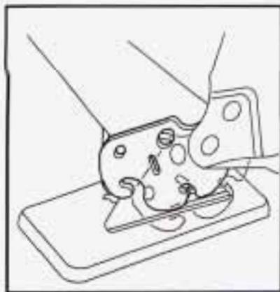
5. Remove the seat by rocking it slightly towards the rear of the vehicle and then pulling it out. This should be done in one motion.
