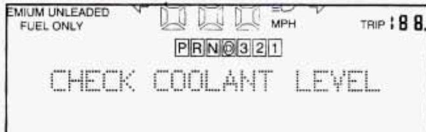
If the CHECK COOLANT LEVEL message comes on, it means you're low on engine coolant.
