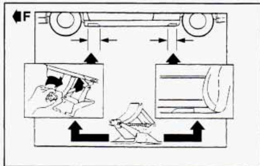
3. Position the jack under the vehicle and raise the jack lift head until it fits firmly into the notch in the vehicle's frame nearest the flat tire.
