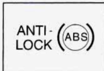
With the anti-lock brake system, the light(s) will come on when you start your engine and may stay on for several seconds. That's normal.
