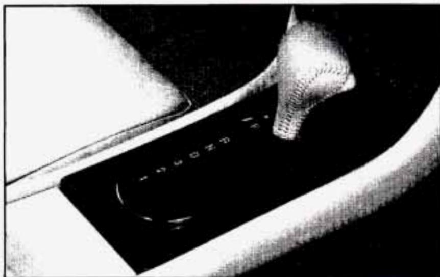
3. Hold in the button on the lever and push the lever all the way toward the front of your vehicle.
