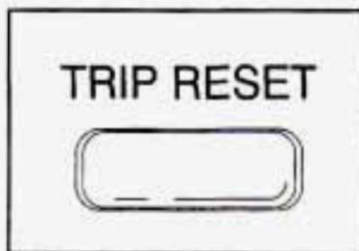
By pressing this button, you can tell how far you've traveled since you last set the trip odometer back to zero.
