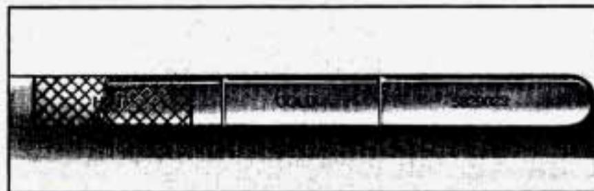
5. Check both sides of the dipstick, and read the lower level. The fluid level must be in the cross-hatched area.
