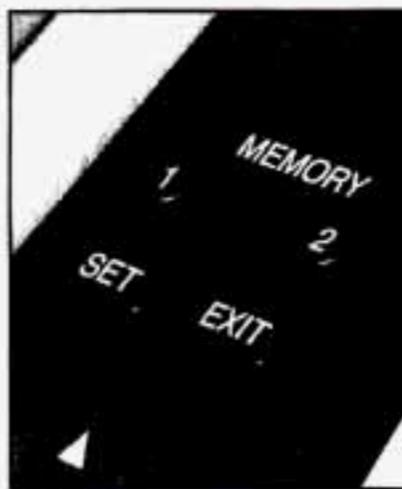
To begin programming, adjust the driver's seat (including lumbar adjustments) and both outside mirrors to a comfortable position and then press the SET button. Within five seconds, press button "1."
