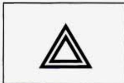
This light on the instrument panel will flash, indicating that the hazard warning flashers are on.
