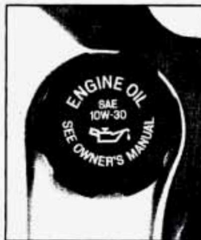
The oil fill cap is located behind the radiator on the passenger's side of the engine. Turn the cap to the left to remove it.
