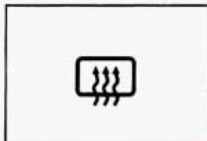
The lines you see on the rear window warm the glass. Press this button to turn on the rear defogger. With it, the rear window and both outside rearview mirrors are heated.
