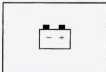
When you turn the key to RUN, this light will come on briefly to show that the generator and battery charging systems are working.
