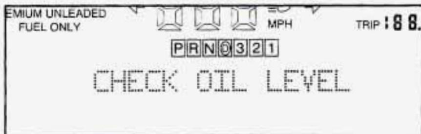
A CHECK OIL LEVEL message will appear when the engine oil is approximately 1 quart (1 L) low. If the message is displayed, check the dipstick level and add oil as needed.
