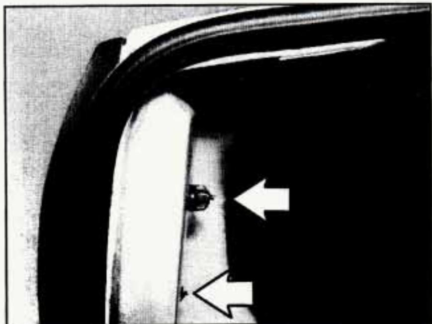
2. Remove the convenience net and pull the trim away to access the wing nuts.
