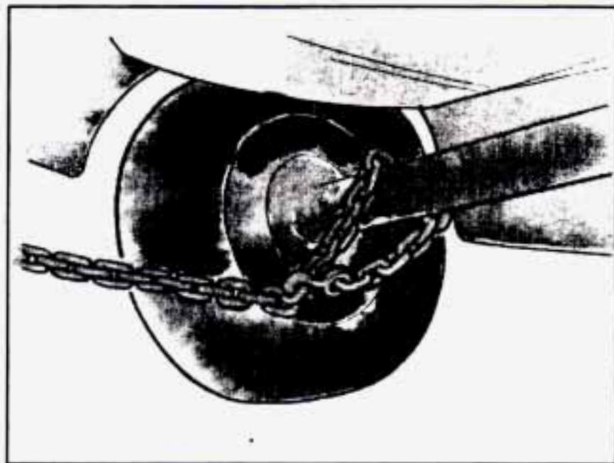
Attach a separate safety chain around the end of each axle inboard of the spring.
