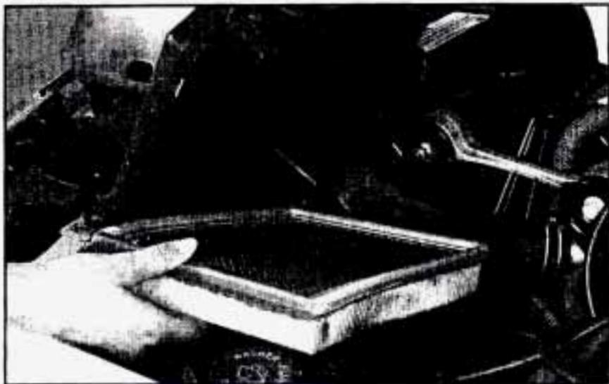
6. Take out the air cleaner filter and remove any loose debris that may be found laying in the air cleaner base.
