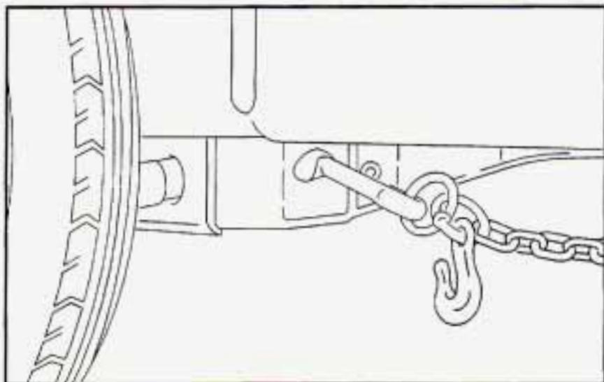
Attach T-hook chains on both sides, in the slotted holes in the bottom of the frame rails, behind the front wheels. These slots are to be used when loading and securing to car-carrier equipment.
