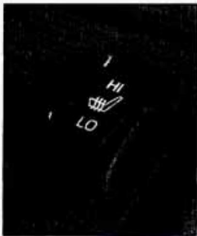
The control is located in the center console. Move the switch to LO or HI to turn on the heating elements in the seat. The LO setting warms the seatback and cushion until the seat approximates body temperature. The HI setting heats the seat to a slightly higher temperature.
