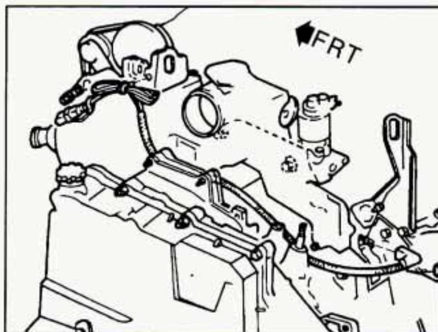
In very cold weather, 0°F (-18°C) or colder, the engine coolant heater can help. You'll get easier starting and better fuel economy during engine warm-up. Usually, the coolant heater should be plugged in a minimum of four hours prior to starting your vehicle.
