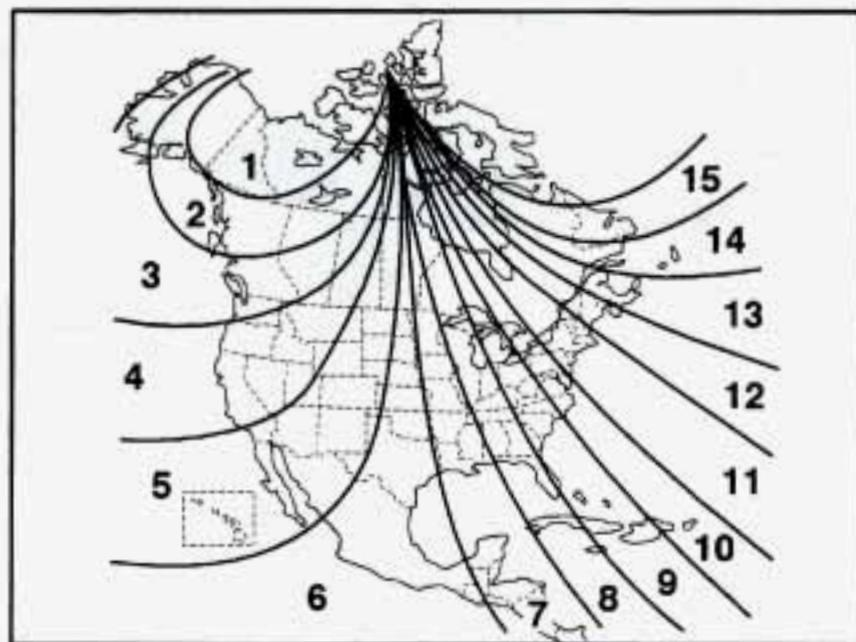
4. Press the COMPASS button on the bottom of the mirror until the new zone number appears in the display. After you stop pressing the button, the display will show a “C” in the direction display within a few seconds. (This is the automatic calibration mode -- you’ll need to drive in a circle to calibrate the mirror. See “Compass Calibration” following.)
