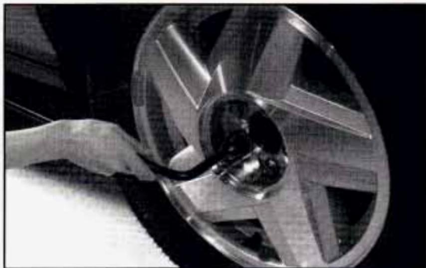
3. Then use the wheel wrench to *loosen* all the wheel nuts. Don't remove them yet.
