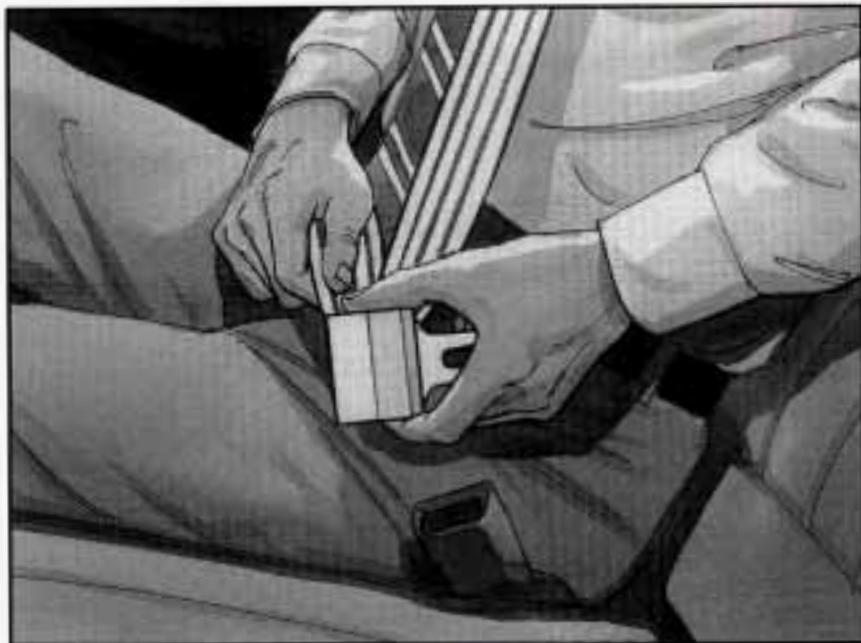
If the belt stops before it reaches the buckle, tilt the latch plate and keep pulling until you can buckle it. Pull up on the latch plate to make sure it is secure.
