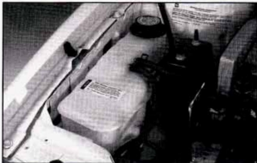
The coolant level should be at or above **FULL COLD**.
