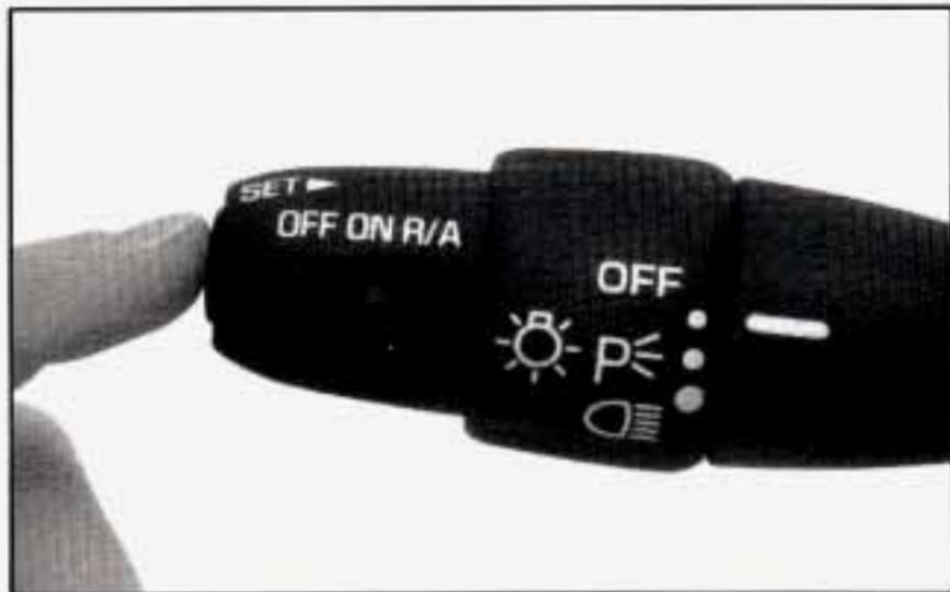
3. Press in the SET button at the end of the lever and release it.
