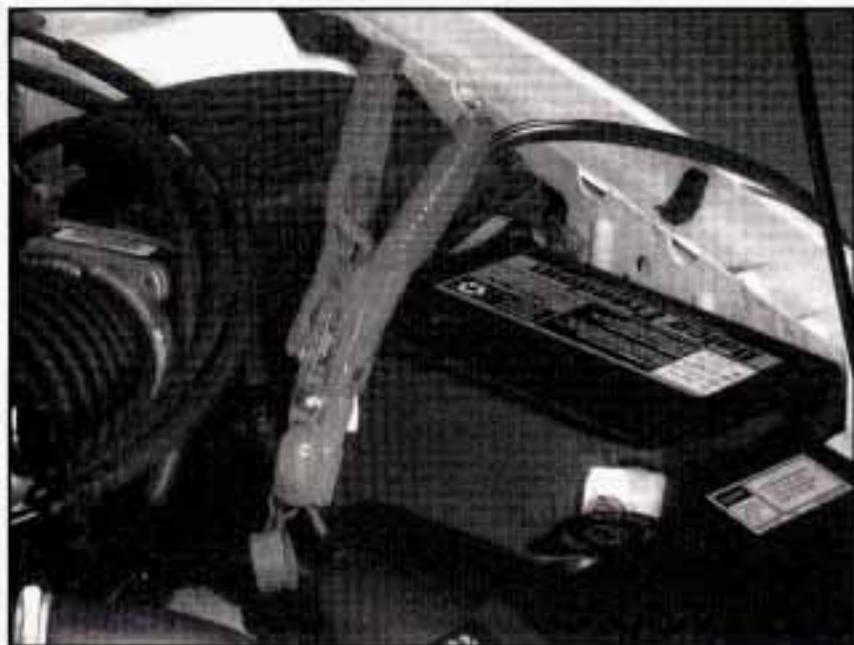
7. Connect the red positive (+) cable to the positive (+) terminal of the vehicle with the dead battery. Use a remote positive (+) terminal if the vehicle has one.
