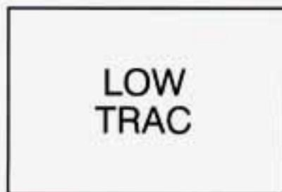
When your Enhanced Traction System is limiting wheel spin, this light will come on.
