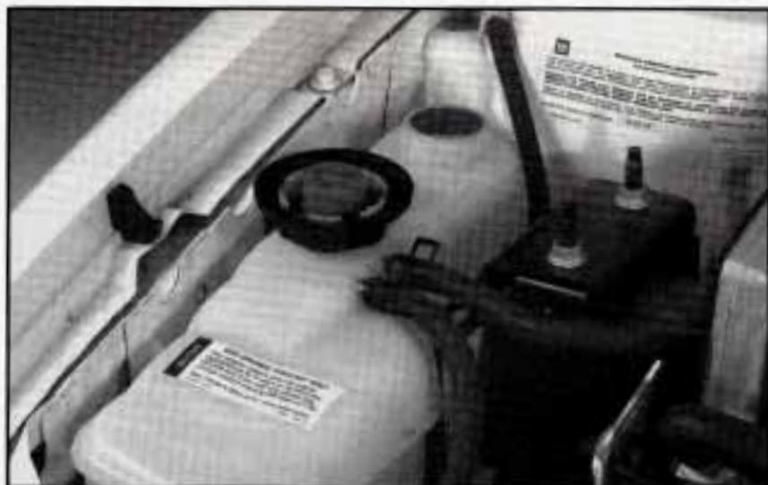
1. You can remove the coolant surge tank pressure cap when the cooling system, including the coolant surge tank pressure cap and upper radiator hose, is no longer hot. Turn the pressure cap slowly about one-quarter turn to the left and then stop.
