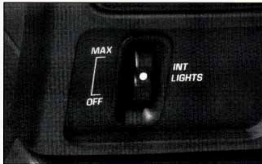
You can brighten or dim the instrument panel cluster lights by rotating the INT LIGHTS switch.
