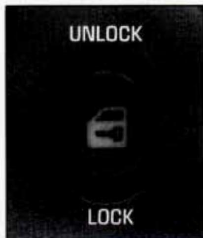
With power door locks, you can lock or unlock all the doors of your vehicle from the driver or front passenger door lock switch.
