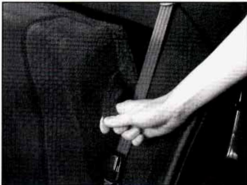
To fold down the rear seat, pull forward on the seat tab.
