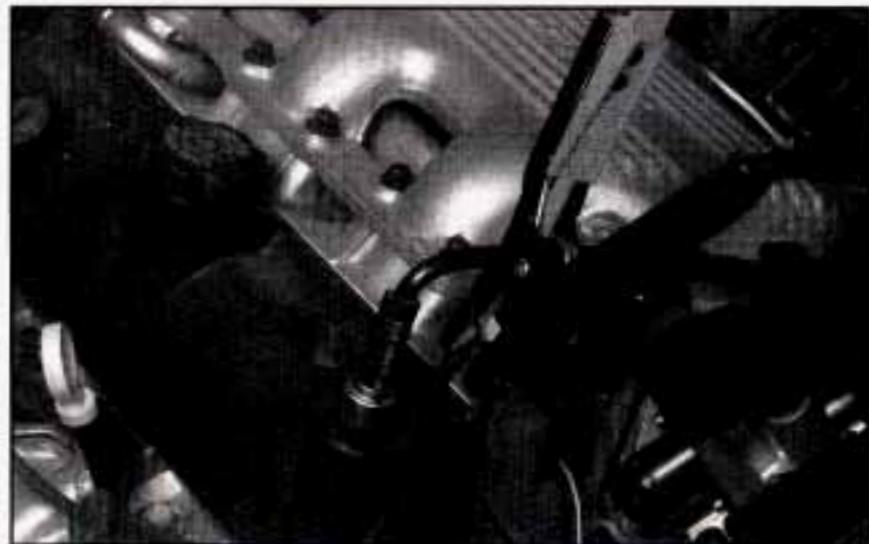
10. Attach the cable at least 18 inches (45 cm) away from the dead battery, but not near engine parts that move. The electrical connection is just as good there, but the chance of sparks getting back to the battery is much less.
