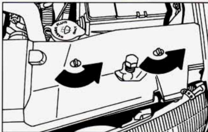
1. On the driver's side only, unscrew the butterfly fasteners. Then lift the plate.
