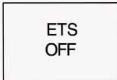
With the Enhanced Traction System (ETS), this warning light should come on briefly as you start the engine.
