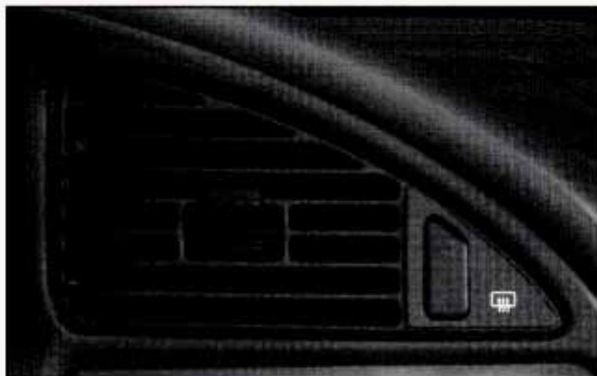
Adjust the direction of airflow by moving the louvered vents with the center control knob.
