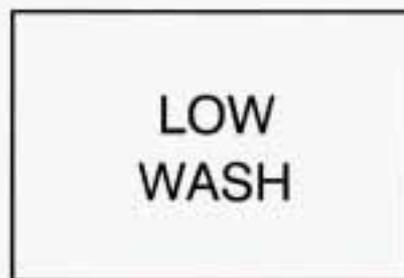
The LOW WASH light will come on when you turn on the ignition, and the fluid container is less than one-third full.
