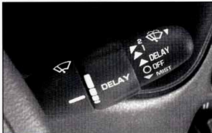
You control the windshield wipers by moving the stalk with the wiper symbol on it up or down.
