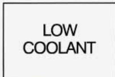
If this light comes on and stays on, the vehicle should promptly be pulled off the road and the coolant level checked.
