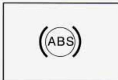
If there's a problem with the anti-lock brake system, this warning light will stay on. See "Anti-Lock Brake System Warning Light" in the Index.
