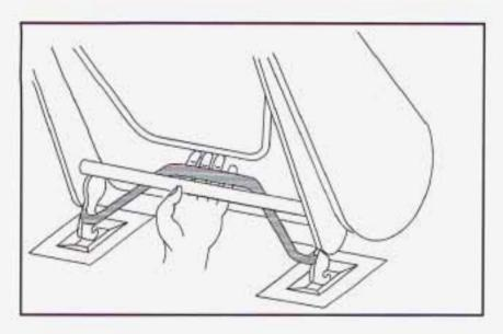
To unlatch the front latches, with the seat folded forward, squeeze the angled latch release bar toward the straight crossbar.
