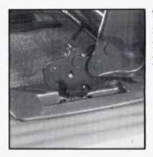
To do this, the seat will need to be angled so that the front hooks clear the floor pins.
