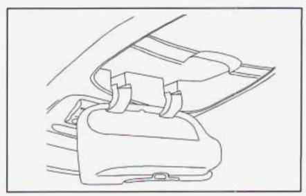
To open the sunglasses storage compartment in the overhead console, press the release button. Then pull the compartment down to the full open position.
