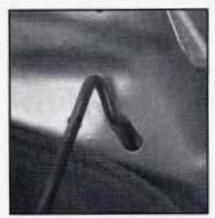
Pull forward on the hood prop to release it from its storage clip. Then put the end of the hood prop into the slot in the underside of the hood.
