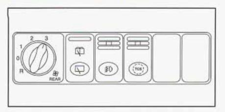
This switchbank is located in the instrument panel below the comfort controls. The switches and controls that you may find in this switchbank are the Rear Fan Knob, Rear Window Wiper/Washer, Fog Lamps and Traction Control. If your vehicle does not have some of the options controlled by these switches, there will be a blank button in its place.
