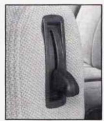
The seatback on the driver's seat folds forward to put items behind the seat. Lift the lever and fold the seatback forward. The seatback will lock into place when you push it back to the upright position.
