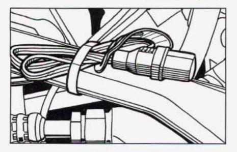
In very cold weather, 0°F (-18°C) or colder, the engine coolant heater can help. You'll get easier starting and better fuel economy during engine warm-up. Usually, the coolant heater should be plugged in a minimum of four hours prior to starting your vehicle.
