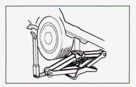
Lower the vehicle by attaching the folding wheel wrench to the jack and rotating the wrench to the left. Lower the jack completely.
