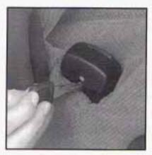
Push up the red center on the buckle with a small pointed object like a key or pen.
