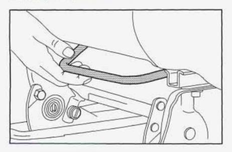
There are two adjustment levers on each section of the split bench seats to adjust the seat forward or rearward. They are located below the center of each section of the split bench, one in front and one in back of the seat.
