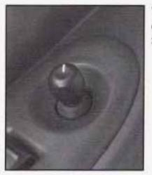
The control on the driver's door controls both outside rearview mirrors.
