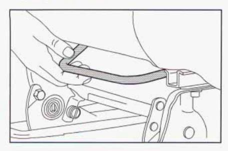
There are two adjustment levers on each seat to adjust the seat forward or rearward. They are located below the center, one in front and one in back of the seat.
