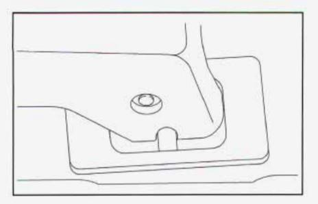
The seat can then be lifted off the front floor pins and removed from the vehicle.
