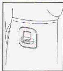
To open or close the sliding door, press and release one of the two power door switches. One is mounted on the wall, just in front of the passenger's side sliding door. The other switch is located in the overhead console switchbank.
