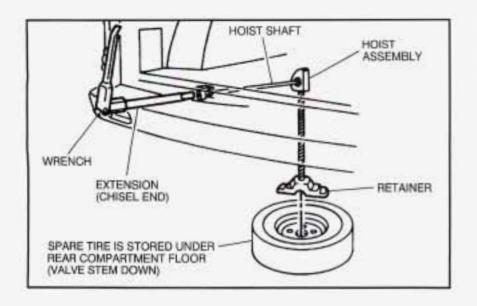
The compact spare tire is located under the vehicle, ahead of the rear bumper. Insert the narrow end of the shaft into the hole above the rear bumper. Then attach the folding wrench to the shaft.
