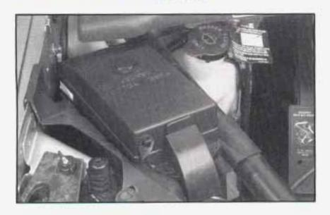
This fuse and relay center is located in the engine compartment, in front of the windshield washer fluid reservoir.
