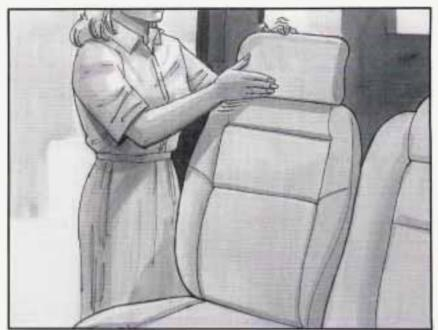
Rotate the head restraint rearward until it touches the top of the seatback. Make sure there is no gap between the lower edge of the head restraint and the top of the seatback.
