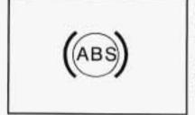
If there's a problem with the anti-lock brake system, this warning light will stay on or flash. See "Anti-Lock Brake System Warning Light" in the Index.
