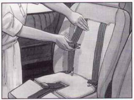
Move both latch plates and both sides of the shoulder harness clip to the bottom of the harness straps.
