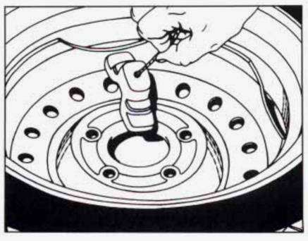
Slide the cable retainer through the center of the spare, then place the compact spare tire near the flat tire.
