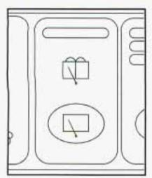
The rear window wiper switch is located in the instrument panel switchbank.
