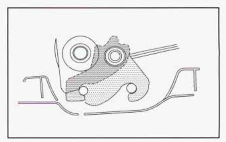
If the front legs are not attached correctly, the rear legs will not attach to the rear set of floor pins.
