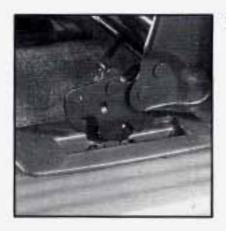
Place the front hooks of the bench seat onto the front two floor pins in the third row. To do this, the seat will need to be angled so that the front hooks clear the floor pins.
