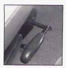
To use, pull up the lever on the front of the seat to unlock it.
