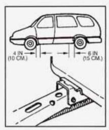
Near each wheel, there is a notch in the vehicle's body. Position the jack and raise the jack head until it fits firmly into the notch in the vehicle's frame nearest the flat tire.
