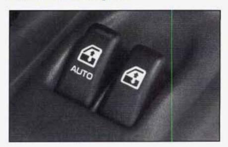
If you have power windows, the switches on the driver's door armrest control the front windows (when the ignition is in RUN or ACCESSORY). The left switch controls the driver's window. The right switch controls the passenger's window.
