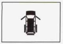
This light will come on if any of the doors or the liftgate are not completely closed and the ignition is turned to RUN or START.
