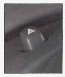
Your hazard warning flashers button is on top of the steering column. Press the button in to turn on your flashers.
