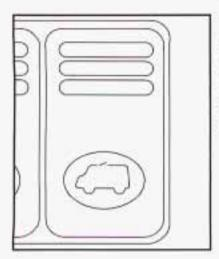
The power sunroof button is on the far right of the overhead console switchbank. The sunroof has two positions, vent and full open.
