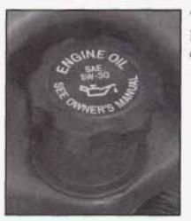
The engine oil fill cap is located just behind the engine oil dipstick.
