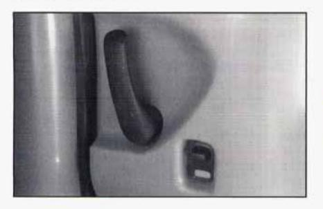
Lock the sliding door from inside the vehicle by moving the manual locking lever down. Unlock it by moving the lever up.
