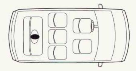
You'll be using the lap belt. Be sure to follow the instructions that came with the child restraint. Secure the child in the child restraint when and as the instructions say.
