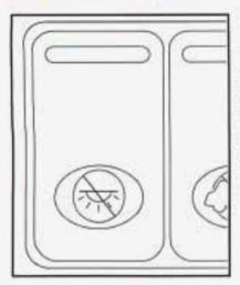
This switch is located in the overhead console switchbank. Press the symbol on the bottom of the rocker switch to override control of the interior lamps and turn off power to the courtesy lamps, reading lamps and glove box lamp.
