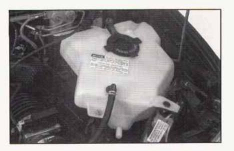
The coolant level should be at or above the FULL HOT mark.
