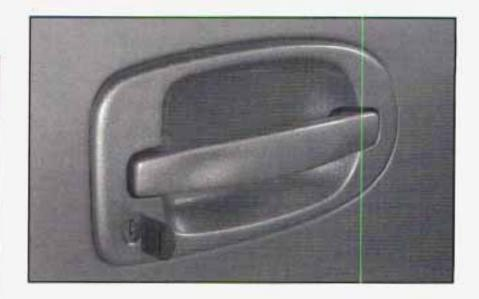
To unlock either front door from the outside with the key, insert the key and turn it toward the front of the vehicle.
