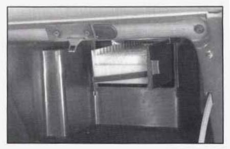
Then squeeze the tab on the left of the inner access panel.
