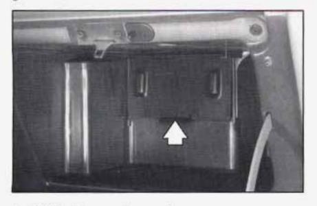
1. Pull the tab up and out on the outer access panel.
