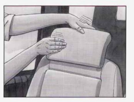
Rotate the head restraint forward and push it all the way down.
