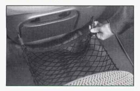
There is a storage net that stretches between the front seats. Pull the hooks towards the passenger's seat and insert them into the holes next to the cupholder.
