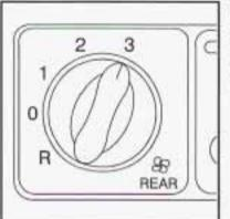
The rear fan control is located below the climate control system, in the switchbank.
