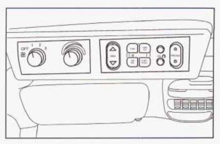
Turn the temperature knob to the left (to the blue area) for cooler air, or to the right (to the red area) for warmer air.
