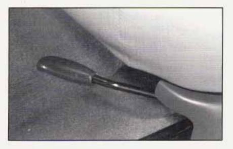
Use the lever on the front left side of the seat to adjust the seat forward or rearward. Pull up the lever on the front of the seat to unlock it. Slide the seat to where you want it. To make sure the seat is locked into place, release the lever and try to move the seat with your body.
