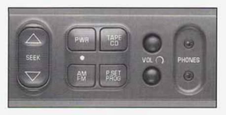
This feature allows rear seat passengers to listen to a different music source than the front seat passengers including AM-FM automatic tone control, cassette tapes or CDs. For example, rear seat passengers may listen to a cassette tape or CD through headphones while the driver listens to the radio through the front speakers. The rear seat passengers have control of the volume for each headphone. Be aware that the front seat audio controls always override the rear seat audio controls.
