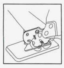
Remove the seat by rocking it slightly toward the rear of the vehicle and then pulling it out. This should be done in one motion.
