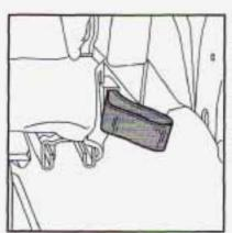
To raise either seatback, pull the nylon strap on the back of the seat while raising the seatback until it locks upright. Push and pull on the seatback to check that it is locked upright.
