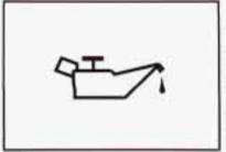
Your vehicle is equipped with an oil pressure warning light. Your oil pressure light lets you know when you may have a problem with your engine oil pressure.
