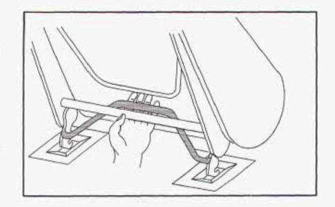
Squeeze the angled gray bar toward the solid gray crossbar while placing the front hooks of the bench seat onto the front two floor pins.
