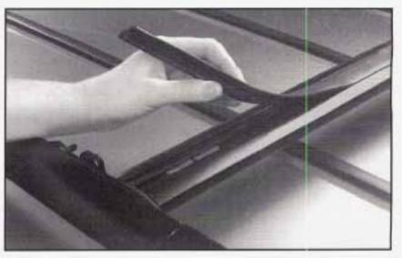
After removing the tiedowns or other equipment, be sure to reinstall the the piece of bumper strip that was cut.
