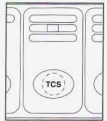
To turn the system off, press the TCS symbol on the bottom of the button in the center console switchbank. The indicator light on the traction control button will go off.
