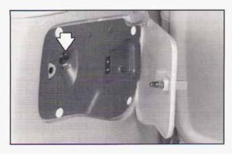
The rear power outlet is located in the rear compartment on the driver's side. To remove the cover, pull the tab on the cover and pull it off.
