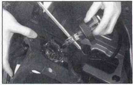
Replace the new bulb through the black retainer ring and into the electrical connector. Push the bulb firmly enough so that the blue tabs hook over the tab on the bulb.
