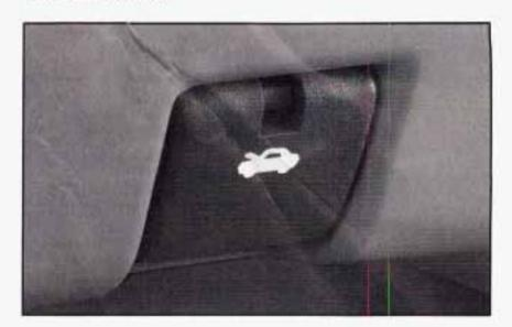
To open the hood, first pull the hood release handle inside the vehicle.
