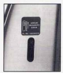
To use the security lock, move the security lock lever all the way up and close the door from the outside.
