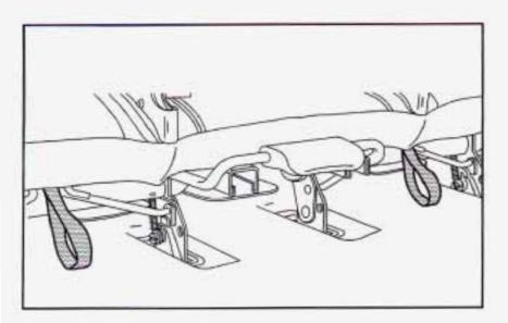
From behind the bench seat, pull the nylon straps at the base of the seat to release the rear latches from the floor pins. Do not let go of the straps until the seat is folded all the way forward.
