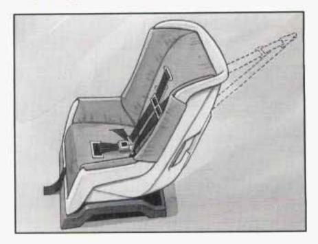
If your child restraint has a top strap, it should be anchored. A child restraint with a top strap should only be used in the second row. If your vehicle has third row seats, anchor brackets for the second row outside positions are located just above the place where the third row lap-shoulder belts meet the floor.
