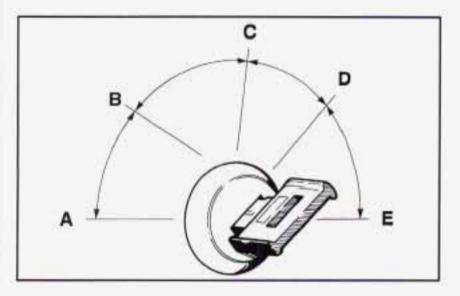
ACCESSORY (A): This is an on position in which you can operate your electrical power accessories. Press in the ignition switch as you turn the top of it toward you.
