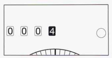
The trip odometer can tell you how far your vehicle has been driven since you last set it to zero. To set it to zero, push the reset button, which is located above and to the right of the temperature gage.
