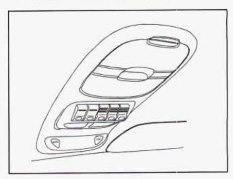
The optional front overhead console has reading lamps, a switchbank, storage compartments, including one for your garage door opener and another one for your sunglasses, and a Driver Information Center (DIC). The features of the optional overhead console are explained on the following pages.
