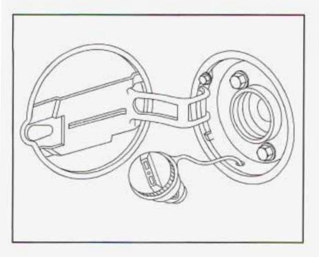
While refueling, hang the cap by the tether from the hook on the filler door hinge, or let the cap hang by the tether as shown.
