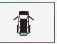
This light will come on if the power sliding door is not completely closed and the ignition is turned to RUN or START. If you shift the transaxle out of PARK (P) while the power sliding door is open or in the process of closing, and the power sliding door override feature is disabled, a buzzer will sound. This is a warning that the power sliding door is not completely closed.
