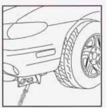
Attach T-hook chains in the front of the wheels, into the front shipping brackets on the frame (both sides). Insert the hook from the inward side of the slot, not the outward side.
