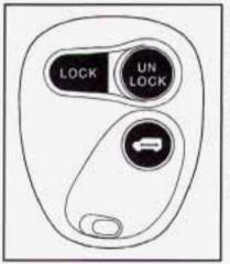
If you have the optional power sliding door (see "Power Sliding Door" later in this section), your remote transmitter will have a button that has a van symbol on it. Press it to open or close the sliding door.
