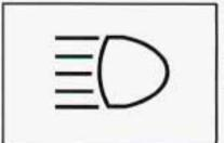
When the high beams are on, this light on the instrument cluster will also be on.
