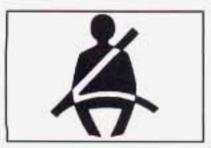
The safety belt light will also come on and stay on for about 70 seconds. If the driver's belt is already buckled, neither the chime nor the light will come on.
