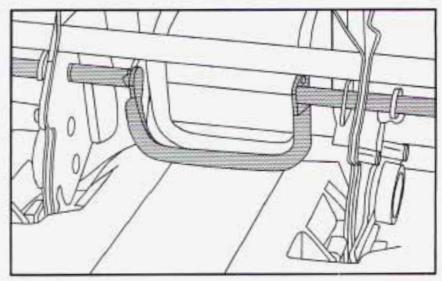
Unhook the front latches by rolling up the gray handle under the seat until the handle locks.
