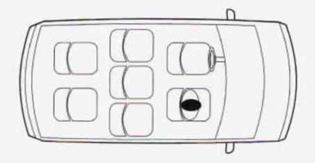
Your vehicle has a front passenger air bag. Never put a rear-facing child restraint in this seat. Here's why:
