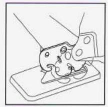
Remove the seat by rocking it slightly toward the rear of the vehicle and then pulling it out. This should be done in one motion.
