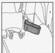
To raise the seatback, pull the nylon strap while raising the seatback until it locks upright. Push and pull on the seatback to check that it is locked.
