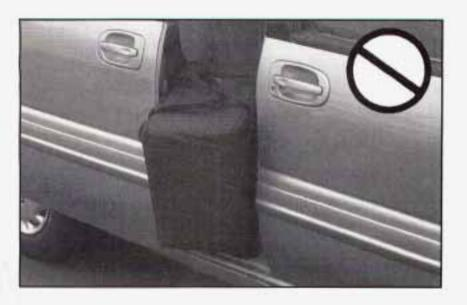
If anything obstructs the power sliding door while it is closing, the door will automatically reverse to the open position, provided it meets sufficient resistance.
