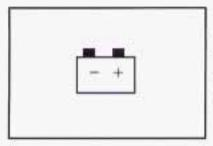
The charging system light will come on when you turn on the ignition as a check to show you it is working. It will remain on as long as the engine is not running.
