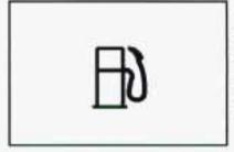
When there is between 4 gallons (15 L) and 2 gallons (7.6 L) of fuel left in the tank, the warning light next to the fuel symbol will go on.
