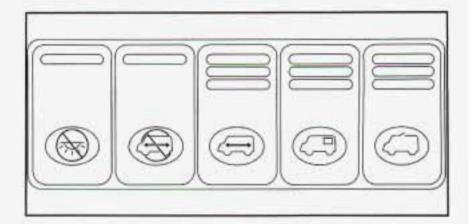
This switchbank is located in the overhead console. The switches that you may find in this switchbank are the Interior Lamps Override, Power Sliding Door Override, Power Sliding Door, Power Rear Quarter Windows and Sunroof. If your vehicle does not have some of the options controlled by these switches, there will be a blank button in its place.
