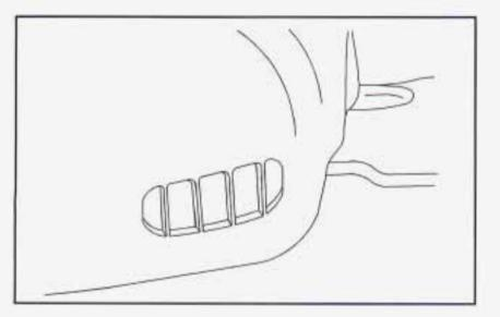
The vent behind the left rear seat is the cold air return vent. Be sure to keep it free of obstructions.
