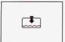
If this light comes on, your system is low on coolant and the engine may overheat.
