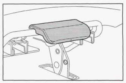
There are two levers to adjust the seat forward or rearward. They are below the center position of the bench, one in front and one in back of the seat.
