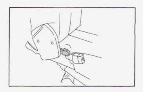
Use the lever on the front of the seatback to raise or lower the seatback to the desired position.
