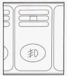
The fog lamps switch is located in the instrument panel switchbank. Push the fog lamp symbol on the rocker button to turn on the lamps.
