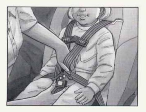
Pull up on both latch plates to make sure they are secure.
