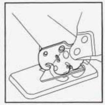
Remove the seat by rocking it slightly toward the rear of the vehicle and then pulling it out.
