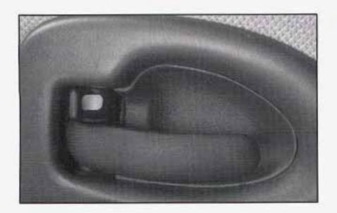
To lock either front door from the inside, push the locking lever forward.
