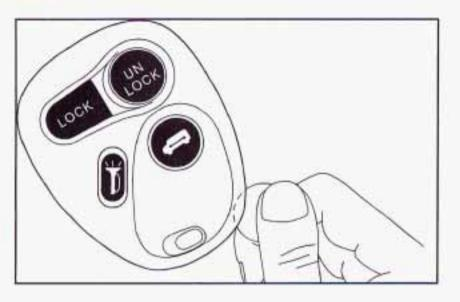
Insert a flat object like a dime into the slot on the side of the transmitter and twist to separate the halves.
