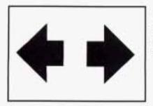
An arrow on the instrument panel will flash in the direction of the turn or lane change.
