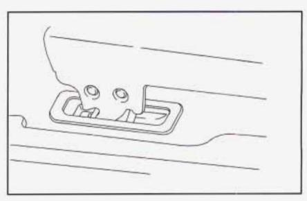
Push the rear of the seat down to lock the rear latches onto the rear set of floor pins.
