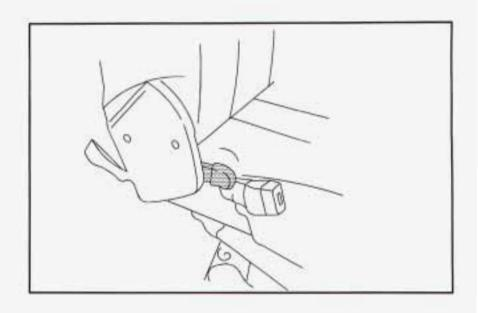
Use the lever on the front of the seatback to raise or lower the seatback to the desired position.
