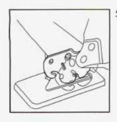
Remove the seat by rocking it slightly at the top toward the rear of the vehicle and then lift at the front latch release lever. This should be done in one motion.
