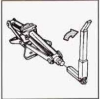
Attach the folding wrench to the jack, and rotate the wrench to the right to raise the jack head a few inches.
