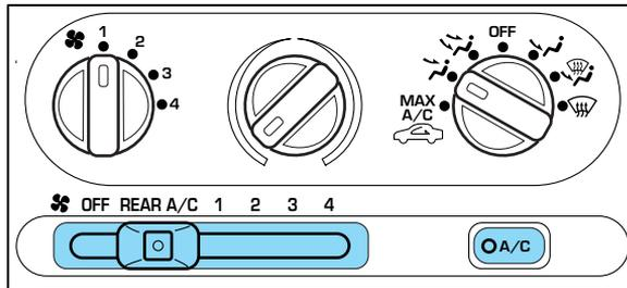
1. Set the main climate control rear fan control to Rear A/C, set the mode selector in any position (other than OFF), and depress the A/C control.
