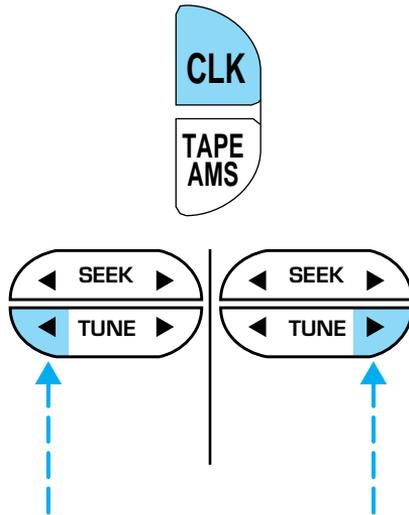
The CLK control will allow you to switch between media display mode (radio station, stereo information, etc.) and clock display mode (time). When in clock mode, the media information will display for ten seconds, when the radio is turned on, and then revert to clock information. Anytime that the media is changed, (new radio station, etc.), the media information will again display for ten seconds before reverting back to the clock. In media mode, the media information will always be displayed.
