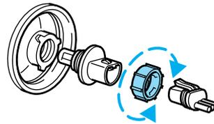
4. Without turning, remove the old bulb from its socket by gently pulling it straight back out of the lamp assembly.
