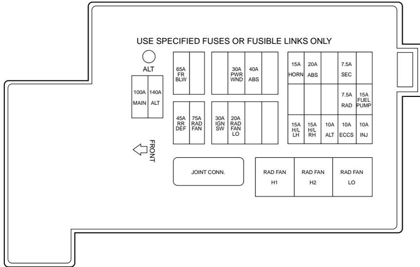
The high-current fuses are coded as follows.
