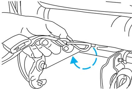
**If the tether strap is clipped incorrectly (as shown) the child safety seat may not be retained properly in the event of a collision.**
