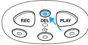
If the **DEL** button is inadvertently pressed or the time allotted (5 seconds) has passed, the indicator light will flash amber and an “error” tone will sound.
