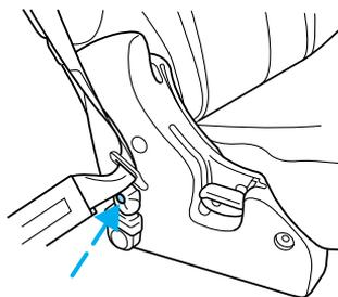
1. (Bench seats only) Disengage the lap/shoulder belt from the seat belt detach anchor by pushing the release control and lifting upward.
