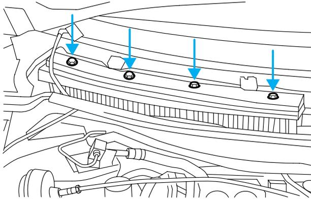
8. Remove four (4) screws from the top surface of the cabin air filter top cover.
