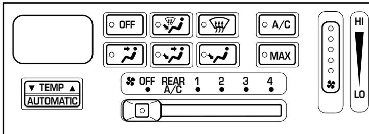
The EATC system will maintain a selected temperature and automatically control airflow. You can override automatic operation with any of the override controls or the fan speed control.
