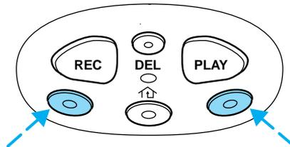
2. Hold the end of your hand-held transmitter 5–14 cm (2–5 inches) away from the HomeLink® Universal Transceiver surface (located on your visor) while keeping the red light in view.
