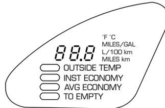
You can select different features for the message center to display by using the message center controls located to the left of the instrument panel.
