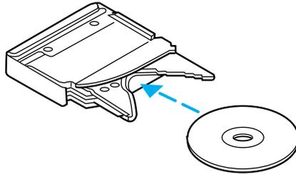
Ensure that the disc holder is evenly inserted and at the same level as the magazine (A). The unit will not operate if the disc holder is not inserted at the same level (B).
