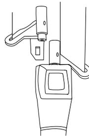
8. Fasten both halves of the chest clip below the child's shoulders and adjust it to comfortably hold the shoulder belts in place on the child's chest. The color green must appear in the indicator window when fastened.
