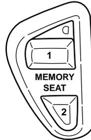
Position three (pressing 1 and 2 simultaneously) is always full rearward and downward for exit mode, but is not programmable.
