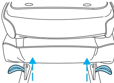
3. Lift up the back of the seat to clear the floor latches and then pull the seat rearward until the front hooks have come out of the floor anchors.
