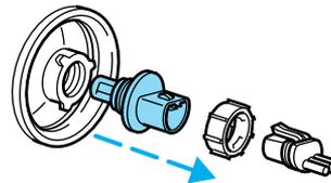
1. With the flat side of the new bulb's plastic base facing upward, insert the glass end of the bulb into the lamp assembly. Turn the bulb left or right to align the grooves in the plastic base with the tabs in the lamp assembly. When the grooves are aligned, push the bulb into the lamp assembly until the plastic base contacts the rear of the lamp assembly.
