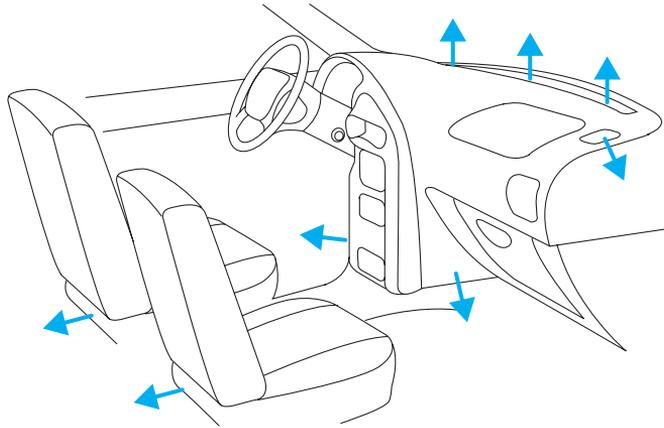
Rear seat heating is provided through the floor ducts located under the front seats. Airflow and temperature to the rear seating are regulated by the main climate control system.
