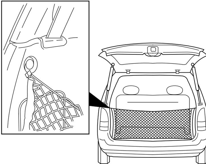
The cargo net helps stabilize lightweight objects in the cargo area. Attach the net to the anchors provided. The cargo restrained in the net must not exceed 22 kg (50 lbs.) or the net may not stay secured.
