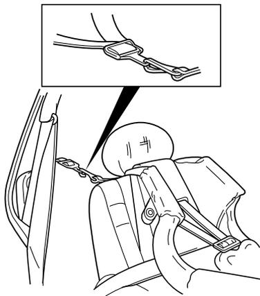
3. Adjust the tether strap length until the hook is about one foot behind the seatback.
