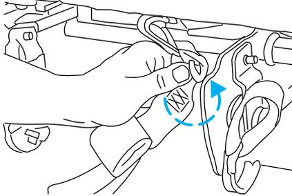
5. Clip the tether strap to the seat tether slot bracket at the lower rear portion of the seatback.
