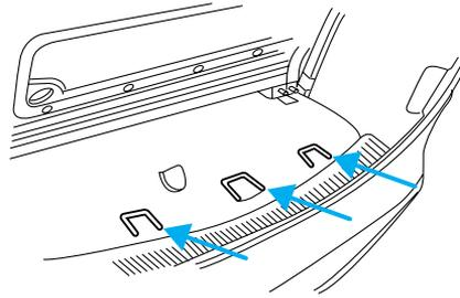
Tether anchorage hardware kits (part number 613D20) including instructions, may be obtained at no charge from any Ford or Lincoln-Mercury dealer. All vehicles built for sale in Canada include a tether anchor hardware kit.
