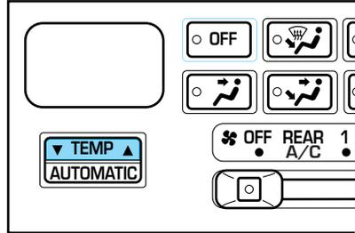
For continuous maximum cooling, push the temperature control until 15°C (60°F) is shown in the display window. The EATC will continue maximum cooling (disregarding the displayed temperature) until a warmer temperature is selected by pressing the temperature controls.
