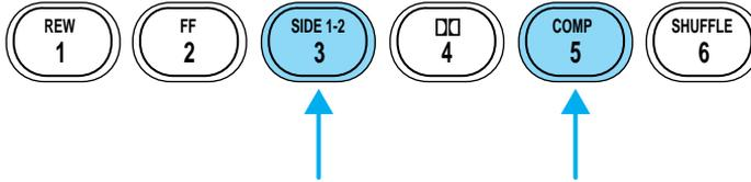
To turn on the rear seat controls, press the memory preset controls 3 and 5 at the same time. The
