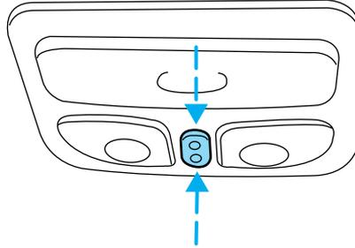
If the battery is disconnected, discharged, or a new battery is installed, the moon roof needs to be opened to the vent position to reset the moon roof positions.
