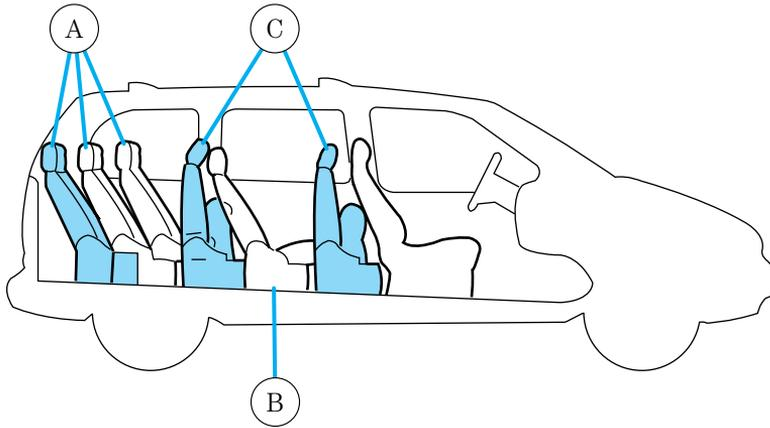
The entire seat can be moved to four seating positions and two storage positions.
