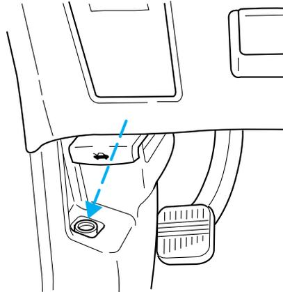
Use the following procedure to reset the fuel pump shut-off switch.
