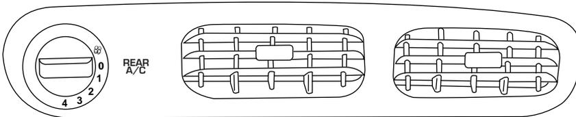
turn the Rear Fan Control on the main climate control system to Rear A/C and turn the Rear A/C Fan Control to 0.
