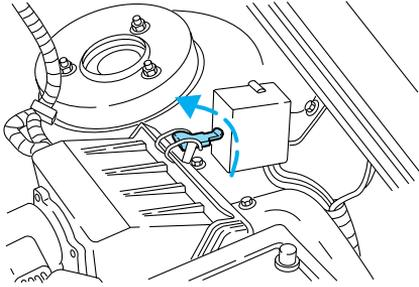
4. Install a new air filter element. Be careful not to crimp the filter element edges between the air filter housing and cover. This could cause filter damage and allow unmetered air to enter the engine if not properly seated.
