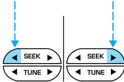
To set the minute, press and hold the CLK control and press the TUNE control:
