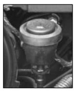
Refer to the Maintenance Schedule to determine how often you should check the fluid level in your clutch master cylinder reservoir and for the proper fluid. See "Owner Checks and Services" and "Recommended Fluids and Lubricants" in the Index.
