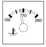
This gage shows the engine coolant temperature.
