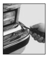
1. Remove the two screws and take out the parking/turn signal lamp assembly.
