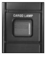
Press the top of the switch to turn the cargo lamp on. Press the bottom of the switch to turn it off.
