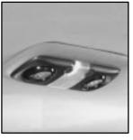
If your vehicle has reading lamps, press the button next to the lamp to turn the lamp on or off. The lamps can be adjusted to point in the direction you want.
