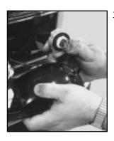
3. Pull the socket out of the lamp assembly.
