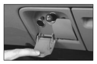
Two accessory power outlets are located near the cigarette lighter. Use these outlets to power mobile telephones or other devices designed to operate with vehicle electrical systems.
