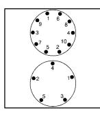
With a torque wrench, tighten the wheel nuts firmly in a crisscross sequence using the proper wheel nut torque.
