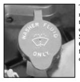
The windshield washer fluid reservoir cap is located on the driver's side of the engine compartment. See "Engine Compartment Overview" in the Index for more information on location.
