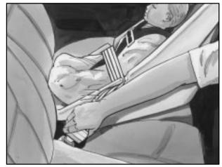
4. Buckle the belt. Make sure the release button is positioned so you would be able to unbuckle the safety belt quickly if you ever had to.
