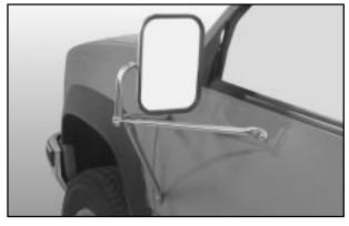
If your vehicle is equipped with the camper-type mirrors, they can be adjusted so that you can have a clear view of any objects that may be behind you.
