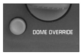
You can use the DOME OVERRIDE button, located below the parking lamp and headlamp knob, to set the dome lamp to come on automatically when a door is opened, or to remain off. To turn the lamp off, press the button "in". Press the button again and return it to the "out" position to set the dome light to come on.
