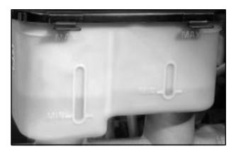
You can check the brake fluid without taking off the cap.
