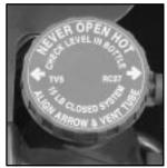
8. Then replace the pressure cap. At any time during this procedure if coolant begins to flow out of the filler neck, reinstall the pressure cap. Be sure the arrows on the pressure cap line up like this.
