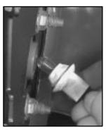
1. Remove the two screws and pull out the parking/turn signal lamp assembly.
