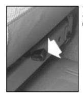
You can adjust the seat with this lever located at the front of the seat.
