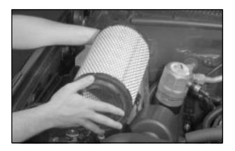
To remove the engine air cleaner/filter:
