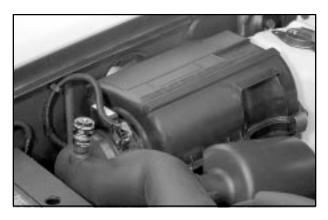
Your engine air cleaner/filter is located between the battery and coolant recovery tank.
