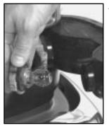
4. Pull the socket out of the lamp assembly.
