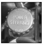
The power steering fluid reservoir cap is located at the front of the engine compartment. See "Engine Compartment Overview" in the Index for more information on location.
