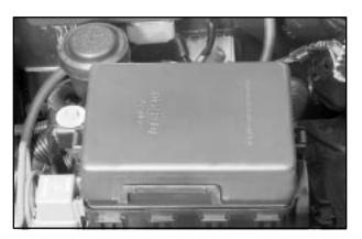
The underhood fuse/relay center is located in the rear of the engine compartment near the brake fluid reservoir. See "Engine Compartment Overview" in the Index for more information on location. Move the retainer clips for the cover to access the fuse block.
