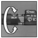
You control the windshield wipers by turning the knob with the wiper symbol on it.
