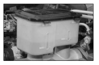
Your brake master cylinder reservoir is filled with DOT-3 brake fluid. See "Engine Compartment Overview" in the Index for the location of the reservoir.
