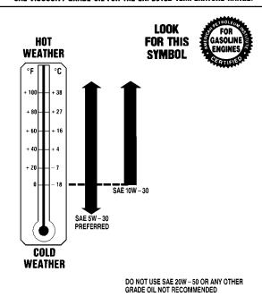
As in the chart shown previously, SAE 5W-30 is best for your vehicle. However, you can use SAE 10W-30 if it's going to be 0°F (-18°C) or above. These numbers on an oil container show its viscosity, or thickness. Do not use other viscosity oils, such as SAE 20W-50.
