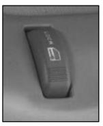
Press the top of the power door lock switch, marked LOCK, on either door to lock both doors at once. Press the ribbed side of the switch to unlock both doors at once.
