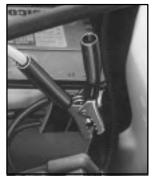
9. Now connect the black negative (-) cable to the good battery's negative (-) terminal.
