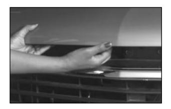
Then go to the front of the vehicle and pull up on the secondary hood release, located just to the passenger's side of the center of the grill.
