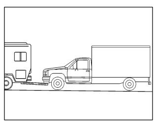
Your vehicle should not be towed with all four wheels on the ground. The transmission has no provisions for internal lubrication while being towed. To properly tow the vehicle, it should be placed on a platform trailer with all four wheels off the ground.
