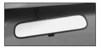
Push the tab under the mirror rearward to reduce glare from headlamps behind you after dark. Pull the tab forward for normal daytime operation.
