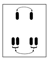
If the tread design for the front tires is different from the dual rear tires, always use the correct rotation pattern shown here when rotating your tires. The rear dual tires are rotated as a pair, and the inside rear tires become the outside rear tires.
