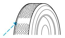
When replacing full size tires, never mix radial bias-belted, or bias-type tires. Use only the tire sizes that are listed on the Certification or Tire Label. Make sure that all tires are the same size, speed rating, and load-carrying capacity. Use only the tire combinations recommended on the label. If you do not follow these precautions, your vehicle may not drive properly and safely.
