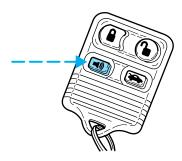
Pressing the trunk control will prevent the alarm from sounding until the trunk is closed again.
