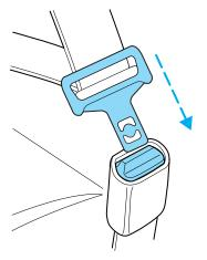
Grasp the shoulder portion and pull downward until the entire belt is extracted.
