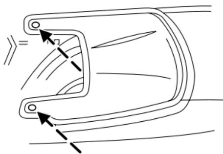
10. Insert boot tongue into groove located on rear of seat.
