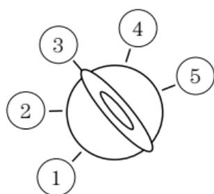
2. LOCK, locks the steering wheel, automatic transmission gearshift lever and allows key removal. For manual transmission, you must depress the ignition release lever.
