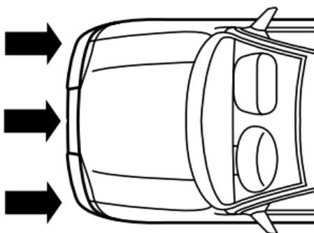
The fact that the air bags did not inflate in a collision does not mean that something is wrong with the system. Rather, it means the forces were not of the type sufficient to cause activation. Air bags are designed to inflate in frontal and near-frontal collisions, not rollover, side-impact, or rear-impacts unless the collision causes sufficient longitudinal deceleration.
