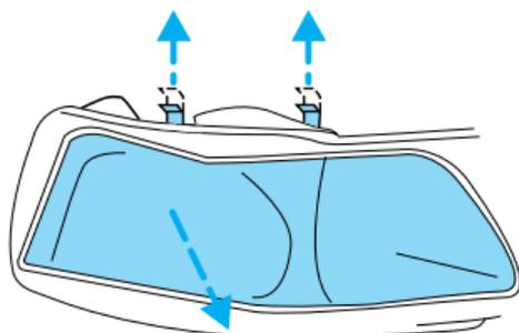
3. Pull headlamp assembly forward disengaging the lamp from the rear hidden snap retainers to expose the back of the bulb.
