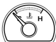
temperature, the needle remains within the normal area (the area between the “H” and “C”). If it enters the red section, the engine is overheating. Stop the vehicle as soon as safely possible, switch off the engine immediately and let the engine cool. Refer to *Engine coolant* in the *Maintenance and care* chapter.
