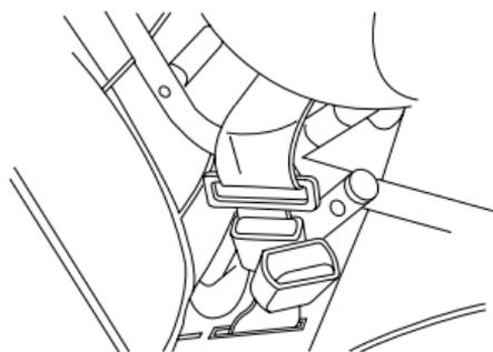
Ford recommends the use of a child safety seat having a top tether strap. Install the child safety seat in a seating position which is capable of providing a tether anchorage. For more information on top tether straps, refer to *Attaching safety seats with tether straps*.
