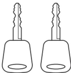
Large metallic objects, electronic devices on the key chain that can be used to purchase gasoline or similar items, or a second key on the same key ring as the **coded key** ignition key may cause vehicle starting issues. If present, you need to keep these objects from
