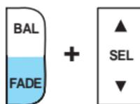
Press the FADE control. Use the SEL control to adjust the sound between the front and rear speakers.
