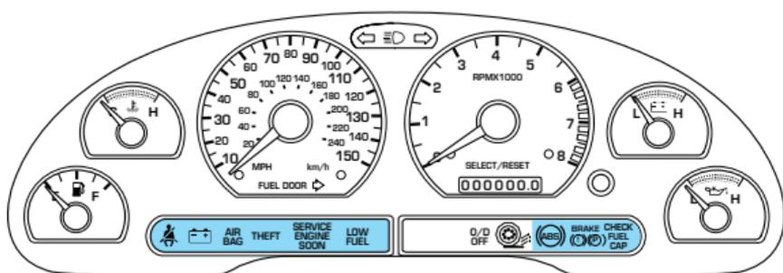
Make sure the corresponding lights illuminate or illuminate briefly. If a light fails to illuminate, have the vehicle serviced.
