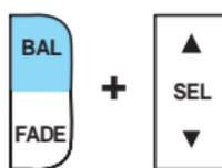
Press the BAL control. Use the SEL control to adjust the sound between the speakers.
