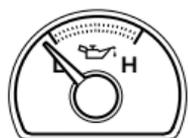
If the gauge indicates low pressure, stop the vehicle as soon as safely possible and switch off the engine immediately. Check the oil level. Add oil if needed (refer to *Engine oil* in the *Maintenance and care* chapter). If the oil level is correct, have your vehicle checked at your dealership or by a qualified technician.
