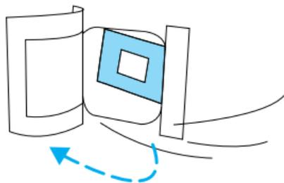
5. Clip the tether strap to the anchor as shown.
