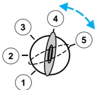
2. If the temperature is above  $-12^{\circ}\text{C}$  ( $10^{\circ}\text{F}$ ) and the engine does not start within five seconds on the first try, turn the key to OFF, wait 10 seconds and try again.
