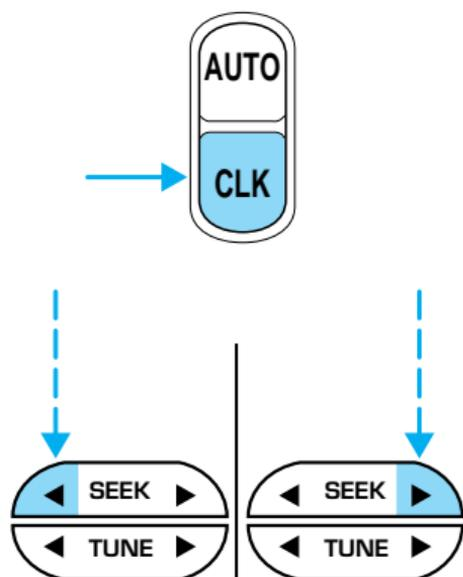
To set the minute, press and hold the CLK control and press TUNE:
