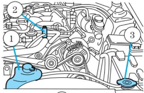
4. Add a **50/50 mixture** of engine coolant and distilled water to the radiator until full.
