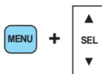
Use the SEL control to select TYPE (displays the RDS program type: rock, jazz, etc), NAME (displays the name of the radio station) or NONE (deactivates the RDS display).
