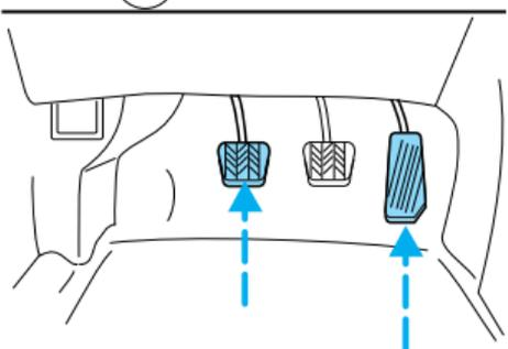
9. Slowly release the clutch pedal while slowly pressing down on the accelerator pedal.
