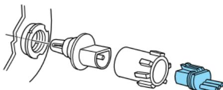
5. Remove the bulb retaining ring by rotating it counterclockwise (when viewed from the rear) to free it from the bulb socket, and slide the ring off the plastic base. Keep the ring to retain the new bulb.
