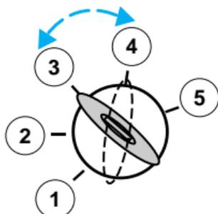
2. Turn ignition to 3 (OFF) then 2 (LOCK) and remove the first **coded key** from the ignition.
