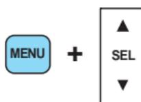
Use the SEL control to select the program type. With the feature on, use the SEEK or SCAN control to find the desired program type from the following selections:
