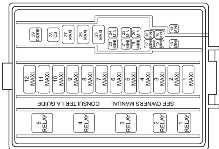
The high-current fuses are coded as follows.
