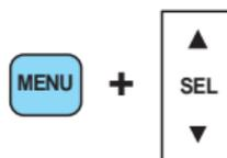
Press the MENU control until compression status is displayed. Press the SEL control to enable the compression feature when COMP OFF is displayed. Press the SEL control again to disable the feature when COMP ON is displayed.
