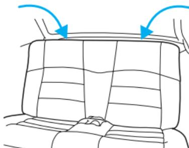
4. Access tether anchors located behind the seatback and pull away vinyl cover to expose anchors.
