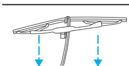
3. Attach the new wiper to the wiper arm and press it into place until a click is heard.
