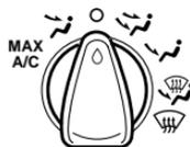
The air conditioning can operate in all modes. However, the air conditioning will only function if the outside temperature is about 6°C (43°F) or higher.
