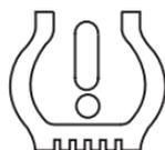
If the light remains on while driving, check the tire pressure refer to “*Checking the tire pressure*” in this chapter. The low tire warning indicator light will also illuminate when using a temporary spare, refer to “*Changing the tires*” in this chapter.
