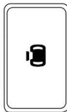
Press the left side of the ON/OFF control in the overhead console to turn off the PSD. This prevents opening the PSD using the rear seat control(s) or the handle; but the door(s) can be opened manually with the handle. The controls in the overhead console for right or left side and the Remote Entry System will remain functional with the system shut OFF.
