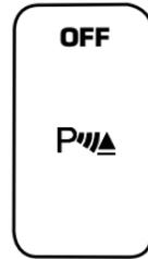
The OFF indicator remains illuminated when the system is disabled. The system defaults to ON every time the reverse gear is selected. Press the control to disable or enable the system.
