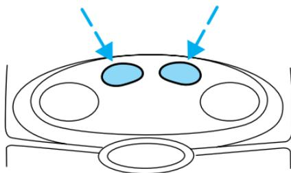
If equipped with a moon roof, the map lamps are located on the rearview mirror. Press the control next to the map lamp to illuminate the lamp.
