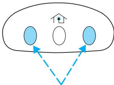
2. Hold the end of your hand-held transmitter 5–14 cm (2–5 inches) away from the HomeLink® Universal Transceiver surface (located on your visor) while keeping the red light in view.
