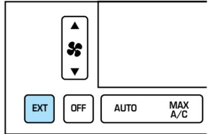
If the selected temperature is changed while the outside temperature is displayed, the new temperature will be displayed for four seconds after it is changed, then the outside temperature will return to the window.
