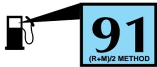
Do not be concerned if your engine sometimes knocks lightly. However, if it knocks heavily under most driving conditions while you are using fuel with the recommended octane rating, see your dealer or a qualified service technician to prevent any engine damage.
