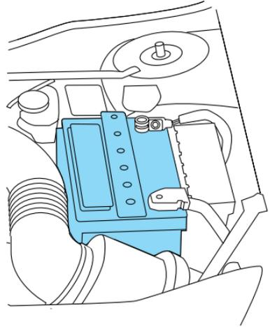
However, for severe usage or in high temperature climates, check the battery electrolyte level. Refer to the scheduled maintenance guide for the service interval schedules.
