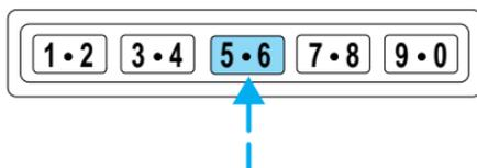
After the factory-set code or personal code has been entered, you can unlock all doors (press 3/4) and release the trunk (press 5/6) as long as the controls are pressed within five seconds of each other.
