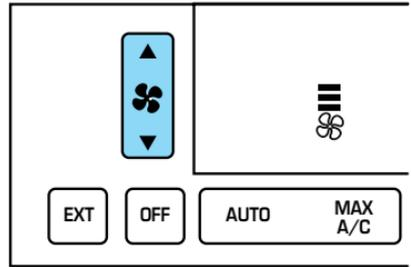
The display will show
