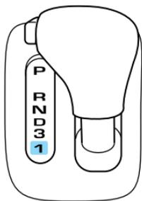
Do not go faster than 61 km/h (38 mph) when in this gear. You can upshift from 1 (First) to overdrive at any time.
