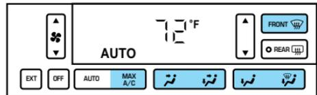
The air conditioning compressor can operate in all modes except
