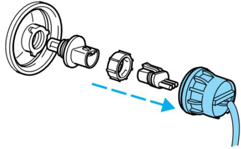
5. Disconnect the electrical connector from the bulb by pulling rearward.
