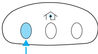
The 2nd or 3rd press from step 3 will activate the door. The HomeLink® Universal Transceiver has now been trained to the receiver. The remaining two buttons may now be programmed if this has not previously been done.
