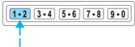
3. Press and hold 1/2 for two seconds. All of the vehicle doors will lock and then unlock to confirm erasure.
