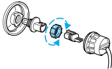
7. Remove the old bulb from the lamp assembly by pulling it straight out of the lamp assembly.
