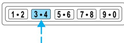
To release the trunk, enter the factory-set code or personal code (driver door unlocks) and press 5/6 within five seconds.
