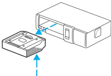
1. Pull the lever to remove a CD tray from the magazine.
