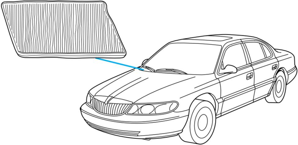
The cabin air filter restricts the entry of airborne dust and pollen particles. The filter is located just in front of the windshield under the cowl vent screen on the passenger side of the vehicle.
