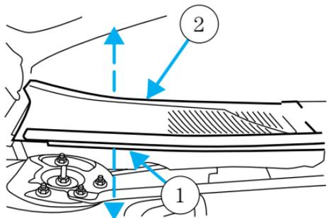
4. Remove the water shield (number 3 in figure) by disengaging the two water shield locking tabs (number 4 in figure), then sliding the water shield toward the front of the vehicle. After the locking tabs are disengaged from the water shield, lift the water shield up and away from the vehicle.
