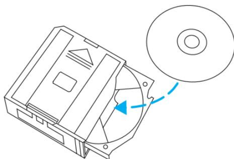
3. Insert each CD tray, with the disc loaded, all the way into the CD magazine.
