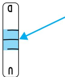
When the horizontal and vertical indicators are set to the “0” mark, the headlamp has been properly aimed.
