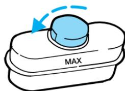
4. Use only brake fluids certified to meet Ford specifications. Refer to *Lubricant specifications* in the *Capacities and specifications* chapter. DOT 3 fluid is recommended. However, if DOT 3 is not available, DOT 4 fluid can be used.
