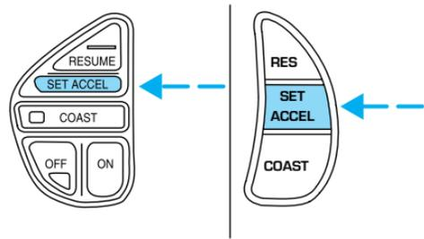
When the SET ACCEL control is pressed and released, the message “SPEED CONTROL SET” will appear for 5 seconds in your message center.
