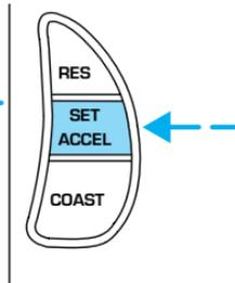
When the SET ACCEL control is pressed, the message “SPEED CONTROL SET” will appear for 5 seconds in your message center.
