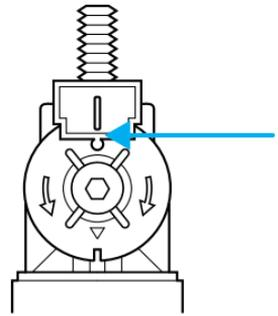
Turning the horizontal adjusting screw in the direction of the arrow changes the horizontal aim as shown.
