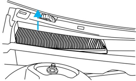
Be careful when installing the new filter. Avoid bending or tearing the filter and make sure it is fully seated in its mounting location after installation.
