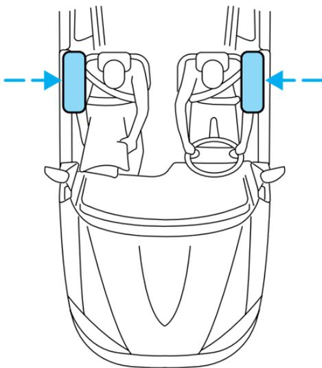
Side air bags, in combination with seat belts, can help reduce the risk of severe injuries in the event of a significant side impact collision.
