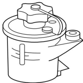
5. If the fluid is low, add fluid in small amounts, continuously checking the level until it reaches the range between the MIN and MAX lines. Be sure to put the cap back on the reservoir.
