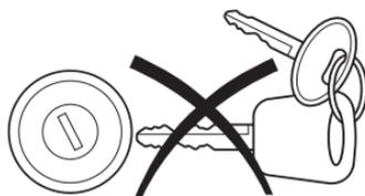
and devices cannot damage the **coded key** ignition key, but can cause a momentary issue if they are too close to the key during engine start. If a problem occurs, turn ignition OFF and restart the engine with all other objects on the key ring held away from the ignition key. Check to make sure the **coded key** ignition key is an approved Ford **coded key** ignition key.
