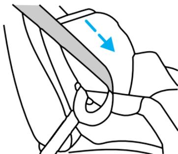
6. Allow the belt to retract. The belt will click as it retracts to indicate it is in the automatic locking mode.
