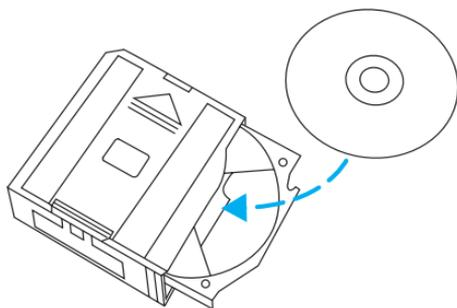
5. Insert each CD tray, with the disc loaded, all the way into the CD magazine.
