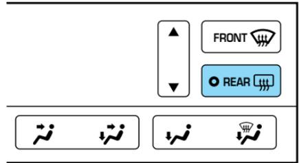
The ignition must be in the ON position to operate the rear window defroster.
