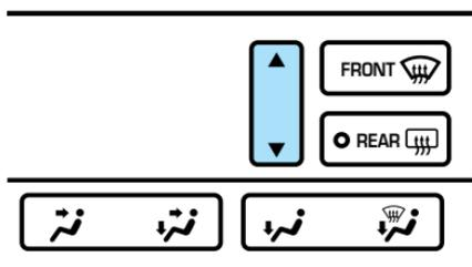
For continuous maximum heating, push the temperature control until 32°C (90°F) is shown in the display window. The EATC will continue maximum heating (disregarding the displayed temperature) until a cooler temperature is selected by pressing the temperature control.
