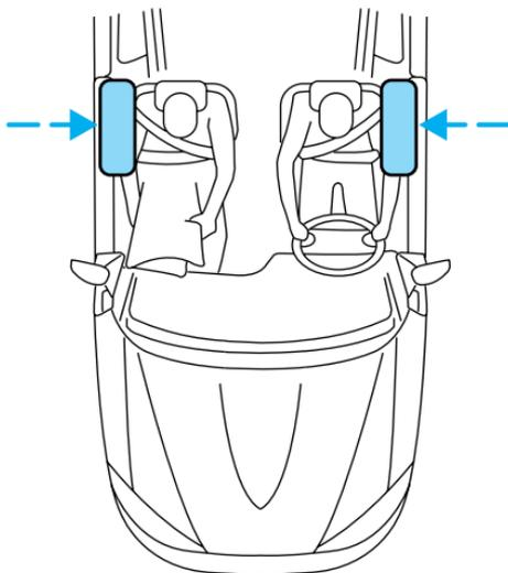
Side air bags, in combination with seat belts, can help reduce the risk of severe injuries in the event of a significant side impact collision.
