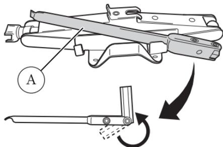
5. Locate pry off notch (if equipped) and remove the center ornament from the aluminum wheel with the tapered end of the wheel nut wrench that came with your vehicle. Insert and twist the handle, then pry against the wheel.
