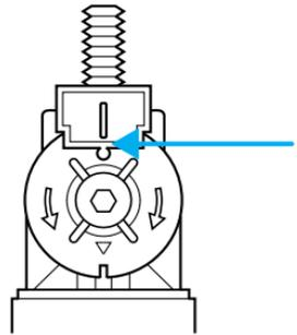
Turning the horizontal adjusting screw in the direction of the arrow changes the horizontal aim as shown.
