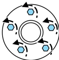
6. Loosen each wheel lug nut one-half turn counterclockwise but do not remove them until the wheel is raised off the ground.
