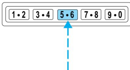
After the factory-set code or personal code has been entered, you can unlock all doors (press 3/4) and release the trunk (press 5/6) as long as the controls are pressed within five seconds of each other.
