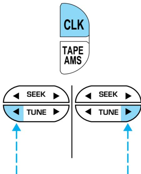
The CLK control will allow you to switch between media display mode (radio station, stereo information, etc.) and clock display mode (time). When in clock mode, the media information will display for 10 seconds, when the radio is turned on, and then revert to clock information. Any time that the media is changed, (new radio station, etc.), the media information will again display for 10 seconds before reverting back to the clock. In media mode, the media information will always be displayed.
