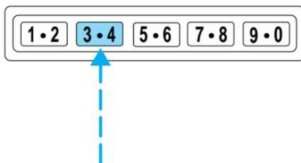
To release the trunk, enter the factory-set code or personal code (driver door unlocks) and press 5/6 within five seconds.
