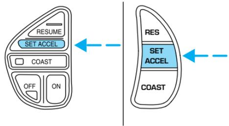
You can accelerate with the accelerator pedal at any time during speed control usage. Releasing the accelerator pedal will return your vehicle to the previously programmed set speed.
