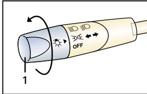
**Turn signal/lighting control lever****OFF** = Lights off
