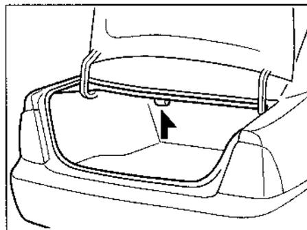
The trunk light is on when the lid is open and off when it's closed.
