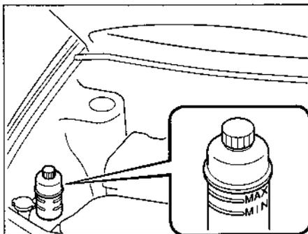
**■ Inspecting Power Steering Fluid Level**
