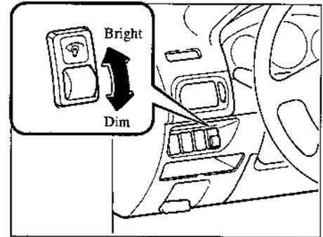
When the parking lights or headlights are on, rotate the thumb-wheel to adjust the brightness of the dashboard lights.
