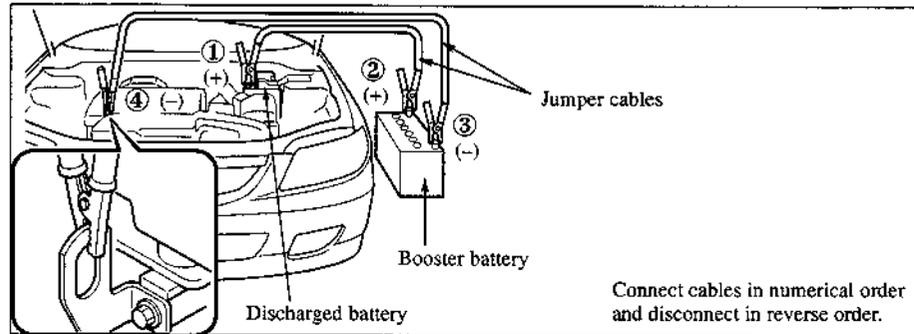
1. Make sure the booster battery is 12 V and that its negative terminal is grounded.
