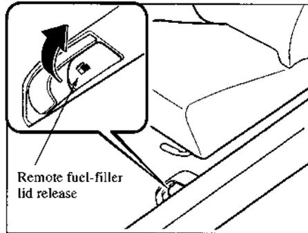
To open, pull up the remote fuel-filler lid release.
