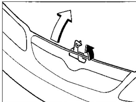
2. Pull the safety catch up and lift the hood.
