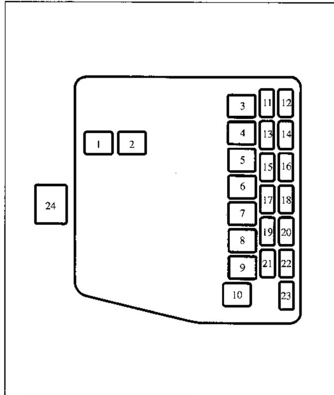
▼ Fuse block (Engine compartment)
