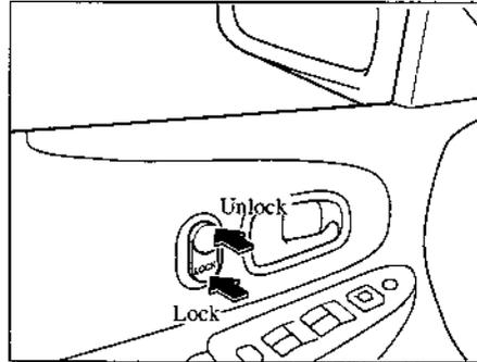
**▼ Locking, unlocking with door-lock switch**
