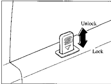
■ **Locking, Unlocking with Door-Lock Button**
