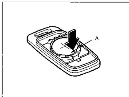
2. Press the portion of the battery indicated by A and remove the battery.
