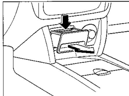
To remove, open and push down on the lock spring.
