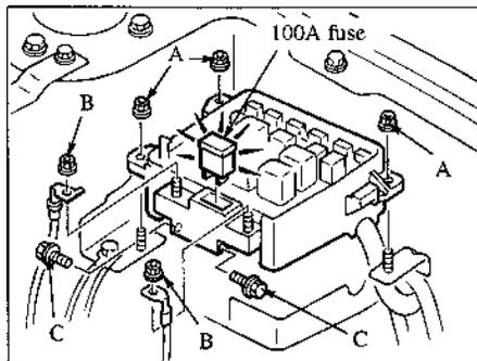
When replacing the 100A fuse:
