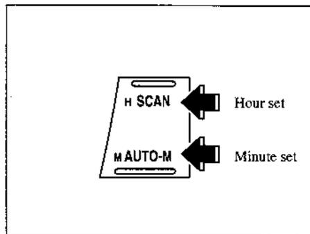
3. To advance the hours, press the hour set button ( H ) to advance the minutes, press the minute set button ( M ) while the time is flashing.
