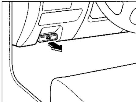
1. With the vehicle parked, pull the release handle to unlock the hood.
