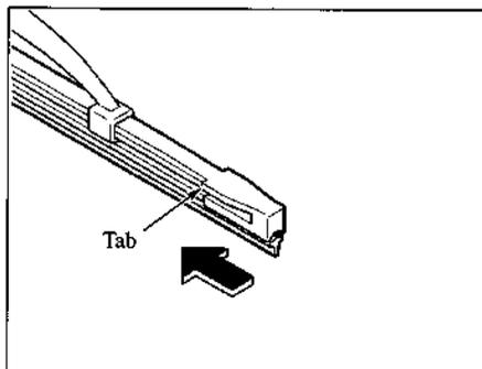
5. Carefully insert the new blade rubber. Then install the blade assembly in the reverse order of removal.
