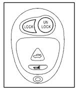
Press UNLOCK once to unlock the driver's door and to turn the interior lamps on (see "Illumination on Remote Activation" in the Index for more details).
