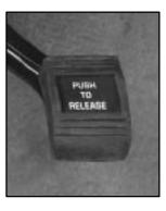
The parking brake is located to the left of the brake pedal near the driver's door.
