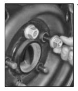
7 Reinstall the wheel nuts with the rounded end of the nuts toward the wheel. Tighten each nut by hand until the wheel is held against the hub.
