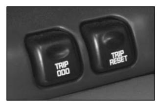
Your trip odometer (trip mode) tells you how far you have driven since you last reset it. To set it to zero, press and hold the TRIP RESET button on the left side of the instrument panel for two to three seconds.
