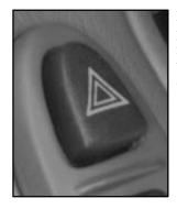
Press the switch located on your instrument panel to make your front and rear turn signal lamps flash on and off.
