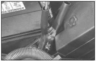
9. Now connect the black negative (-) cable to the good battery's negative (-) terminal. Don't let the other end touch anything until the next step. The other end of the negative cable *doesn't* go to the dead battery.
