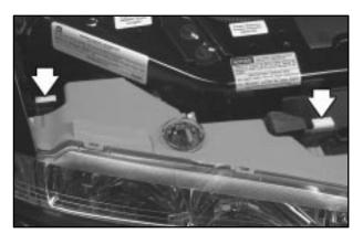
2. Pull straight up on the two headlamp retainers to release the assembly locator tabs and take the retainers off. At the same time, hold the headlamp assembly in position by applying a little pressure against the headlamp lens. This prevents the lamp from falling out.
