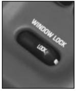
The driver's window controls also include a lock-out switch. Press LOCK to stop front and rear passengers from using their window switches.
