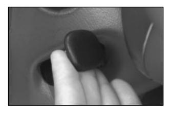
A tilt wheel allows you to adjust the steering wheel before you drive. You can also raise it to the highest level to give your legs more room when you exit and enter the vehicle.
