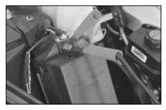
7. Connect the red positive (+) cable to the positive (+) terminal of the vehicle with the dead battery. Use a remote positive (+) terminal if the vehicle has one.
