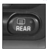
The rear window defogger uses a warming grid to remove fog from the rear window. Press the button to turn the defogger on. It will turn itself off after about 15 minutes (automatic control) or 10 minutes (manual control).
