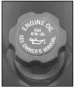
The engine oil fill cap is located toward the front of the engine compartment near the yellow looped engine oil dipstick. See "Engine Compartment Overview" in the Index for more information on location.
