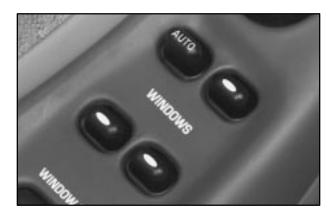
Switches located on the driver's door armrest operate each of the windows when the ignition is on. In addition, each passenger door has an individual window switch.
