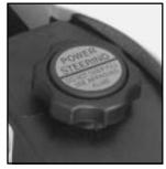
The power steering fluid reservoir is toward the middle of the engine compartment, on the passenger's side.
