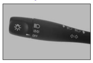
The lamp controls are located on the multifunction lever on the left of the steering wheel. They control the following systems:
