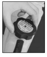
. You can remove the coolant surge tank pressure cap when the cooling system, including the coolant surge tank pressure cap and upper radiator hose, is no longer hot.
