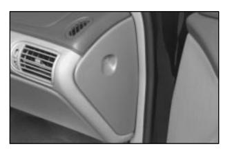
These fuses are located in a fuse block on the passenger's side of the instrument panel. Pull off the passenger's side cover to expose the fuses.
