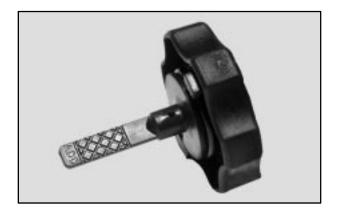
The level should be at the tre cross-hatched area. If necessary, add only enough fluid to bring the level up to the mark.
