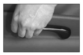
The levers for the driver's and the passenger's front seatbacks are located on the outboard side of each seat cushion. Lift the lever to release the seatback, then move the seatback to where you want it. Release the lever to lock the seatback in place. Pull up on the lever without pushing on the seatback and the seatback will move forward.
