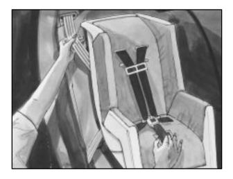
If your vehicle has the child restraint locking feature on the shoulder belt retractor, pull the rest of the shoulder belt all the way out of the retractor to set the lock. To tighten the belt, feed the shoulder belt back into the retractor while you push down on the child restraint. If you're using a forward-facing child restraint, you may find it helpful to use your knee to push down on the child restraint as you tighten the belt.
