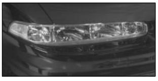
Your vehicle has a headlamp system equipped with horizontal and vertical aim indicators. The aim has been pre-set at the factory and should need no further adjustment. This is true even though your vertical and horizontal aim indicators may not fall exactly on the "0" (zero) marks on their scales.
