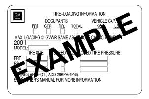
Two labels on your vehicle show how much weight it may properly carry. The Tire-Loading Information label is inside the trunk lid. The label tells you the proper size, speed rating and recommended inflation pressures for the tires on your vehicle. It also gives you important information about the number of people that can be in your vehicle and the total weight you can carry. This includes the weight of all occupants, cargo and all nonfactory-installed options.
