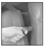
To fold down the rear seatback, pull the seat tab latch forward or pull the remote release straps in the trunk.
