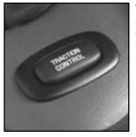
To turn the system on or off, press the TRACTION CONTROL button on the console.
