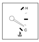
You have a gage that shows the engine coolant temperature. If the gage moves into the shaded area near the hot mark, your engine is too hot.
