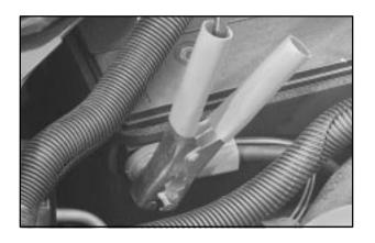
8. Don't let the other end touch metal. Connect it to the positive (+) terminal of the good battery. Use a remote positive (+) terminal if the vehicle has one.
