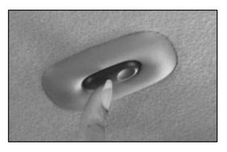
The sunroof includes a sliding glass panel and a sunshade. The switch works only when the ignition or retained accessory power (RAP) is active. See "Retained Accessory Power (RAP)" in the Index.
