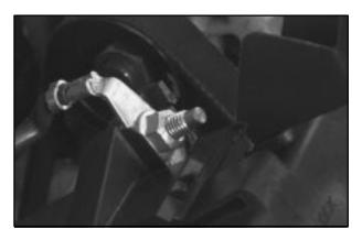
Before you connect the cables, here are some basic things you should know. Positive (+) will go to positive (+) and negative (-) will go to a heavy, unpainted metal engine part. Don't connect positive (+) to negative (-), or you'll get a short that would damage the battery and maybe other parts, too. Don't connect negative (-) to negative (-) on the dead battery, either, as this can cause sparks.
