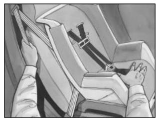
If your vehicle has the child restraint locking feature on the shoulder belt retractor, pull the rest of the shoulder belt all the way out of the retractor to set the lock. To tighten the belt, feed the shoulder belt back into the retractor while you push down on the child restraint. You may find it helpful to use your knee to push down on the child restraint as you tighten the belt.
