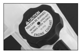
The coolant surge tank is located in the engine compartment toward the rear of the engine on the passengers' side of the vehicle. See "Engine Compartment Overview" in the Index for more information on location.
