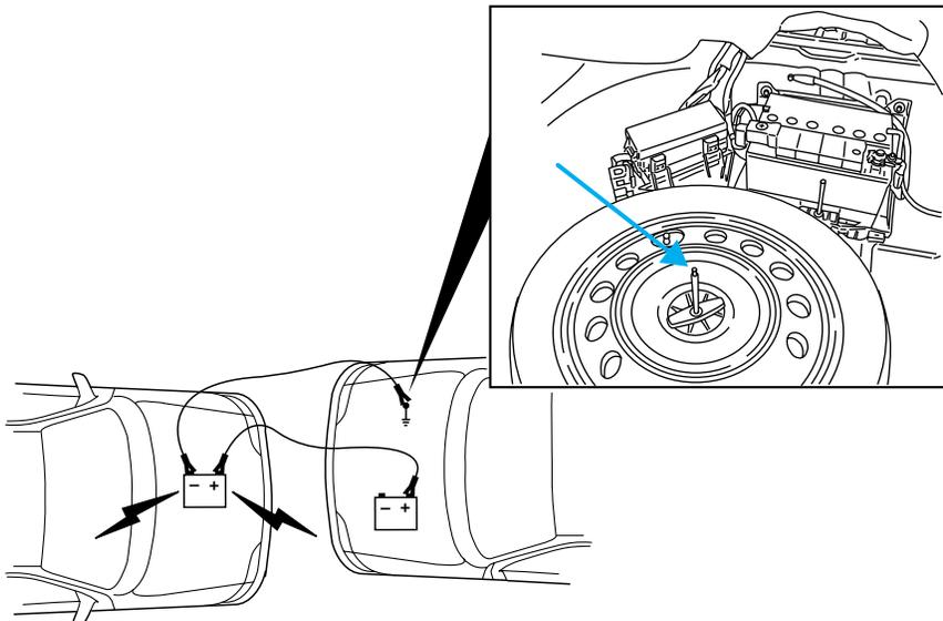
4. Make the final connection of the negative (-) cable to the spare tire tie-down stud. (Your vehicle may be equipped with a plastic cap on top of the tire tie-down stud. This cap must be removed prior to attaching the cable to the stud.)
