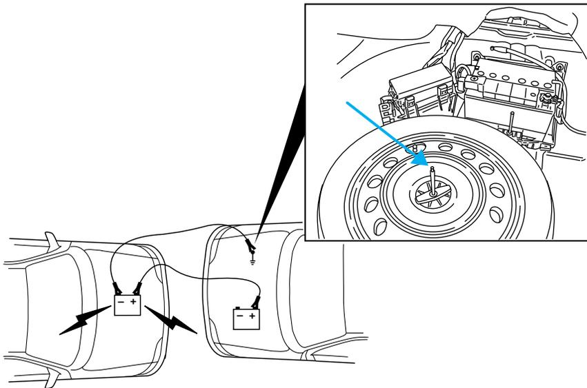
**Remove the jumper cables in the reverse order that they were connected.**
