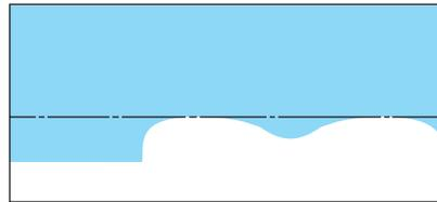
5. Locate the vertical adjuster on each headlamp, then use a 6 mm allen wrench or screwdriver to adjust the headlamp up or down.
