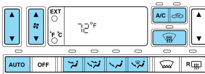
Press AUTO, any of the override controls, the fan speed control, or the driver temperature selection control to turn the DATC system on in the single zone control. While in single zone control the driver and passenger set temperatures are equalized, and only the driver's set temperature is displayed. The DATC system will only operate when the ignition is in the RUN position.
