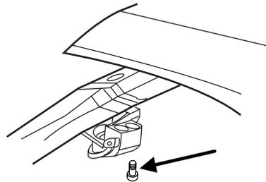
8. Turn and lock the levers fully forward. The levers are locked when you feel the spring engage and the levers are pointing toward the front of the vehicle.
