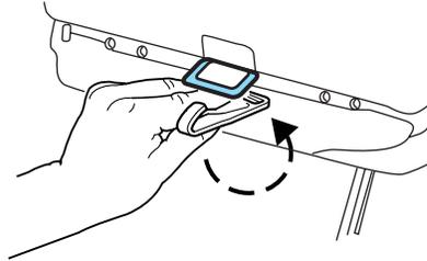
6. Clip the tether strap to the anchor on the seat frame.
