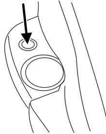
4. Push the convertible top ▲ switch, holding it until the top unfolds and moves forward toward the windshield header.
