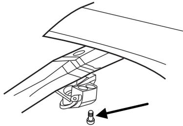
3. Push the two screws down into the windscreen panel of your vehicle.
