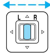
2. Move the control in the direction you wish to tilt the mirror.
