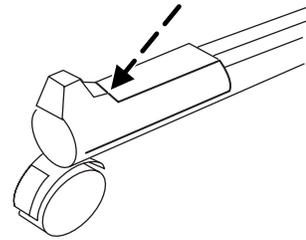
9. Buckle and tighten the retaining strap and unlock the cart wheels before moving the top and cart.
