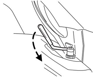
7. Using the mounting key, loosely screw in the two screws at the front of the top by two or three turns. The two screws are already located in the windscreen panel of your vehicle.
