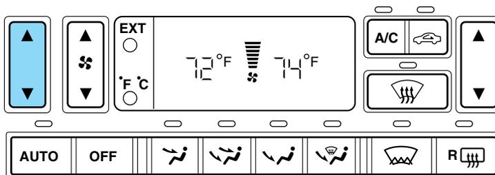
The display window indicates the selected temperature and manual control of fan speed (
