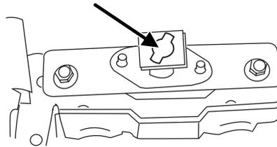
3. Lower the rear of the top into position so that the pins are placed into the bracket receivers.
