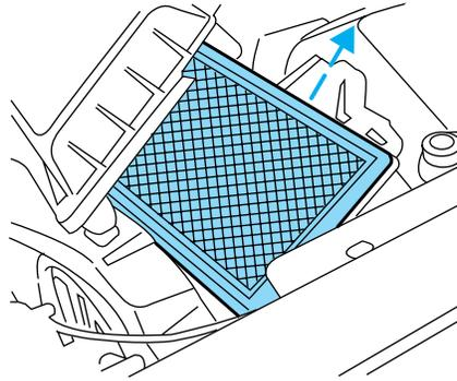
4. Wipe the air filter housing and cover clean to remove any dirt or debris and to ensure good sealing.
