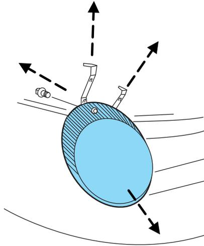
4. Rotate bulb socket counterclockwise and remove from lamp assembly.
