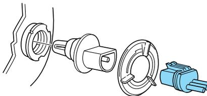
5. Remove the bulb retaining ring by rotating it counterclockwise (when viewed from the rear) to free it from the bulb socket, and slide the ring off the plastic base. Keep the ring to retain the new bulb.
