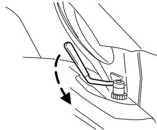
9. Using the mounting key, finish tightening the screws at the front of the removable top all the way so that they are secure.
