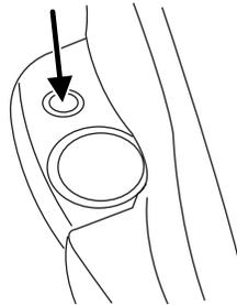
4. Undo the locking levers at the rear right and left sides of the vehicle. Rotate the levers rearward while applying a slight upward force to the top.
