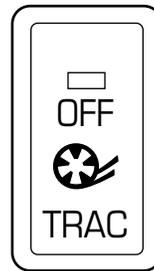
If the Traction Control<sup>™</sup> system is cycled excessively, the brake portion of the system will shut down to prevent the rear brakes from overheating. A limited Traction Control<sup>™</sup> function using only engine torque reduction will still help control wheels from over-spinning. When the rear brakes have cooled down, the system will again function normally. Anti-lock braking is not affected by this condition and will function normally during the cool down period.
