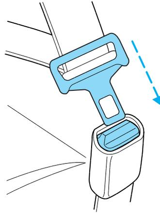
5. To put the retractor in the automatic locking mode, grasp the shoulder portion of the belt and pull downward until all of the belt is extracted and a click is heard.
