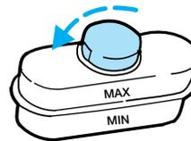
4. Use only brake fluids certified to meet Ford specification ESA-M6C25-A. Refer to *Lubricant specifications* in this chapter. DOT 3 fluid is recommended. However, if DOT 3 is not available, DOT 4 fluid can be used.
