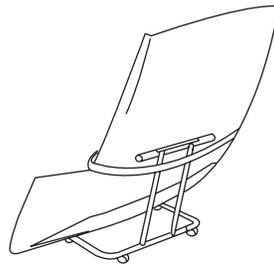
To unlock the wheels, pull up on the lower portion of the plastic tab located on the tip of each wheel.
