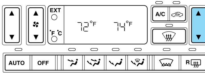
Press the passenger temperature control to turn the DATC system on in dual zone control. While in dual zone control, independent temperatures are maintained for both the driver and passenger, and both set temperatures are displayed.
