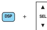
Use the SEL control to select the desired signal mode (the selected mode will appear in the display). The following signal modes can be selected:
