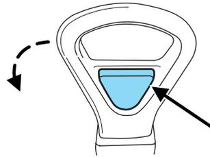
4. Push the convertible top ▼ switch on the instrument panel and hold until the top is completely stored in the stowage compartment.
