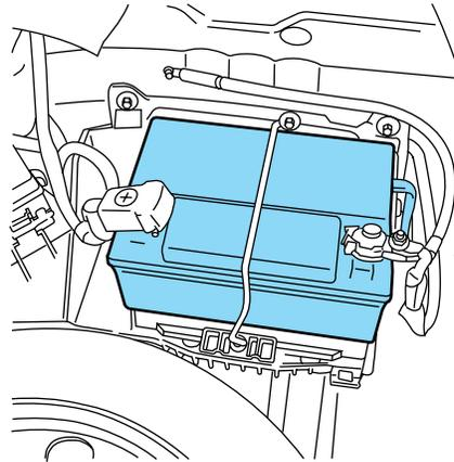
Your battery is designed to purge any battery gases to the outside of the vehicle by means of a vent hose. This vent hose **MUST** be attached at all times. Replacement batteries must be of the same vented design.
