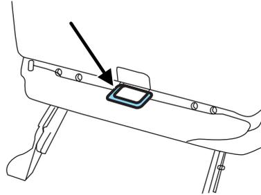
3. Route the child safety seat tether strap under the head restraint and over the back of the seat.
