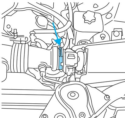
2. Release the two clamps that secure the cover to the air filter housing and place the cover aside.
