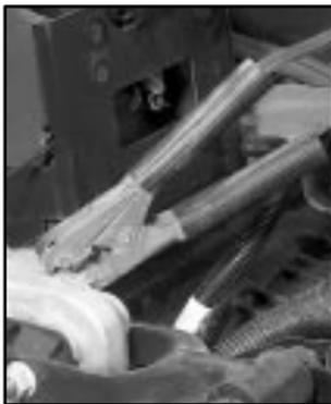
9. Connect the other end of the negative (-) cable at least 18 inches (45 cm) away from the dead battery, but not near engine parts that move. The electrical connection is just as good there, and the chance of sparks getting back to the battery is much less.
