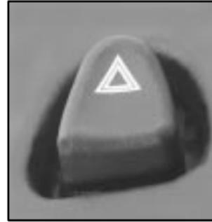
The hazard warning flasher button is located on top of the steering column.
