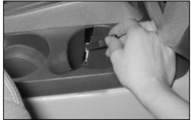
4. Press the shift lock release lever in with the access panel cover.
