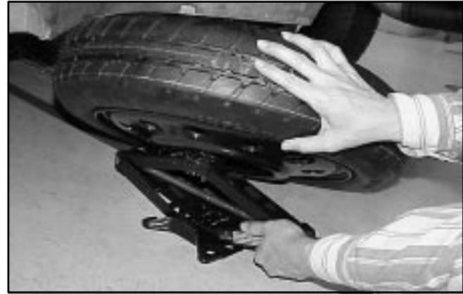
7. Disconnect the wrench from the jack and carefully remove the jack. Use one hand to push against the spare while firmly pulling the jack out from under the spare tire with the other hand.
