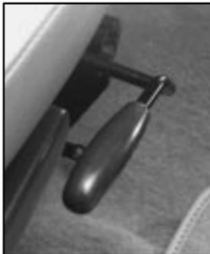
To move the seat, pull the lever located on the front of the seat up to unlock it.
