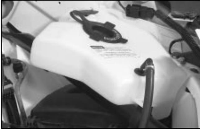
The engine coolant reservoir is located in the engine compartment on the driver's side of the vehicle. See "Engine Compartment Overview" in the Index for more information on location.
