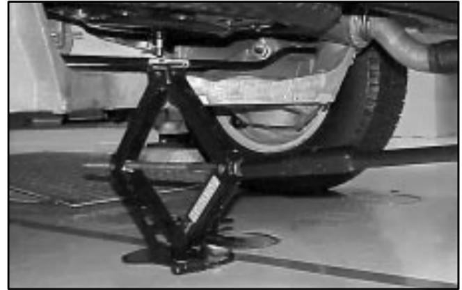
4. Turn the folding wrench clockwise to raise the jack until it lifts the secondary latch spring.
