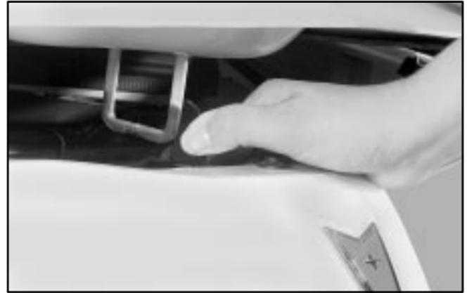
2. Go to the front of the vehicle and slide the secondary hood release from left to right.
