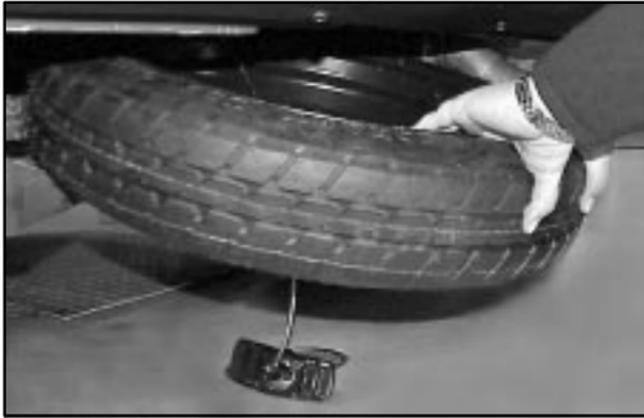
7. Grasp the spare tire with both hands and pull it out from under the vehicle.
