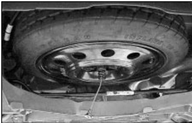
If the spare tire will not lower, the secondary latch may be engaged and causing the tire not to lower. Do the following to check the cable:
