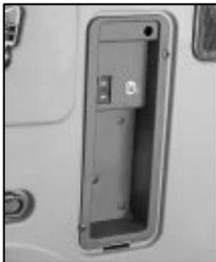
The air inflator is located in the rear compartment on the driver's side. To remove the cover, pull the tab on the cover and pull it off.
