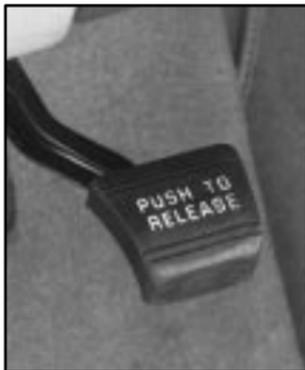
To set the parking brake, hold the regular brake pedal down with your right foot and push down on the parking brake pedal with your left foot.
