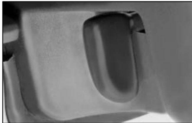
The lever that allows you to tilt the steering wheel is located on the left side of the steering column.
