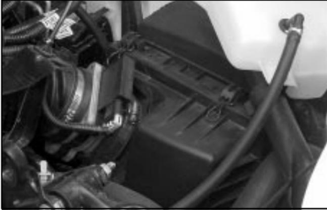
The engine air cleaner/filter is located at the front of the engine compartment on the driver's side of the vehicle, under the engine coolant reservoir.
