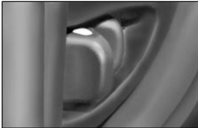
To lock any door from the inside, press the manual locking lever forward. To unlock any door from the inside, pull back on the manual locking lever.
