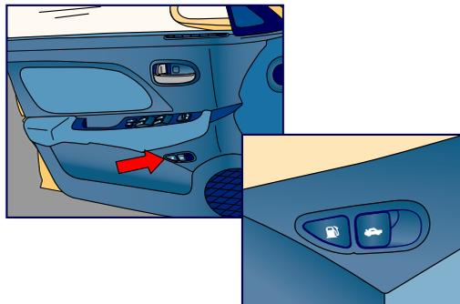
The trunk / fuel door releases are located on the driver's door as shown.
