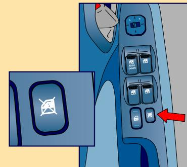
Press the lock switch to deactivate the passenger power window switches.
