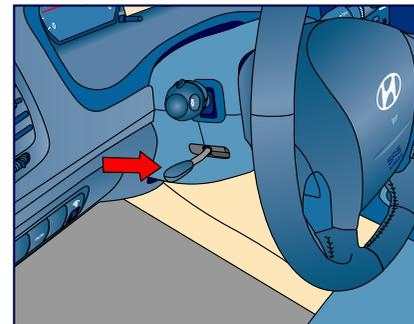
Pull and hold lever while adjusting steering wheel tilt, and then release the lever.
