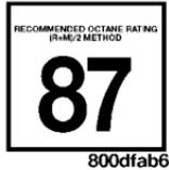
The 2.7L engine is designed to meet all emissions regulations and provide excellent fuel economy and performance when using high quality unleaded “regular” gasoline having an octane rating of 87. The use of premium gasoline is not recommended. Under normal conditions, the use of premium gasoline will not provide a benefit over high quality regular gasolines, and in some circumstances may result in poorer performance.
