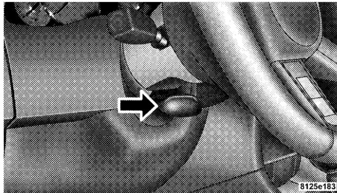
To unlock the steering column, pull the control handle outward. To tilt the steering column, move the steering wheel upward or downward as desired. To lengthen or shorten the steering column, pull the steering wheel outward or push it inward as desired. To lock the steering column in position, push the control handle inward until fully engaged.
