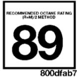
The 3.5L & 5.7L engine is designed to meet all emissions regulations and provide satisfactory fuel economy and performance when using high quality unleaded gasoline having an octane range of 87 to 89. The
