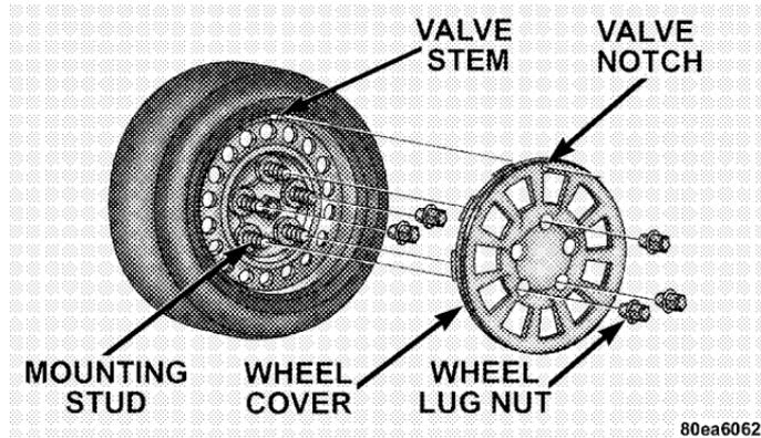
2. Install two lug nuts on the mounting studs, which are on each side of the stud that is in alignment with the valve stem. Install the lug nuts with the cone shaped end of the nut toward the wheel. Lightly tighten the lug nuts.
