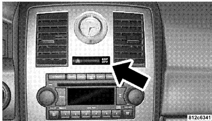
**NOTE:** To improve the vehicle's traction when driving with snow chains, or starting off in deep snow, sand, or gravel, switch off the ESP by pressing the ESP OFF button.
