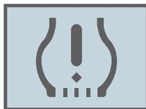
**TPMS MALFUNCTION INDICATOR:** Illuminates and stays illuminated when there is a malfunction with the TPMS system. Have the system checked by an authorized Hyundai dealer as soon as possible.
