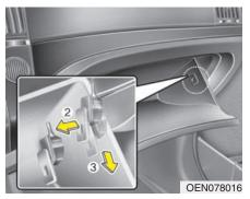
2. With the glove box open, remove the stoppers on both sides to allow the glove box to hang freely on the hinges.
