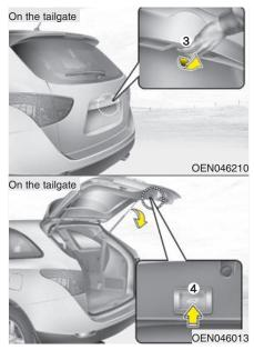
The power tailgate can be opened and closed automatically with the transmitter (or smart key), the main control button on the driver side crash pad, or the sub control button or handle switch on the tailgate.
