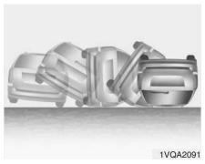
Air bags may not inflate in rollover accidents because air bag deployment would not provide protection to the occupants.
