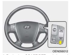
Push the COAST/SET switch, and release it at the desired speed. The SET indicator light in the instrument cluster will illuminate. Release the accelerator at the same time. The desired speed will automatically be maintained.
