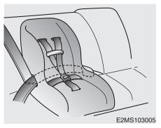
C030102AUN-EU Placing a passenger seat belt into the auto lock mode
