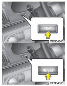
Tripmeter A or B can be selected by pressing the TRIP button for less than 1 second.
