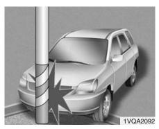
Air bags may not inflate if the vehicle collides with objects such as utility poles or trees, where the point of impact is concentrated to one area and the full force of the impact is not delivered to the sensors. C041100AEN
