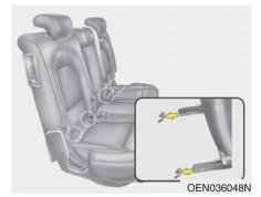
LATCH anchors have been provided in vour vehicle. The LATCH anchors are located in the left and right outboard rear seating positions. Their locations are shown in the illustration. There is no LATCH anchor provided for the center rear seating position.
