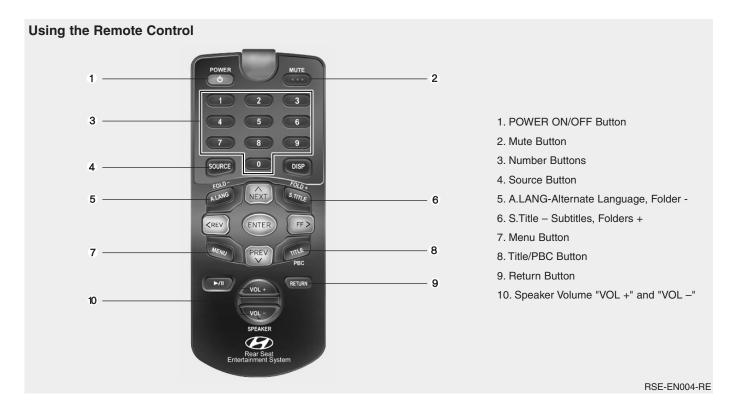
In addition to buttons and functions available from the RSE control panel, the remote control has several additional buttons and operation control functions. The remote control is an infrared device and should be pointed at the RSE monitor for best results.
