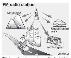
FM broadcasts are transmitted at high frequencies and do not bend to follow the earth's surface. Because of this, FM broadcasts generally begin to fade at short distances from the station. Also, FM signals are easily affected by buildings, mountains, or other obstructions. These can result in certain listening conditions which might lead you to believe a problem exists with your radio. The following conditions are normal and do not indicate radio trouble:
