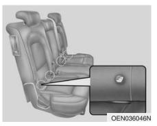
There is a child restraint symbol located on the lower portion of each side of the rear seatbacks. These symbols indicate the position of the lower anchors for child restraints so equipped.
