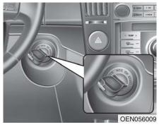
If the battery is weak or the smart key does not work correctly, you can start the engine by inserting the smart key in the ignition switch.
