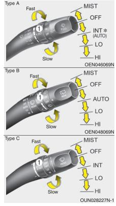
Operates as follows when the ignition switch is turned ON.
