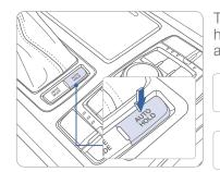
The Auto Hold feature assists in steep hill areas. It holds the brake until the accelerator pedal is pressed.
