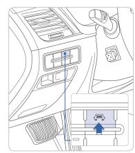
The Lane Keeping Assist System detects lane markers on the road, and assists the driver's steering to help keep the vehicle between lanes.
