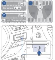
The BSD (Blind spot detection) system uses a radar sensor to alert the driver while driving. It senses the rear side territory of the vehicle and provides information to the driver.
