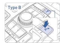
The parking assist system assists the driver during movement of the vehicle by chiming if any object is sensed within the distance of 39.5 inches in front and 47.2 inches in behind the vehicle.
