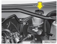
If the level is low, add fluid to the MAX level. The level will fall with accumulated mileage. This is a normal condition associated with the wear of the brake linings. If the fluid level is excessively low, have the brake system checked by an authorized HYUNDAI dealer.
