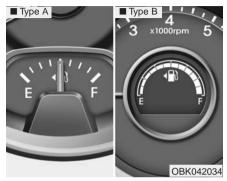
On inclines or curves, the fuel gauge pointer may fluctuate or the low fuel warning light may come on earlier than usual due to the movement of fuel in the tank.
