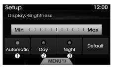
Use the **O** TUNE knob to adjust the screen brightness or set the Brightness on Automatic, Daylight, or Night mode.
