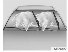
Contamination of either the windshield or the wiper blades with foreign matter can reduce the effectiveness of the windshield wipers. Common sources of contamination are insects, tree sap, and hot wax treatments used by some commercial car washes. If the blades are not wiping properly, clean both the window and the blades with a good cleaner or mild detergent, and rinse thoroughly with clean water.
