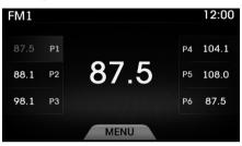
After selecting the frequency Press and hold the desired preset ~ 6 key.
