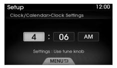
Use the TUNE knob to select the Hour, Minutes and AM/PM setting and use TUNE knob to change settings.
