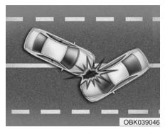
In an angular collision, the force of impact may direct the occupants in a direction where the air bags would not provide additional occupant protection, and thus the sensors may not deploy any air bags.
