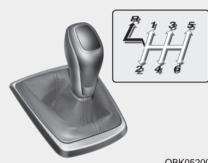
The gearshift lever must be returned to the neutral position before shifting into R (Reverse).
