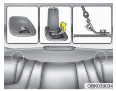
Securing a child restraint seat with "Tether Anchor" system Child restraint hook holders are located on the package tray.
