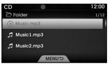
Turn the O TUNE knob to search for the desired file and press the O TUNE knob to select.
