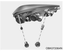
*Turn signal light and side marker bulb replacement*
