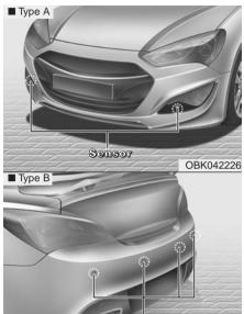
The parking assist system assists the driver during movement of the vehicle by chiming if any object is sensed within the distance of 24 in. (60 cm) in front and 47 in. (120 cm) behind the vehicle. This system is a supplemental system and it is not intended to nor does it replace the need for extreme care and attention of the driver.
