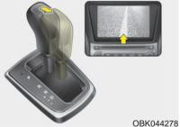
The rear camera display will activate when the back-up light is ON with the ignition switch ON and the shift lever in the R (Reverse) position. This system is a supplemental system that helps the driver by displaying objects behind the vehicle when backing up.
