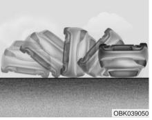
• Side impact and curtain air bags may not inflate in a rollover accident unless the side of the vehicle is struck with sufficient force to cause air bag inflation to occur.
