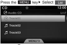
Turn the  $\bigcirc$  TUNE knob to search for the desired track and press the  $\bigcirc$  TUNE knob to select.
