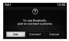
If *Bluetooth*<sup>®</sup> Wireless Technology devices are paired but none are currently connected, pressing the PHONE key or the *c* key on the steering wheel displays the following screen. Press the [Pair] button to pair a new device or press the [Connect] to connect a previously paired device.
