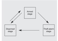
This system is designed to provide protection from unauthorized entry into the car. This system is operated in three stages: the first is the "Armed" stage, the second is the "Theft-alarm" stage, and the third is the "Disarmed" stage. If triggered, the system provides an audible alarm with blinking of the hazard warning lights.
