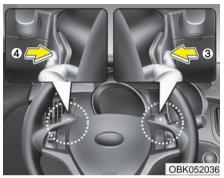
In sport mode, it is possible to shift the gear by using either the shift lever or the steering wheel shift paddles (dynamic shift).
