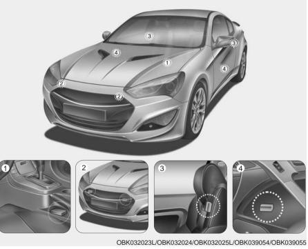
Air bag collision sensors(1) SRS control module(2) Front impact sensor
