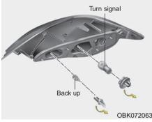
8. Install the socket in the assembly by aligning the tabs on the socket with the slots in the assembly. Push the socket into the assembly and turn the socket clockwise.
