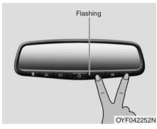
For first-time programming, press and hold the two outside buttons (
