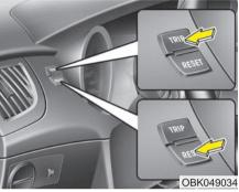
Odometer/Tripmeter (if equipped)
