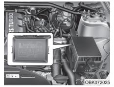
Engine compartment fuse panel
