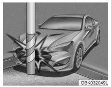
• Air bags may not inflate if the vehicle collides with objects such as a utility pole or tree, where the point of impact is concentrated and the collision energy is absorbed by the vehicle structure.
