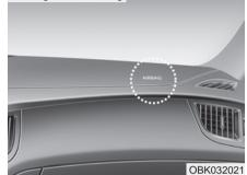
The purpose of the SRS is to provide the vehicle's driver and/or the front passenger with additional protection than that offered by the seat belt system alone in case of a frontal impact of sufficient severity. The SRS uses sensors to gather information about the impact severity. The advanced SRS offers the ability to control the air bag inflation within two levels. A first stage level is provided for moderate-severity impacts. A second stage level is provided for more severe impacts.
