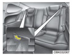
3. Remove the belt webbing from the rear shoulder belt guide and move the rear belt webbing to the outside so it does not interfere with the seatback when folding.
