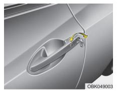
2. Turn the key toward the rear of the vehicle to unlock and toward the front of the vehicle to lock.
