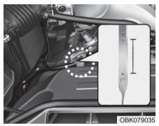
Checking the engine oil level
