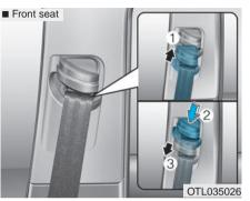
To adjust the height of the seat belt anchor, lower or raise the height adjuster into an appropriate position.
