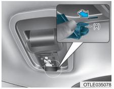
4. Insert the small tongue plate (A) into the slot on the belt assembly pocket located in the headliner.
