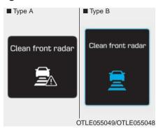
When the sensor lens cover is blocked with dirt, snow, or debris, the AEB system operation may stop temporarily. If this occurs, a warning message will appear on the LCD display. Remove any dirt, snow, or debris and clean the radar sensor lens cover before operating the AEB system.
