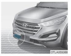
In order for the AEB system to operate properly, always make sure the radar sensor lens cover is clean and free of dirt, snow, and debris. Dirt, snow, or foreign substances on the lens may adversely affect the sensing performance of the radar.
