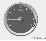
The tachometer indicates the approximate number of engine revolutions per minute (rpm).
