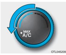
The MAX A/C mode is used to cool the inside of the vehicle faster. Air flow is directed toward the upper body and face.
