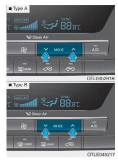
The mode selection button controls the direction of the air flow through the ventilation system. The air flow outlet direction is cycled as follows:
