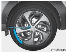
Loosen the wheel lug nuts counterclockwise one turn each in the order shown above, but do not remove any lug nuts until the tire has been raised off of the ground.
