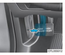
Always set the parking brake before leaving the vehicle. To apply the parking brake:
