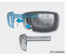
To remove the mechanical key from the smart key fob, press and hold the release button (1) and pull the mechanical key out.
