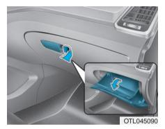
To open the glove box, pull the handle and the glove box will automatically open. Close the glove box after use.
