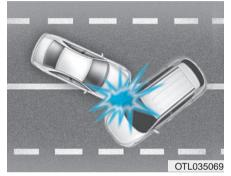
In an angled collision, the force of impact may direct the occupants in a direction where the air bags would not be able to provide any additional benefit, and thus the sensors may not deploy any air bags.
