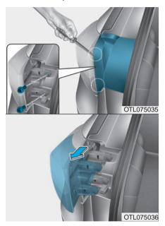
Stop/tail Lamp, Turn signal Lamp and Side marker lamp
