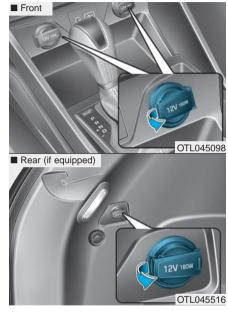
The power outlet is designed to provide power for mobile telephones or other devices designed to operate with vehicle electrical systems. The devices should draw less than 180 W with the engine running.
