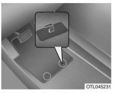
ALWAYS use the Floor Mat Anchors to attach the front floor mats to the vehicle. The anchors on the front floor carpet keep the floor mats from sliding forward.
