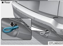
If towing is necessary, we recommend you have it done by an authorized HYUNDAI dealer or a commercial tow truck service. If towing service is not available in an emergency, your vehicle may be temporarily towed using a cable or chain secured to the emergency towing hook at the front (or rear) of the vehicle.
