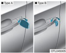
If you lock the driver's door with turning the key toward the front of the vehicle, all vehicle doors will lock. If you unlock the driver's door with turning the key toward the rear of the vehicle, the driver's door will unlock.
