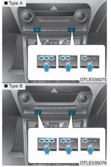
While the engine is running, push either of the switches to warm the driver's seat or front passenger's seat.
