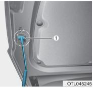
4. Pull out the support rod and hold the hood open with the support rod (1).
