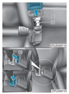
3. Slip the large tongue plate (C) out of the pocket (D) located on the belt assembly. 4. Pull the large tongue plate and insert it into the seat belt buckle (E) located on the left hand (driver) side of the center seat. Insert the buckle until an audible "click" is heard, indicating that the latch is locked. Make sure the belt is not twisted.
