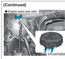
2. Make sure that the tiny protrusions inside the coolant cap should be securely interlocked.
