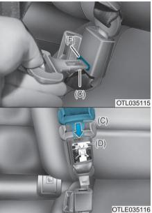
and allow the webbing to retract automatically.3. Slip the large tongue plate (C) into the pocket (D) located on the belt
