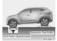
A full-time AWD vehicle should not be tested on a 2WD roll tester. If a 2WD roll tester must be used, perform the following procedure:
