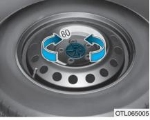
Turn the winged hold down bolt counterclockwise to remove the spare tire.
