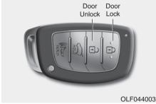
To lock the doors, press the button on the outside door handle while carrying the Smart Key with you or press the Door Lock button on the Smart Key. Press the button on the driver's outside door handle while carrying the Smart Key with you or press the Door Unlock button on the Smart Key, the driver's door will unlock. If you press the button on the front passenger's outside door, all doors will unlock.
