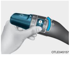
Fog lamps are used to provide improved visibility when visibility is poor due to fog, rain or snow, etc. Use the switch next to the headlamp switch to turn the fog lamps ON and OFF.
