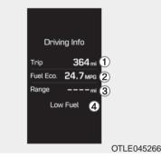
At the end of each driving cycle, the Driving Info message is displayed. This display shows the trip distance, the average fuel economy, and the remaining vehicle range.
