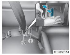
Press the release button on the rear center seat belt buckle (E) located on the left hand (driver) side of the center seat and remove the large tongue plate (C).
