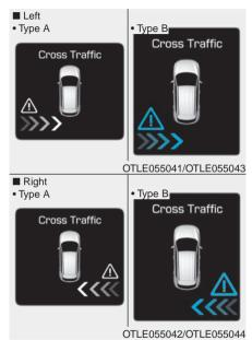
If the vehicle detected by the sensors approaches your vehicle, the warning chime will sound, the warning light on the outer side view mirror will blink and a message will appear on the LCD display.
