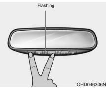
When programming the buttons for the first time, press and hold the left and center buttons (1<sup>⊕</sup>, 1<sup>⊕</sup>) simultaneously for approximately 20 seconds until the indicator light begins to flash. (This procedure erases the factory-set default codes. Do not perform this step to program additional hand-held transmitters.)
