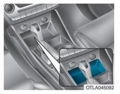
You can use the AUX port to connect audio devices and the USB port to plug in a USB device or iPod<sup>®</sup>.
