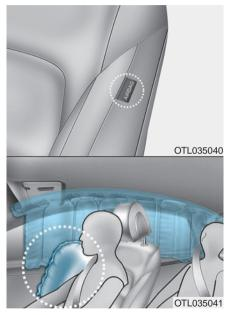
Your vehicle is equipped with a side air bag in each front seat. The purpose of the air bag is to provide the vehicle's driver and the front passenger with additional protection than that offered by the seat belt alone. The side air bags are designed to deploy during certain side impact collisions, depending on the crash severity, angle, speed and point of impact. The side and curtain air bags on both sides of the vehicle may deploy if a rollover or possible rollover is detected.
