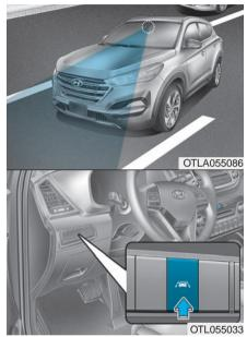
The Lane Departure Warning (LDWS) System feature is designed to monitor the vehicle's position relative to the lane in front of you and detect when the vehicle begins to move out of its lane.
