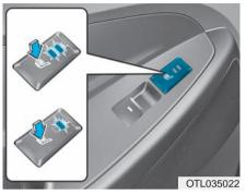
While the engine is running, push either of the switches to warm the rear seat.
