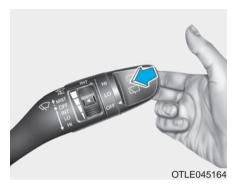
In the OFF position, pull the lever gently toward you to spray washer fluid on the windshield and to run the wipers 1-3 cycles. The spray and wiper operation will continue until you release the lever. If the washer does not work, you may need to add washer fluid to the washer fluid reservoir. If equipped with the Headlamp Washer, washer fluid will be sprayed on the headlamp at the same time you operate the windshield washer when:
