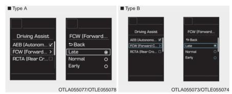
The driver can select the initial warning activation time in the User Settings in the Driver LCD display. The options for the initial Forward Collision Warning include the following:
