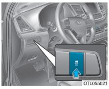
The Electronic Stability Control (ESC) system helps to stabilize the vehicle during cornering maneuvers. ESC checks where you are steering and where the vehicle is actually going. ESC applies braking pressure to any one of the vehicle's brakes and intervenes in the engine management system to assist the driver with keeping the vehicle on the intended path. It is not a substitute for safe driving practices. Always adjust your speed and driving to the road conditions.
