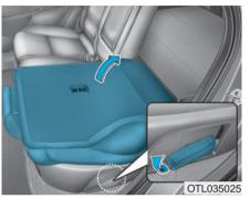
5. To use the rear seat, lift and pull the seatback rearward. Pull the seatback firmly until it clicks into place. Make sure the seatback is locked in place.
