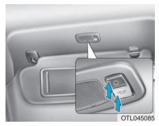
The vanity mirror lamp is located in the headliner just behind the sun visor. Push the switch to turn the vanity light on or off.
