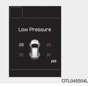
This warning message is displayed if the tire pressure is low. The corresponding tire on the vehicle will be illuminated.
