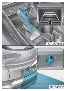
The Rear View Camera will activate when the engine is running and the shift lever is in the R (Reverse) position. This is a supplemental system that provides a view of the area behind the vehicle through the A/V display while the vehicle is in the R (Reverse) position.
