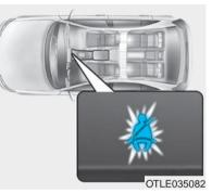
The front passenger's seat belt warning light will activate to the following table when the ignition switch is in "ON" position.
