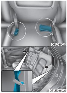
3. Insert the rear seat belt buckle in the pocket between the rear seatback and cushion, and insert the rear seat belt webbing in the guide to prevent the seat belt from being damaged.
