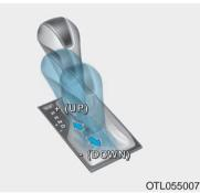
In Manual Shift Mode, moving the shift lever backwards and forwards will allow you to select the desired range of gears for the current driving conditions.
