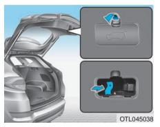
Your vehicle is equipped with the emergency liftgate safety release lever located on the bottom of the liftgate. To unlock and open the liftgate manually from inside the luggage compartment, perform the following steps:
