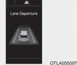
If your vehicle speed exceeds 40 mph (64 km/h) and the LDWS button is ON, the system is enabled. If your vehicle departs from the projected lane in front of you, the LDWS operates as follows:
