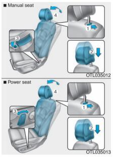
To reinstall the head restraint:
