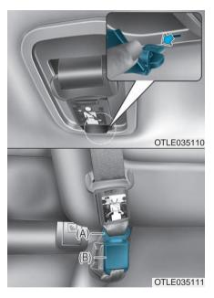
1. Extract the small tongue plate from the slot on the belt assembly pocket located in the headliner. 2. Insert the small tongue plate (A) into the primary buckle (B) located on the right hand (passenger) side of the center seat. Insert the buckle until an audible "click" is heard, indicating that the latch is locked. Make sure the belt is not twisted.
