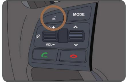
**HELP** provides guidance on commands that can be used within the current function.
