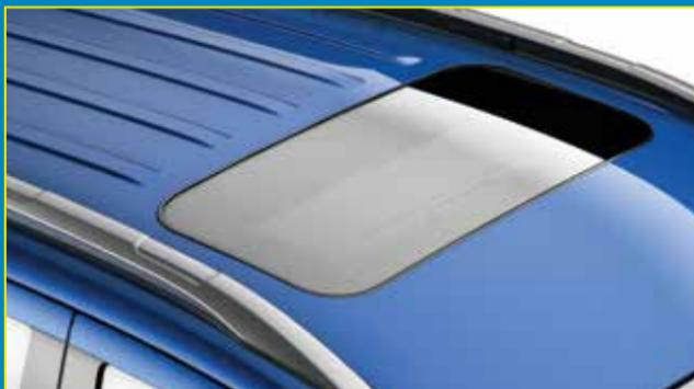
The moonroof has a one-touch open and close feature. To stop it during a one-touch operation, press the control a second time.
