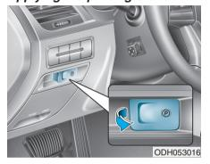
To apply the EPB (Electronic Parking Brake):
