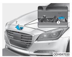
Raise the hood slightly, push the secondary latch up (1) inside of the hood center and lift the hood (2). After it has been raised about halfway, it will raise completely by itself.
