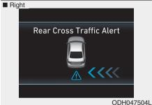
If the vehicle detected by the sensors approaches your vehicle, the warning chime will sound, the warning light on the side view mirror will blink and a message will appear on the LCD display.
