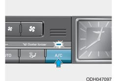
Push the A/C button to turn the air conditioning system on (indicator light will illuminate).
