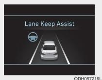
When the conditions below are met. LKAS will be enable to assist steering.
