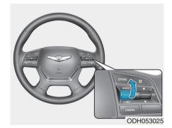
If any method other than the CRUISE toggle switch was used to cancel cruising speed and the system is still activated, the cruising speed will automatically resume when you push the toggle switch up (RES+) or down (SET-).
