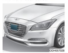
In order for the AEB system to operate properly, always make sure the radar sensor cover is clean and free of dirt, snow, and debris. Dirt, snow, or foreign substances on the lens may adversely affect the sensing performance of the radar.
