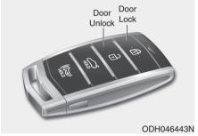
To lock the doors, press the button on the outside door handle while carrying the smart key with you or press the door lock button on the smart key. Press the button on the driver's outside door handle while carrying the smart key with you or press the unlock button on the smart key, the driver's door will unlock. If you press the button on the front passenger's outside door, all doors will unlock.
