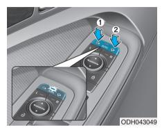
The side view mirror can be folded or unfolded by pressing the switch when:
