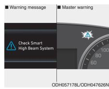
When the Smart High Beam is not working properly, the warning message will come on for a few second. After the message disappears, the master warning light ( ) will illuminate.
