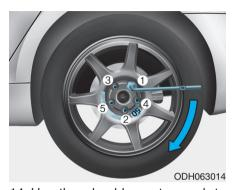
14. Use the wheel lug nut wrench to tighten the lug nuts in the order shown. Double-check each lug nut until they are tight. After changing tires, we recommend that an authorized retailer of Genesis Branded products tighten the lug nuts to their proper torque as soon as possible. The wheel lug nut should be tightened to 79~94 lbf·ft (11~13 kgf·m).
