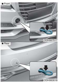
If towing is necessary, we recommend you to have it done by an authorized retailer of Genesis Branded products or a commercial tow truck service. If towing service is not available in an emergency, your vehicle may be temporarily towed using a cable or chain secured to the emergency towing hook at the front (or rear) of the vehicle.
