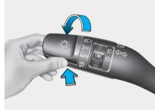
The Smart High Beam is a system that automatically adjusts the headlamp range (switches between high beam and low beam) according to the brightness of other vehicles and
