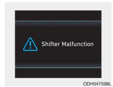
The warning message appears on the LCD display, when the transmission or the shift lever does not properly operate in the P (Park) position. In this case, we recommend you to
