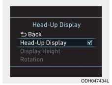
To activate the head up display, select "Head-up Display" on the "User Settings Mode" in the cluster.
