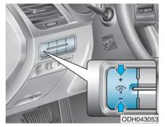
When the Engine Start Stop button is in the ON position, press the illumination control button to adjust the instrument panel illumination intensity and AVN monitor illumination intensity.
