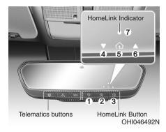
Your vehicle may be equipped with a Gentex Automatic-Dimming Mirror with a Z-Nav™ Electronic Compass Integrated Display an and HomeLink® Wireless Control System. During nighttime driving, this feature will automatically detect and reduce rearview mirror glare while the compass indicates the direction the vehicle is pointed. The HomeLink® Universal Transceiver allows you to activate your garage door(s), electric gate, home lighting, etc.
