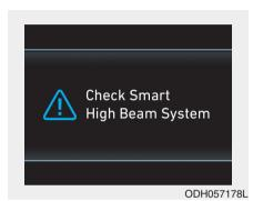
This warning message is displayed if there is a problem with the Smart High Beam System. We recommend you to have the vehicle inspected by an authorized retailer of Genesis Branded products.
