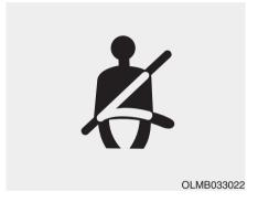
The driver's seat belt warning light and chime will come on according to the following table when the Engine Start/Stop button is in the ON position.
