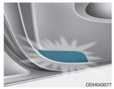
The door courtesy lamp comes ON when the door is opened to assist entering or exiting the vehicle. It also serves as a warning to passing vehicles that the vehicle door is open.
