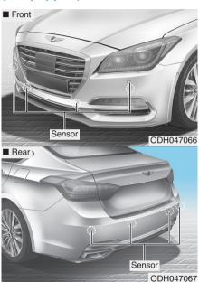
The Parking Assist System assists the driver during movement of the vehicle by chiming if any object is sensed within the distance of 39 inches (100 cm) in front and 47 inches (120 cm) behind the vehicle.
