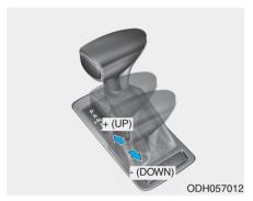
Whether the vehicle is stationary or in motion, manual shift mode is selected by pushing the shift lever from the D (Drive) position into the manual gate. To return to D (Drive) range operation, push the shift lever back into the main gate.
