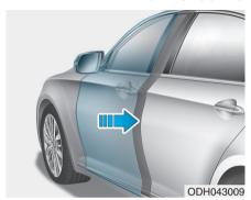
If a door isn't closed completely but is closed to the first detent position, the door will close automatically.
