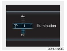
The brightness of the instrument panel illumination is displayed when it is adjusted.
