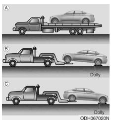
If emergency towing is necessary, we recommend having it done by an authorized retailer of Genesis Branded products or a commercial tow-truck service. Proper lifting and towing procedures are necessary to prevent damage to the vehicle. The use of wheel dollies or flatbed is recommended.
