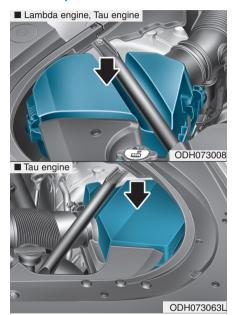
The air cleaner filter can be cleaned for inspection using compressed air. Do not attempt to wash or to rinse it, as water will damage the filter. If soiled, the air cleaner filter must be replaced.
