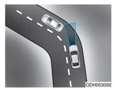
The Smart Cruise Control System may not detect a moving vehicle in your lane, and then your vehicle could accelerate to the set speed. Also, the vehicle speed will decrease when the vehicle ahead is recognized suddenly.
