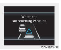
If the vehicle ahead (vehicle speed: less than 20 mph (30km/h)) disappears to the next lane, the warning chime will sound and a message will appear. Adjust your vehicle speed for vehicles or objects that can suddenly appear in front of you by depressing the brake pedal.
