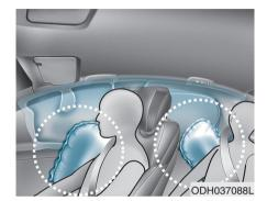
Your vehicle is equipped with a side air bag in each front and outboard rear seat. The purpose of the air bag is to provide the vehicle's driver and/or the front and outboard rear passenger with additional protection than that offered by the seat belt alone.
