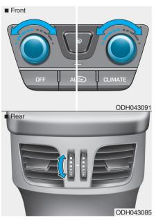
Turn the temperature control knob to set the desired temperature.
