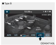
When driving, the auto air conditioner controls CO2 concentration and helps maintain pleasant air in a vehicle.
