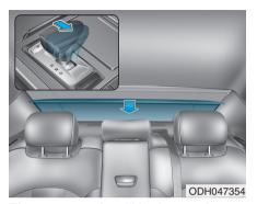
The rear curtain will be lowered automatically when you shift the shift lever into R (Reverse) and raised automatically when you shift the shift lever from R (Reverse) into P (Park). After the rear curtain is lowered by shifting into R (Reverse), if you drive more than 12 mph (20 km/h) with the shift lever in D (Drive), the rear curtain will be raised automatically.
