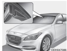
Auto defogging reduces the probability of fogging up the inside of the windshield by automatically sensing the moisture on the inside of the windshield.
