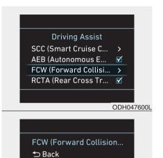
The driver can select the initial warning activation time in the User Settings in the LCD display.
