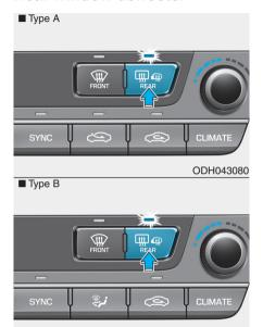
The defroster heats the window to remove frost, fog and thin ice from the interior and exterior of the rear window, while engine is running.
