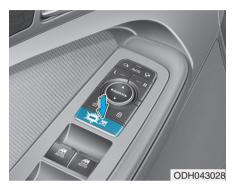
The driver can disable the power window switches on the rear passenger's doors by pressing the power window lock switch. The indicator will be illuminated.
