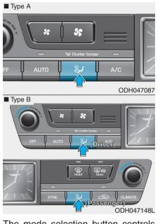
The mode selection button controls the direction of the air flow through the ventilation system.
