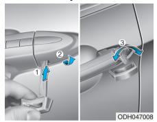
First, remove the cover (1~2), and then turn the key toward the rear of the vehicle to unlock and toward the front of the vehicle to lock (3).
