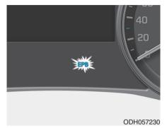
If the EPB Malfunction Indicator remains on, comes on while driving, or does not come on when the Engine Start/Stop button is in the ON position, this indicates the EPB may have malfunctioned. Have your vehicle checked by an authorized retailer of Genesis Branded products as soon as possible.
