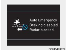
Auto Emergency Braking disabled. Radar blocked
