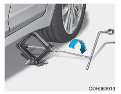
Insert the jack handle into the jack and turn it clockwise, raising the vehicle until the tire clears the ground. Make sure the vehicle is stable on the jack.
