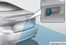
The Rear View Camera will activate when the engine is running and the shift lever is in the R (Reverse) position
