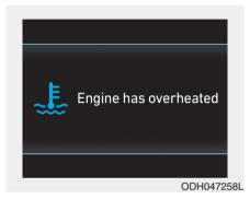
This warning message illuminates when the engine coolant temperature is above 120°C (248°F). This means that the engine is overheated and may be damaged.
