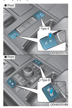
The air ventilation seats are provided to cool the front seats by blowing air through small vent holes on the surface of the seat cushions and seatbacks.
