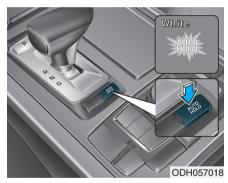
Press the [AUTO HOLD] switch. The AUTO HOLD indicator will illuminate white and the system will be in the standby position.
