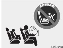
though your vehicle is equipped with the OCS, never install a child restraint in the front passenger's seat. An inflating air bag can forcefully strike a child or child restraint resulting in serious or fatal injury.
