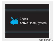
This warning message illuminates if the active hood system has a malfunction
