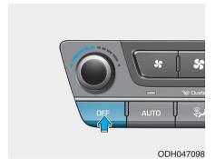
Push the OFF button of the front to turn off the air climate control system. However, you can still operate the mode and air intake buttons as long as the Engine Start/Stop button
