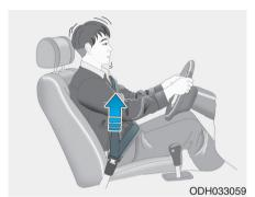
The purpose of the Pre-Active Seat Belt is to tighten the seat belt when a collision is sensed, driving emergency braking, or when a loss of control is sensed.
