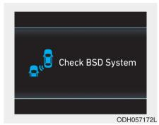
This warning message illuminates if there is a malfunction with the Blind Spot Detection (BSD) system. And the BSD system will be automatically deactivated. We recommend that the vehicle be inspected by an authorized retailer of Genesis Branded products.
