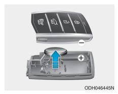
Battery Type: CR2032 To replace the battery:
