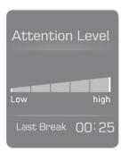
The Driver Attention Alert (DAA) system displays the condition of the driver's fatigue level and inattentive driving practices. The DAA system monitors the lane markers and driver's inputs to the steering wheel, accelerator pedal and brake pedal.
