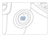
With the ignition OFF and foot OFF of brake pedal, press the Engine Start / Stop button.
