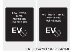
This message is displayed when the temperature of the high-voltage (hybrid) battery is too low or too high. This warning message is to protect the battery and the hybrid system.
