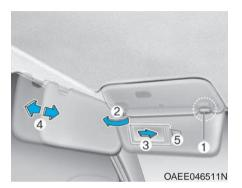
To use a sunvisor, pull it downward. To use a sunvisor for a side window, pull it downward, unsnap it from the bracket (1) and swing it to the side (2). To use the vanity mirror, pull down the sunvisor and slide the mirror cover (3). Adjust the sunvisor forward or backward (4) as needed (if equipped). Use the ticket holder (5) to hold tickets (if
