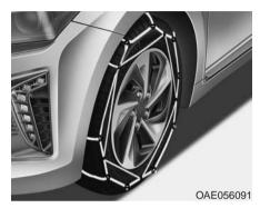
Since the sidewalls of radial tires are thinner than other types of tires, they may be damaged by mounting some types of tire chains on them. Therefore, the use of snow tires is recommended instead of tire chains. If tire chains must be used, use genuine HYUNDAI parts and install the tire chain after reviewing the instructions provided with the tire chains. Damage to your vehicle caused by improper tire chain use is not covered by your vehicle manufacturer's warranty.
