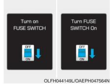
If the fuse switch is OFF, "Turn on FUSE SWITCH" or "Turn FUSE SWTICH On" message will appear.
