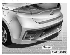
The Rear Parking Assist System assists the driver during reverse movement of the vehicle by chiming if any object is sensed within approximately 50 in (120 cm) behind the vehicle.
