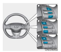
To change the trip mode, toggle the "\land , \subset " switch on the steering wheel.
