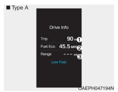
At the end of each driving cycle, the Driving Info message is displayed. This display shows the trip distance (1), the average fuel economy (2), and the remaining vehicle range (3).
