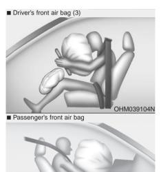
After complete inflation, the air bag immediately starts deflating, enabling the driver to maintain forward visibility and the ability to steer or operate other controls.
