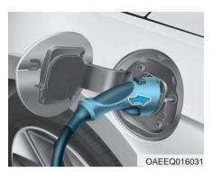
7. Hold the charging connector handle and connect it to the vehicle normal charging inlet. Push the connector until you hear a "clicking" sound. If the charging connector and charging terminal are not connected properly, this may cause a fire.
