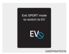
This message is displayed when [EV/HEV] button is pressed but it is impossible to switch from the HEV mode to EV mode because the SPORT mode is engaged.
