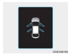
This warning is displayed indicating which door, or hood, or liftgate is open.
