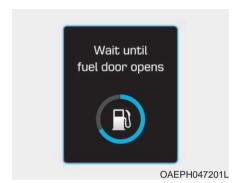
This message is displayed when you attempt to open the fuel filler door with the fuel tank pressurized. Wait until the fuel tank is depressurized.
