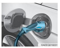
5. Hold the charging connector handle and connect it to the vehicle normal charging inlet. Push the connector until you hear a "clicking" sound. If the charging connector and charging terminal are not connected properly, this may cause a fire.
