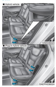
The high-voltage battery cooling duct is located on the left side of the rear seats.
