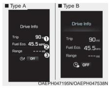
At the end of each driving cycle, the Driving Info message is displayed. This display shows the trip distance (1), average fuel economy (2), remaining vehicle range (3), and charging status (4).
