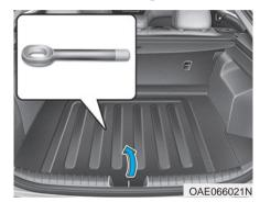
1. Open the liftgate, and take the towing hooks out from the tool case.
