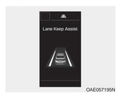
This mode displays the state of the Smart Cruise Control (SCC) and Lane Keeping Assist System (LKAS).
