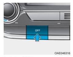
Push the OFF button to turn the climate control system off.
