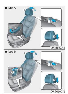
To reinstall the head restraint:
