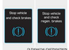
Either message is displayed when a failure occurs in the brake system. In this case, park the vehicle in a
