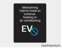
This message is displayed when the vehicle maintains the HEV mode to allow heating or air conditioning. The mode does not change when the driver presses the [EV/HEV] button to switch from the HEV mode to EV mode while the heating and cooling system is on and the coolant temperature is below 7 °F (-14 °C).
