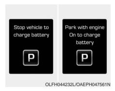
Either message is displayed when the hybrid battery power (SOC) level is low.
