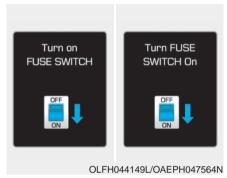
Either message is displayed if the fuse switch located on the fuse box under the steering wheel is OFF.
