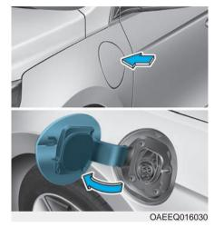
3. Press center edge of the charging door to open the charging door.
