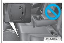
Never touch the safety plug. The safety plug is attached to high voltage hybrid battery system.
