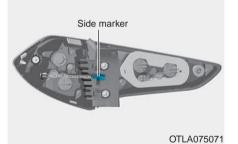
Remove the socket from the assembly by turning the socket counterclockwise until the tabs on the socket align with the slots on the assembly.
