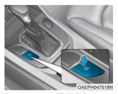
Pressing the [EV/HEV] button changes the plug-in hybrid system modes, between Electric (CD) mode and Hybrid (CS) mode.
