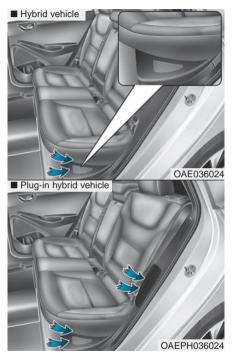
The high voltage battery cooling duct is located on the left side of the rear seats. The cooling duct cools down the high voltage battery.
