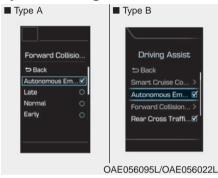
The driver can activate the AEB by placing the Engine Start/Stop button to the ON position and by selecting:
