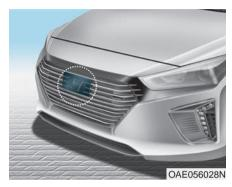
In order for the AEB system to operate properly, always make sure the radar sensor cover is clean and free of dirt, snow, and debris. Dirt, snow, or foreign substances on the lens may adversely affect the sensing performance of the sensor.
