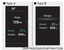
The range is the estimated distance the vehicle can be driven with the remaining fuel in the fuel tank (Gasoline) and high-voltage (hybrid) battery (Electric).
