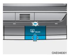
The defroster heats the window to remove frost, fog and thin ice from the interior and exterior of the rear window while the vehicle is in the ready ( ) mode.
