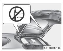
Do not hold the part (gas lifter) that supports the liftgate. Be aware that the deformation of the part may cause vehicle damage and a risk of safety accident.
