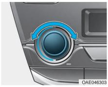
Turn the temperature control knob to the desired temperature. If the temperature is set to the lowest setting (Lo), the air conditioning system will operate continuously. After the interior has cooled sufficiently, adjust the knob to a higher temperature set point whenever possible. To turn the automatic operation off, select any button of the following:
