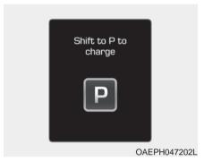
This message is displayed when the charging connector is plugged with the shift lever in R (Reverse), N (Neutral) or D (Drive). Move the shift lever to P (Park) and re-start the charging process.
