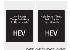
This message is displayed when the temperature of the high-voltage (hybrid) battery is too low or high. This warning message is to protect the battery and the hybrid system.
