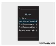
The driver can activate the Aux. Battery Saver+ function by placing the Engine Start/Stop button to the ON position and by selecting:
