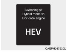
This message is displayed when the vehicle is automatically switched to the HEV mode to lubricate engine while the Engine Start/Stop button is in the ON position.
