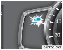
Check if the charging indicator light of the high voltage battery on the instrument cluster is turned ON. Charging is not done when the charging indicator lamp is OFF.
