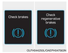
Either message is displayed when the brake performance is low or the regenerative brake does not work properly due to a failure in the brake system.
