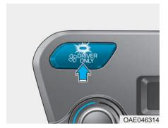
If you press the DRIVER ONLY button(\$\mathbf{S}^{DRIVER}\_{ONLY}) and the indicator light illuminates, air mostly blows in the direction of the driver's seat.
