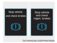
Either message is displayed when a failure occurs in the brake system. In this case, park the vehicle in a safe location and tow your vehicle to the nearest authorized HYUNDAI dealer and have the vehicle inspected.
