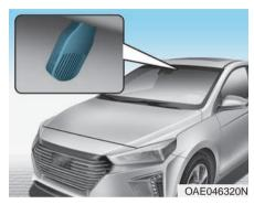
Auto defogging system reduces the possibility of fogging up the inside of the windshield by automatically sensing the moisture on inside the windshield.
