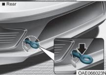
If towing is necessary, we recommend you to have it done by an authorized HYUNDAI dealer or a commercial tow truck service. If a towing service is not available in an emergency, your vehicle may be temporarily towed using a cable or chain secured to the emergency towing hook at the rear of the vehicle.
