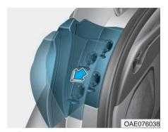
4. Remove the rear combination lamp assembly from the body of the vehicle.
