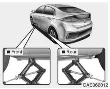
Insert the jack handle into the jack and turn it clockwise, raising the vehicle until the tire clears the ground. Make sure the vehicle is stable on the jack.
