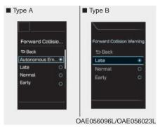
The driver can select the initial warning activation time on the LCD display. Go to the 'User Settings → Driving Assist → FCW (Fwd. Collision Warning) → Late/Normal/Early'.
