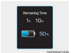
This message is displayed to notify the remaining time to fully charge the battery.
