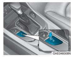
When the Engine Start/Stop button is in the ON position or when the vehicle is in the ready ( ) mode, press the heated steering wheel button to warm the steering wheel. The indicator on the button will illuminate.
