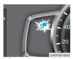
Check if the charging indicator light of the high voltage battery on the instrument cluster is turned ON. Charging is not done when the charging indicator lamp is OFF.
