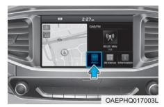
Press [PHEV] on the [Home] screen or the [All menus] screen and the menus related to plug-in hybrid ([ECO Driving], [Energy Information], [EV Range], [Charging Settings], [Charging Stations]) are displayed.
