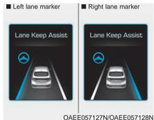
A visual warning appears on the cluster LCD display. Either the left lane marker or the right lane marker in the cluster LCD display will blink depending on which direction the vehicle is veering.
