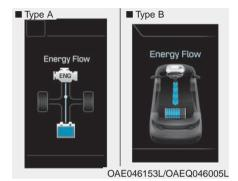
When the vehicle is stopped, the high-voltage battery is charged up by the engine.
