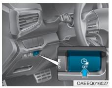
• If you press the scheduled charging deactivation (ﷺ) button to immediately charge the battery, charging must be initiated 3 minutes after the charging cable has been connected.
