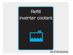
This message is displayed when the inverter coolant is nearly empty.
