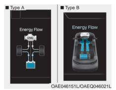
Both the motor and the engine power are used to drive the vehicle.
