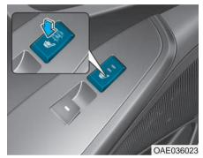
While the vehicle is in the ready ( ) mode, push either of the switches to warm the rear seat.
