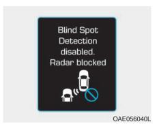
Blind Spot Detection disabled. Radar blocked.
