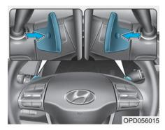
The paddle shifter is functional when the shift lever is in the D (Drive) or S (Sport) position, or the manual shift mode.
