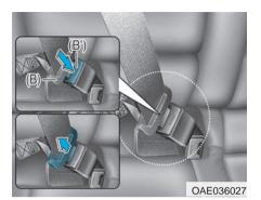
Pull the tongue plate (B) and insert it into the buckle (B') until an audible "click" is heard, indicating the latch is locked. Make sure the belt is not twisted.
