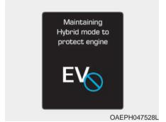
This message is displayed when the [EV/HEV] button is pressed but it is impossible to switch from the HEV mode to EV mode due to engine lubrication.
