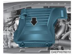
The air cleaner filter can be cleaned for inspection using compressed air. Do not attempt to wash or to rinse it, as water will damage the filter.
