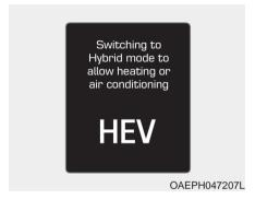
This message is displayed when the vehicle automatically switches to HEV mode to allow heating or air conditioning. It is when the coolant temperature is low (below 7 °F (-14 °C)) and the driver turns on the heating or cooling system.
