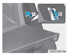
When the vehicle is under regular maintenance, make sure to separate the (-) cable before maintenance.
