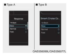
The sensitivity of vehicle speed when following the front vehicle to maintain the set distance can be adjusted on the LCD display.
