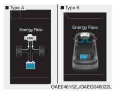
Only the engine power is used to drive the vehicle.
