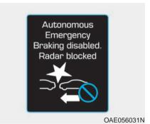
Autonomous Emergency Braking disabled. Radar blocked
