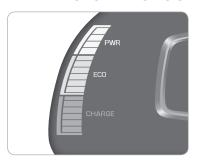
The hybrid system gauge indicates whether the current driving condition is fuel efficient or not.
