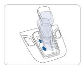
Shift the lever from D into the manual gate to activate manual shift mode. Manual shift mode is a recalibrated automatic mode that will hold gears longer and downshift at higher RPM for a more dynamic driving style. Gasoline engine will be engaged more frequently.
