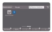
Press the NAV button in the navigation head unit. Select the [Destination] tab and find a destination by using the [Destination] menu.
