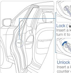
Lock ( 🕞 ) Insert a key into the hole and turn it to the lock ( $\square$ ) position.
