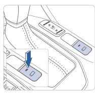
This parking support system displays an all-around view of the vehicle when parking. Press the switch to activate/ deactivate the system.
