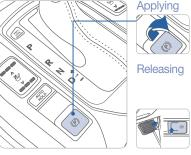
Stop the vehicle then pull the EPB switch.
