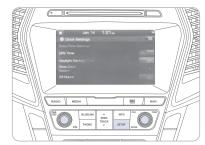
Press SETUP button (A) and press the on-screen CLOCK button. Enable GPS Time and the time and
