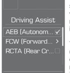
The Autonomous Emergency Braking (AEB) system is designed to detect and monitor the vehicle ahead or detect a pedestrian in the roadway and warn the driver if a collision is imminent.
