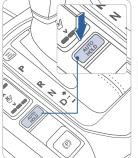
The Auto Hold feature assists in steep hill areas. It holds the brake until the accelerator pedal is pressed.
