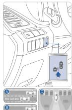
The BSD system sensor senses the rear side territory of the vehicle and provides information to the driver. Press the BSD switch. If vehicle speed exceeds 9mph the system will activate. Press the switch again to deactivate the system.
