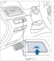
The Lane Departure Warning System detects the lane on the road and warns the driver if the vehicle leaves the lane when the vehicle speed is over 37mph.
